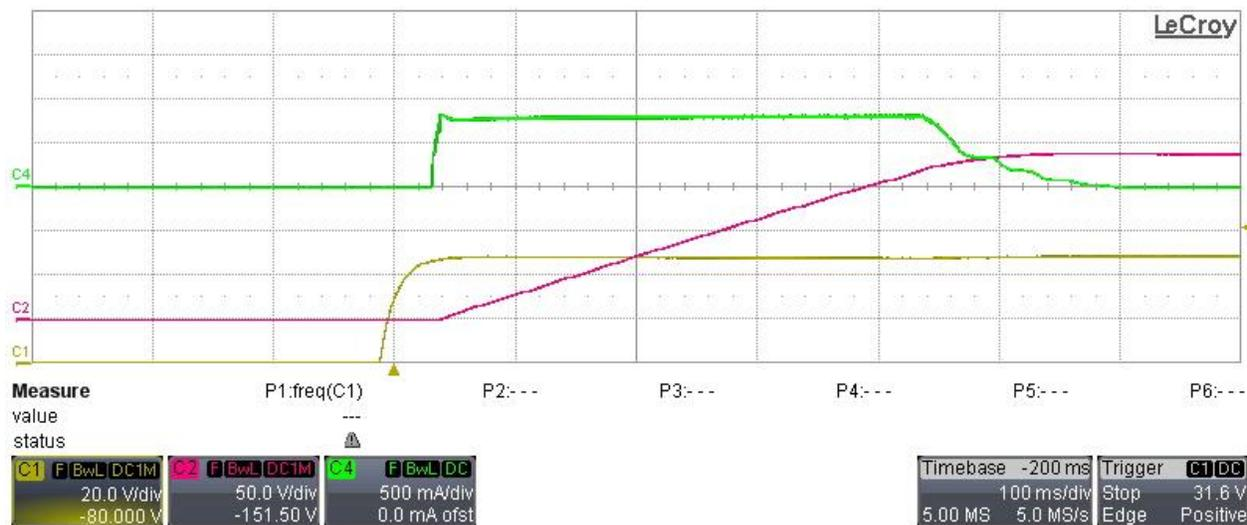
**Same condition as above but with a constant-voltage electronic load, se to 180V:**
