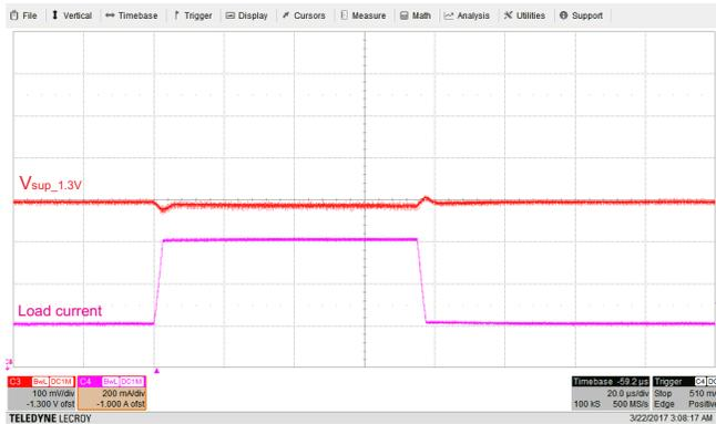
Figure 12.  $V_{sup\_1.3V}$  Transient Response (14  $V_{IN}$ , 400- to 800-mA Load Step, Measured at J6)
