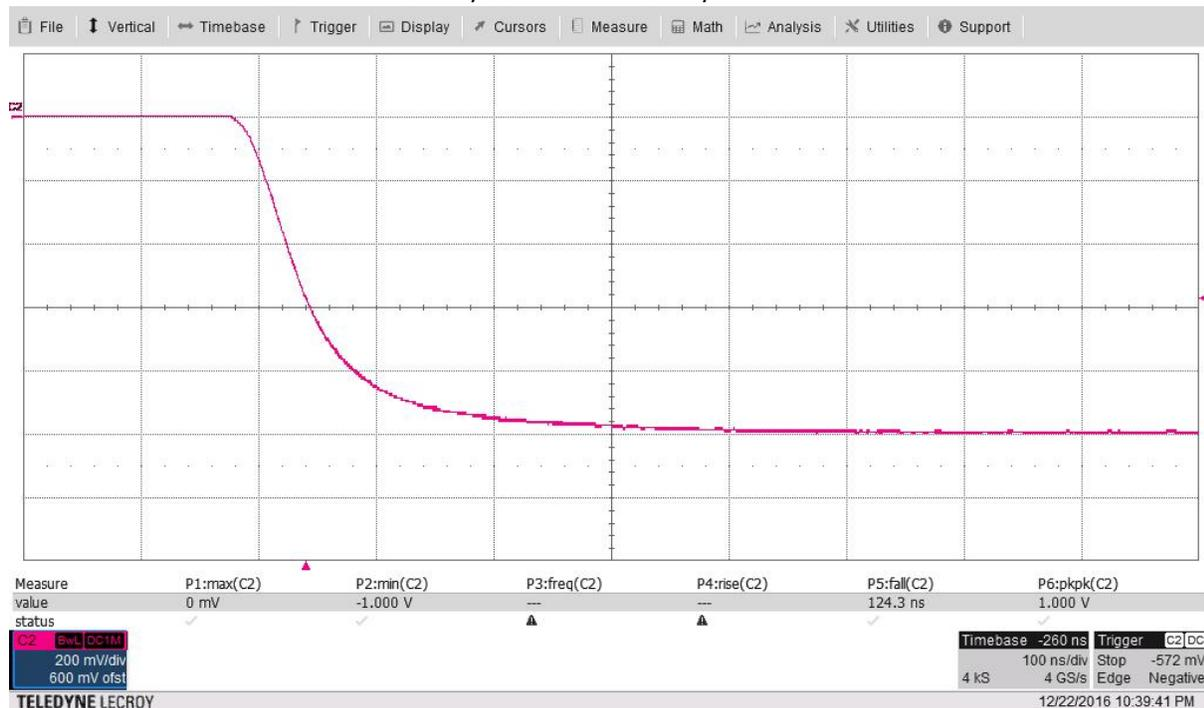
R528 now at 75 ohms sets speed of turn on and can be changed to get faster or slower turn on.
