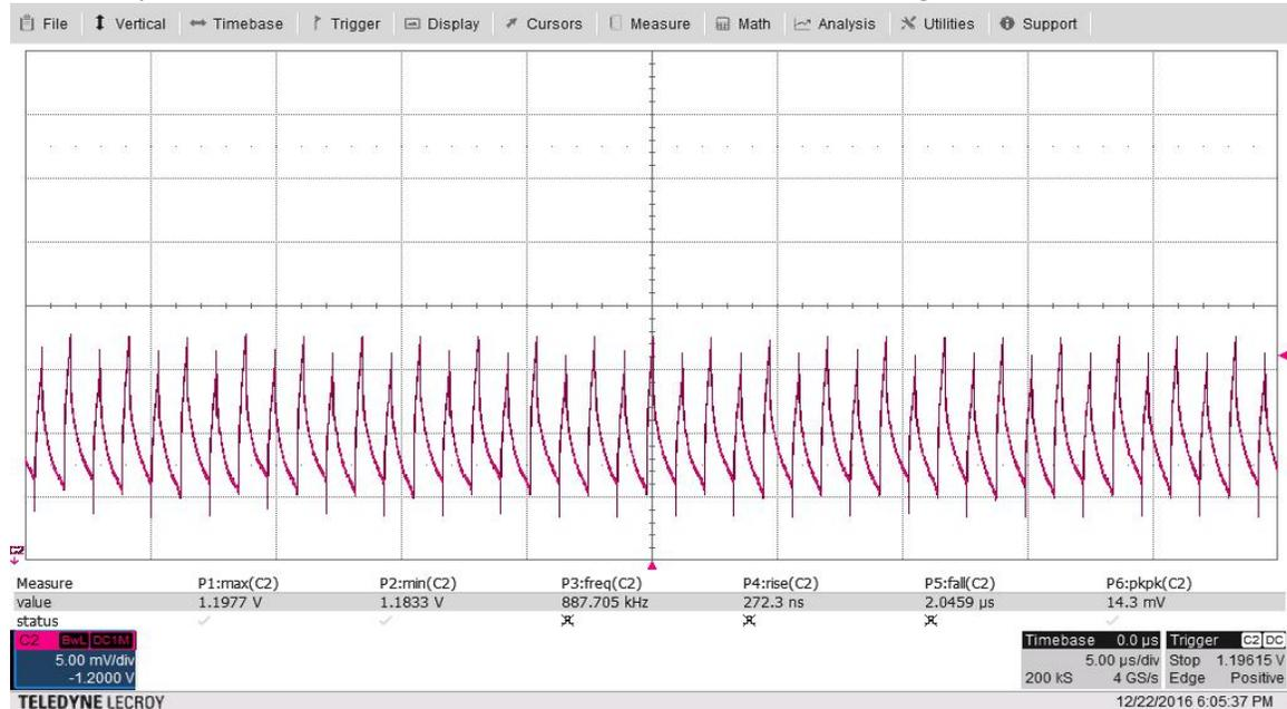
Now up to 14.3mV p-p No evidence of hard saturation of inductors:
