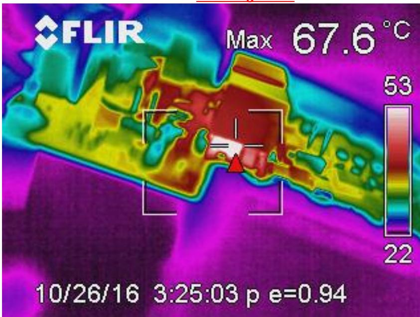
With fan and inductors on top GUI reading 4 degrees C hotter than what I can capture on edges.
