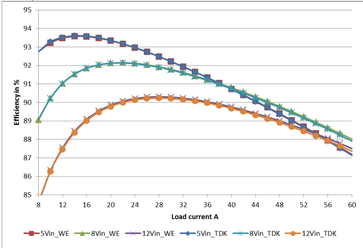
Conclusion: Efficiency variations are very small between the two type of inductors with greatest variation at max 60A load and 12Vin: Here efficiency for model t1 using TDK is 87.362% vs. model t2 with Wurth at 87.498% for a 0.138% difference. Model t3 with Wurth came in at 87.415%, or only 0.053% better than the TDK model.
