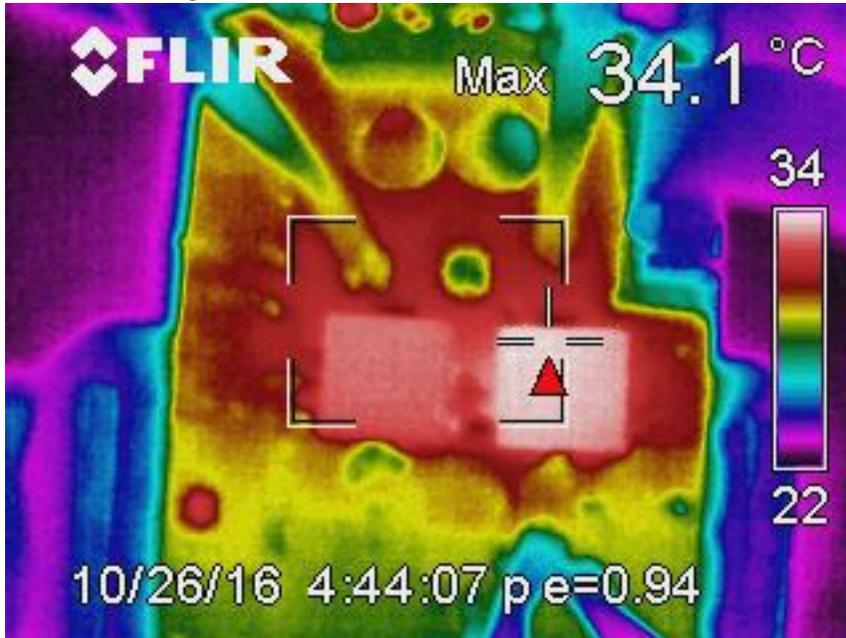
Master inductor core about 2 degrees hotter than slave core
