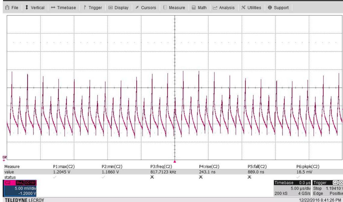
18.5mV p-p: **Based upon this ~70A saturation threshold, max recommended steady state load with TDK inductors is 50A.**
