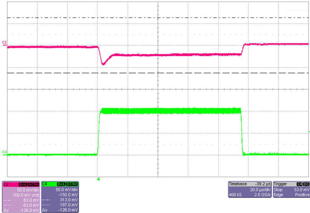
Figure 3-9. Transient Response (5 V<sub>IN</sub>, 0-A to 1-A Load Step)
