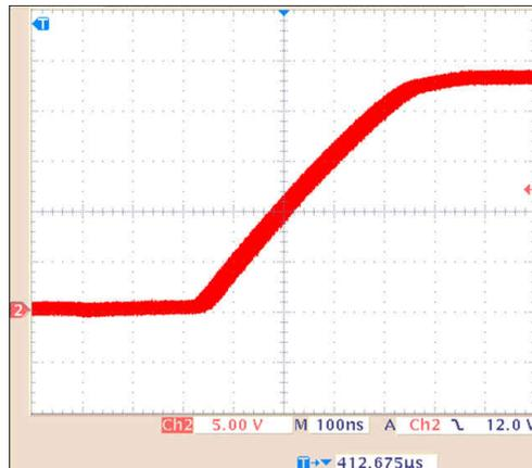
Figure 3-10. Master Cycle Jitter
