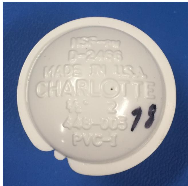
**Figure 5. Cap With Hole for Test Leak Apparatus**
