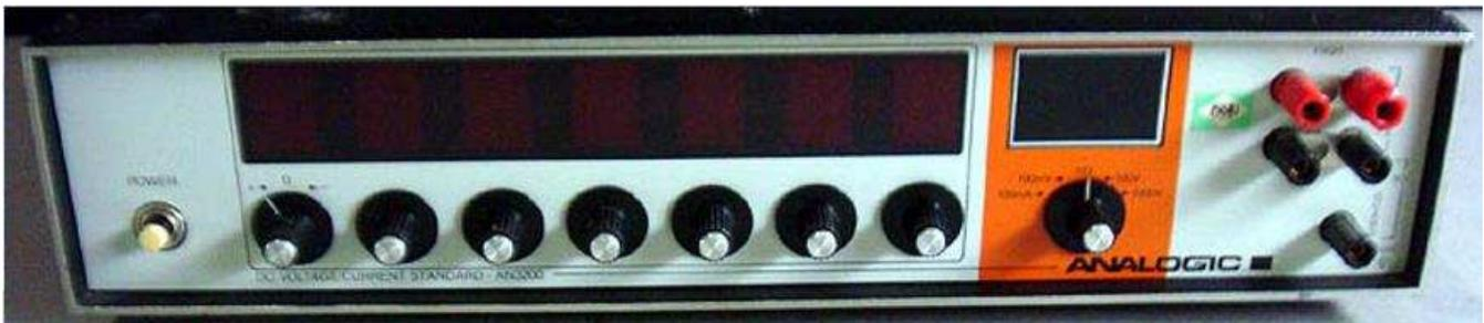
Figure 23. Analogic AN3200 DC Voltage Calibrator
