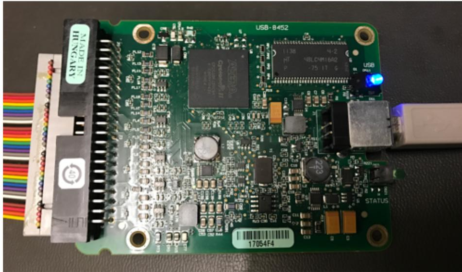
**Figure 25. NI USB-8452 Interface Board**
