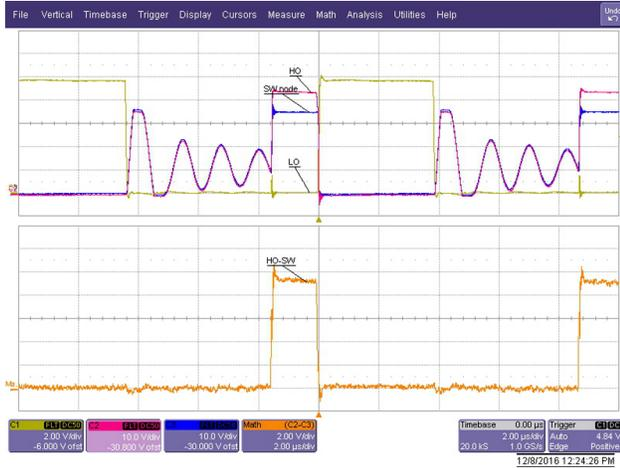
**Figure 65. Switching Waveforms With Adaptive Dead-Time Settings**
