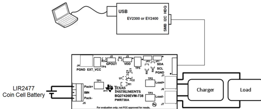
Figure 8. LIR2477 Characterization Setup
