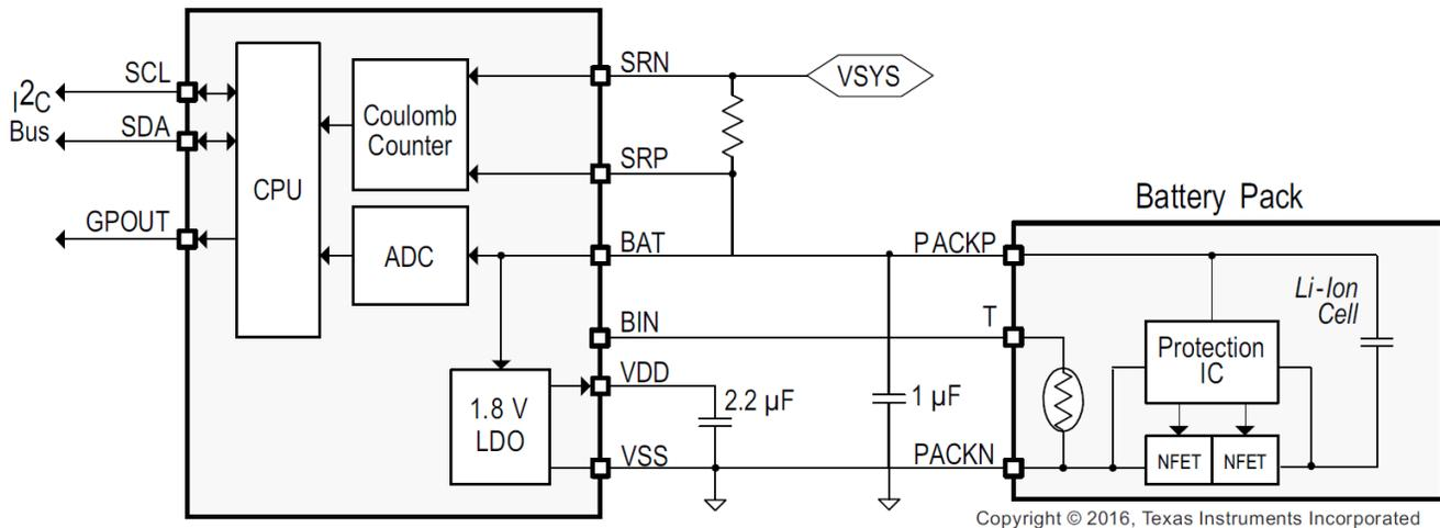
**Figure 4. bq27426 Functional Block Diagram**
