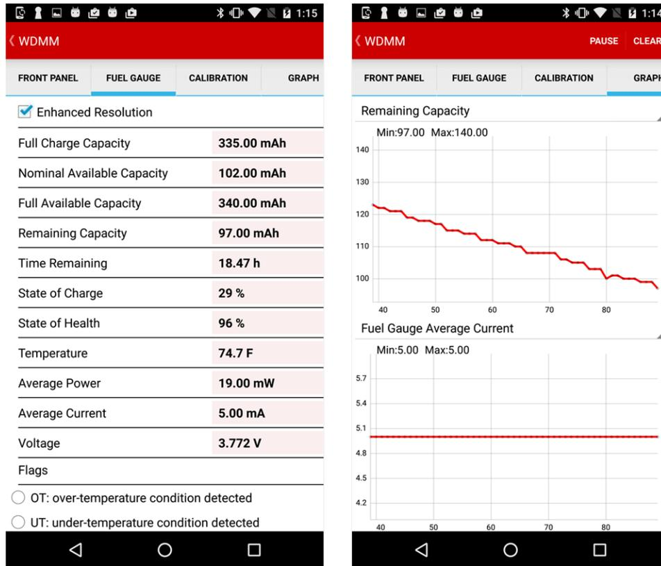
Figure 7. TIDC-01012 Fuel Gauge Snapshots
