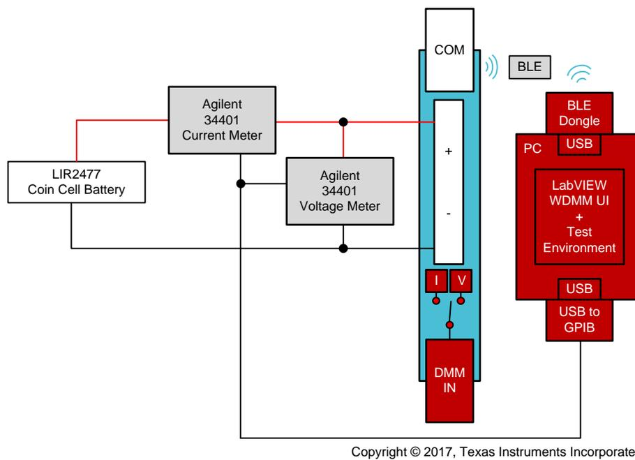
**Figure 9. Fuel Gauge Test Setup**
