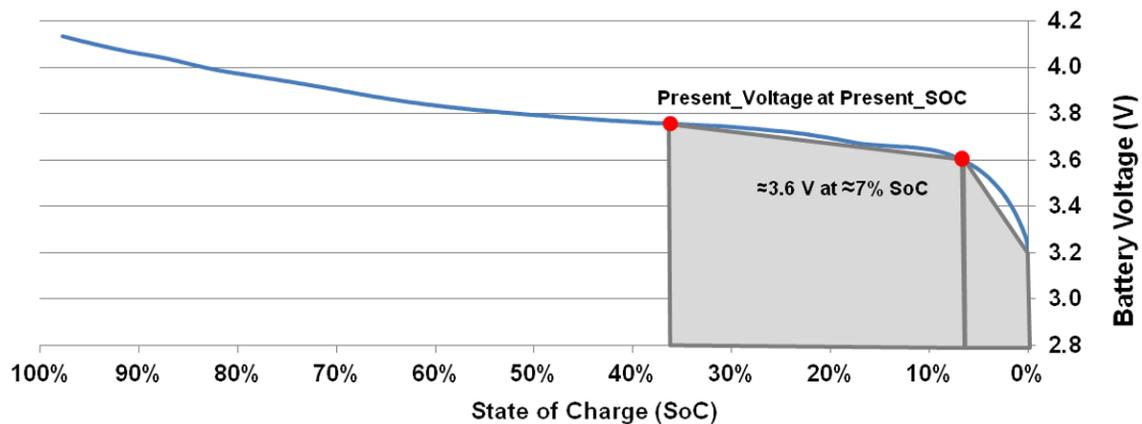
**Figure 6. Remaining Average Voltage Estimation**
