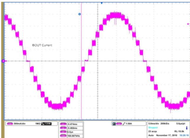
**Figure 19. 40 V, 1k PPS 1/8 Microstep Mode Current**
