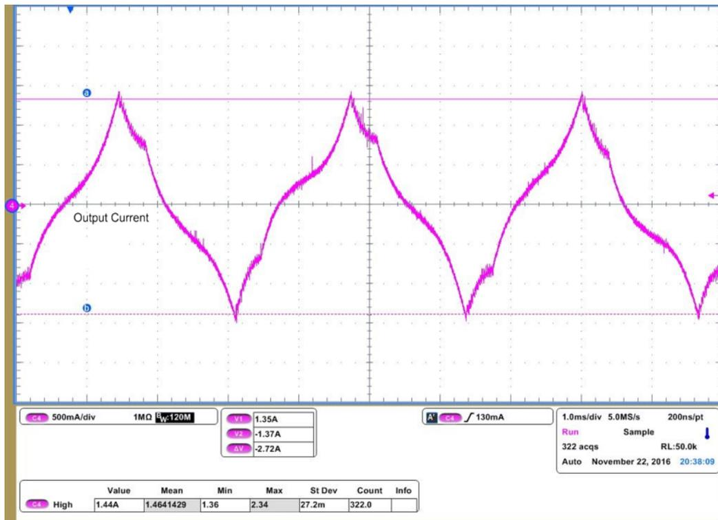
Figure 15. 40k PPS, 24 V, 2-A Full-Scale, 1/32 Microstep Mode
