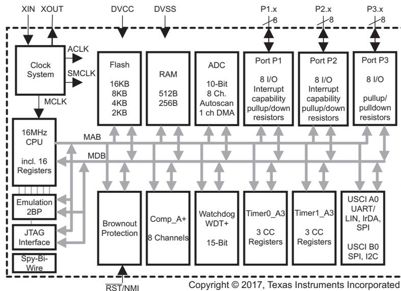
**Figure 2. MSP430G2553 Functional Block Diagram**
