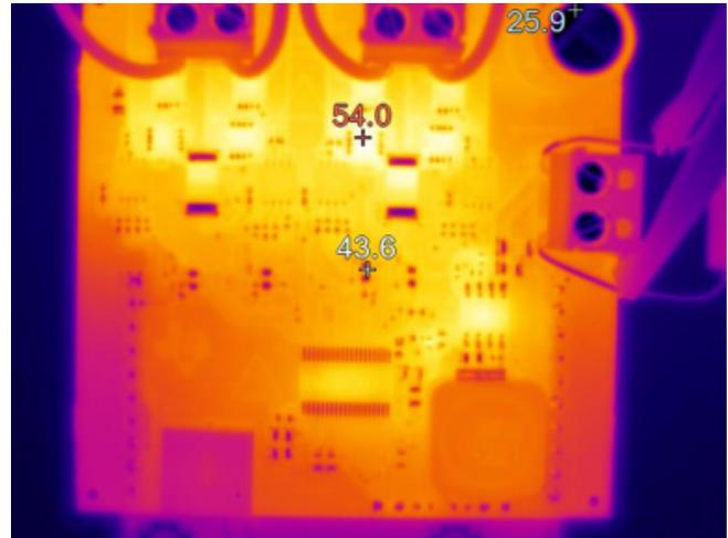
Figure 22. 50 V, 1k PPS 1/8 Microstep Mode Thermal Image
