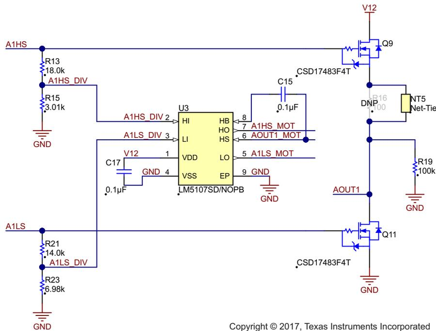
**Figure 9. Interface from DRV8711 to High-Voltage FETs**
