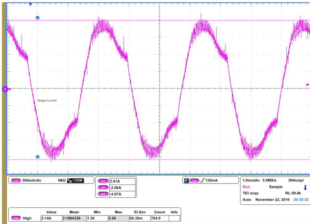
Figure 16. 40k PPS, 48 V, 2-A Full-Scale, 1/32 Microstep Mode
