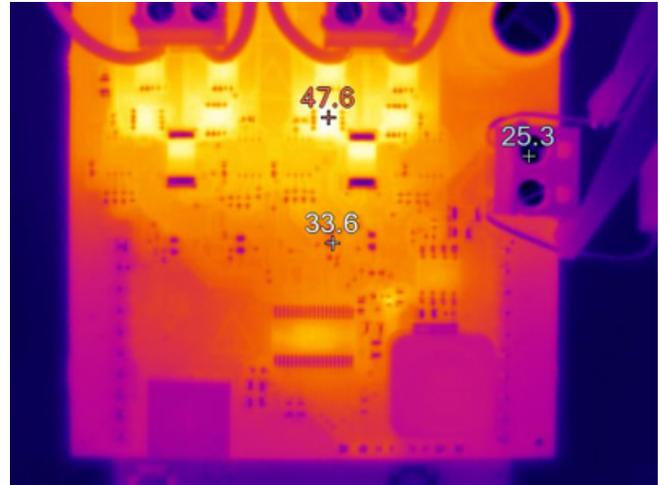
**Figure 18. 30 V, 1k PPS 1/8 Microstep Mode Thermal Image**
