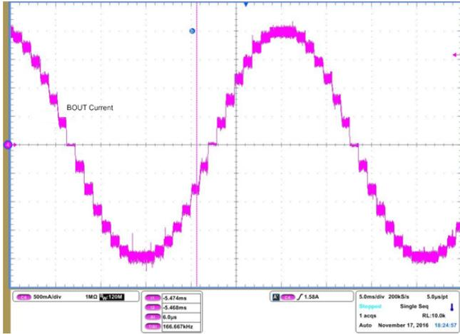
**Figure 17. 30 V, 1k PPS 1/8 Microstep Mode Current**
