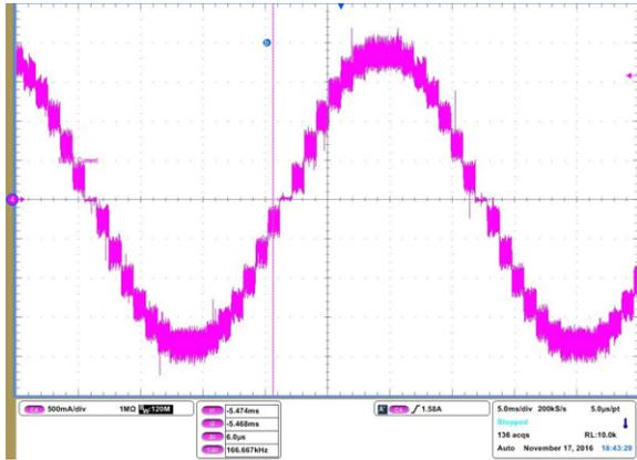
**Figure 25. 70 V, 1k PPS 1/8 Microstep Mode Current**
