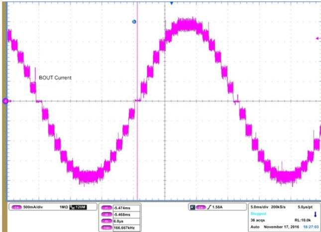
Figure 21. 50 V, 1k PPS 1/8 Microstep Mode Current
