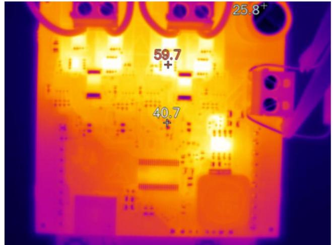
**Figure 26. 70 V, 1k PPS 1/8 Microstep Mode Thermal Image**
