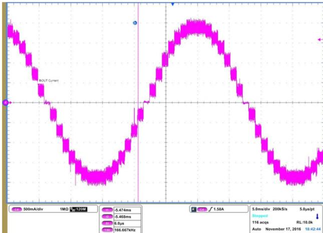
Figure 23. 60 V, 1k PPS 1/8 Microstep Mode Current
