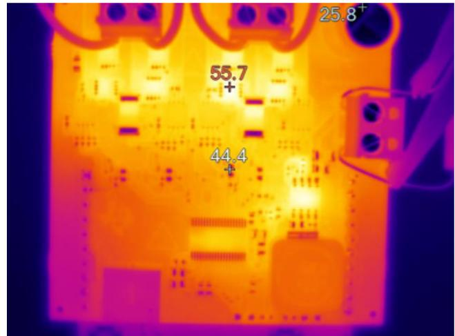
Figure 24. 60 V, 1k PPS 1/8 Microstep Mode Thermal Image
