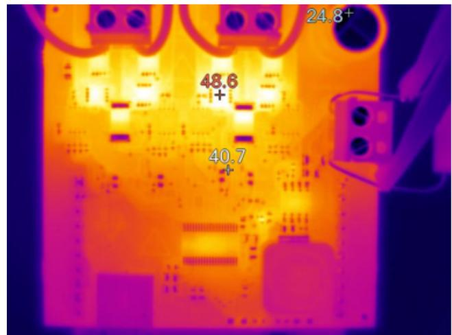
**Figure 20. 40 V, 1k PPS 1/8 Microstep Mode Thermal Image**
