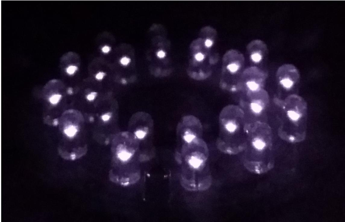
**Figure 18. IR LED Illuminated Ring**
