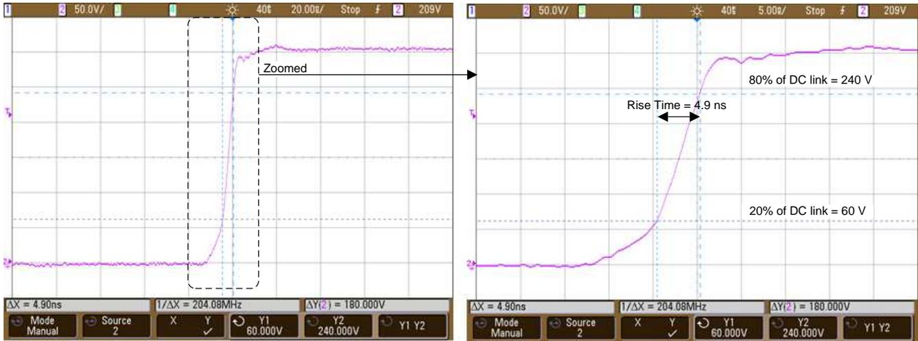
**Figure 27. Turn-off Transition at 1.6 A**
