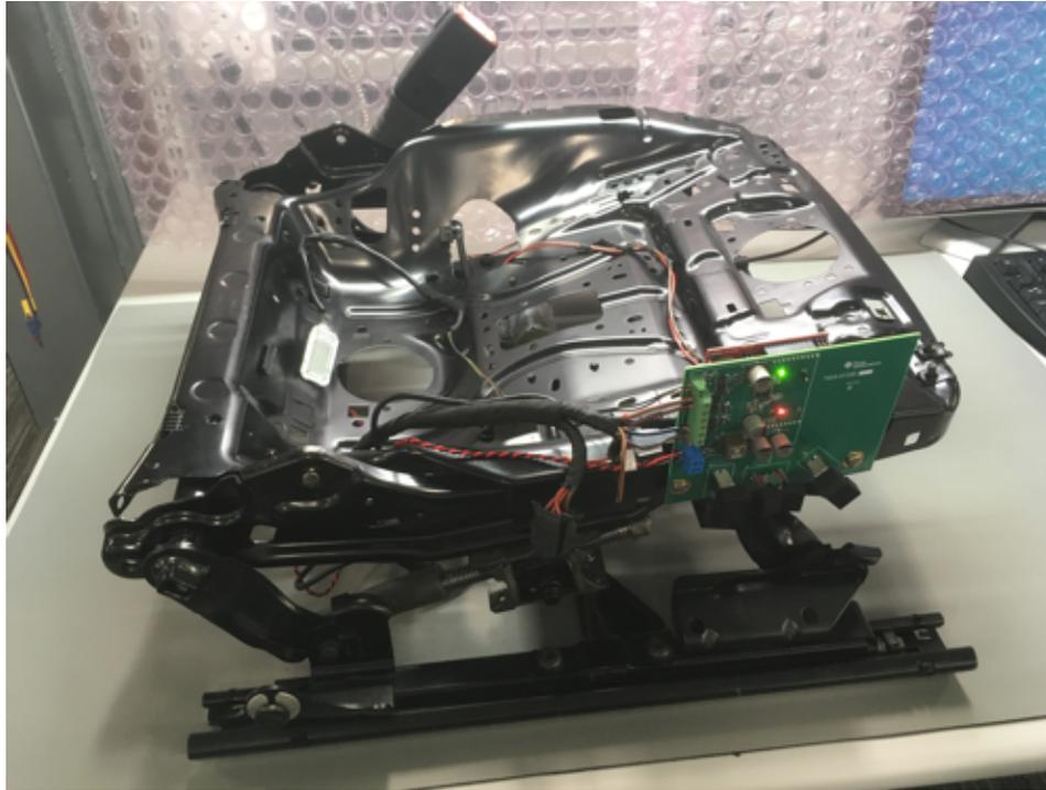
**Figure 21. TIDA-01330 Board Mounted on Test Hardware**
