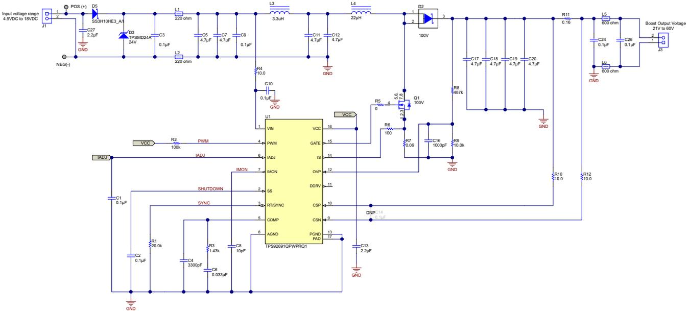
Figure 5. TPS92691-Q1 LED Driver in Boost Configuration
