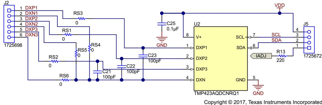
Figure 6. Temperature Sensing Section
