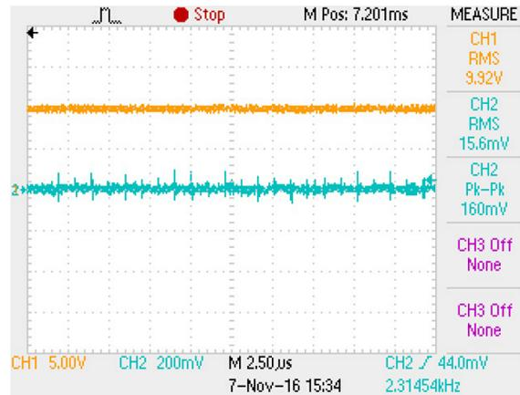
Figure 21. Boost Regulator Output
