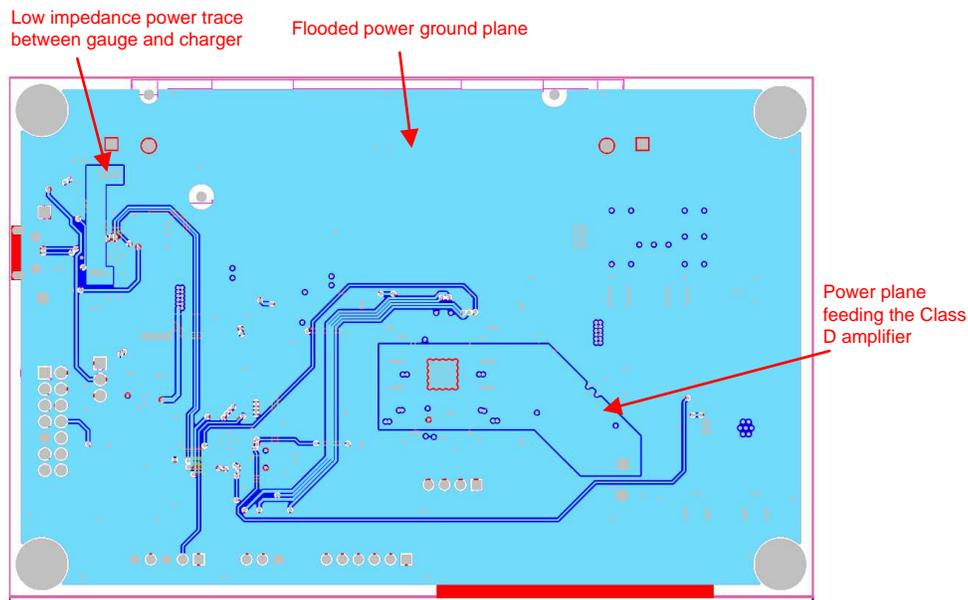
Figure 30. PCB Inner Layer 3 (Power and Ground Plane Layer) Layout
