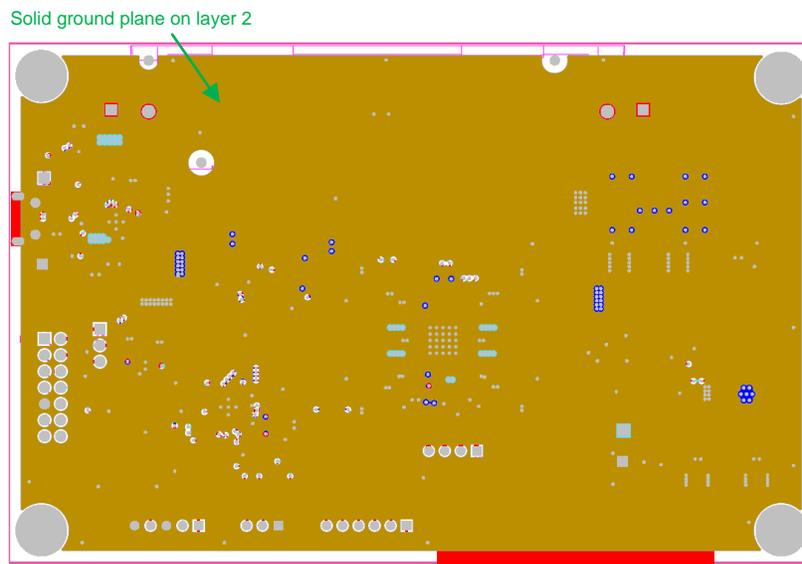
**Figure 29. PCB Inner Layer 2 (Ground Plane Layer) Layout**
