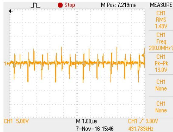
Figure 23. Class D Output Differential
