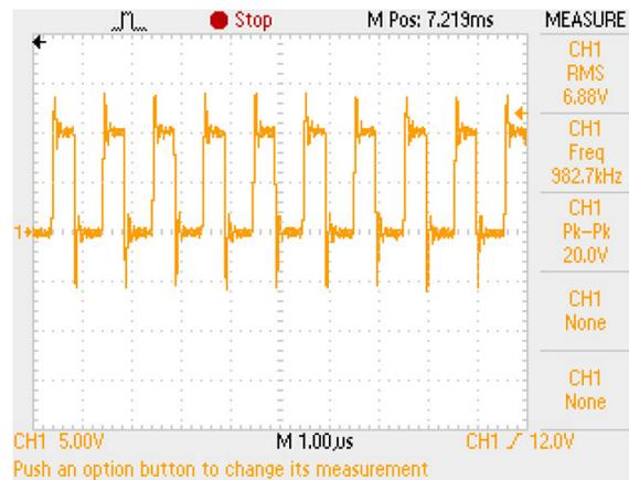
Figure 22. Class D Output Ground Reference
