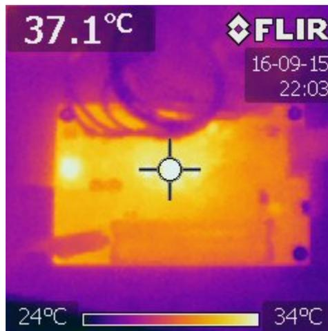
Figure 27. Boost and Class D Thermal
