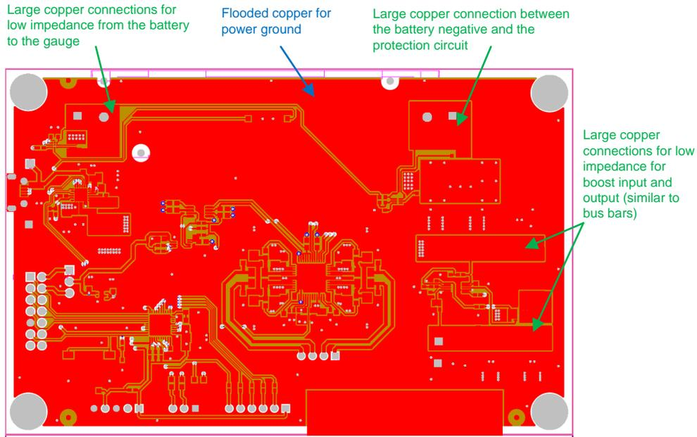
**Figure 28. PCB Top Layer 1 (Component Layer) Layout**
