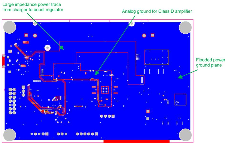
Figure 31. PCB Bottom Layer 4 (Analog Ground and Ground Plane Layer) Layout
