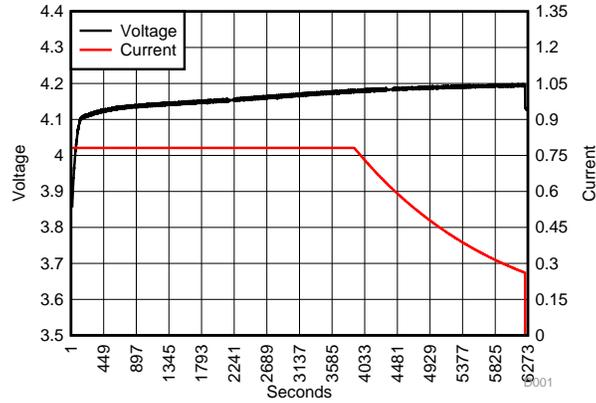
**Figure 25. Charge Cycle Plot**
