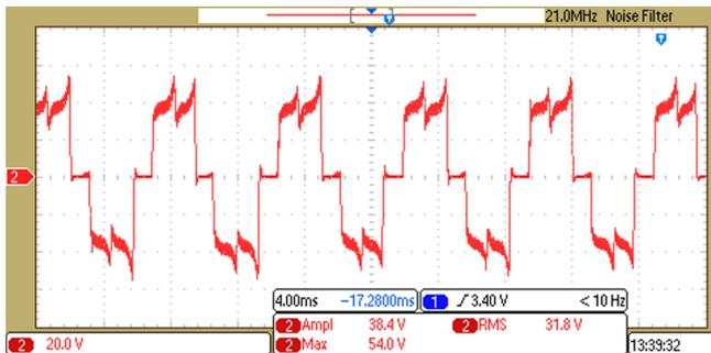
**Figure 33. Load Test Results at 18-V DC Input, 31.8- $A_{RMS}$  Winding Current, 90% Duty Cycle**
