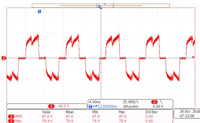
Figure 37. Load Test Results at 18-V DC Input, 48.2-A<sub>RMS</sub> Winding Current, 95% Duty Cycle
