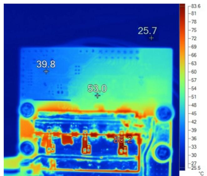
Figure 38. Thermal Image at 18-V DC Input, 48.2-A<sub>RMS</sub> Winding Current, 95% Duty Cycle
