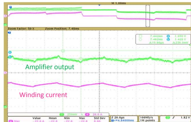
Figure 44. Current Sense Amplifier Output at Negative Winding Current
