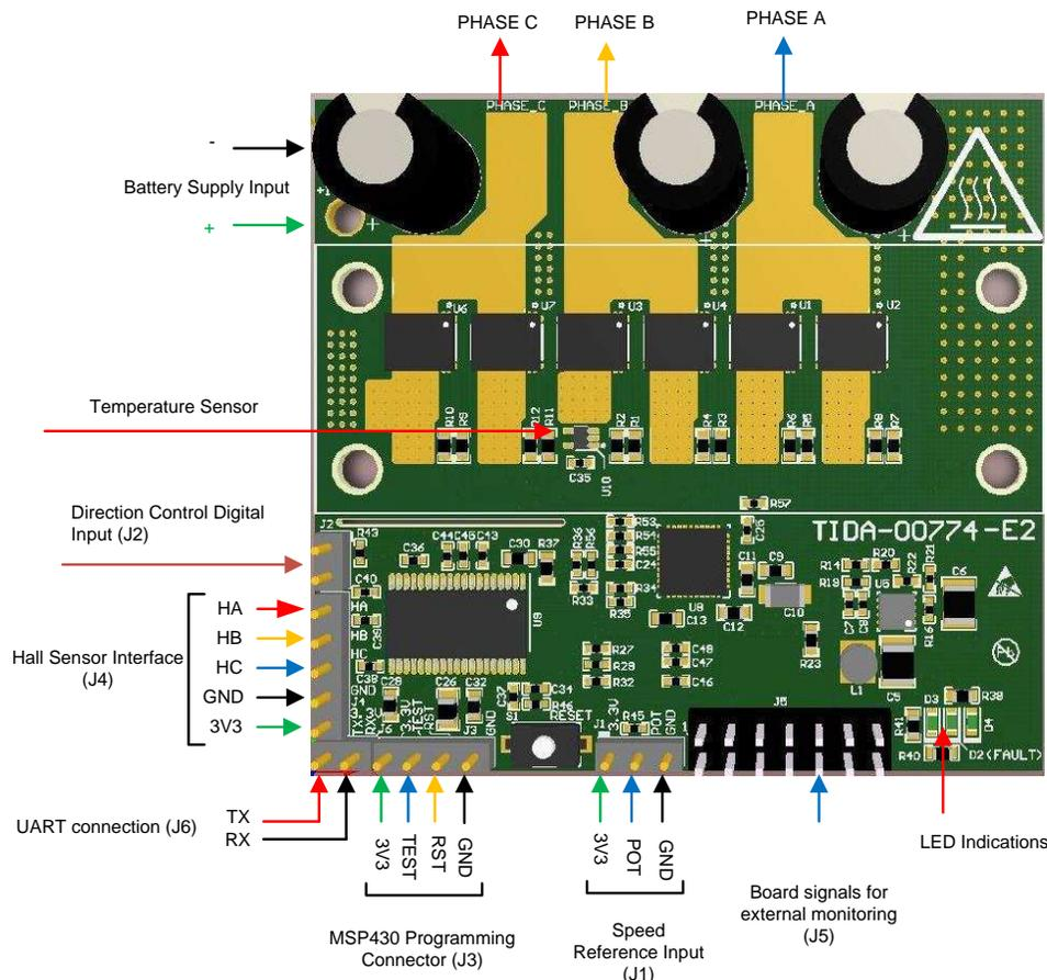
Figure 15. TIDA-00774 PCB Connectors
