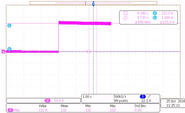
Figure 53. 120-A Peak Current in Motor Winding During Motor Stall
