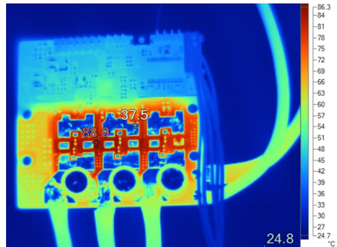
**Figure 34. Thermal Image at 18-V DC Input, 31.8- $A_{RMS}$  Winding Current, 90% Duty Cycle**
