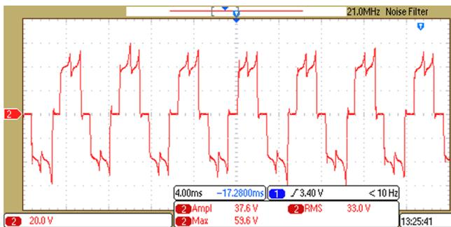
**Figure 31. Load Test Results at 18-V DC Input, 33- $A_{RMS}$  Winding Current, 100% Duty Cycle**
