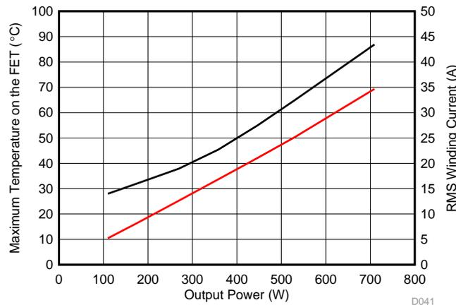
Figure 41. Maximum FET Temperature at Different Power Levels
