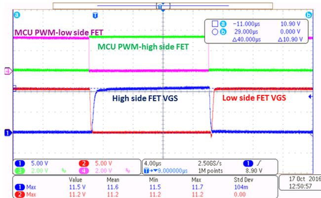
Figure 19. Low-Side and High-Side Gate Drive Voltage at 18-V DC
