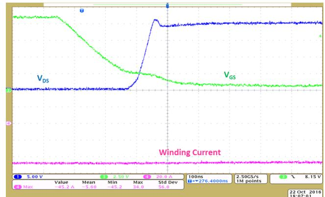
Figure 24. Turnoff—Low-Side VGS and VDS at 45-A Winding Current
