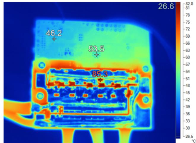
Figure 36. Thermal Image at 18-V DC Input, 42-A<sub>RMS</sub> Winding Current, 100% Duty Cycle
