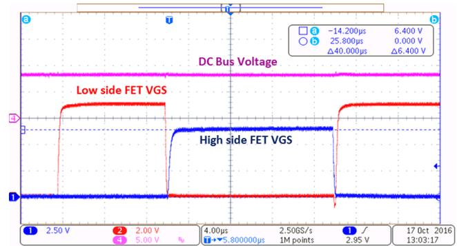
Figure 20. High-Side and Low-Side Gate Drive Voltage at 8-V DC
