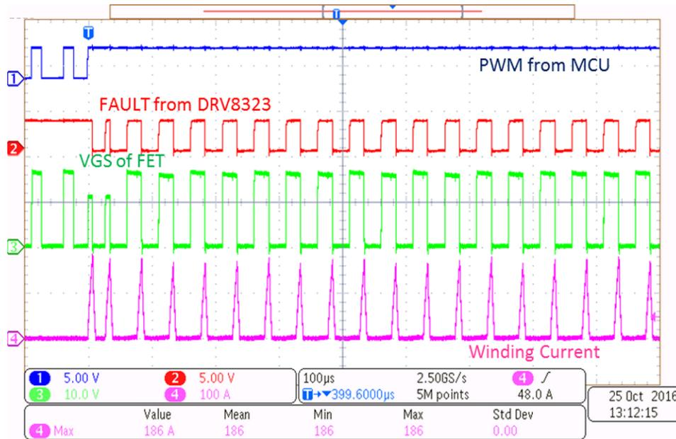
Figure 49. Cycle-by-cycle Overcurrent Protection With Inverter Output Shorted
