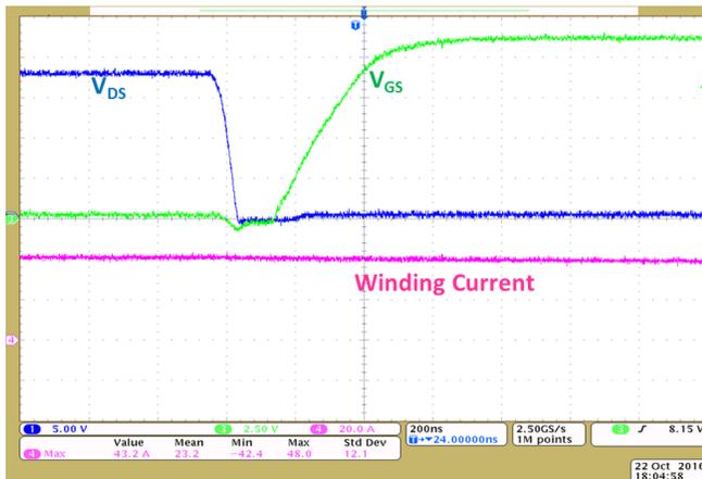
Figure 23. Turnon—Low-Side VGS and VDS at 43-A Winding Current
