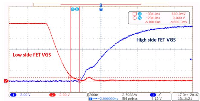
Figure 22. Dead Time at Low-Side VGS Trailing Edge
