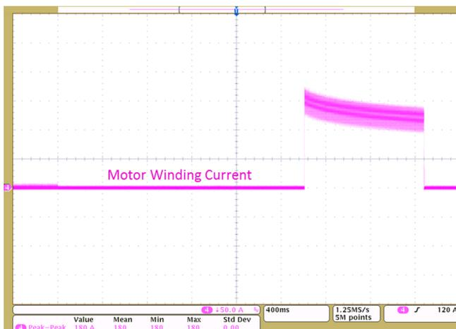
Figure 55. 160-A Peak Current in Motor Winding During Motor Stall
