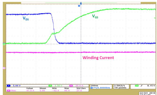
Figure 26. Turnon—High-Side VGS and VDS at 42-A Winding Current
