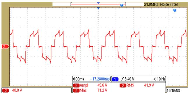
Figure 35. Load Test Results at 18-V DC Input, 42-A<sub>RMS</sub> Winding Current, 100% Duty Cycle
