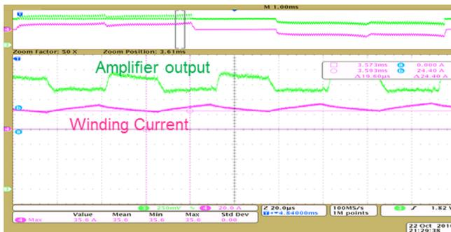
Figure 43. Current Sense Amplifier Output at Positive Winding Current
