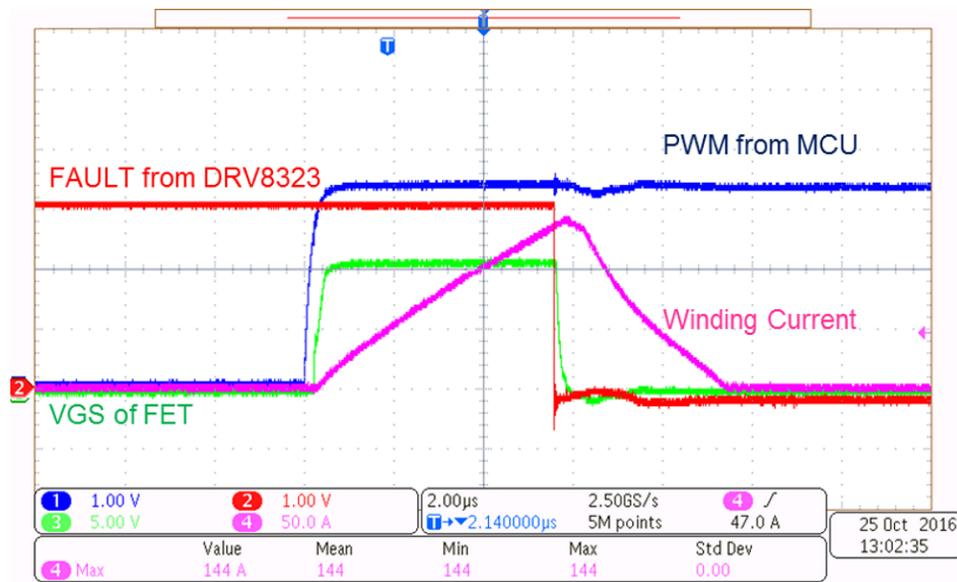
Figure 52. Overcurrent Latch Protection With Inverter Output Shorted
