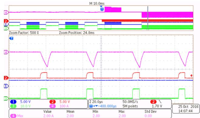
Figure 47. Zoomed View of Cycle-by-Cycle Overcurrent Protection With Motor Stall
