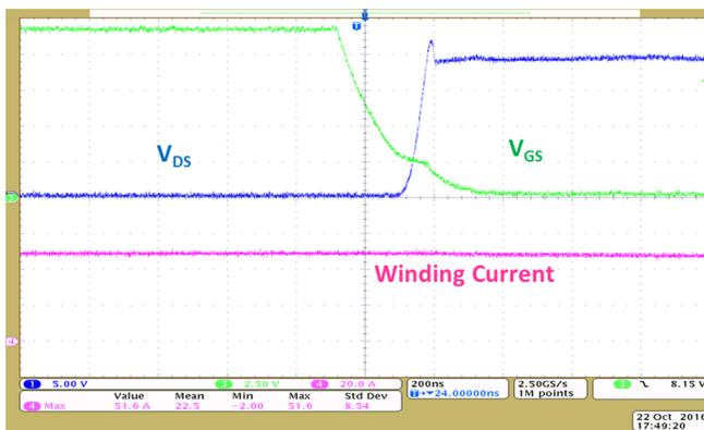
Figure 25. Turnoff—High-Side VGS and VDS at 52-A Winding Current
