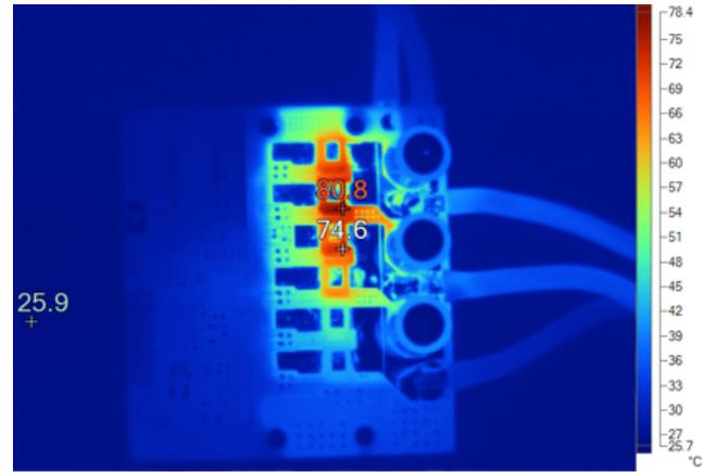
Figure 54. Thermal Image of Board After 3 Seconds With 120-A Peak Current in Motor Winding
