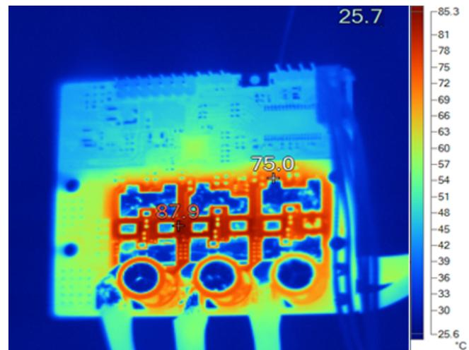
**Figure 32. Thermal Image at 18-V DC Input, 33- $A_{RMS}$  Winding Current, 100% Duty Cycle**
