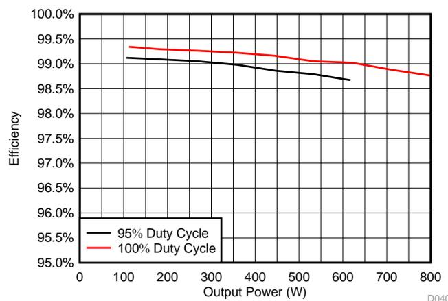
**Figure 40. Inverter Efficiency versus Output Power With Heat Sink**
