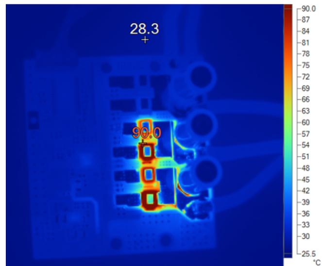
Figure 56. Thermal Image of Board After 1 Second With 160-A Peak Current in Motor Winding
