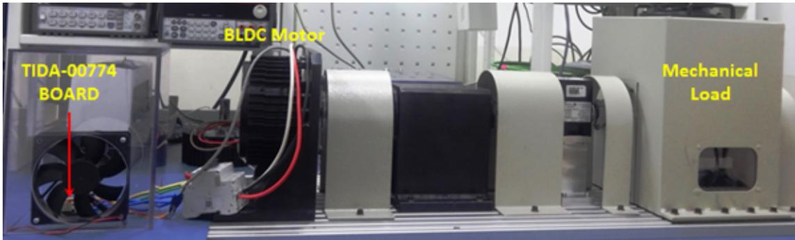
Figure 17. Board and Motor Test Setup
