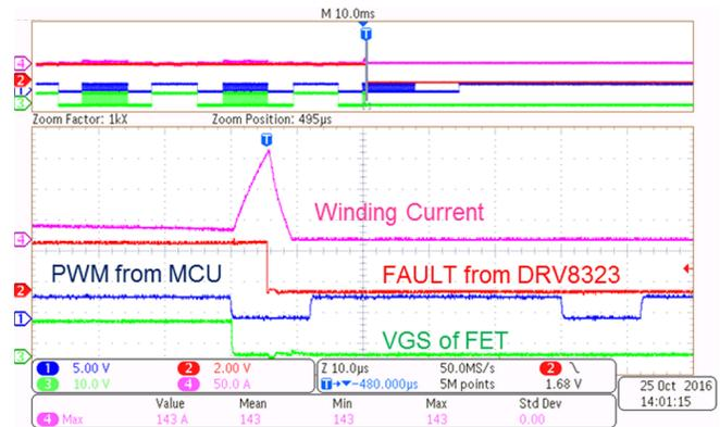
Figure 50. Overcurrent Latch Protection With Motor Stall by VDS Sensing
