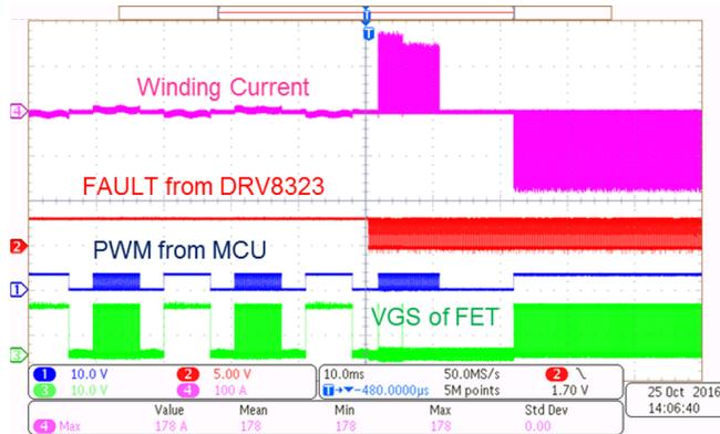
Figure 46. Cycle-by-Cycle Overcurrent Protection With Motor Stall
