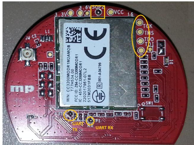
Figure 2. CC3200-MODULE Programming Interface
