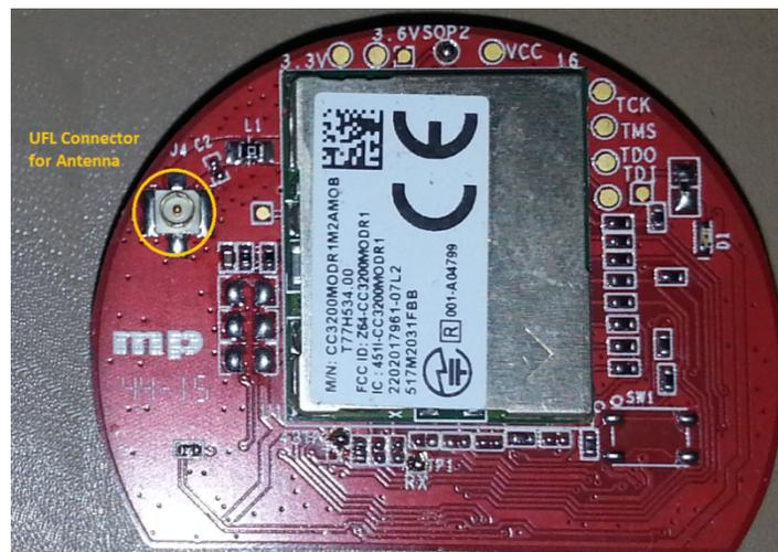
**Figure 1. CC3200-MODULE UFL Connector Location**
