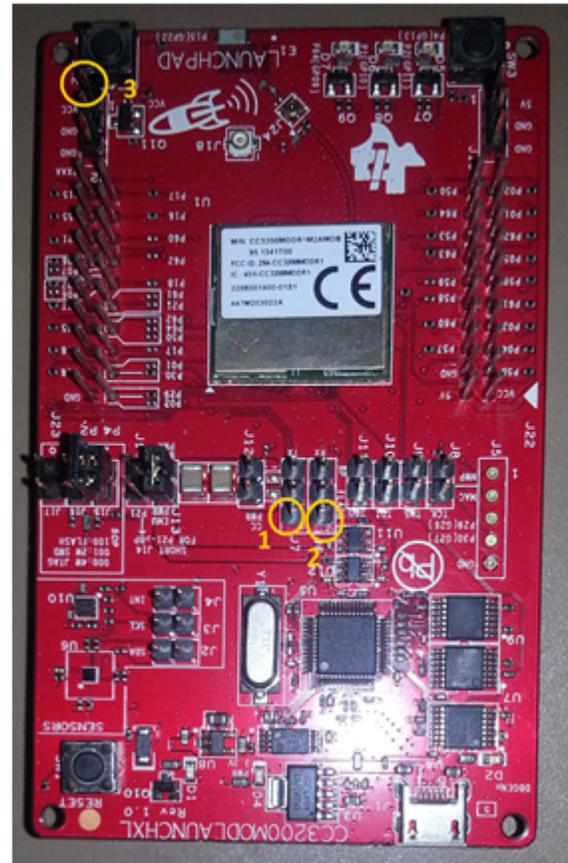
**Figure 10. CC3200-MODULE to CC3200-LAUNCHXL Connection Locations**
