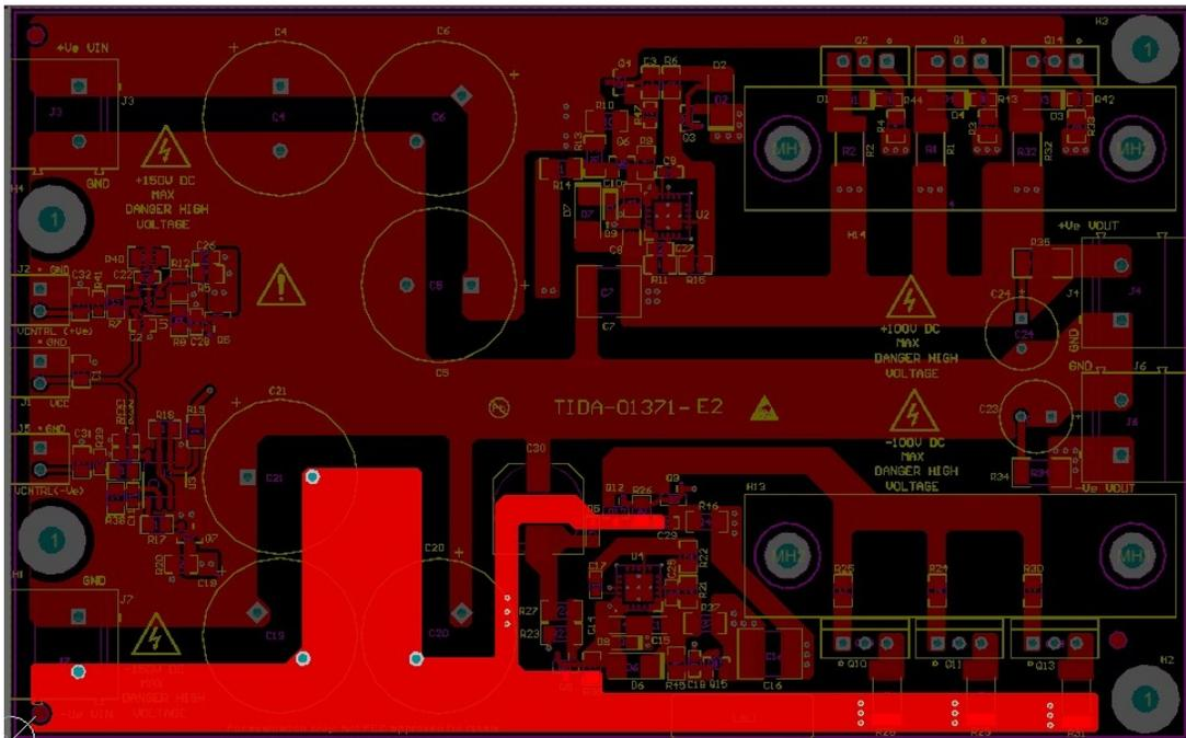
Figure 38. Layout Showing  $-VIN$  Plane
