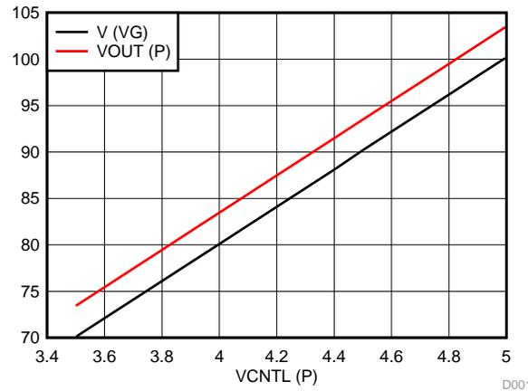
Figure 24. Transfer Characteristics for Positive Regulator (at Input Voltage of 110 V)
