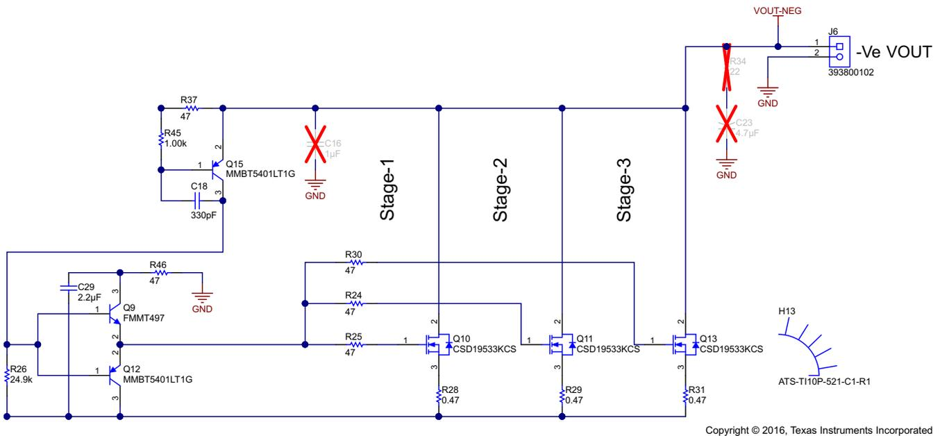
Figure 17. Current Scaling Using N-Channel MOSFETs (Negative Regulator)
