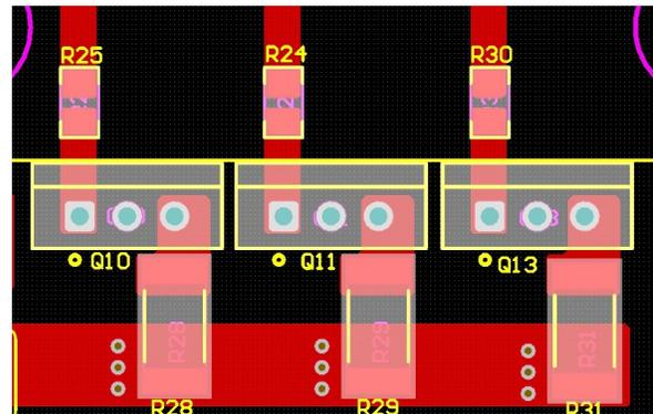
Figure 33. Placements for MOSFETs and Adjacent Circuits for Negative Regulator
