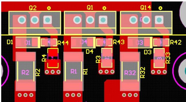
Figure 32. Placements for MOSFETs and Adjacent Circuits for Positive Regulator
