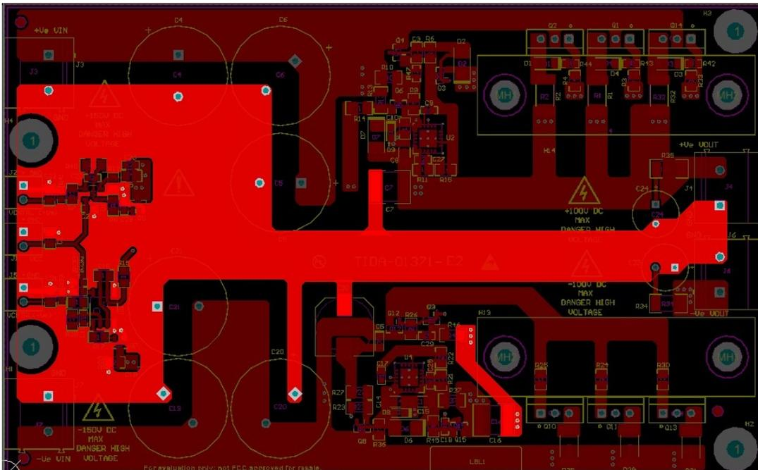
Figure 37. Layout Showing GND Plane
