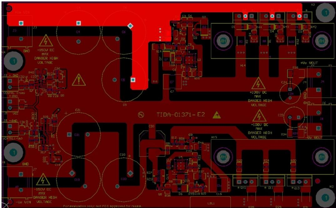
Figure 36. Layout Showing +VIN Plane
