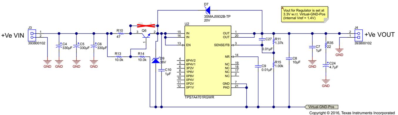
Figure 9. Positive Regulator Using TPS7A4701 and Virtual Ground
