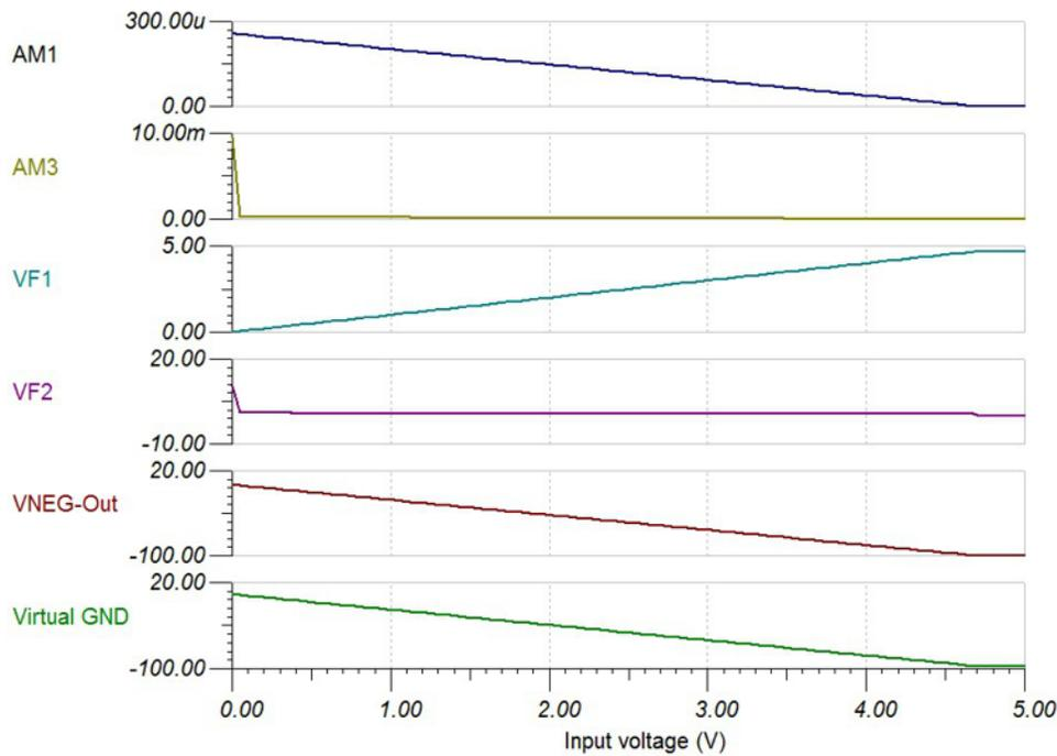
Figure 14. DC Transfer Characteristics: Control Voltage versus Negative  $V_{OUT}$  and Virtual Ground
