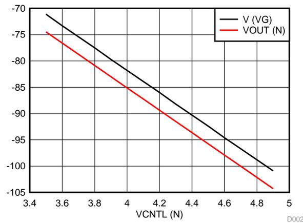
Figure 25. Transfer Characteristics for Negative Regulator (at Input Voltage of -110 V)
