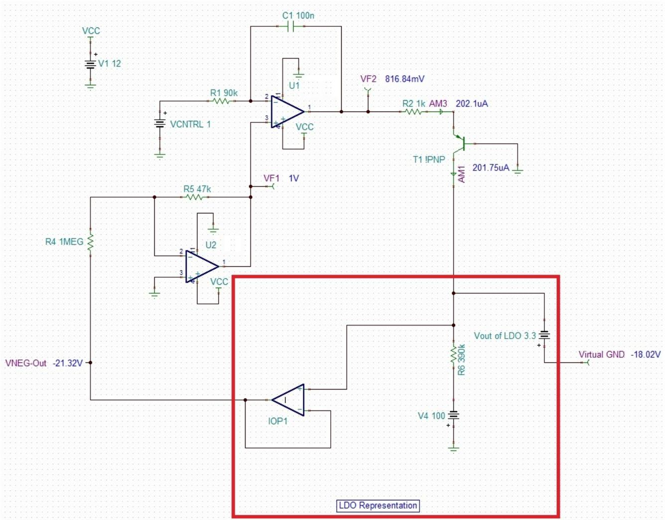
Figure 13. TINA Simulation for DC Amplifier for Floating Regulator Ground (Negative Regulator)
