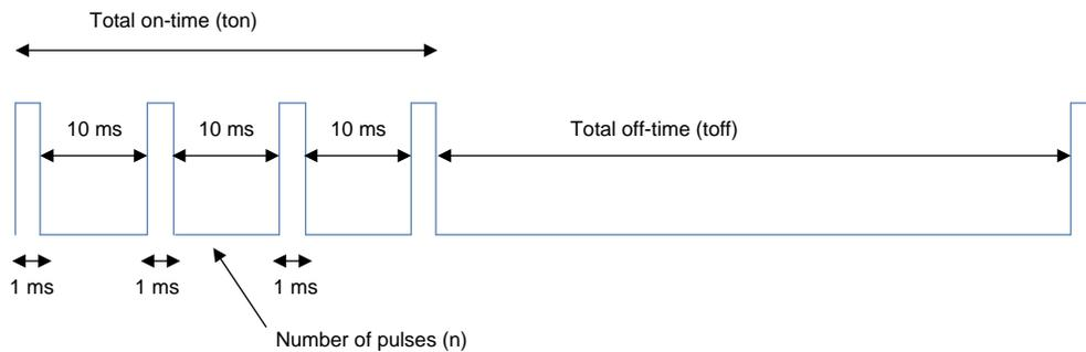
Figure 3. Elastography—Driving Waveform for Ultrasound Transducers
