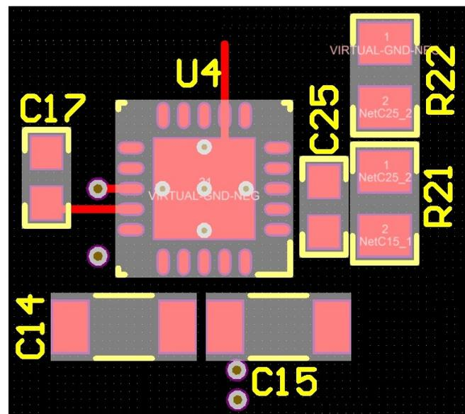
**Figure 31. Placements for TPS7A3301 and Adjacent Components**
