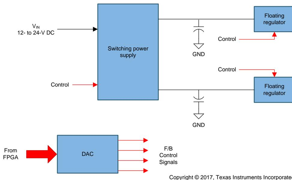
**Figure 1. Typical Power Supply Scheme in Medical Ultrasound Application**
