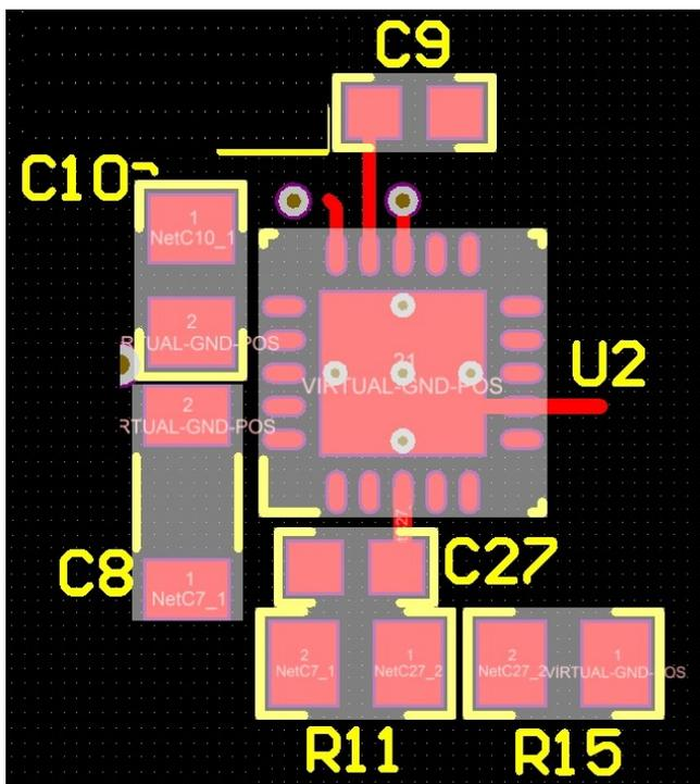
**Figure 30. Placements for TPS7A4701 and Adjacent Components**
