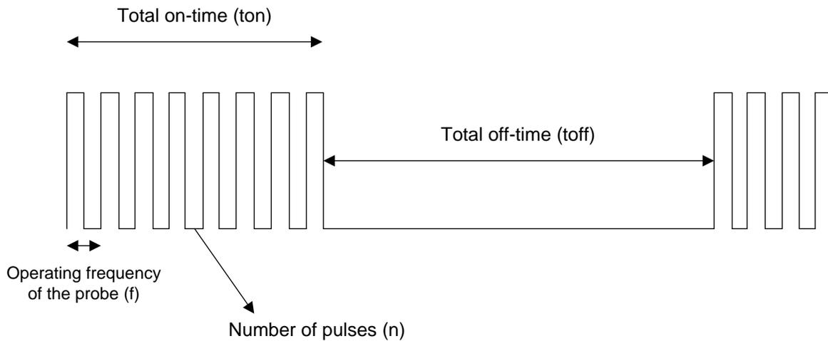
**Figure 2. Standard Driving Waveform for Ultrasound Transducers**
