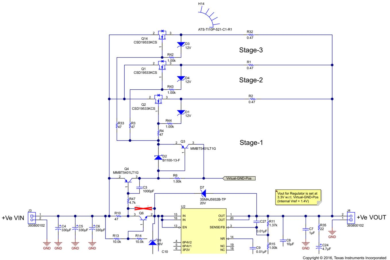
Figure 10. Current Scaling Using N-Channel MOSFETs (Positive Regulator)
