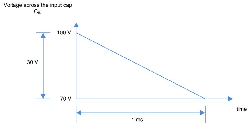
**Figure 20. Current Delivering Ability of Input Capacitor**
