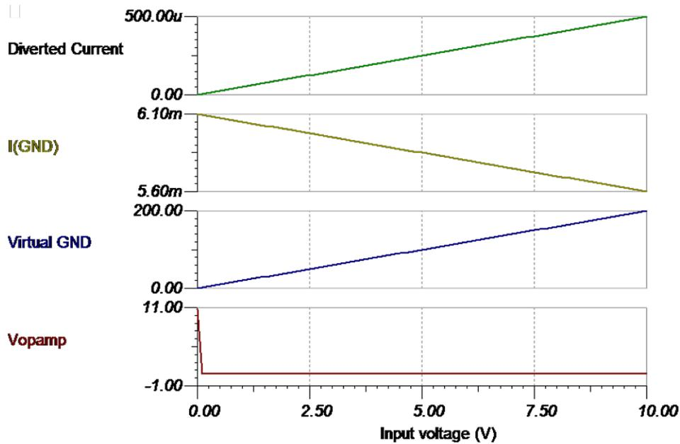
Figure 6. DC Transfer Characteristics: Control Voltage versus Virtual Ground
