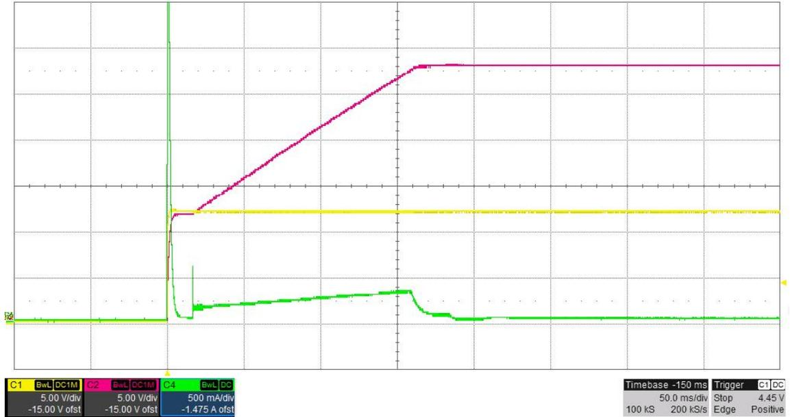
The photo below shows the output voltage startup waveform after the application of 12V in with the 28V output loaded to 0.10A. The input current is shown in green. (5V/DIV, 500mA/DIV, 50ms/DIV)
