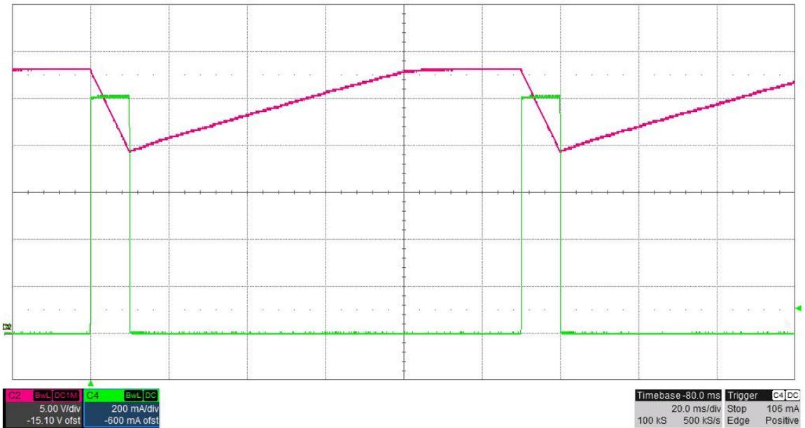
The photo below shows the output voltage when the load current is stepped between 0A and 1.25A.
