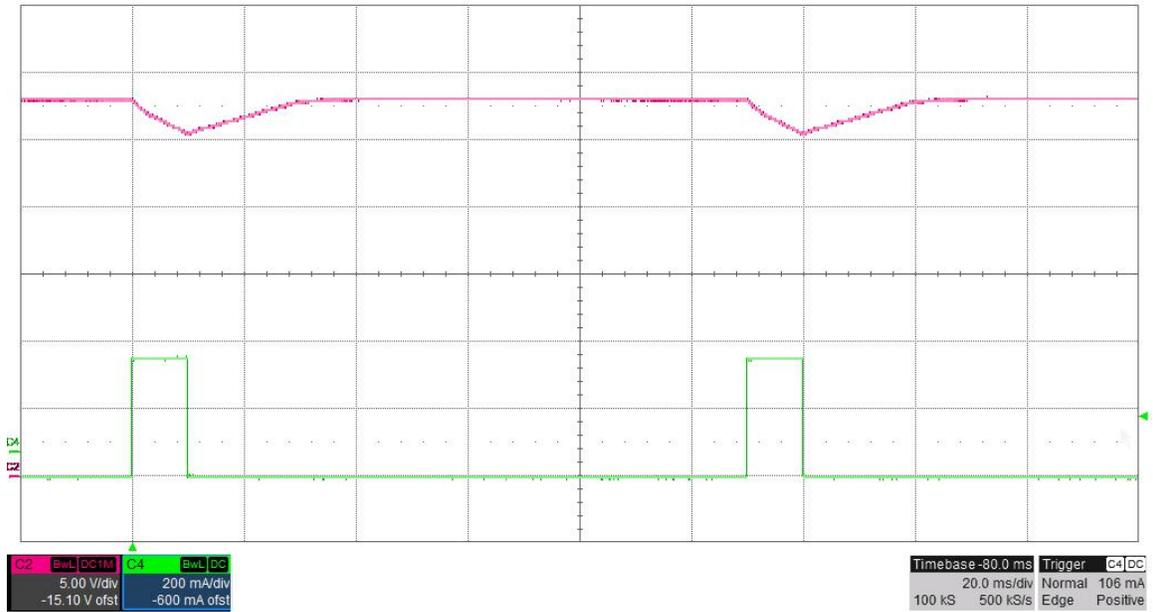
The photo below shows the output voltage when the load current is stepped between 0A and 0.5A.
