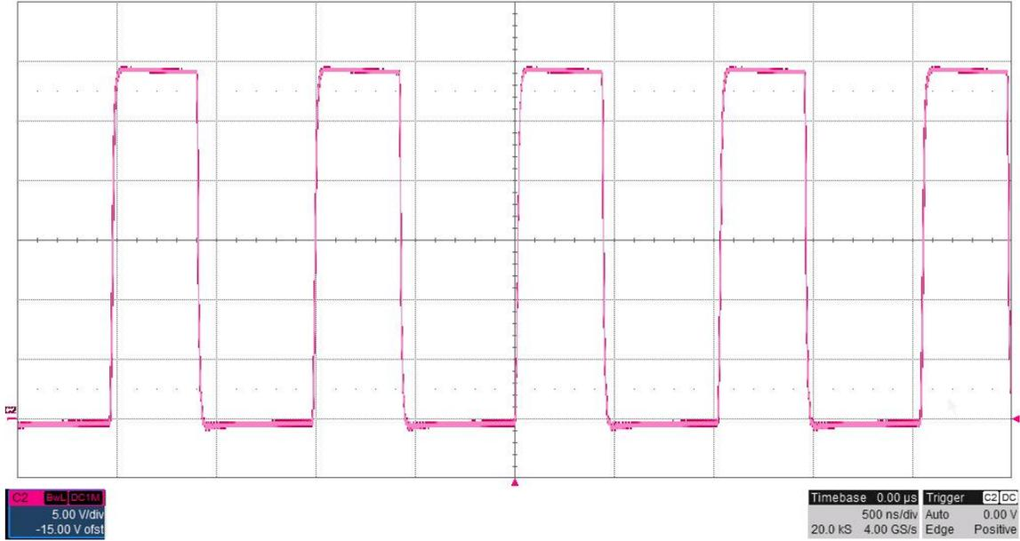
The photo below shows the switch node voltage (SW pin). The input voltage is 12V and the 28V output is loaded to 0.025A. The converter is operating in discontinuous conduction mode. (5V/DIV, 500nS/DIV)
