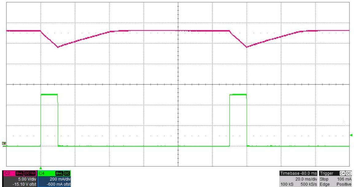
The photo below shows the output voltage when the load current is stepped between 0A and 1A.
