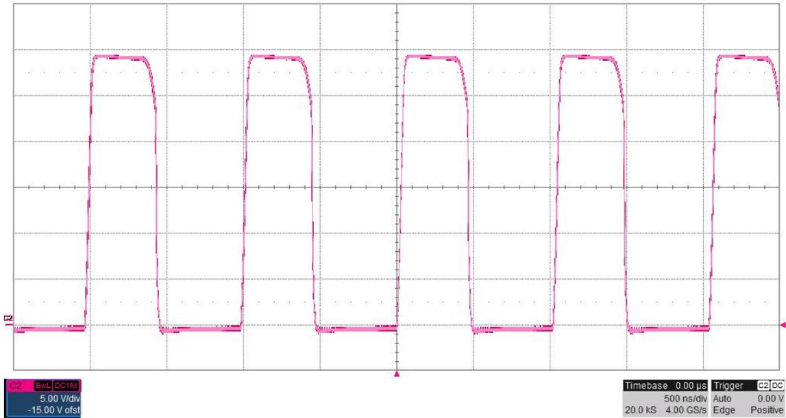
The photo below shows the switch node voltage (SW pin). The input voltage is 12V and the 28V output is loaded to 0A. The converter is operating in discontinuous conduction mode. (5V/DIV, 500ns/DIV)
