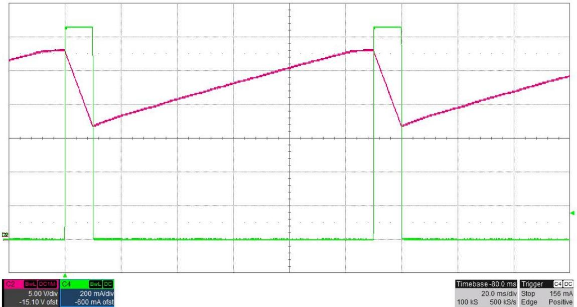
The photo below shows the output voltage when the load current is stepped between 0A and 0.35A.  $V_{in} = 12V$ . Ch2 is the voltage at R2 (output of INA139). Ch1 is the voltage at diode D2 Anode. The current loop is in control when  $V_{out}$  is less than 28V. (1V/DIV, 500mA/DIV, 20mS/DIV)
