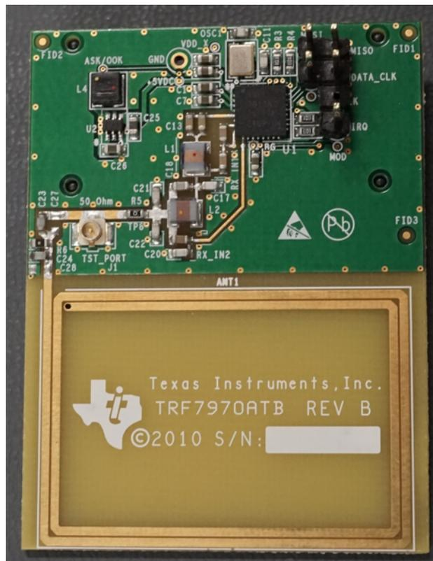
**Figure 13. Front View of the TRF7970ATB**
