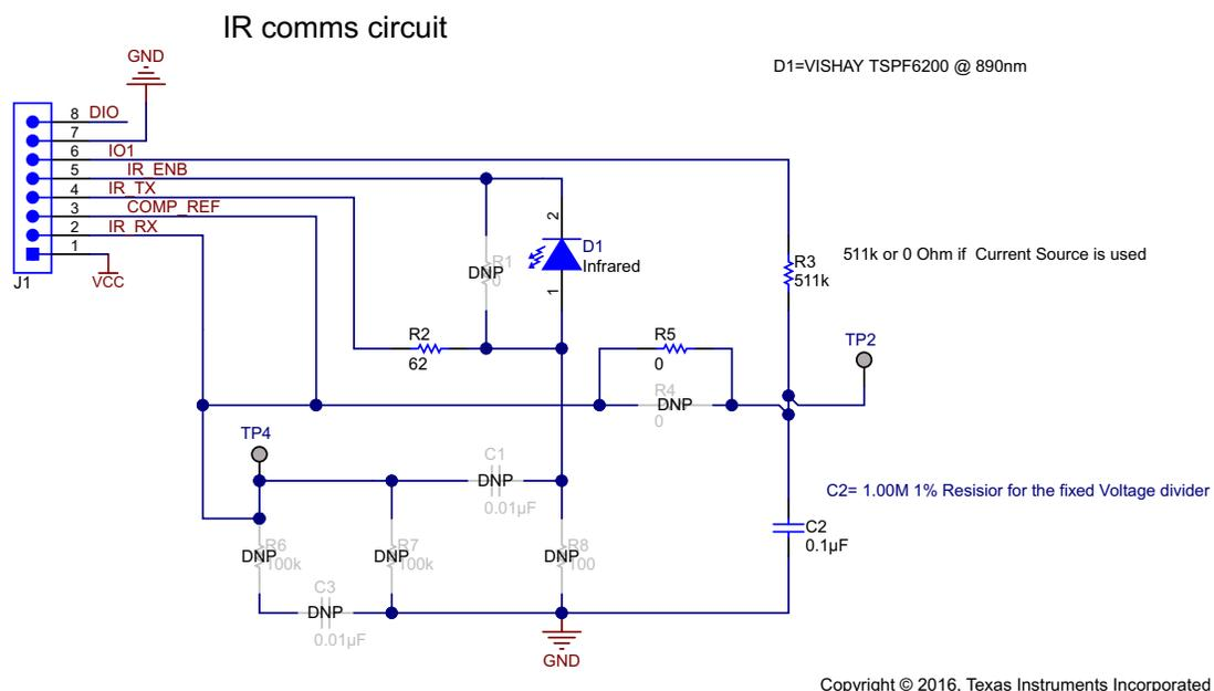
**Figure 3. TIDA-01212 Schematic**
