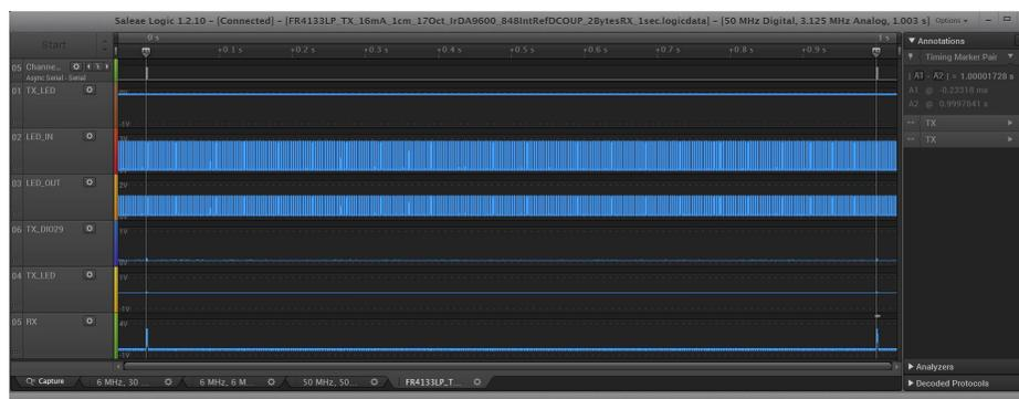
**Figure 9. Transmit IR LED Pulses Train and RX Polling Period of 1 Second**
