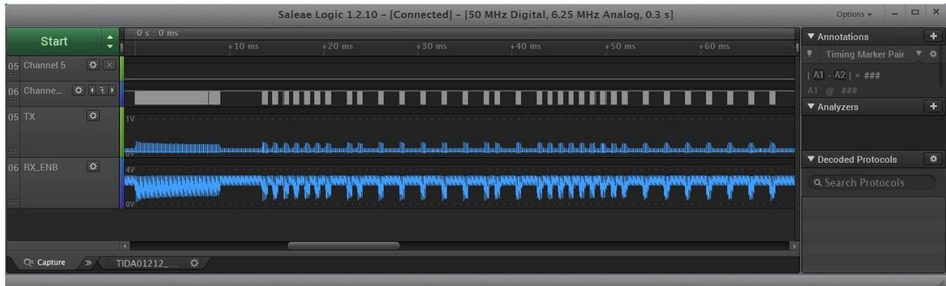
Figure 11. IR Input Signal From TV RC Using NEC IR Protocol
