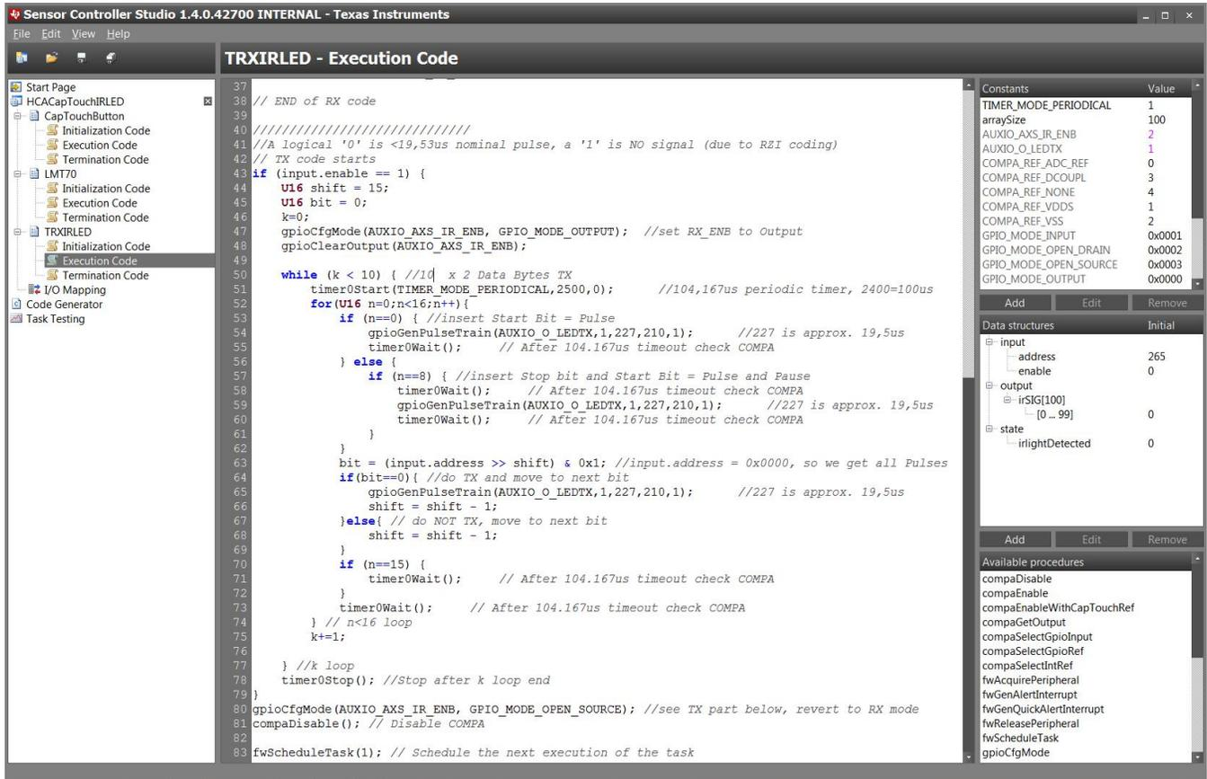
Figure 8. Execution Code for TRXIRLED Task (Transmit Example)
