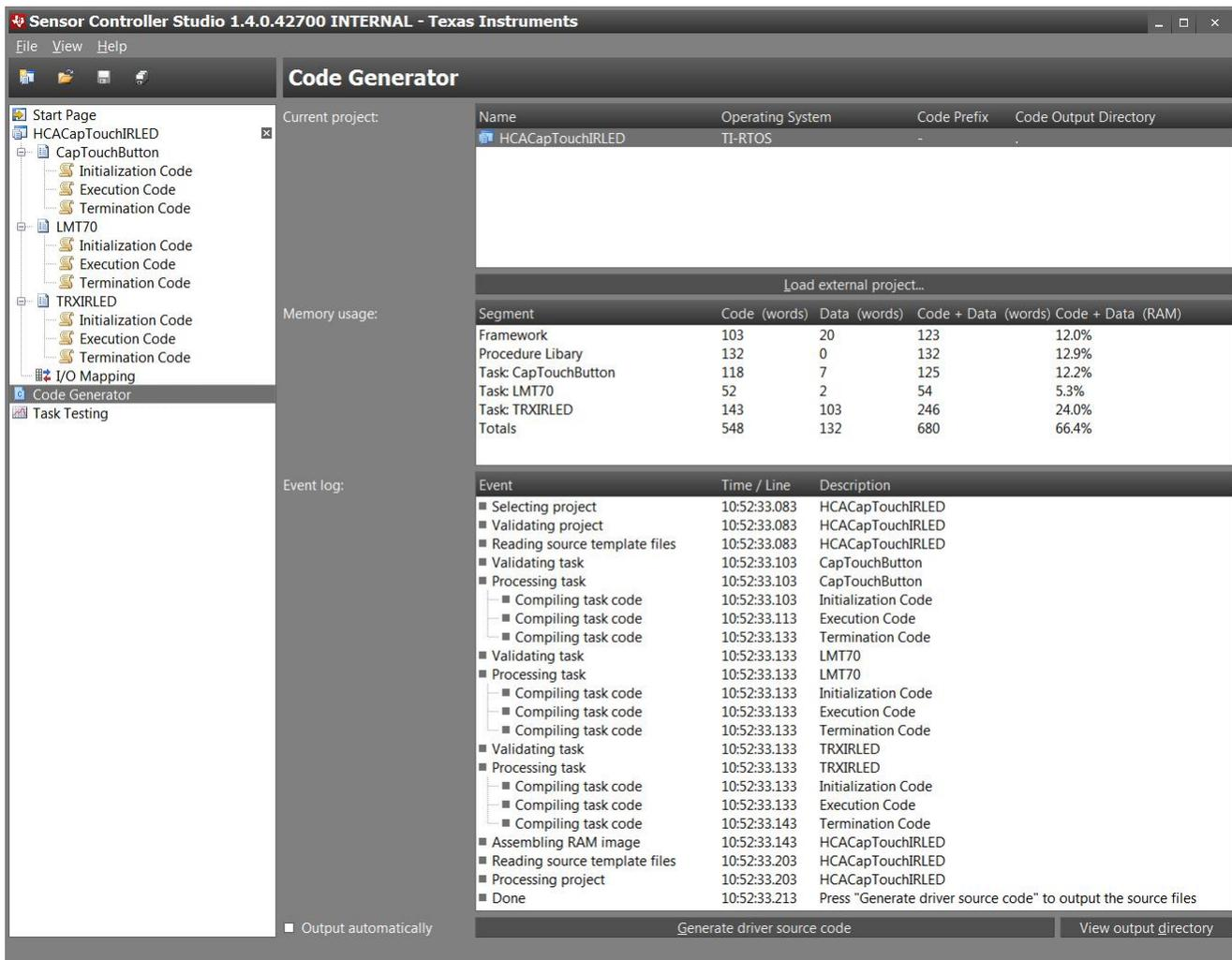
**Figure 5. SCE Project for HCA (CapTouchButton, LMT70A Readout, and IR LED Comm Port)**
