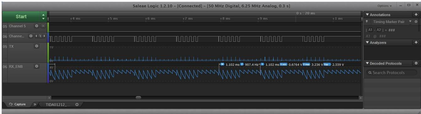
Figure 14. Timing of Logical "0" as per NEC IR Protocol
