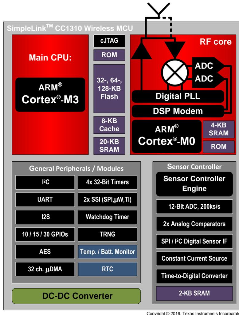
**Figure 2. CC1350 Block Diagram**
