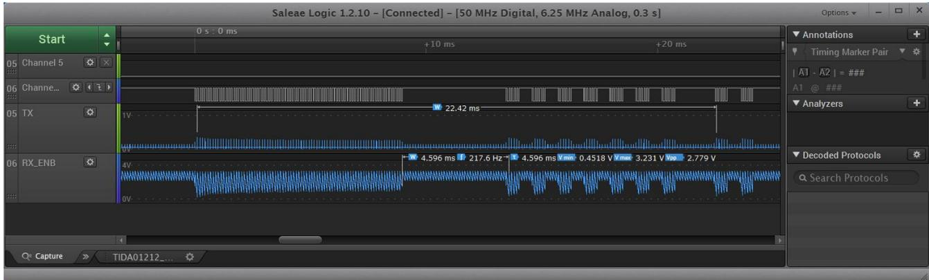
Figure 13. Timings for IR From TVR Using NEC IR Protocol, Preamble, Low Phase, and First Bits
