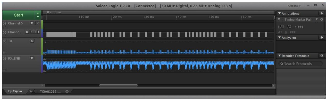
Figure 12. RX\_ENB is the Analog Signal Input to COMPA (Using an Internal Reference of  $DCOUP_L = 1.27$  V)
