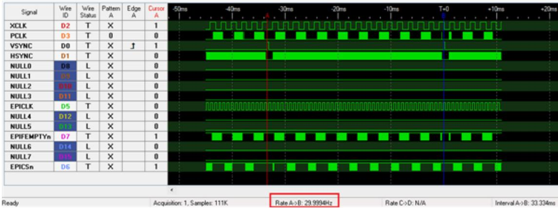
Figure 24. Frame and Line Rate for Data Capture
