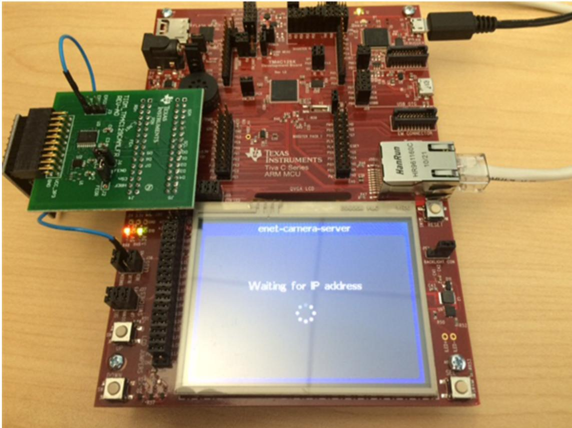
**Figure 20. Board View When Acquiring IP Address**
