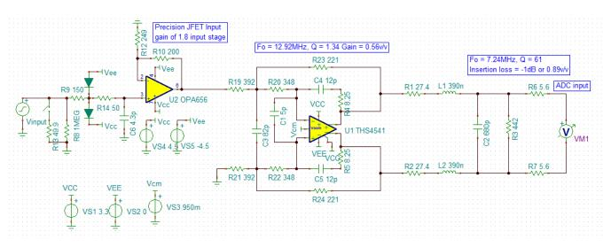
Figure 4. Input Circuit With OPA656, THS4541, and Low-pass Filter
