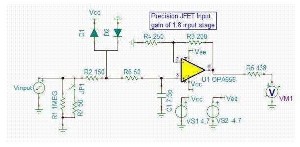
Figure 2. Circuit for Input Buffer Stage (OPA656)
