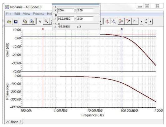
Figure 3. Frequency Response of Input Buffer Stage (OPA656)
