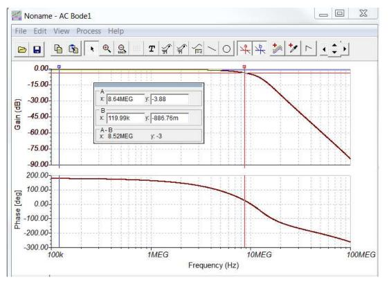
Figure 6. Frequency Response of Input Circuit
