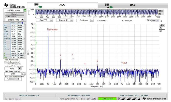
Figure 8. FFT 1-MHz –1-dBFS Input Signal
