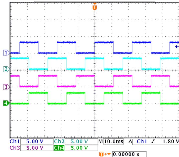
Figure 12. Output of SN74HC595/Input to ULN2003A (Full-Step Pattern, Counterclockwise)
