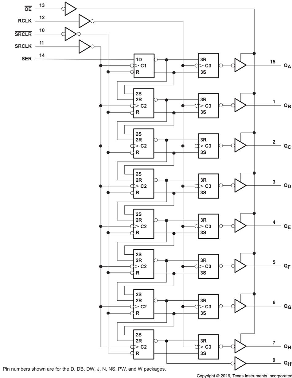
Figure 6. SN74HC595 Logic Diagram
