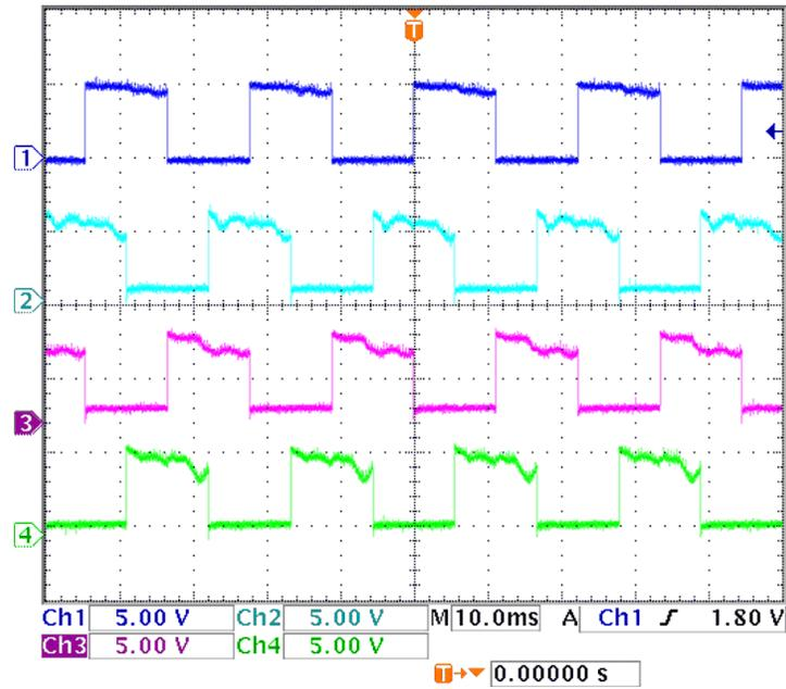
Figure 13. ULN2003A Output Motor Drive Pattern (Full-Drive Pattern, Clockwise)
