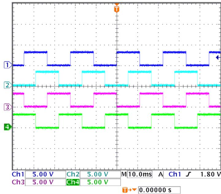
Figure 11. Output of SN74HC595 and Input to ULN2003A (Full-Step Pattern, Clockwise)
