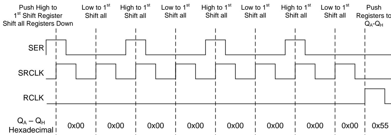
Figure 7. Bit-Banging to Set SN74HC595 Outputs
