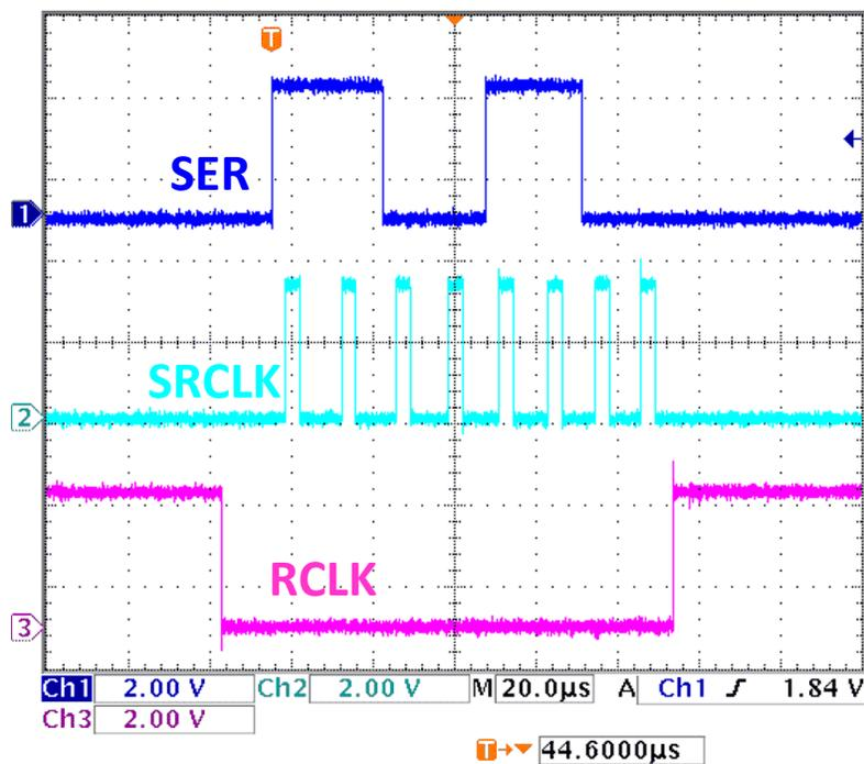
Figure 10. Oscilloscope Waveform of SER, SRCLK, and RCLK Input to SN74HC595
