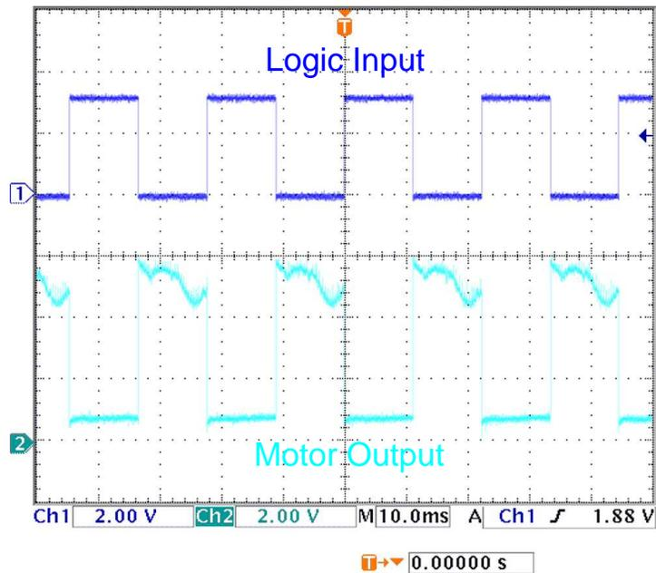
Figure 14. ULN2003A Logic Input and ULN2003A Drive Output
