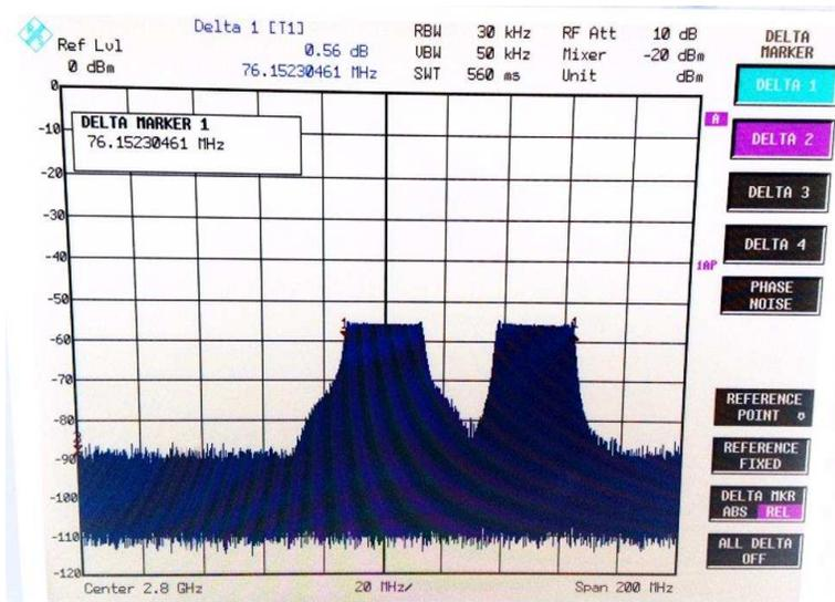
Figure 12. Measured Transmit Bandwidth
