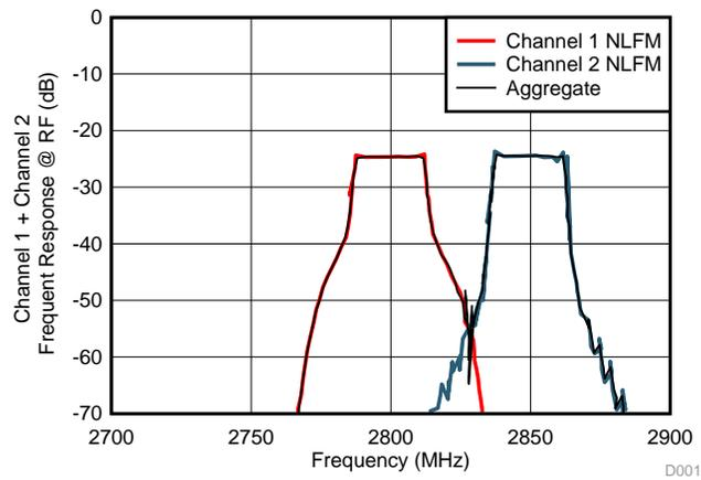
Figure 11. Aggregate Signal Frequency Response at RF (Ideal)
