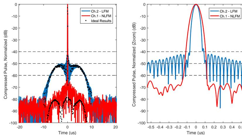
**Figure 13. Measured Output of Pulse-Compression Filters**
