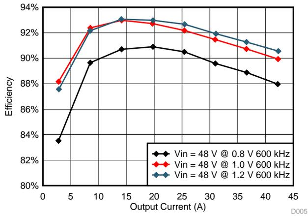
**Figure 15. Efficiency Curve without Controller Loss Versus Vout Change (Through I²C)**
