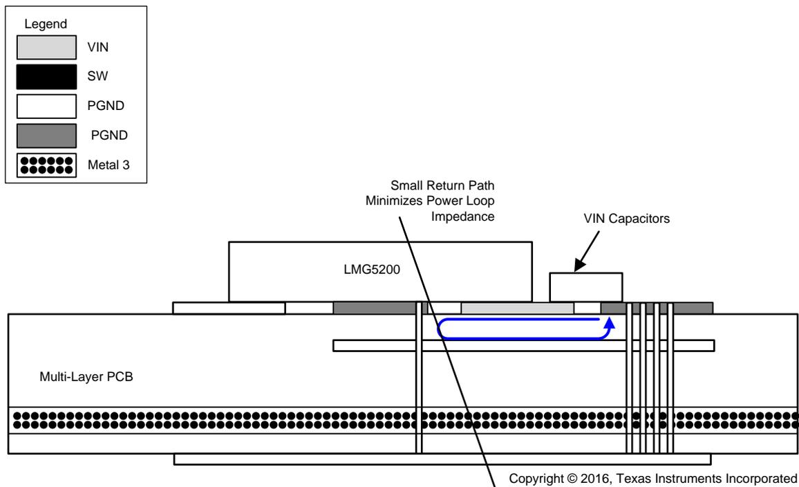
**Figure 17. Multilayer Board Cross Section With Return Path Directly Underneath for Power Loop**
