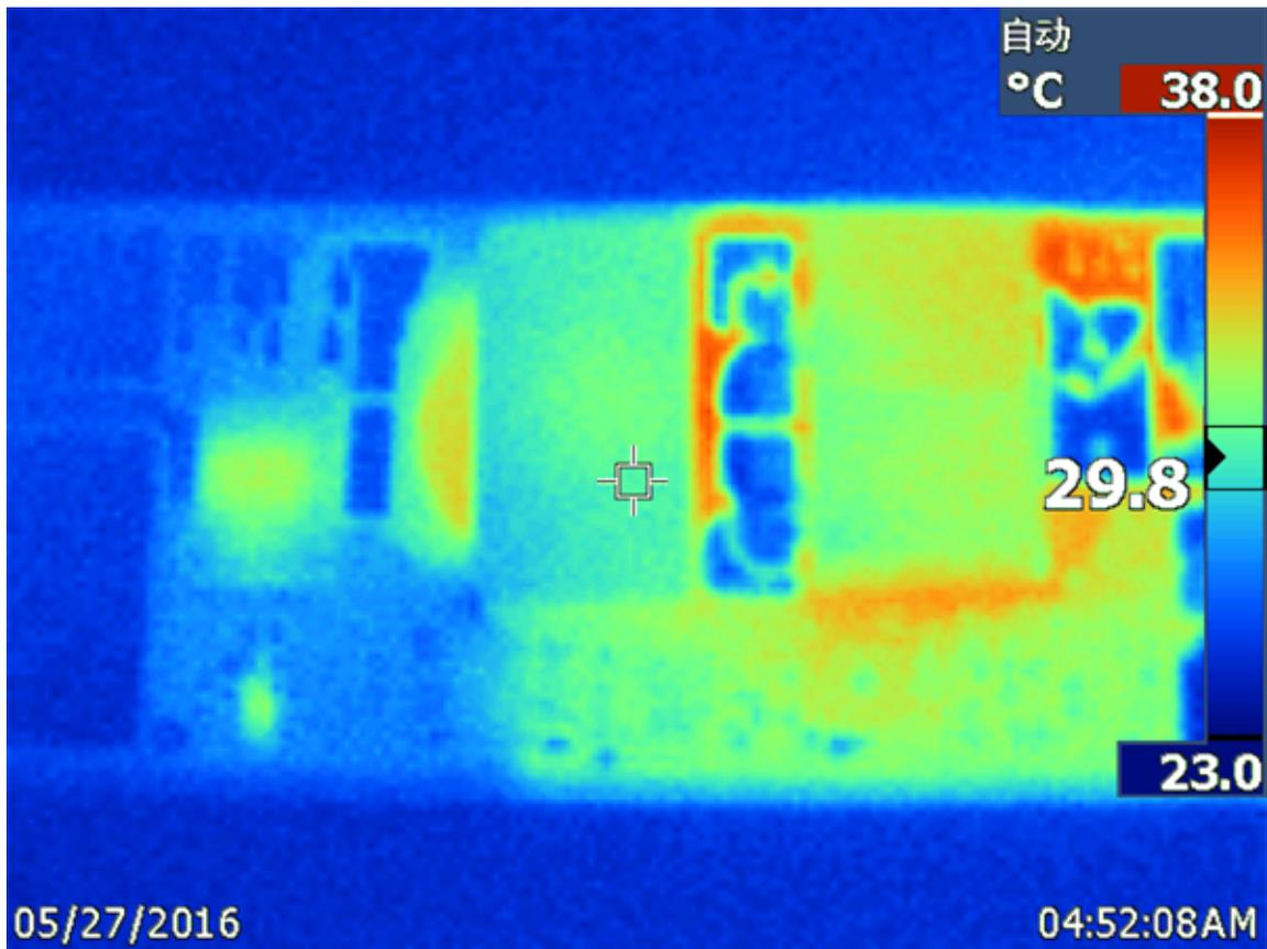
Figure 16. 48-V Input at Full Load (1.0 V and 40 A)
