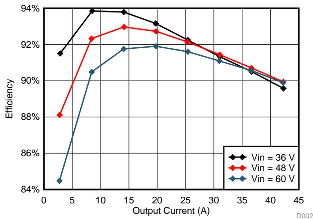
Figure 12. Efficiency Curve Without Controller Loss Versus Output Current
