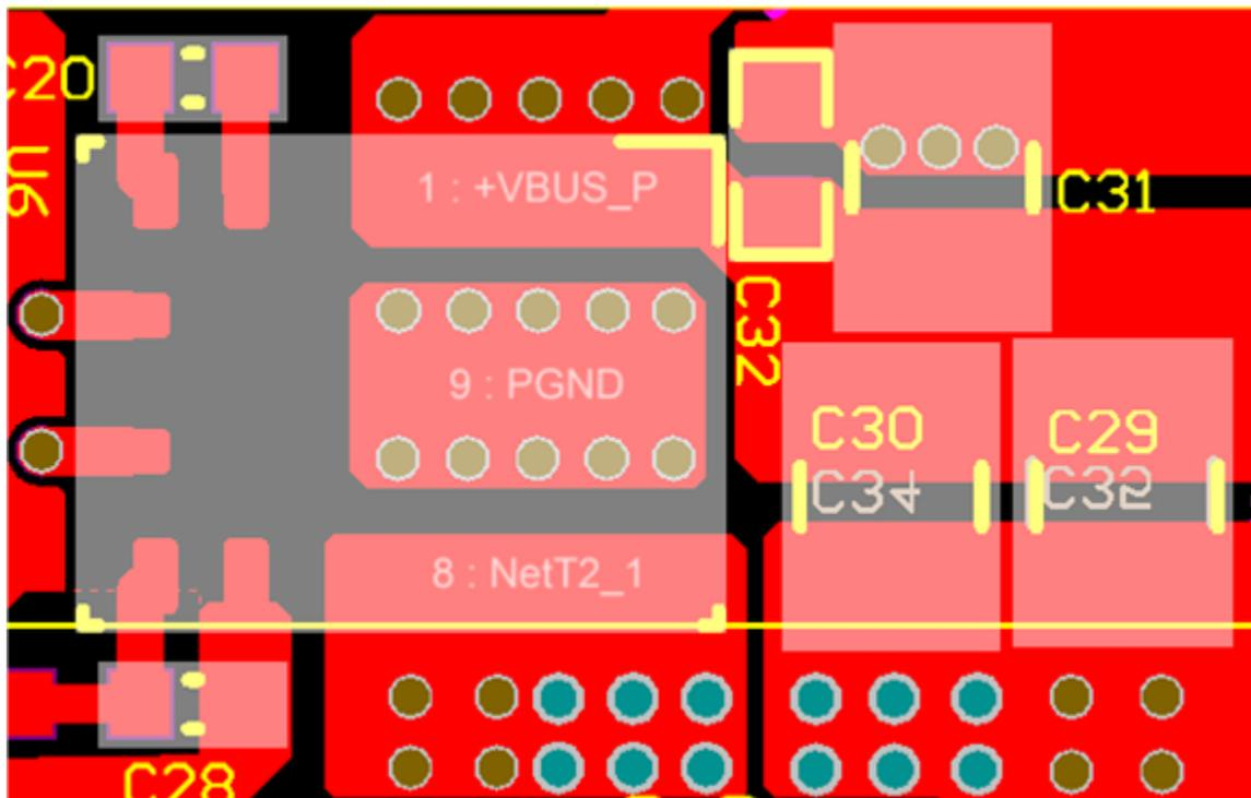
**Figure 18. LMG5200 Top Layer Placement**
