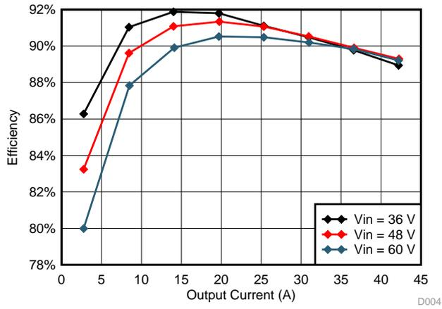
**Figure 14. Efficiency Curve with Controller Loss Versus Output Current**
