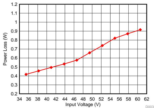
Figure 13. Power Loss (No Load) Versus Input Voltage
