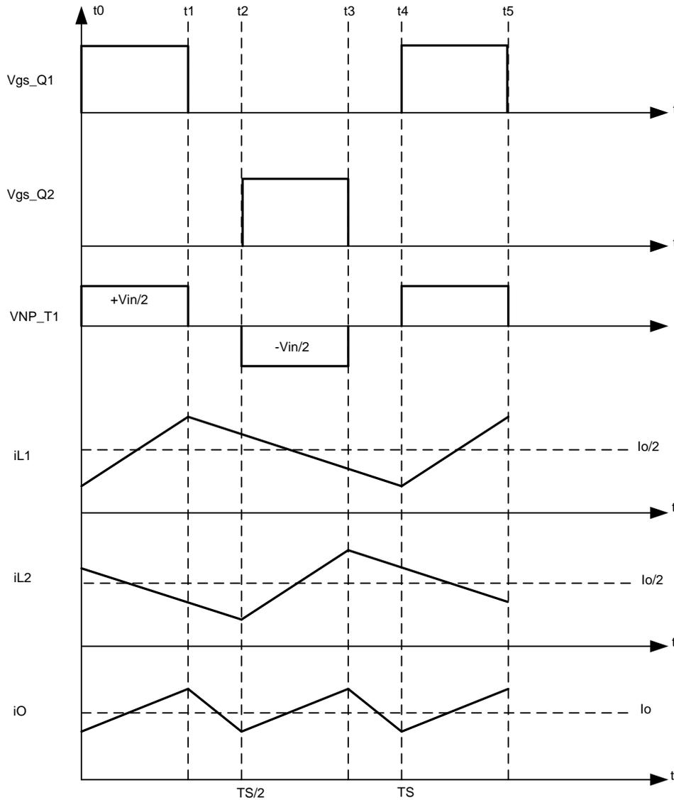
**Figure 6. Half-Bridge with Current Doubler Timing Diagram**
