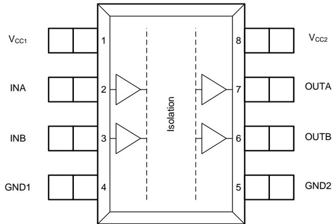
Figure 4. ISO7420 Block Diagram
