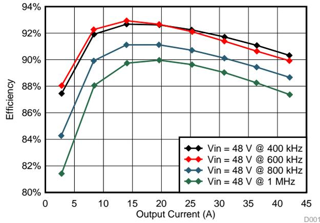
Figure 11. Efficiency Curve Without Controller Loss Versus Switching Frequency
