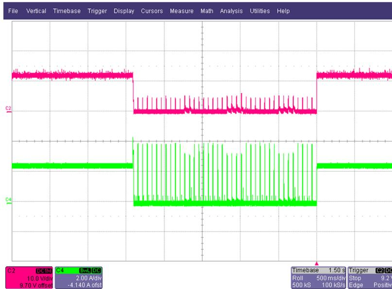
**Figure 23. Response During Short-Circuit and Auto-Recovery After Removal of Short**
