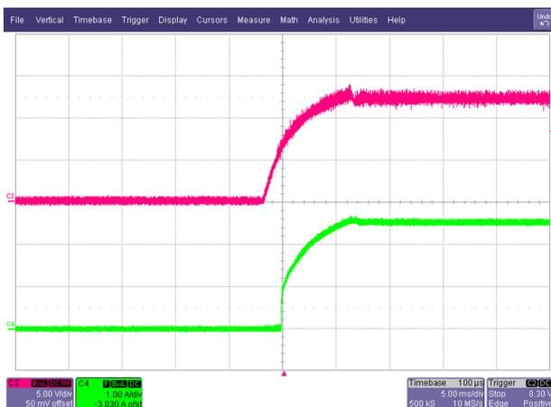
Figure 17. 12-V\_ISO/2.75-A Output Turnon Waveform at 400-V DC
