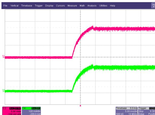
Figure 18. 12-V/0.25-A Output Turnon Waveform at 400-V DC
