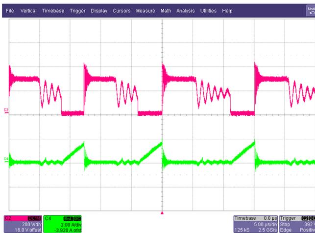
Figure 10. SW Node Waveform and MOSFET Current at  $V_{INDC} = 165\text{-V}$ , Full Load
