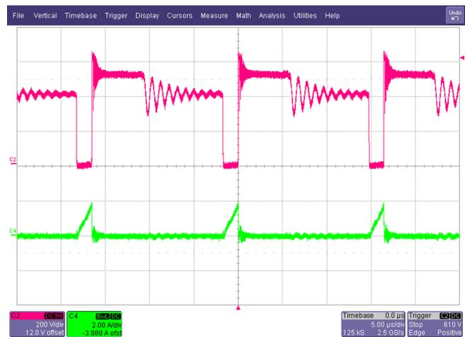
Figure 11. SW Node Waveform and MOSFET Current at  $V_{INDC} = 400\text{-V}$ , Full Load
