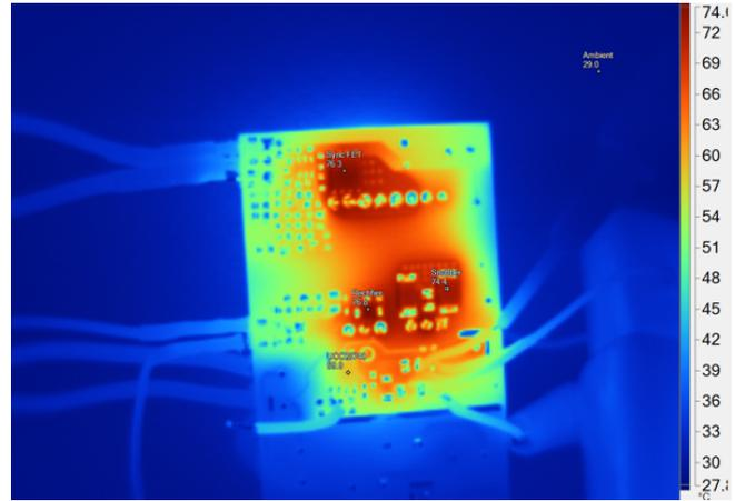
Figure 25. Bottom-Side Thermal Image at 400-V DC Input, Full Load, Without Fan
