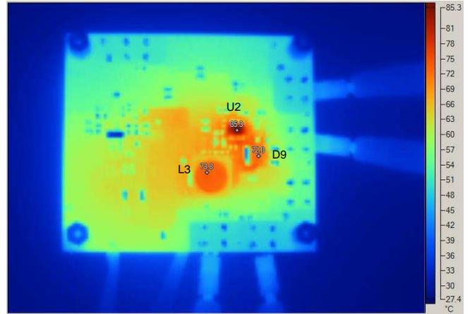
**Figure 45. Thermal Image of Board Bottom Side With  $V_{IN} = 24\text{ V}$  and  $P_{OUT} = 31.5\text{ W}$**
