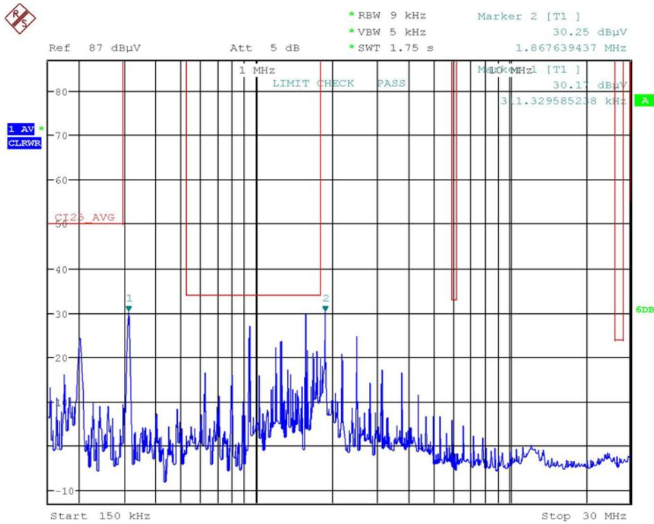
**Figure 104. Measured Average Noise of Test Circuit 4 (150 kHz to 30 MHz, Limit Line: CISPR 25 Class 5 Average, Limit Check: Pass)**
