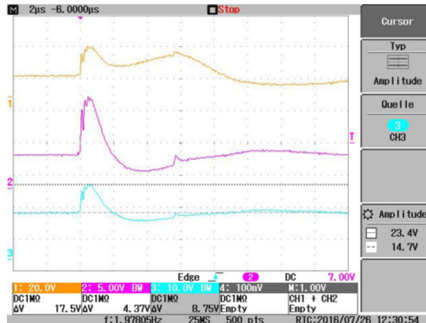
Figure 71. Output Overshoot During Pulse 2a Test
