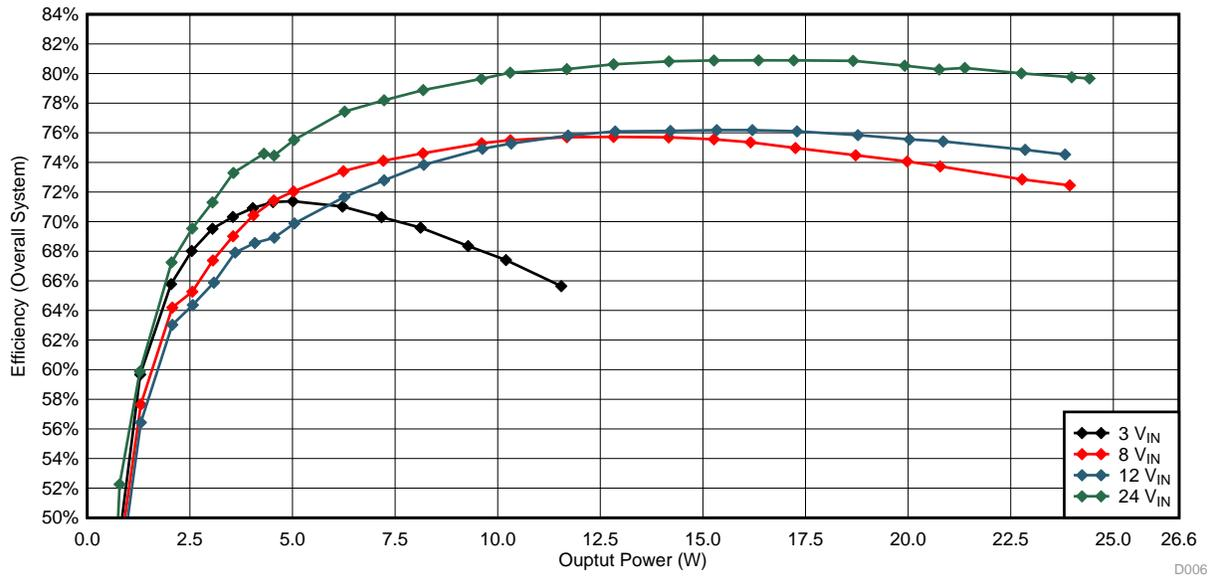
Figure 20. Measured Efficiency of Total System
