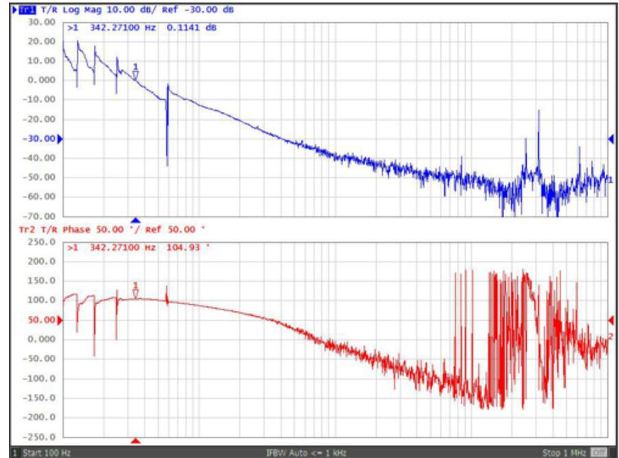
**Figure 60. Loop Frequency Response of Buck-Boost Converter With  $V_{IN} = 3.0\text{ V}$  and  $I_{OUT} = 0.5\text{ A}$**
