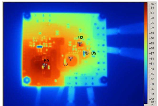
**Figure 49. Thermal Image of Board Bottom Side With  $V_{IN} = 6\text{ V}$  and  $P_{OUT} = 21\text{ W}$**
