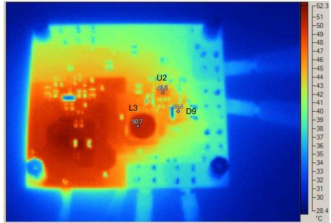
Figure 51. Thermal Image of Board Bottom Side With  $V_{IN} = 6\text{ V}$  and  $P_{OUT} = 10\text{ W}$
