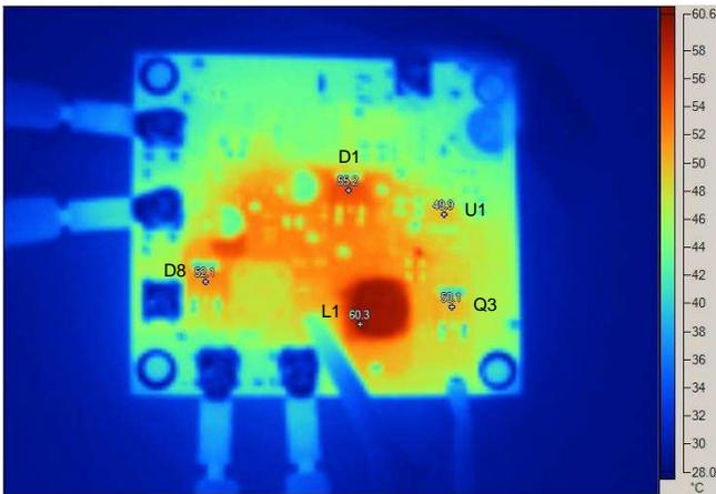
**Figure 46. Thermal Image of Board Top Side With  $V_{IN} = 24\text{ V}$  and  $P_{OUT} = 20\text{ W}$**
