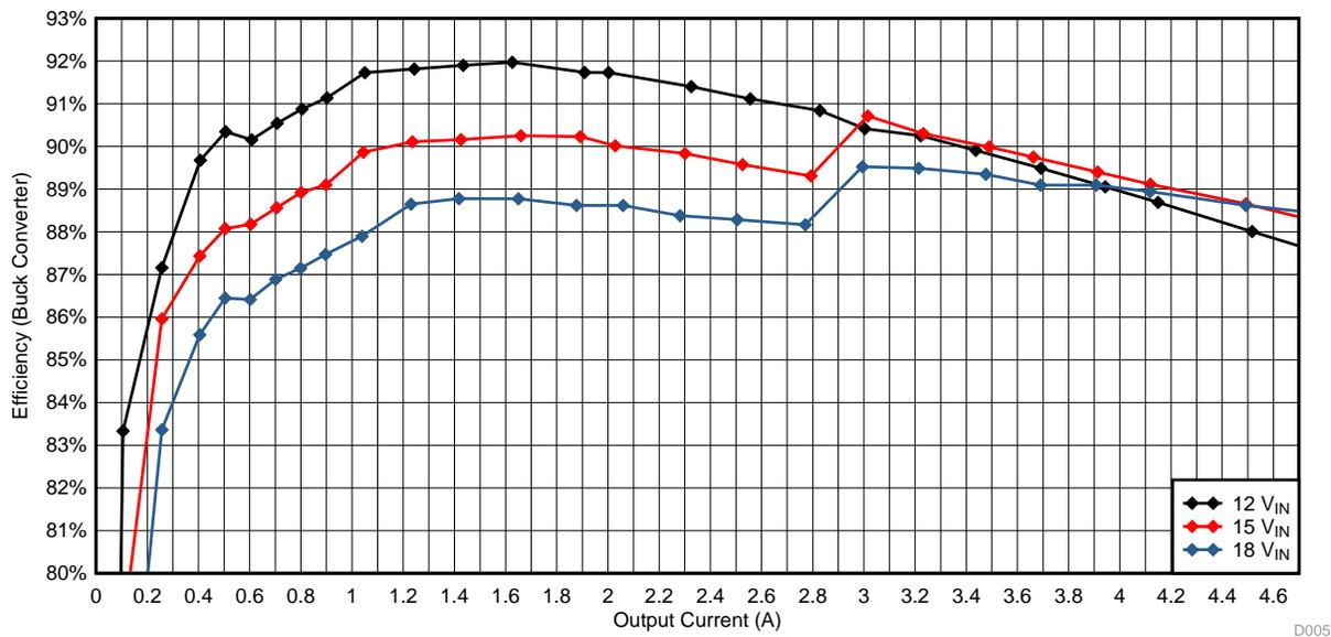
Figure 19. Measured Efficiency of Buck Converter
