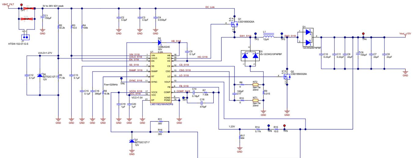
Figure 4. Schematic of Buck-Boost DC-DC Converter
