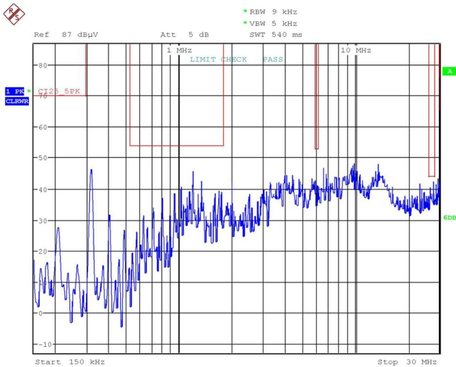
Figure 93. Measured Peak Noise of Test Circuit 1 (150 kHz to 30 MHz, Limit Line: CISPR 25 Class 5 Peak, Limit Check: Pass)
