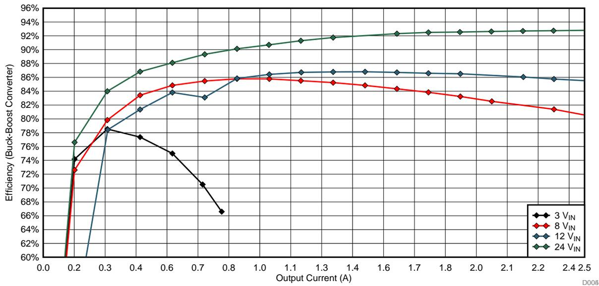
Figure 18. Measured Efficiency of Buck-Boost Converter
