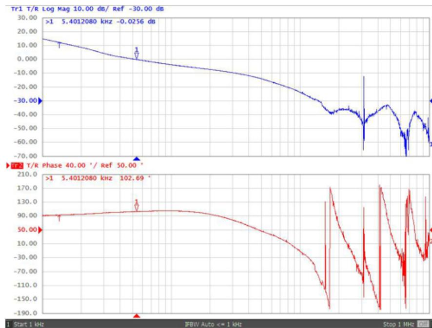
**Figure 53. Loop Frequency Response of Buck-Boost Converter With  $V_{IN} = 13\text{ V}$  and  $I_{OUT} = 0.5\text{ A}$**
