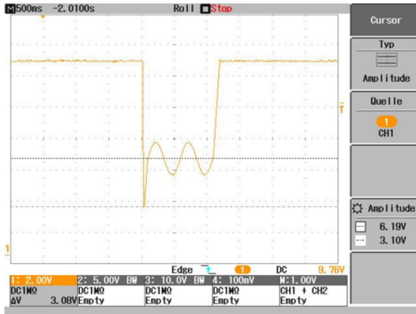
Figure 85. Severe Cold Cranking Test Pulse (Level 3)
