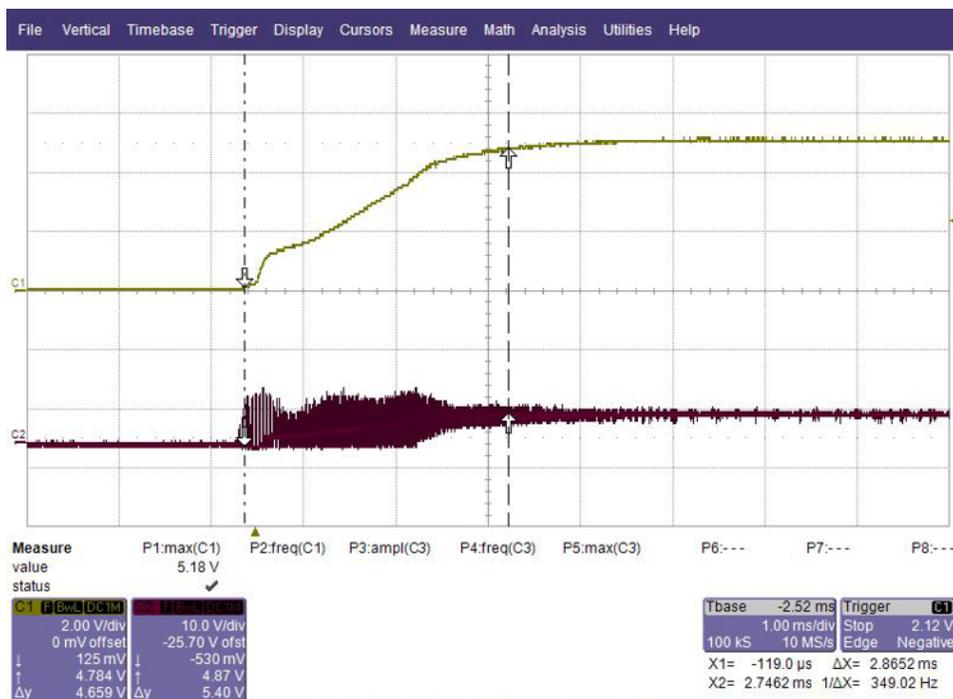
Figure 15. Start-up Waveform of Buck Converter
