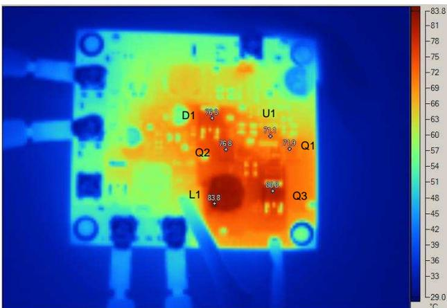
**Figure 48. Thermal Image of Board Top Side With  $V_{IN} = 6\text{ V}$  and  $P_{OUT} = 21\text{ W}$**
