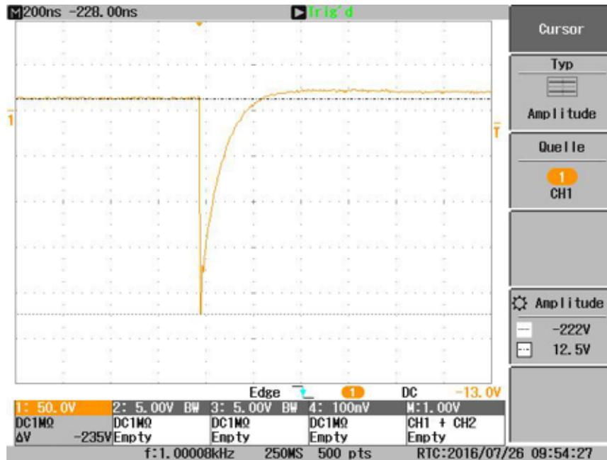
Figure 72. Pulse 3a Test Pulse
