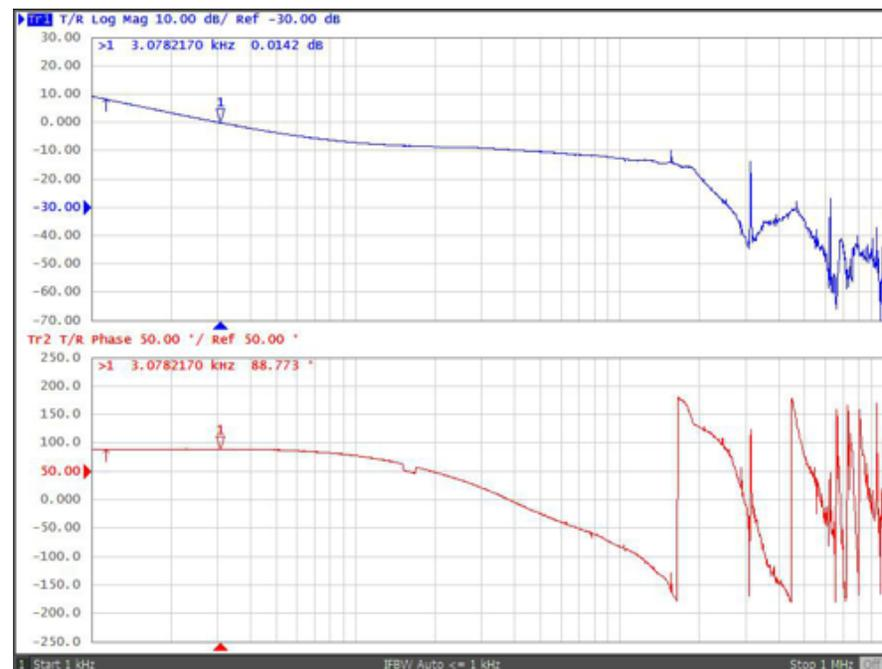
**Figure 58. Loop Frequency Response of Buck-Boost Converter With  $V_{IN} = 6\text{ V}$  and  $I_{OUT} = 0.9\text{ A}$**
