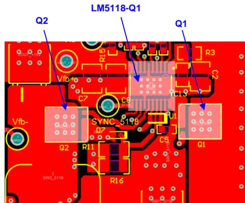
**Figure 118. Place MOSFETs Close to Buck-Boost Controller**
