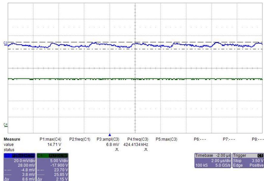
Figure 26. Output Voltage Ripple of Buck-Boost Converter Under  $V_{IN} = 8\text{ V}$  and  $I_{OUT} = 0.1\text{ A}$
