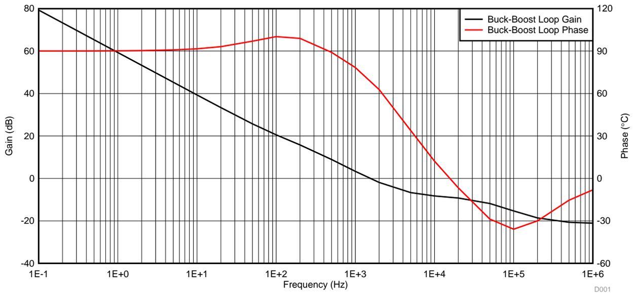
Figure 6. Calculated Loop Response of LM5118 Buck-Boost Modulator
