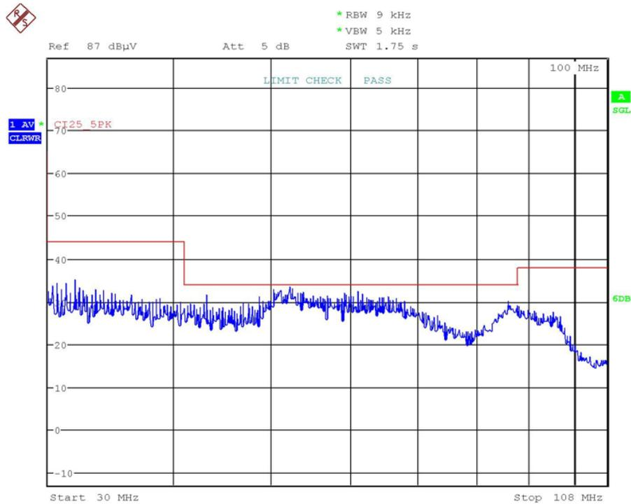
**Figure 108. Measured Peak Noise of Test Circuit 1 (30 to 108 MHz, Limit Line: CISPR 25 Class 5 Peak, Limit Check: Pass)**
