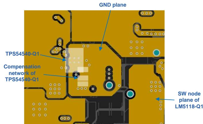
**Figure 124. Place Compensation Network Close to Controller and Away From Any Switch Node**
