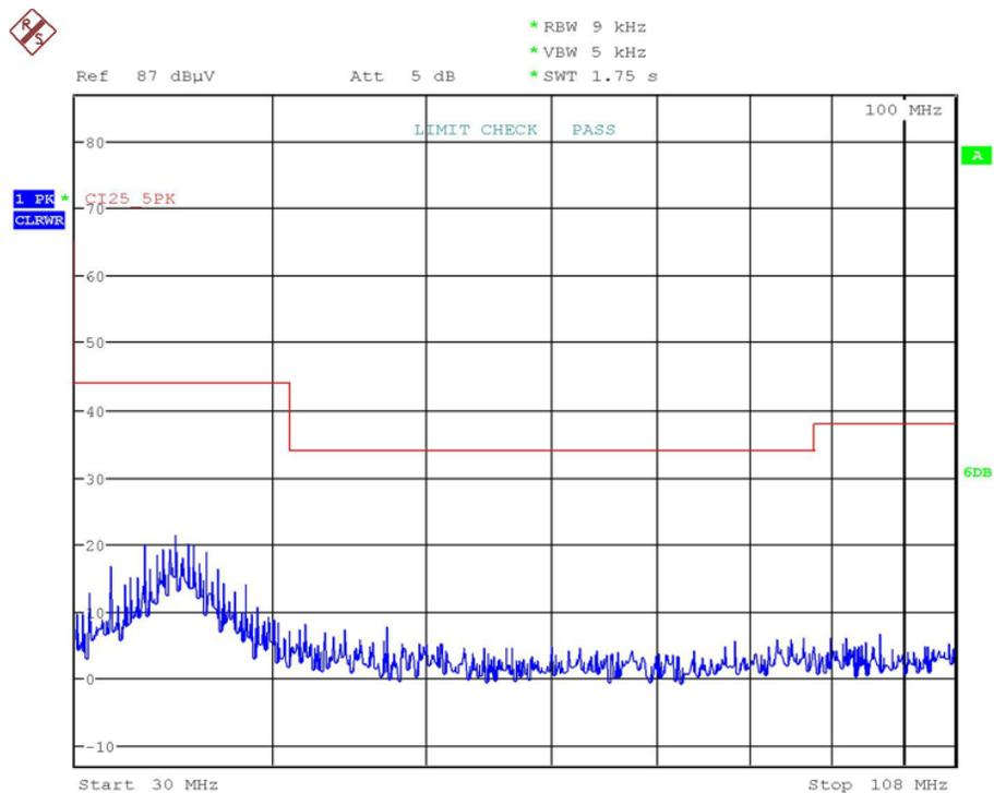
**Figure 113. Measured Peak Noise of Test Circuit 2 (30 to 108 MHz, Limit Line: CISPR 25 Class 5 Peak, Limit Check: Pass)**
