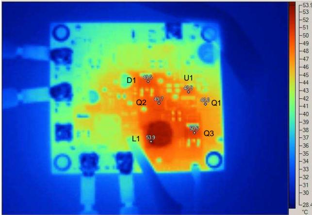
Figure 50. Thermal Image of Board Top Side With  $V_{IN} = 6\text{ V}$  and  $P_{OUT} = 10\text{ W}$
