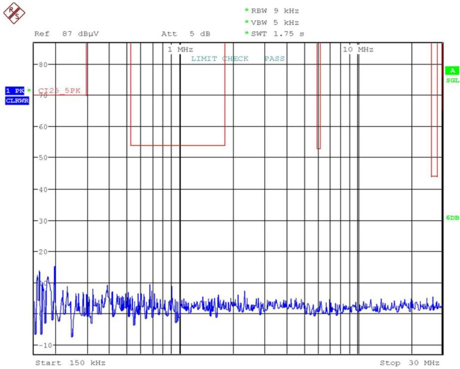
Figure 89. Ambient Noise (150 kHz to 30 MHz)
