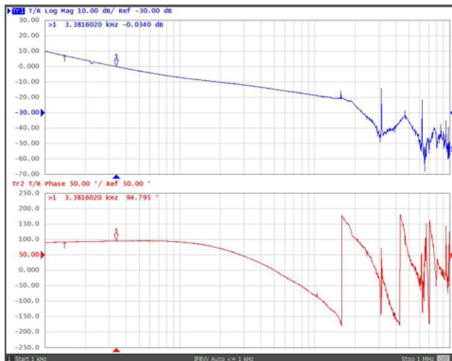
**Figure 57. Loop Frequency Response of Buck-Boost Converter With  $V_{IN} = 6\text{ V}$  and  $I_{OUT} = 0.5\text{ A}$**
