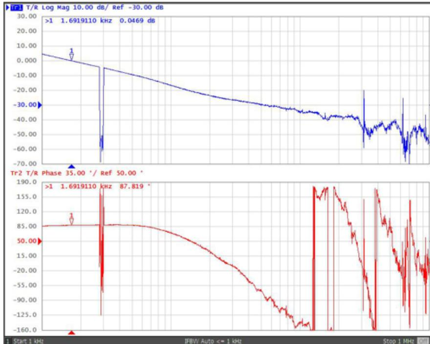
**Figure 59. Loop Frequency Response of Buck-Boost Converter With  $V_{IN} = 3.0\text{ V}$  and  $I_{OUT} = 0.2\text{ A}$**
