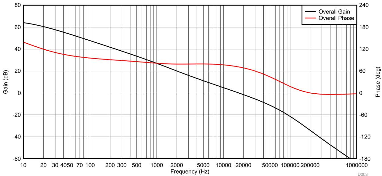
Figure 9. Calculated Loop Response of LM54540-Q1 Buck Converter
