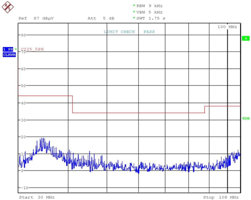
Figure 103. Measured Peak Noise of Test Circuit 4 (30 to 108 MHz, Limit Line: CISPR 25 Class 5 Peak, Limit Check: Pass)
