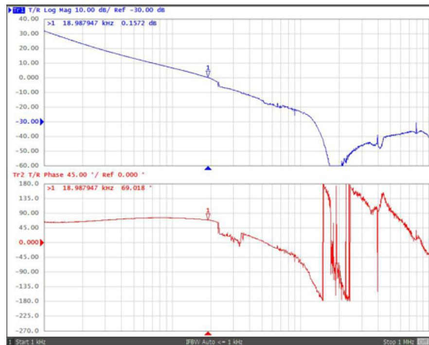
Figure 64. Loop Frequency Response of Buck Converter With  $V_{IN} = 9\text{ V}$  and  $I_{OUT} = 4\text{ A}$
