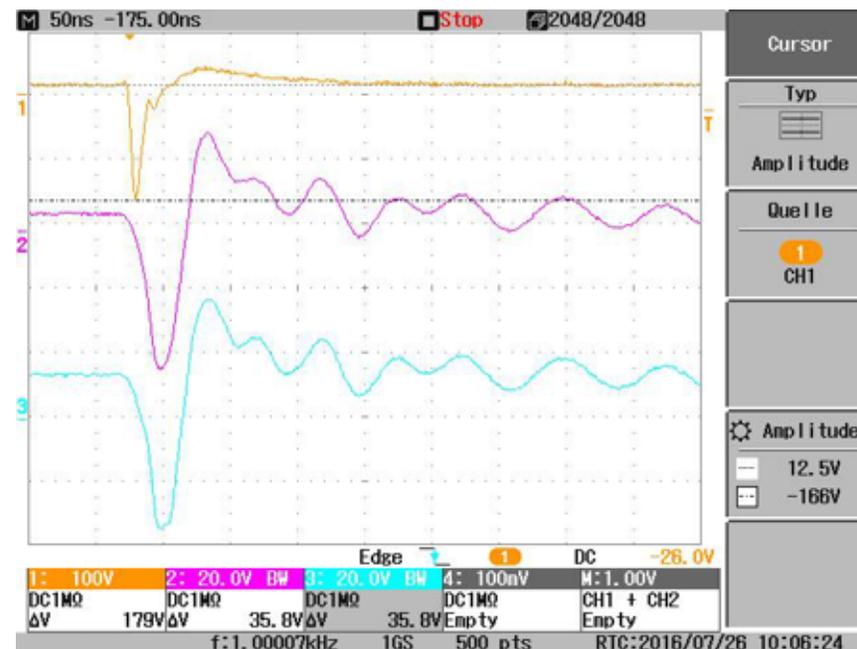
Figure 74. Output Voltage Undershoots During Pulse 3a Test
