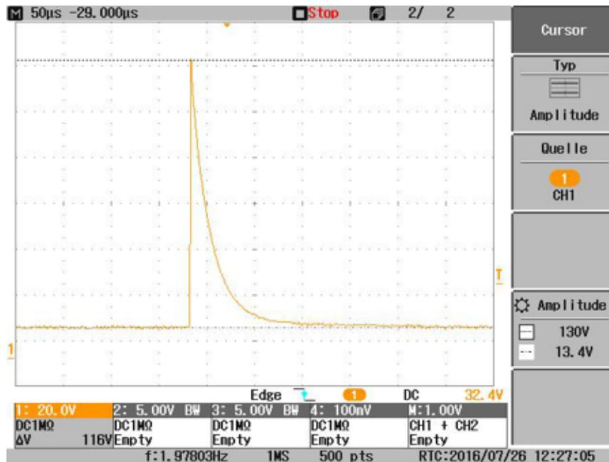
Figure 69. Pulse 2 Test Pulse
