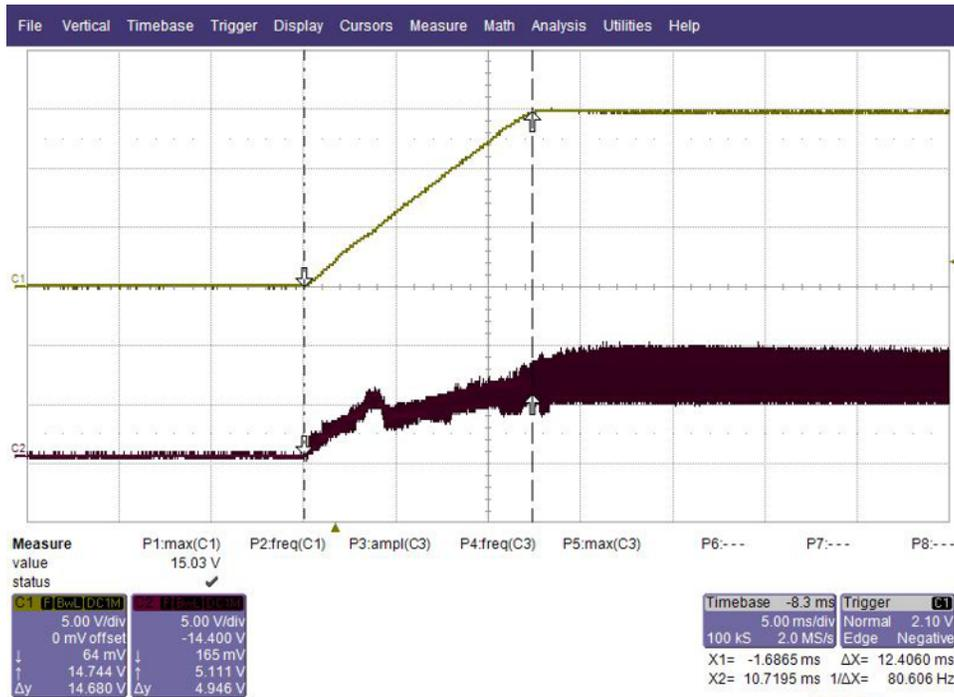
**Figure 14. Start-up Waveform of Buck-Boost Converter**
