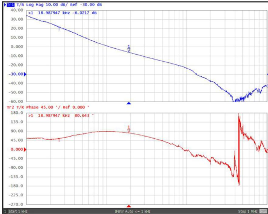
**Figure 61. Loop Frequency Response of Buck Converter With  $V_{IN} = 15\text{ V}$  and  $I_{OUT} = 1\text{ A}$**
