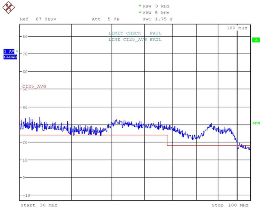
**Figure 110. Measured Average Noise of Test Circuit 1 (30 to 108 MHz, Limit Line: CISPR 25 Class 5 Average, Limit Check: Fail)**
