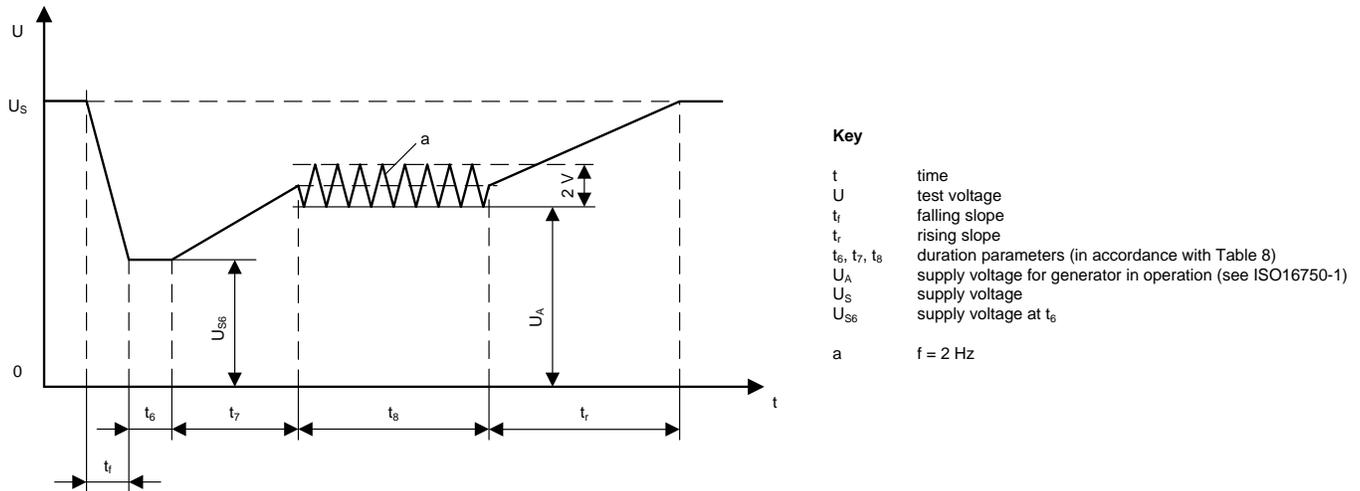
Figure 82. Battery Cranking Profile per ISO16750-2 Standard
