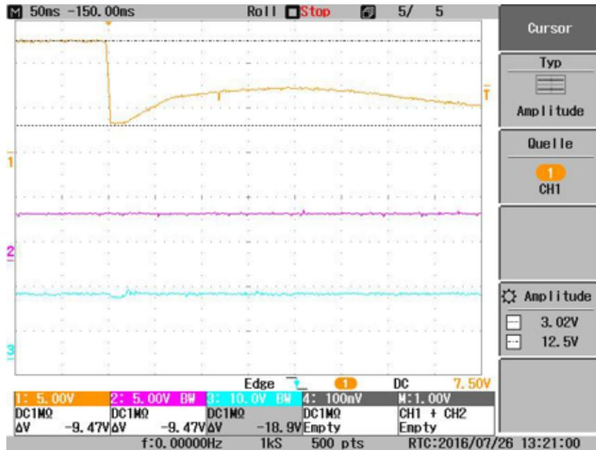
Figure 87. Expanded Time Scale at Beginning Transient of Cold Cranking Pulse (Level 3)
