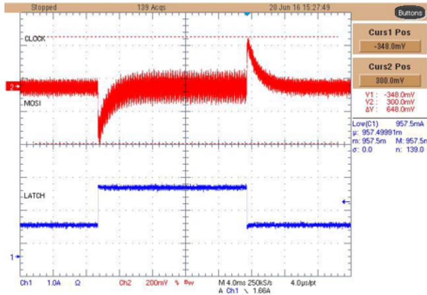
Figure 32. Load Transient Response of Buck-Boost Converter Under  $V_{IN} = 13\text{ V}$  and  $I_{OUT}$  Switching Between 2.2 A and 1 A
