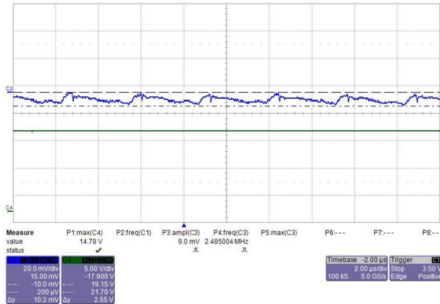
Figure 24. Output Voltage Ripple of Buck-Boost Converter Under  $V_{IN} = 3.0 \text{ V}$  and  $I_{OUT} = 0.1 \text{ A}$
