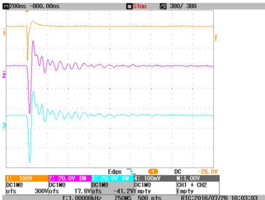
Figure 73. Outputs of Power Rails During Pulse 3a Test
