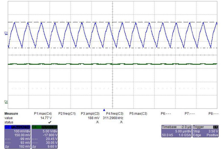
**Figure 29. Output Voltage Ripple of Buck-Boost Converter Under  $V_{IN} = 13\text{ V}$  and  $I_{OUT} = 2.2\text{ A}$**
