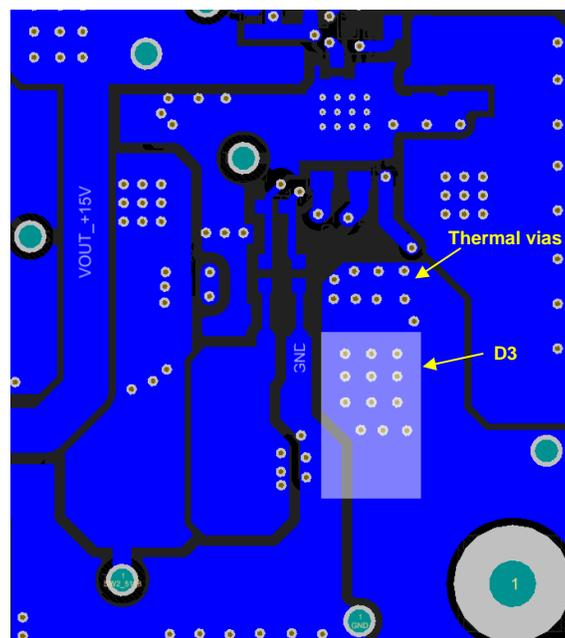
**Figure 125. Thermal Via Placement for Increased Cooling of Schottky Diode D3**
