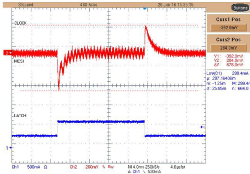
Figure 35. Load Transient Response of Buck-Boost Converter Under  $V_{IN} = 3.0\text{ V}$  and  $I_{OUT}$  Switching Between 0.8 A and 0.3 A
