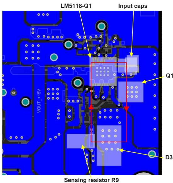
**Figure 119. Buck Switching Loop of LM5118-Q1**
