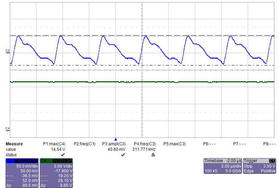
Figure 25. Output Voltage Ripple of Buck-Boost Converter Under  $V_{IN} = 3.0 \text{ V}$  and  $I_{OUT} = 0.6 \text{ A}$
