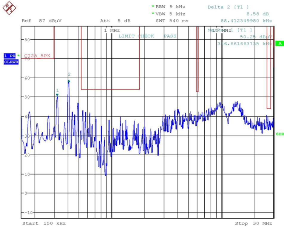
**Figure 100. Measured Peak Noise of Test Circuit 3 (150 kHz to 30 MHz, Limit Line: CISPR 25 Class 5 Peak, Limit Check: Pass)**
