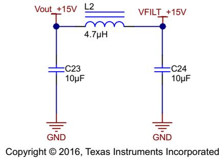
Figure 11. Schematic of DM EMI Filter for Buck Converter
