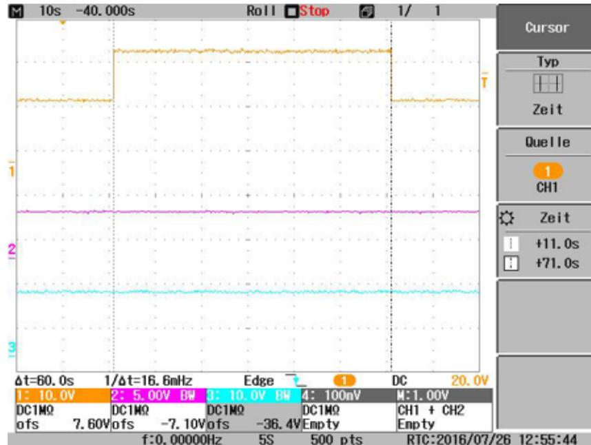
Figure 79. Outputs of Power Rails During Jump Start Test
