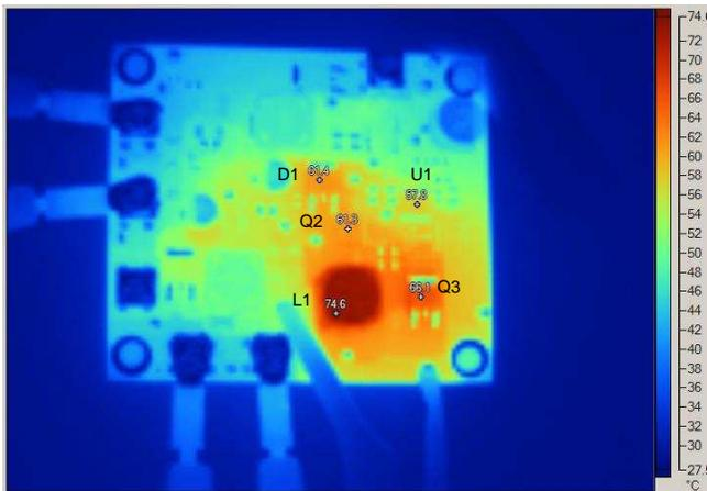
Figure 42. Thermal Image of Board Top Side With  $V_{IN} = 13\text{ V}$  and  $P_{OUT} = 20\text{ W}$
