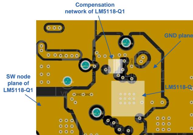
Figure 123. Place Compensation Network Close to Controller and Away From Any Switch Node
