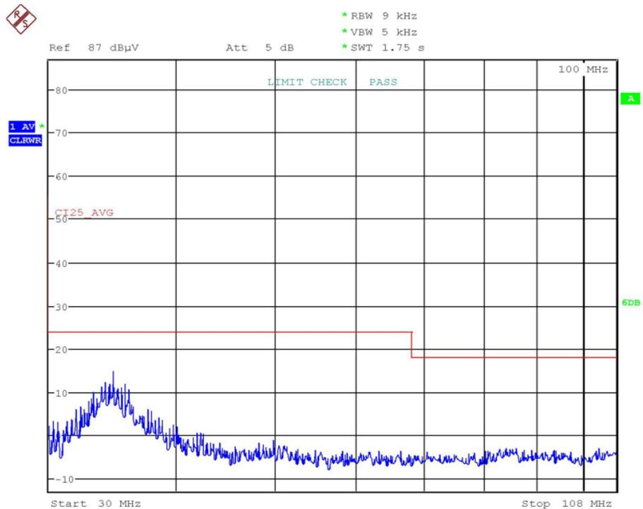
**Figure 115. Measured Average Noise of Test Circuit 2 (30 to 108 MHz, Limit Line: CISPR 25 Class 5 Average, Limit Check: Pass)**
