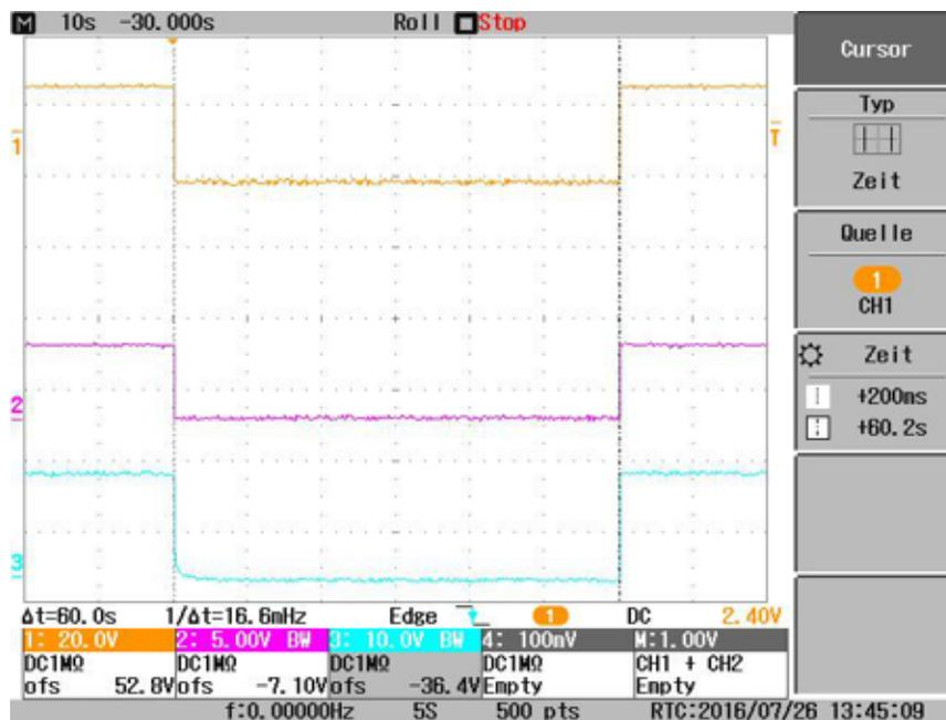
Figure 81. Outputs of Power Rails During Reversed voltage Test
