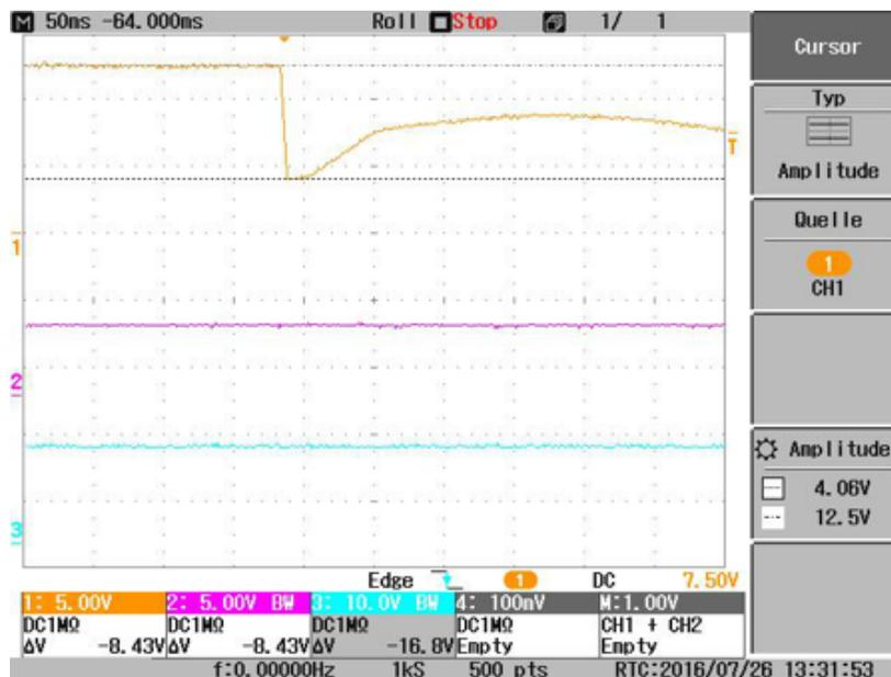
Figure 84. Expanded Time Scale at Beginning of Cold Cranking Pulse (Level 2)
