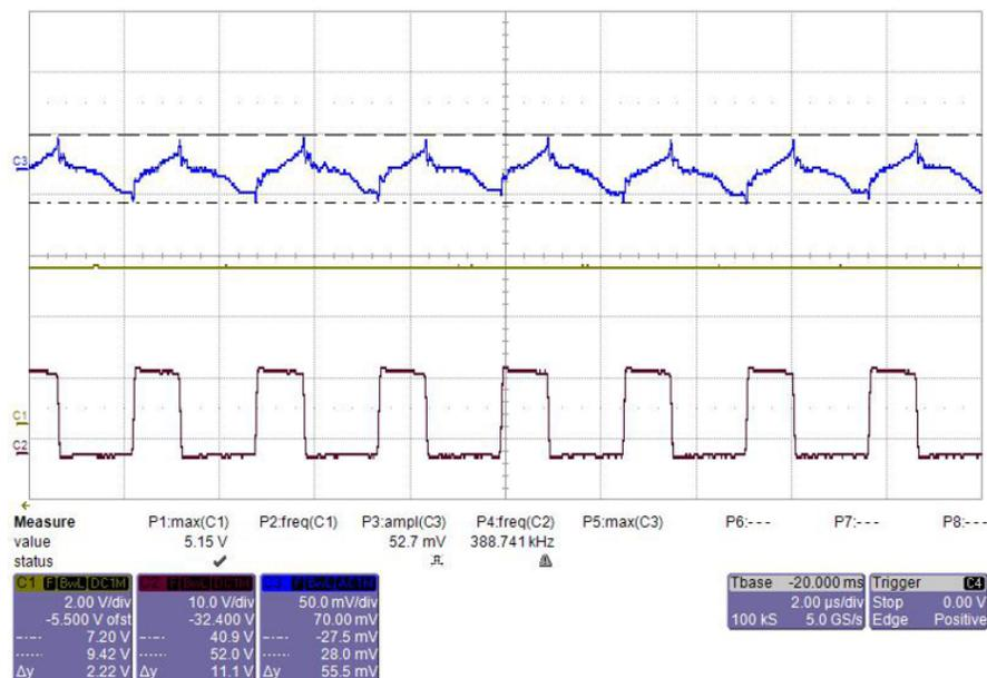
Figure 31. Output Voltage Ripple of Buck Converter Under  $V_{IN} = 15\text{ V}$  and  $I_{OUT} = 4.1\text{ A}$
