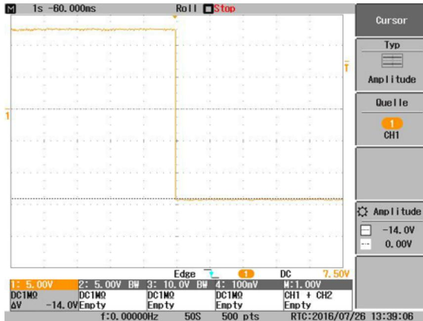
Figure 80. Applied Reversed Voltage Waveform
