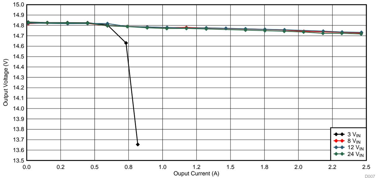
Figure 22. Load Regulation of Buck-Boost Converter
