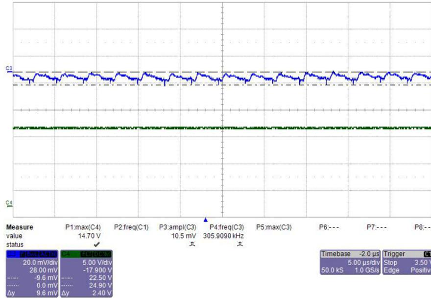
**Figure 28. Output Voltage Ripple of Buck-Boost Converter Under  $V_{IN} = 13\text{ V}$  and  $I_{OUT} = 0.1\text{ A}$**
