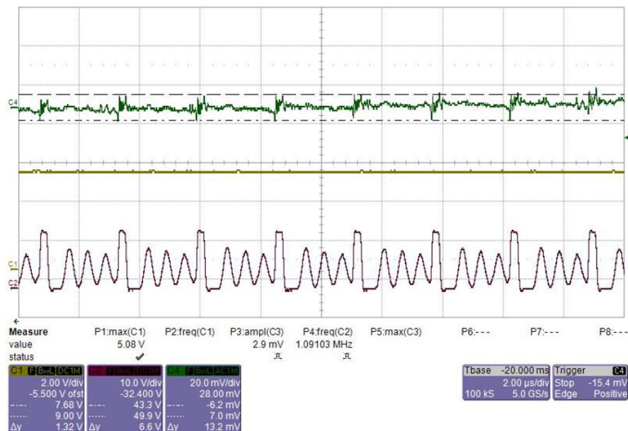
Figure 30. Output Voltage Ripple of Buck Converter Under  $V_{IN} = 15\text{ V}$  and  $I_{OUT} = 0.1\text{ A}$
