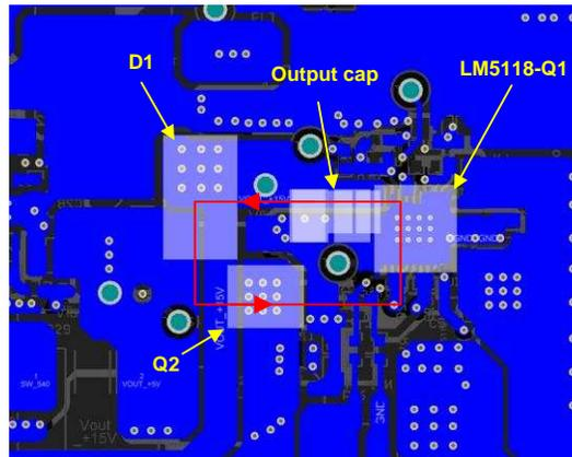
**Figure 120. Boost Switching Loop of LM5118-Q1**
