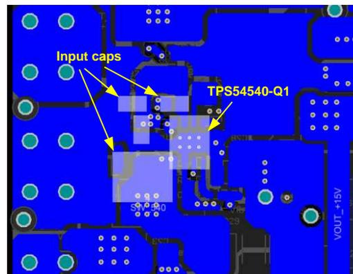
**Figure 121. Place Input Capacitors Close to Buck Converter**
