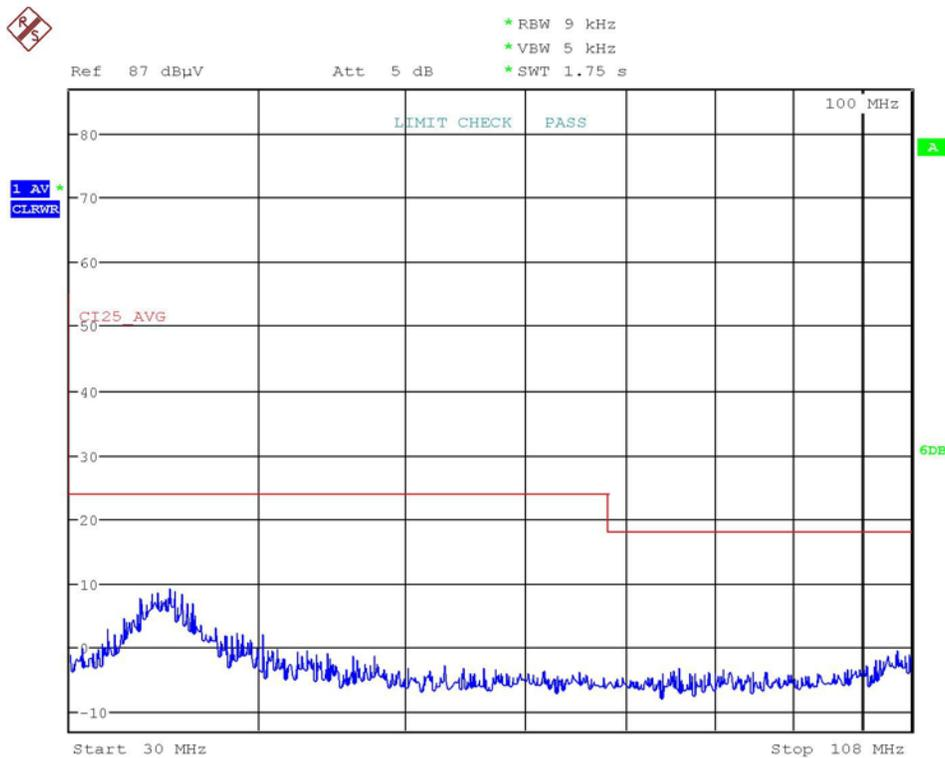
**Figure 105. Measured Average Noise of Test Circuit 4 (30 to 108 MHz, Limit Line: CISPR 25 Class 5 Average, Limit Check: Pass)**
