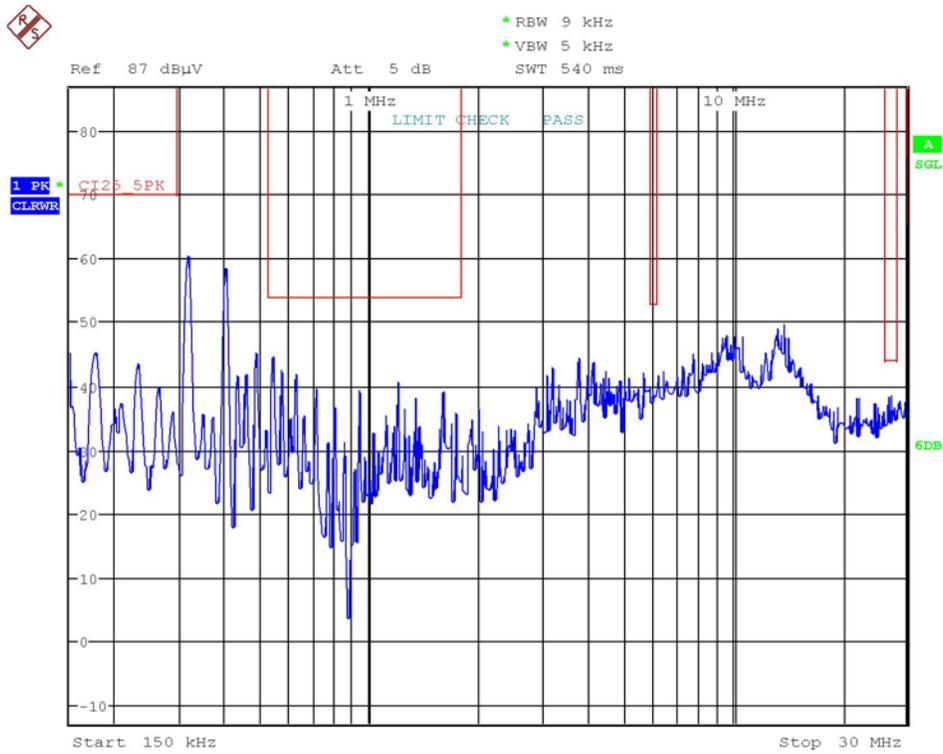
**Figure 98. Measured Peak Noise of Test Circuit 2 (150 kHz to 30 MHz, Limit Line: CISPR 25 Class 5 Peak, Limit Check: Pass)**
