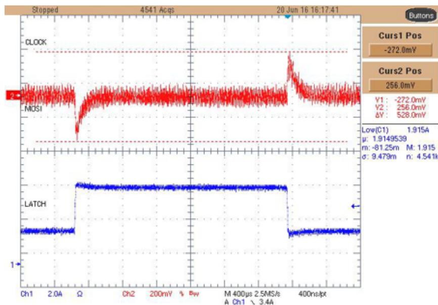
Figure 36. Load Transient Response of Buck Converter Under  $V_{IN} = 13\text{ V}$  and  $I_{OUT}$  Switching Between 4.7 A and 2 A
