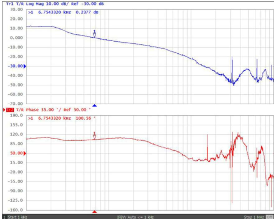
**Figure 55. Loop Frequency Response of Buck-Boost Converter With  $V_{IN} = 24\text{ V}$  and  $I_{OUT} = 0.5\text{ A}$**
