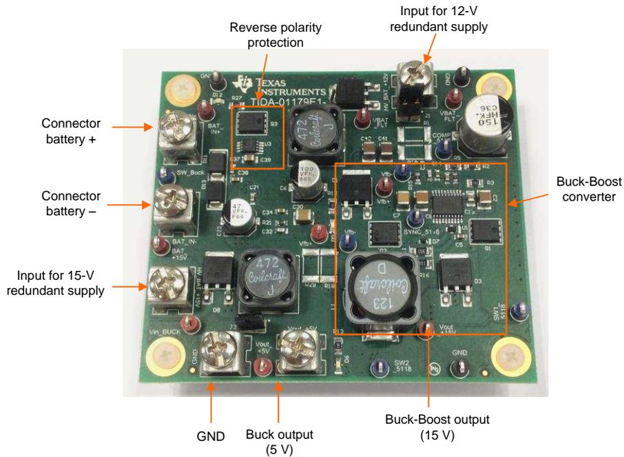
Figure 12. TIDA-01179 PCB Board Top Side
