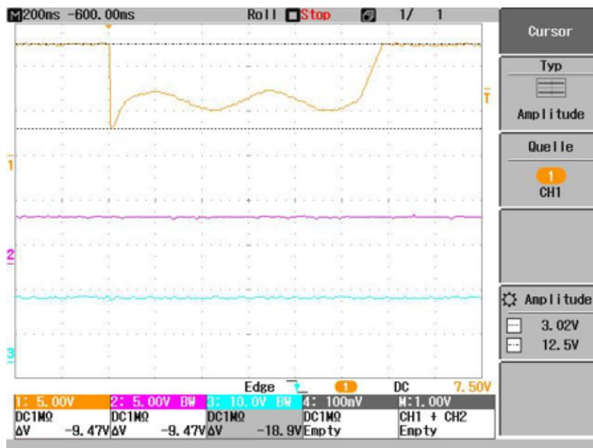
Figure 86. Outputs of Power Rails During Severe Cold Cranking Test (Level 3)
