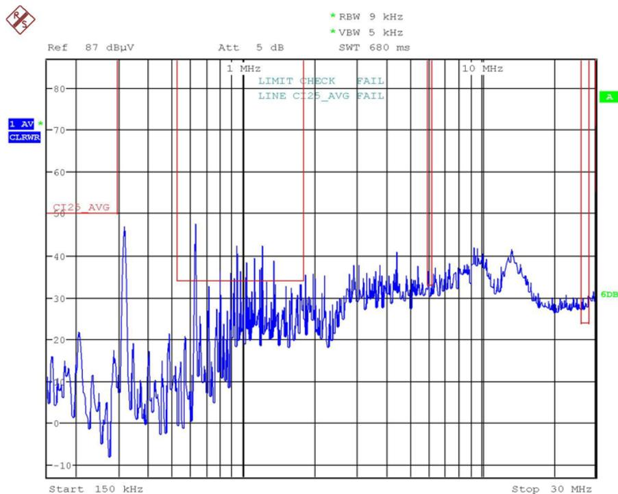
**Figure 109. Measured Average Noise of Test Circuit 1 (150 kHz to 30 MHz, Limit Line: CISPR 25 Class 5 Average, Limit Check: Fail)**
