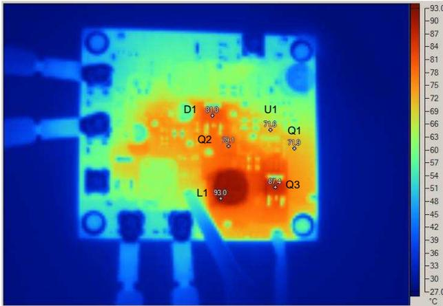
Figure 40. Thermal Image of Board Top Side With  $V_{IN} = 13\text{ V}$  and  $P_{OUT} = 31.55\text{ W}$
