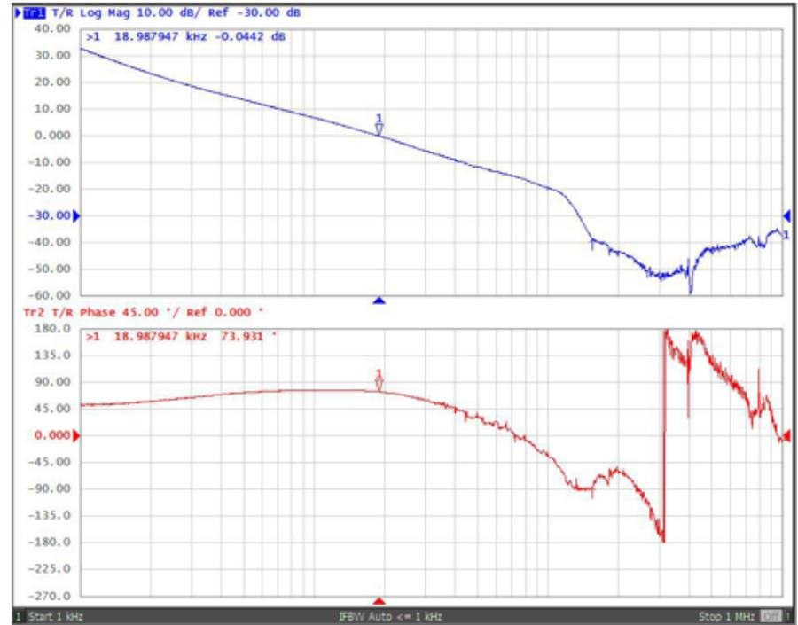
**Figure 62. Loop Frequency Response of Buck Converter With  $V_{IN} = 15\text{ V}$  and  $I_{OUT} = 4\text{ A}$**
