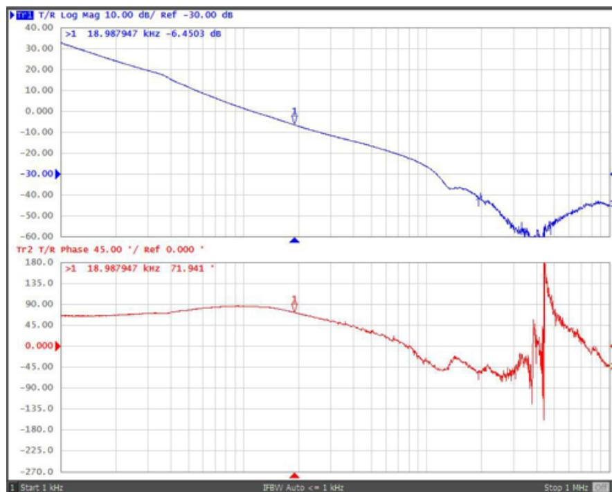
Figure 63. Loop Frequency Response of Buck Converter With  $V_{IN} = 9\text{ V}$  and  $I_{OUT} = 1\text{ A}$
