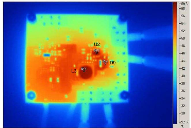
**Figure 47. Thermal Image of Board Bottom Side With  $V_{IN} = 24\text{ V}$  and  $P_{OUT} = 20\text{ W}$**
