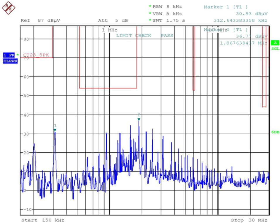
Figure 102. Measured Peak Noise of Test Circuit 4 (150 kHz to 30 MHz, Limit Line: CISPR 25 Class 5 Peak, Limit Check: Pass)
