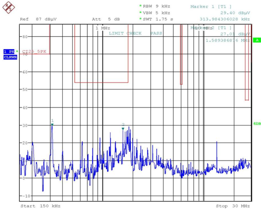
**Figure 112. Measured Peak Noise of Test Circuit 2 (150 kHz to 30 MHz, Limit Line: CISPR 25 Class 5 Peak, Limit Check: Pass)**
