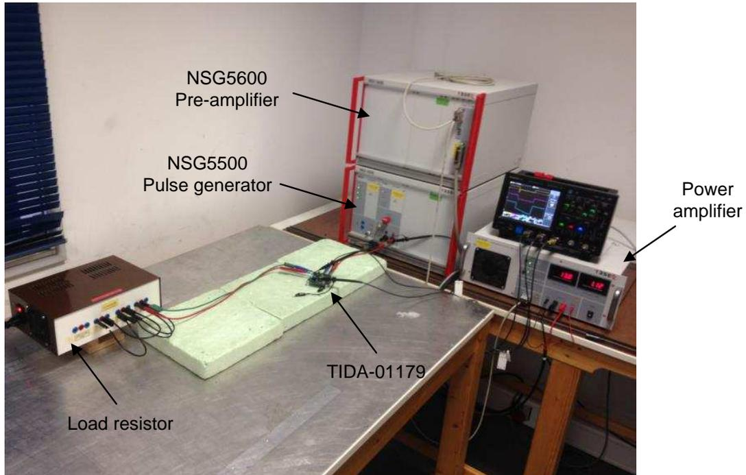
**Figure 65. Measurement Setup for Electrical Transients Test**
