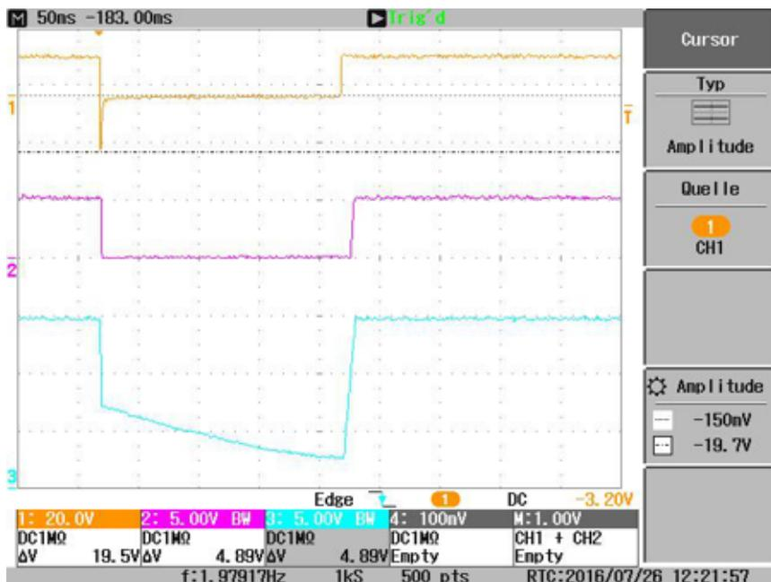
Figure 67. Outputs of Power Rails During Pulse 1 Test
