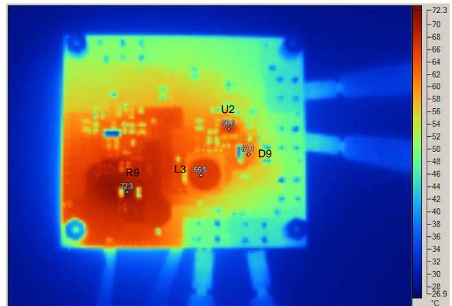
Figure 43. Thermal Image of Board Bottom Side With  $V_{IN} = 13\text{ V}$  and  $P_{OUT} = 20\text{ W}$
