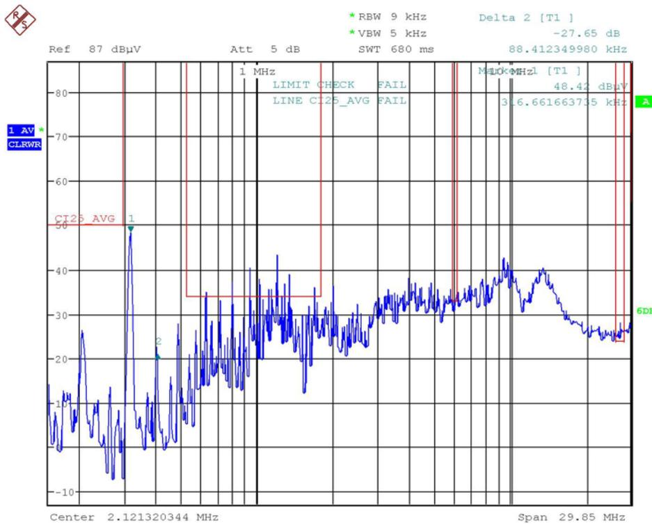
**Figure 95. Measured Average Noise of Test Circuit 1 (150 kHz to 30 MHz, Limit Line: CISPR 25 Class 5 Average, Limit Check: Fail)**
