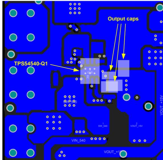
Figure 122. Place Output Capacitors Close to Buck Converter
