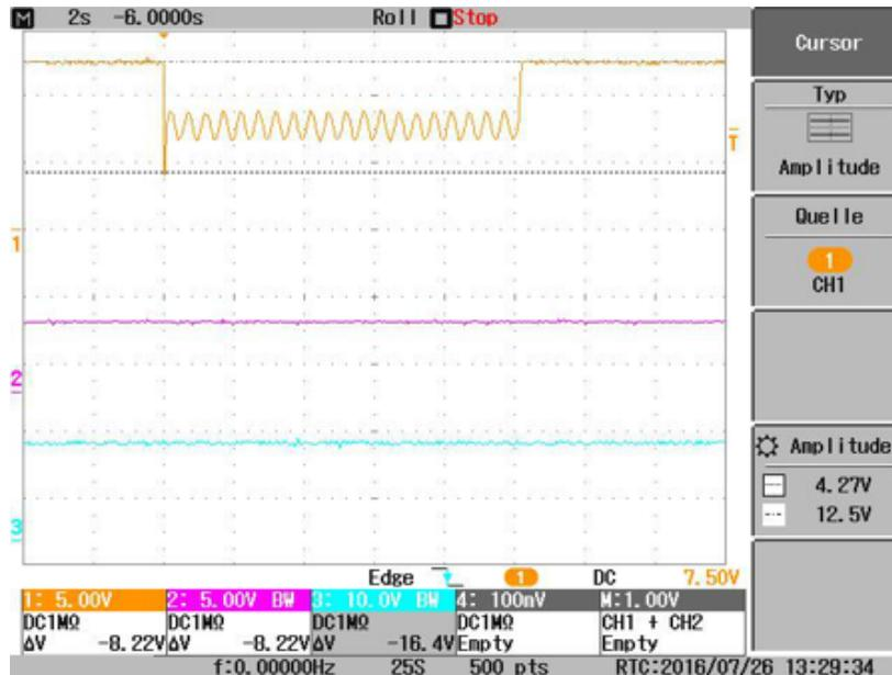
Figure 83. Cold Cranking Test Pulse (Level 2)
