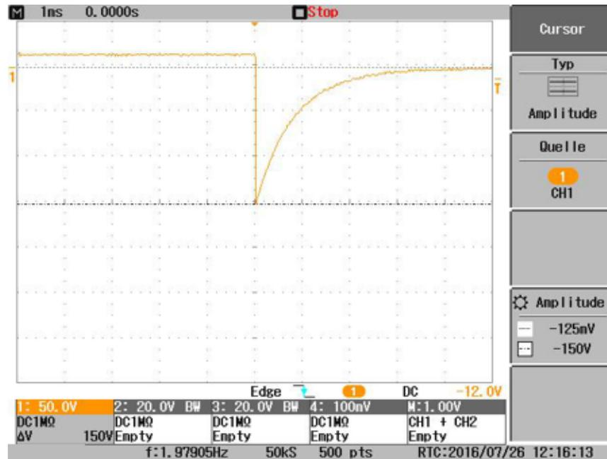
Figure 66. Pulse 1 Test Pulse
