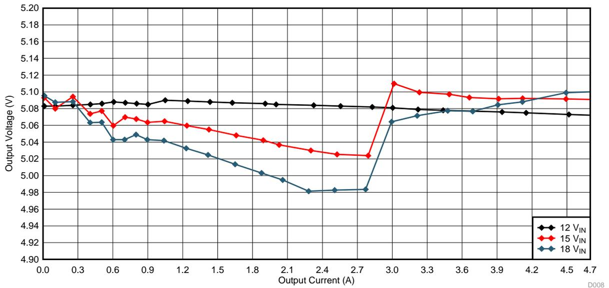
Figure 23. Load Regulation of Buck Converter
