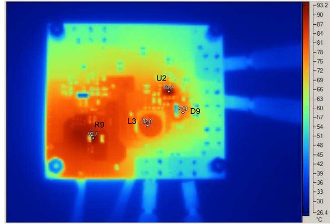
Figure 41. Thermal Image of Board Bottom Side With  $V_{IN} = 13\text{ V}$  and  $P_{OUT} = 31.55\text{ W}$
