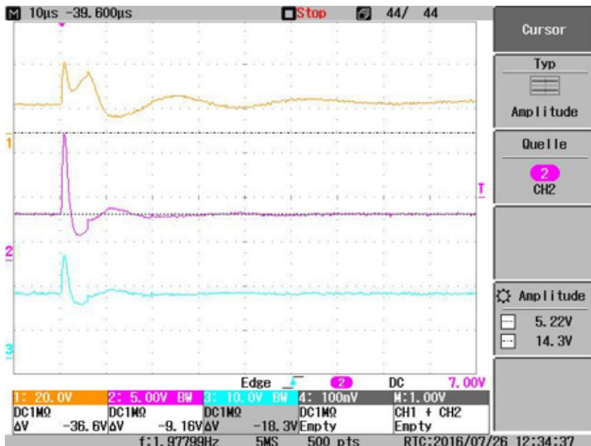
Figure 70. Outputs of Power Rails During Pulse 2a Test
