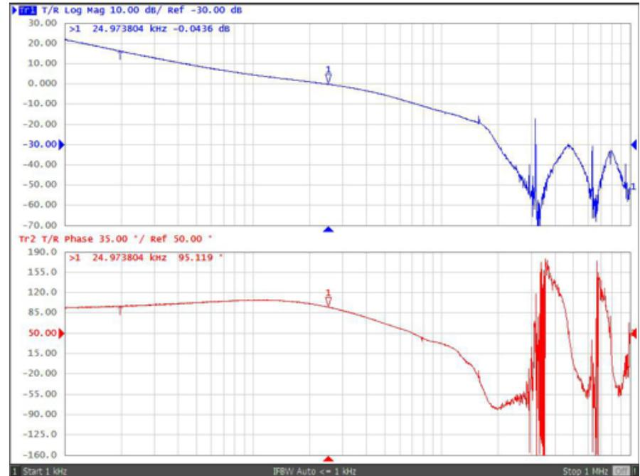
**Figure 56. Loop Frequency Response of Buck-Boost Converter With  $V_{IN} = 24\text{ V}$  and  $I_{OUT} = 2.2\text{ A}$**
