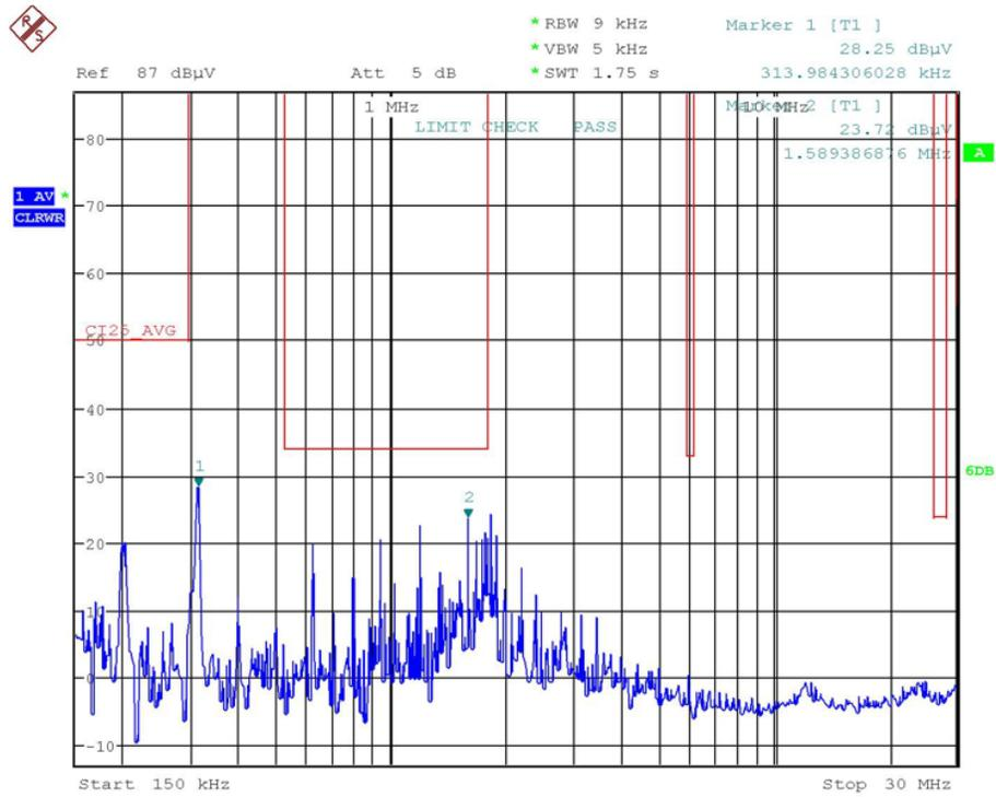
**Figure 114. Measured Average Noise of Test Circuit 2 (150 kHz to 30 MHz, Limit Line: CISPR 25 Class 5 Average, Limit Check: Pass)**
