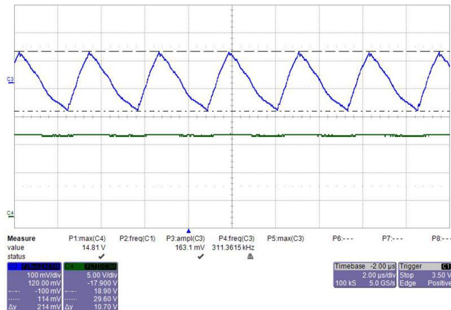
Figure 27. Output Voltage Ripple of Buck-Boost Converter Under  $V_{IN} = 8\text{ V}$  and  $I_{OUT} = 2.2\text{ A}$
