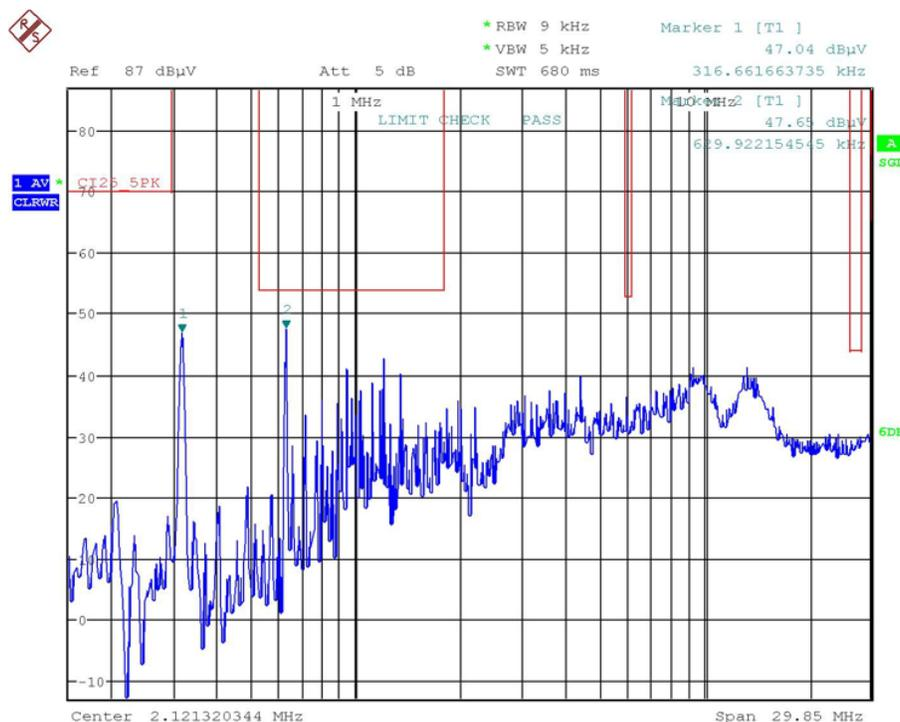
Figure 107. Measured Peak Noise of Test Circuit 1 (150 kHz to 30 MHz, Limit Line: CISPR 25 Class 5 Peak, Limit Check: Pass)
