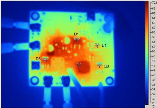
**Figure 44. Thermal Image of Board Top Side With  $V_{IN} = 24\text{ V}$  and  $P_{OUT} = 31.5\text{ W}$**
