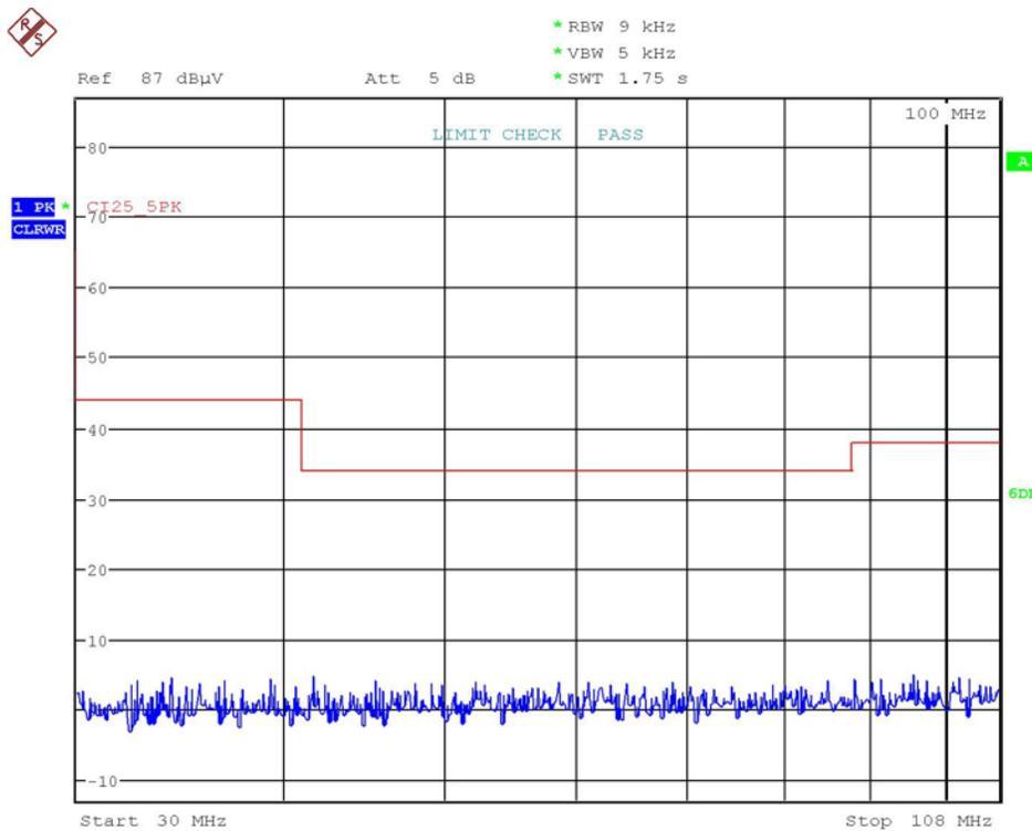
Figure 90. Ambient Noise (30 to 108 MHz)
