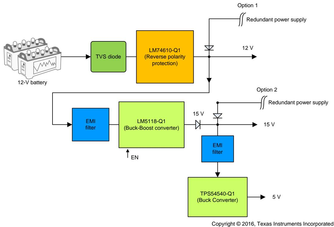
**Figure 2. TIDA-01179 Block Diagram**
