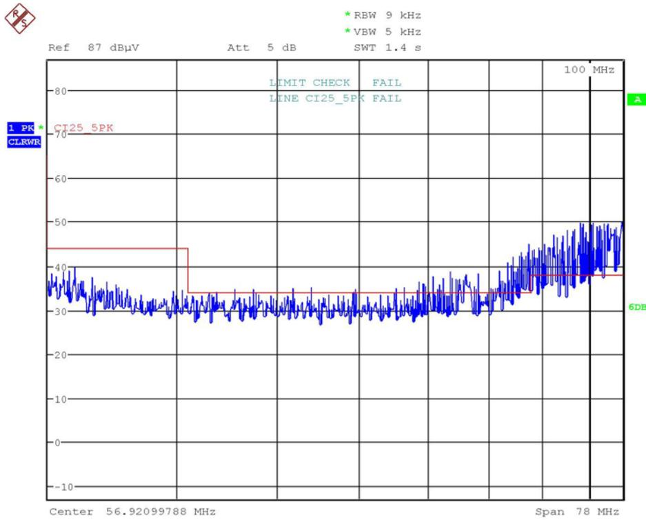
**Figure 94. Measured Peak Noise of Test Circuit 1 (30 to 108 MHz, Limit Line: CISPR 25 Class 5 Peak, Limit Check: Fail)**
