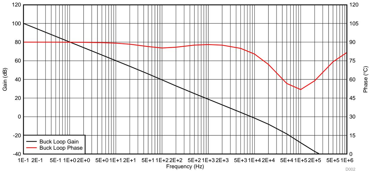
Figure 7. Calculated Loop Response of LM5118 Buck Modulator
