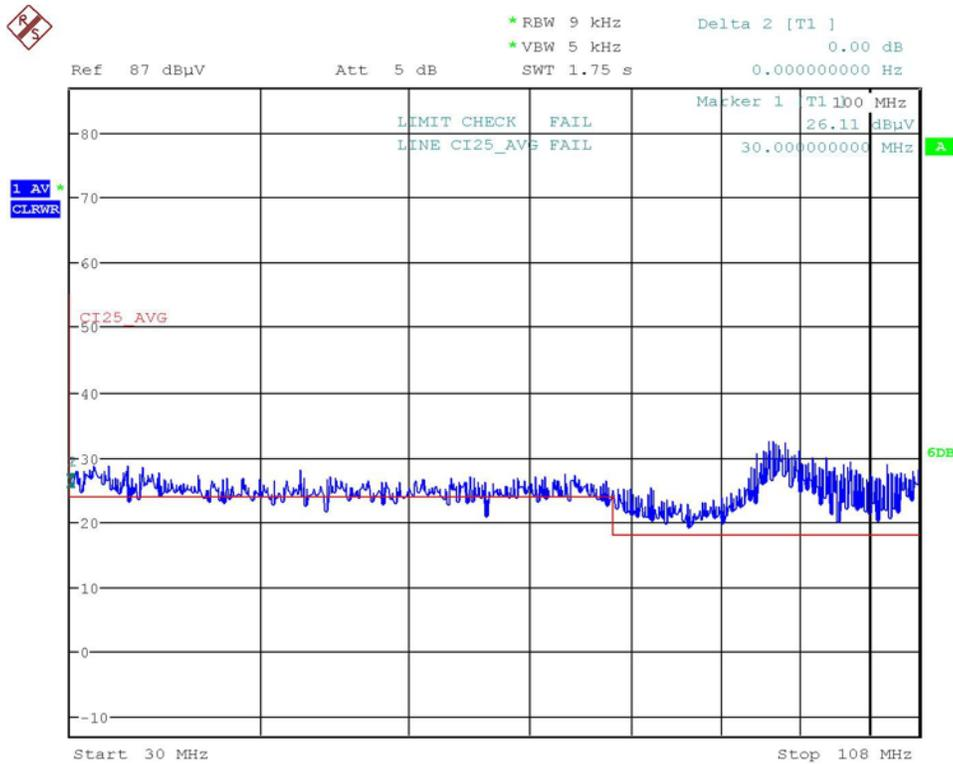
**Figure 96. Measured Average Noise of Test Circuit 1 (30 to 108 MHz, Limit Line: CISPR 25 Class 5 Average, Limit Check: Fail)**
