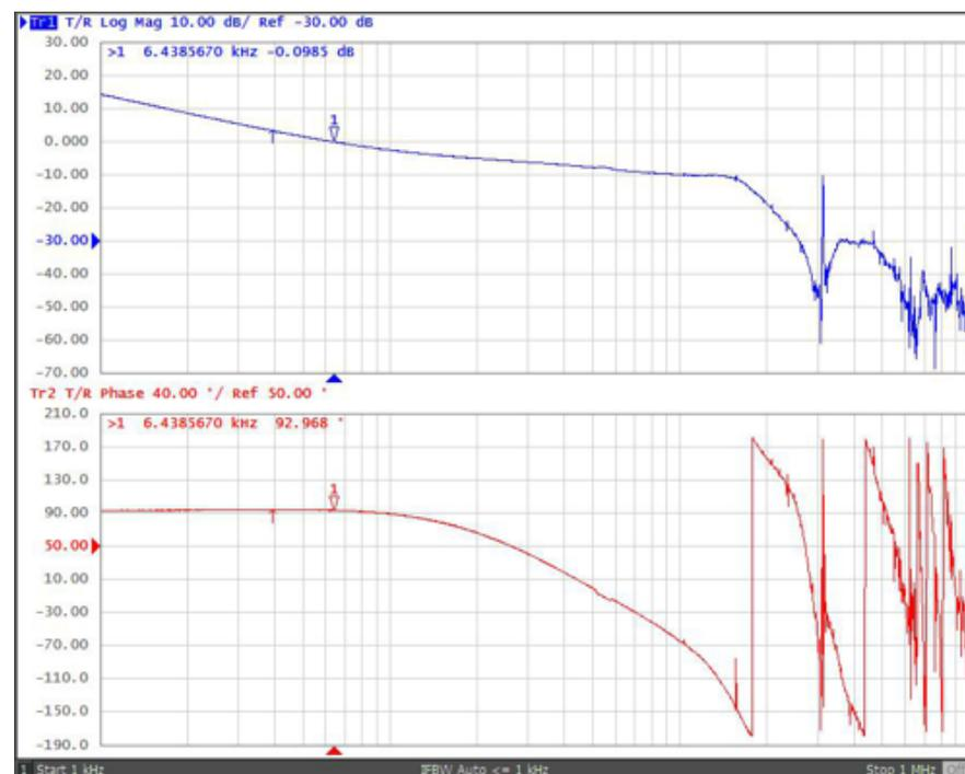
**Figure 54. Loop Frequency Response of Buck-Boost Converter With  $V_{IN} = 13\text{ V}$  and  $I_{OUT} = 2.2\text{ A}$**
