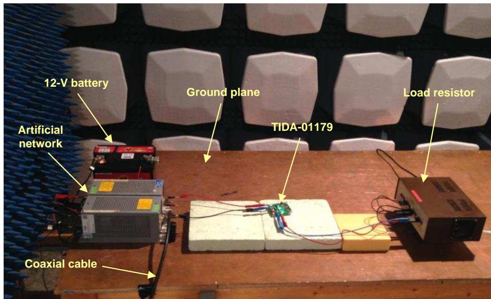
**Figure 88. Conducted Emission Measurement Setup**
