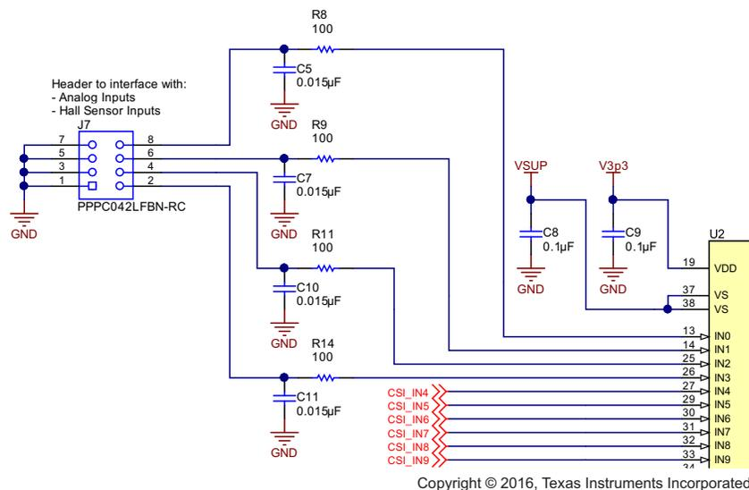
**Figure 15. J7 Input Schematic for External Analog and Digital Inputs**
