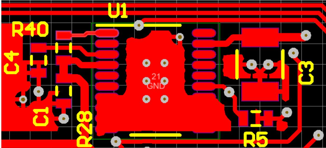
Figure 69. Voltage Regulator Capacitor Placement
