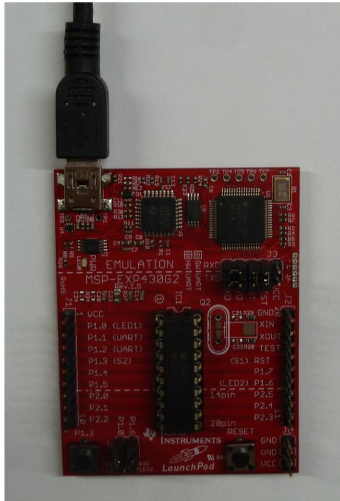
**Figure 23. MSP430™ LaunchPad™ USB Connection and Jumper Settings**
