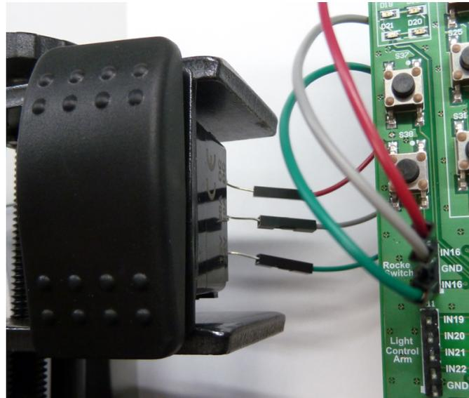
Figure 28. J8 External Rocker Switch Input Header
