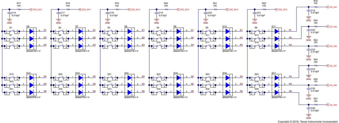
Figure 13. Matrix Configuration Switch Schematic
