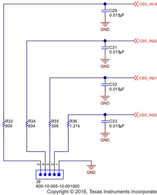
Figure 18. Light Control Arm Input Schematic
