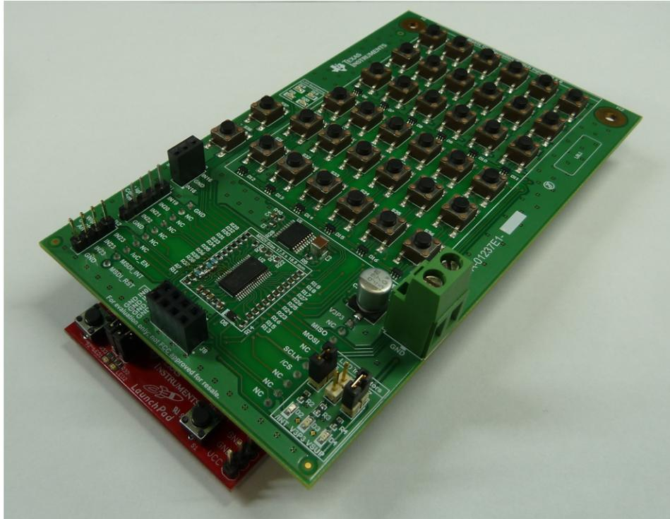
Figure 24. Orientation of TIDA-01237 Board on MSP430™ LaunchPad™
