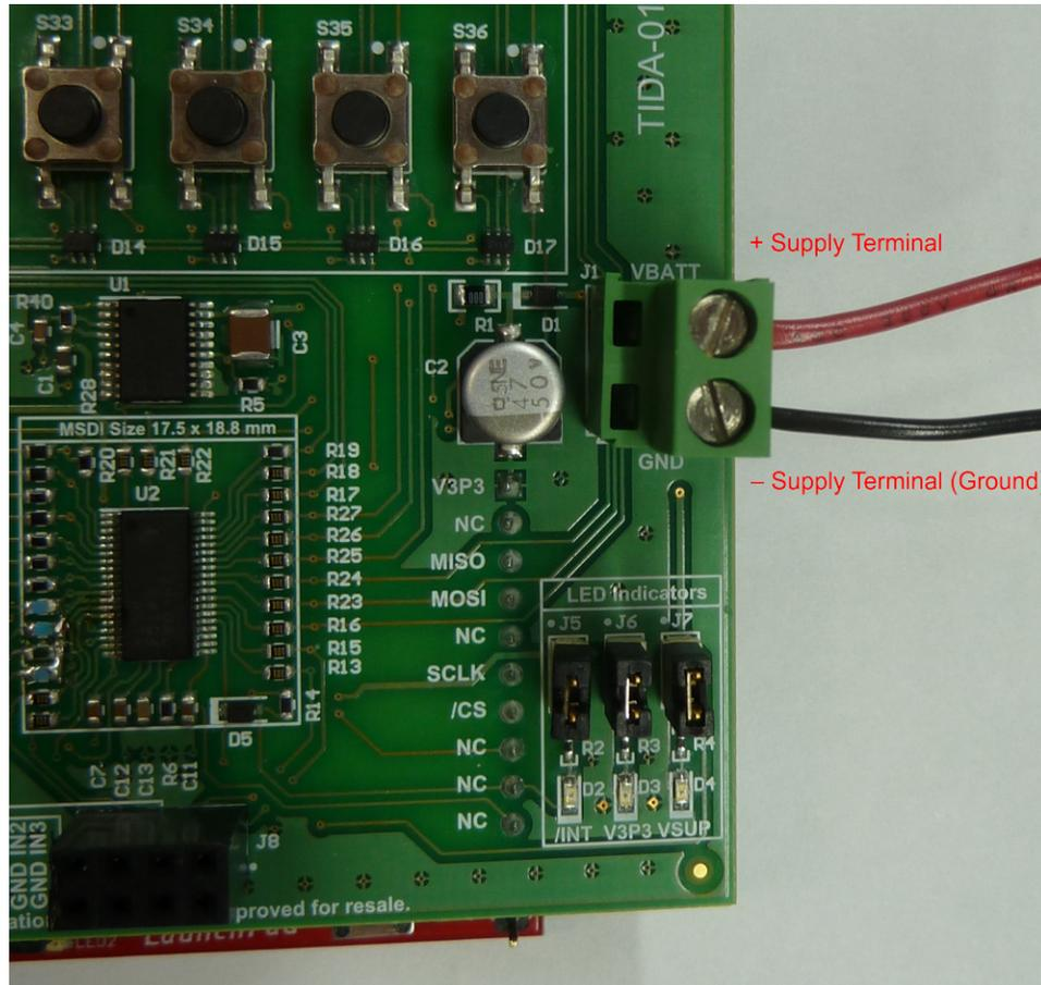
Figure 25. External Supply Connections
