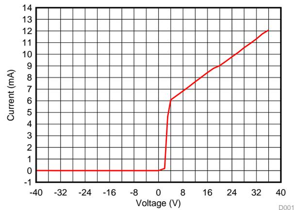
**Figure 34. Input Supply Voltage Versus Input Supply Current**
