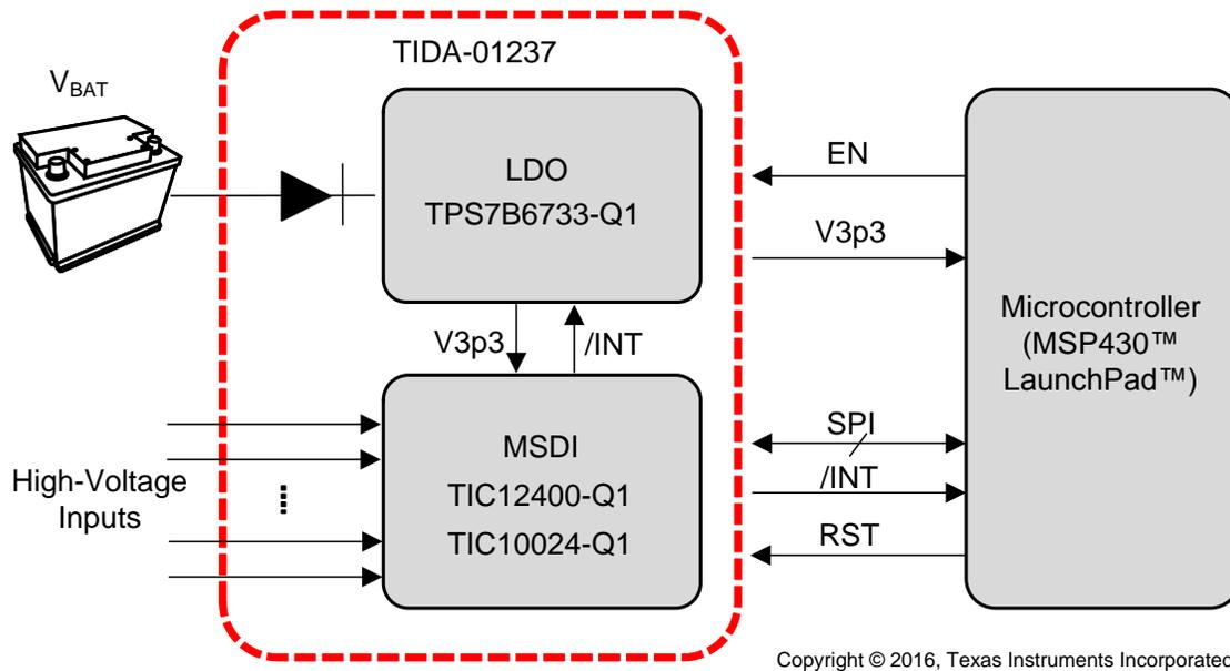
**Figure 1. TIDA-01237 Block Diagram**
