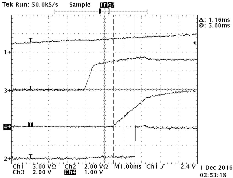
Figure 35. TPS7B6733-Q1 RESET Delay Function
