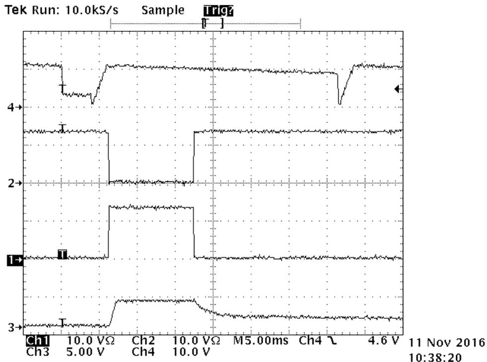
Figure 36. Power Supply Control for Ultra-Low-Power Sleep Mode
