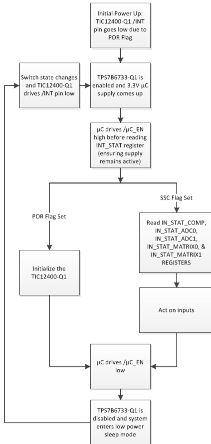
**Figure 11. Program Flow With Low-Power Sleep Mode**
