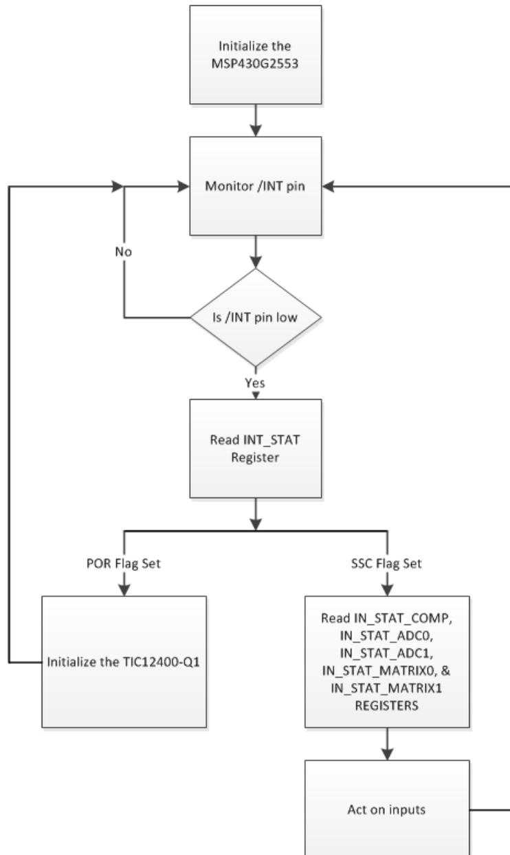
**Figure 12. Program Flow Without Low-Power Sleep Mode**
