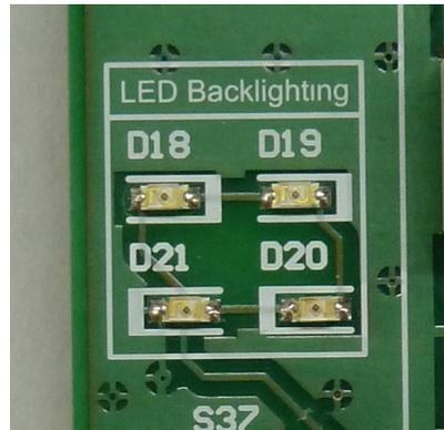
Figure 30. Button and Switch LED Backlighting
