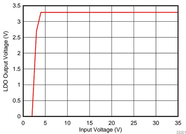
**Figure 33. Input Supply Voltage Versus 3.3-V Regulated Supply Voltage**
