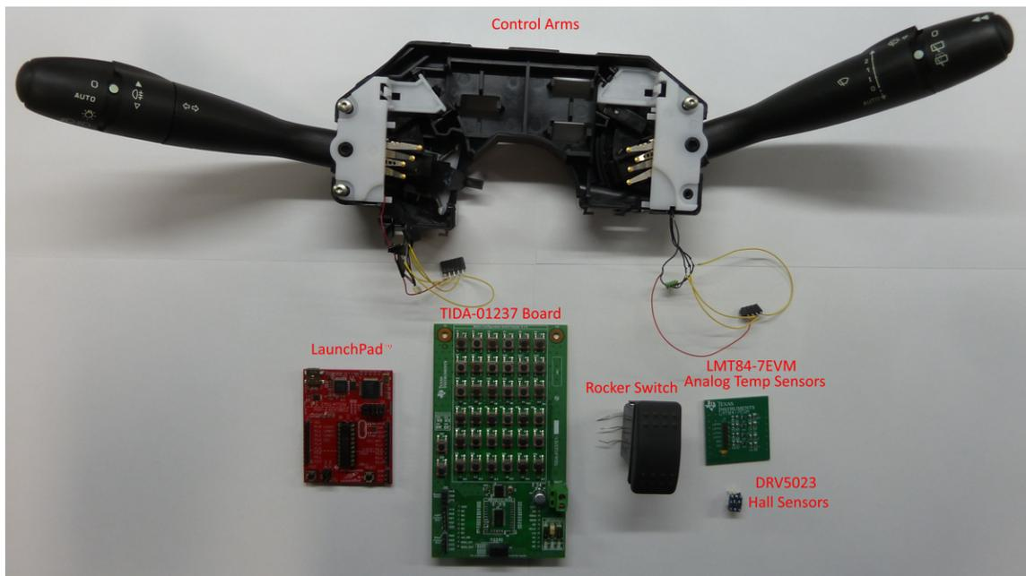
Figure 22. Hardware Test Setup
