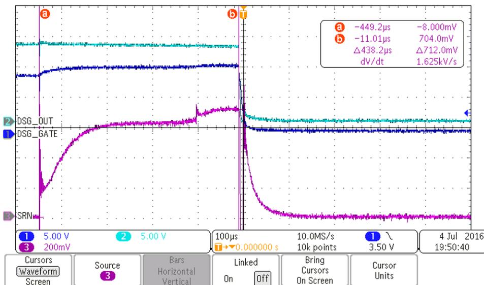
**Figure 17. Short Circuit Discharge Test Captured Plot**
