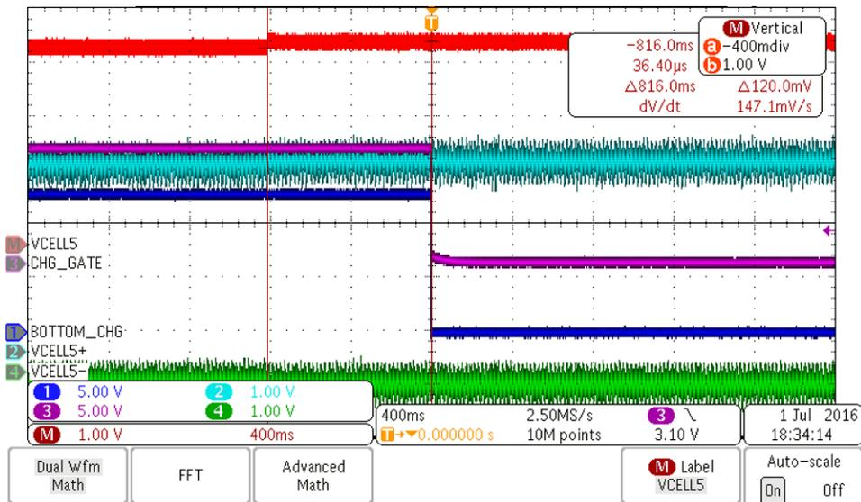
Figure 24. Bottom bq76930 OV Protection Test
