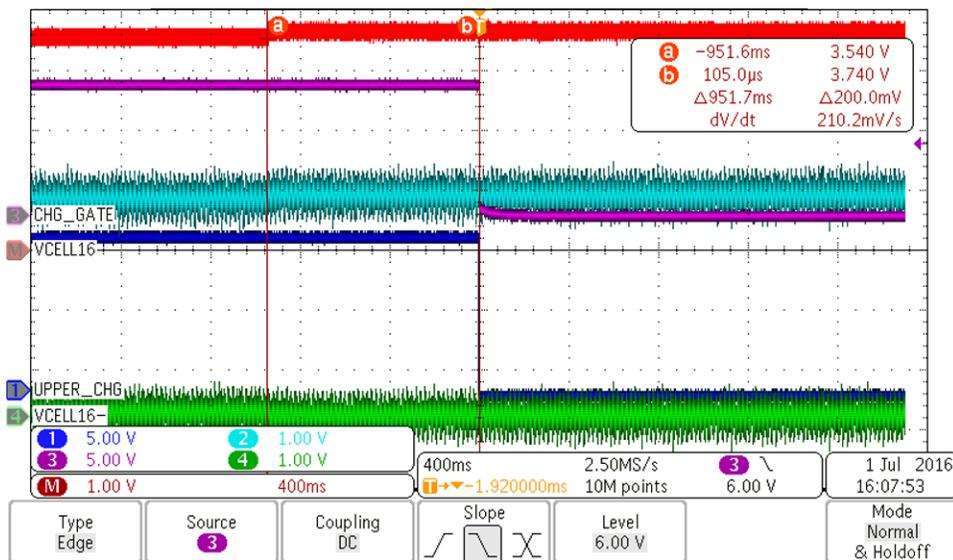
Figure 22. Upper bq76930 OV Protection Test
