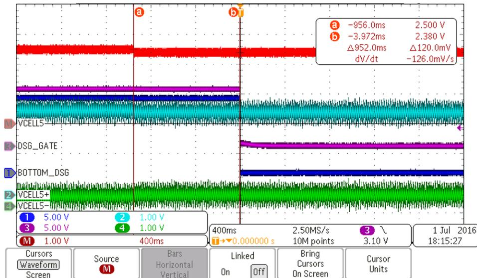
**Figure 28. Bottom bq76930 UV Protection Test**
