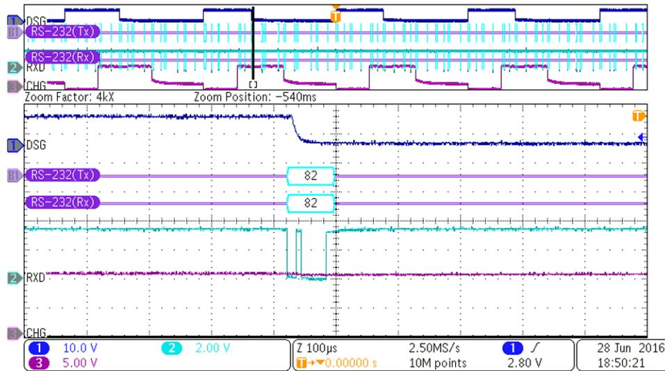
Figure 44. One Response Byte for UpperDsgFetOff
