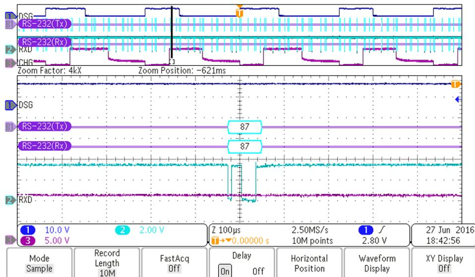
Figure 41. One Response Byte for BottomChgFetOn
