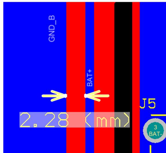
**Figure 49. Keep Enough Clearance Between BAT+ and GND\_B or BAT-**
