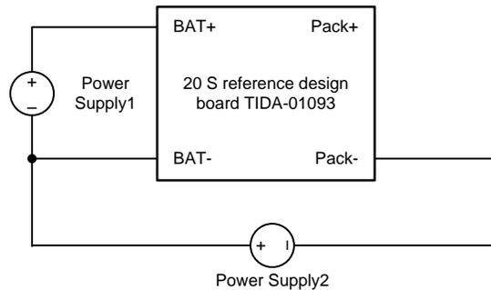
**Figure 13. Charger Detect Test**
