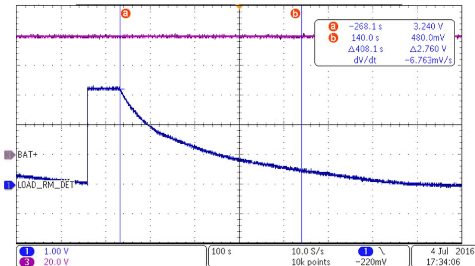
Figure 21. Load Removal Test 80-V Battery Voltage
