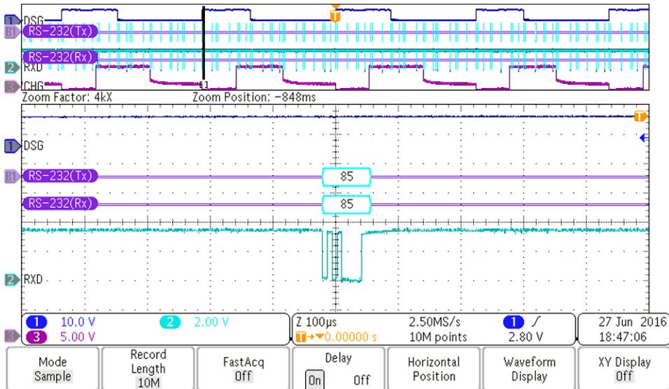
Figure 35. One Response Byte for BottomDsgFetOn
