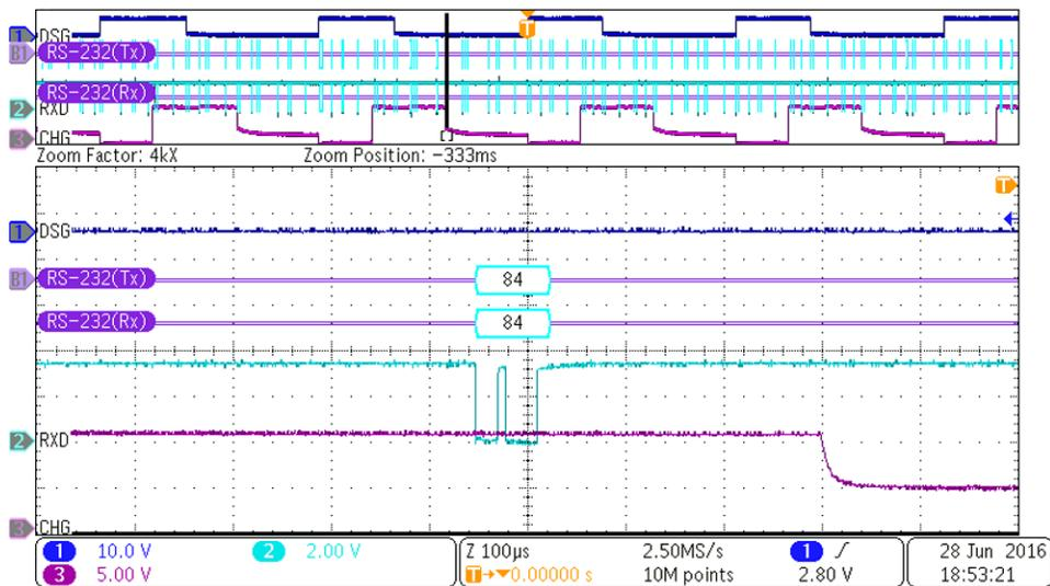
Figure 47. One Response Byte for UpperChgFetOff
