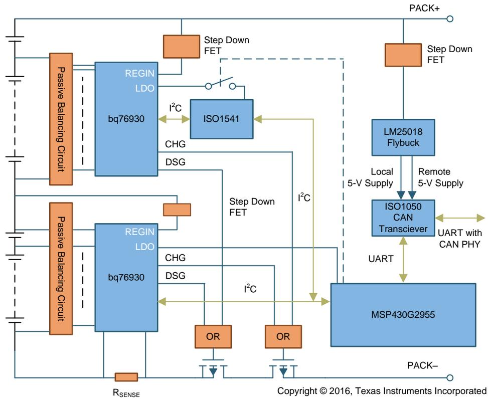
Figure 1. TIDA-01093 Block Diagram
