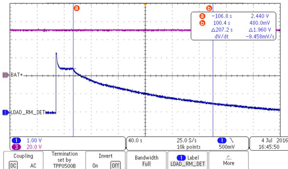
**Figure 19. Load Removal Test With 50-V Battery Voltage**
