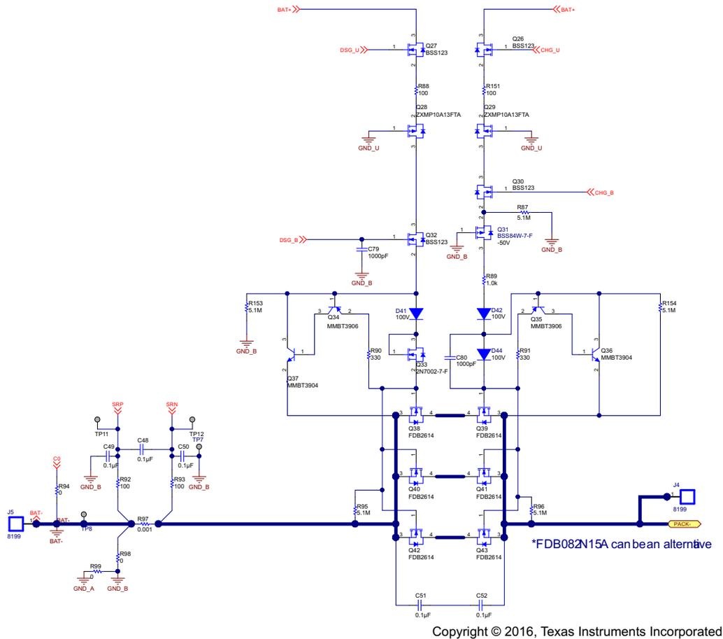
Figure 3. FETs Control Signal Schematic
