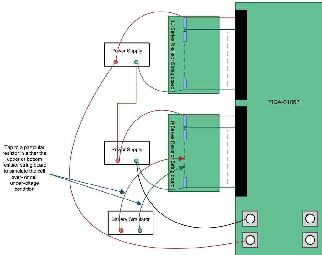
Figure 15. Cell OV or Cell UV Test Diagram
