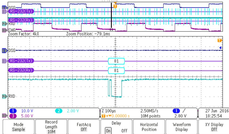
Figure 32. One Response Byte for UpperDsgFetOn
