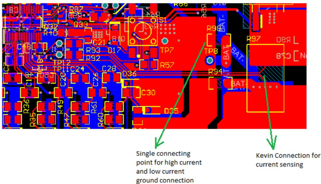
**Figure 48. Ground Connection and Current Sensing**
