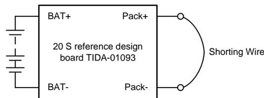
**Figure 12. Short Circuit Discharge Test**
