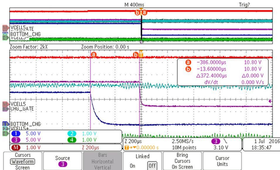
**Figure 25. Zoomed-in Plots for Bottom bq76930 OV Protection Test**
