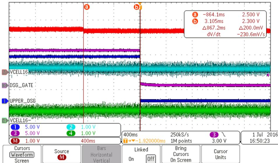
Figure 26. Upper bq76930 UV Protection Test
