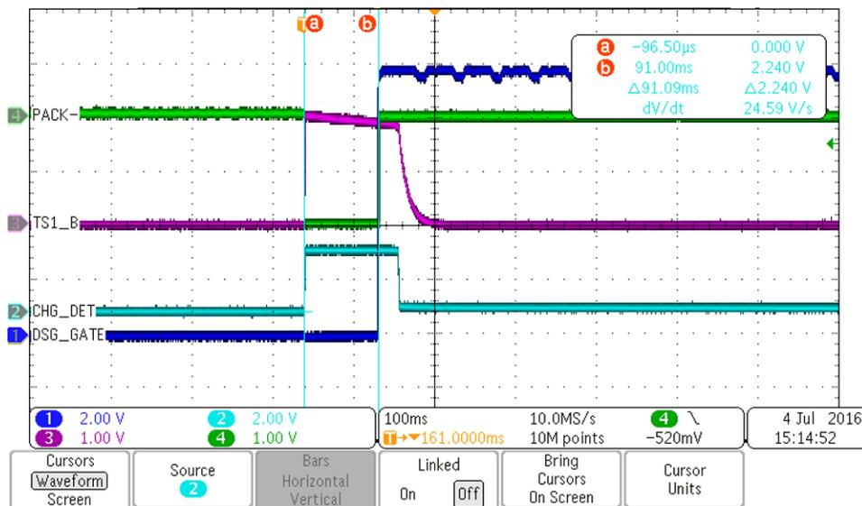
Figure 18. Typical Charger Detect Plot
