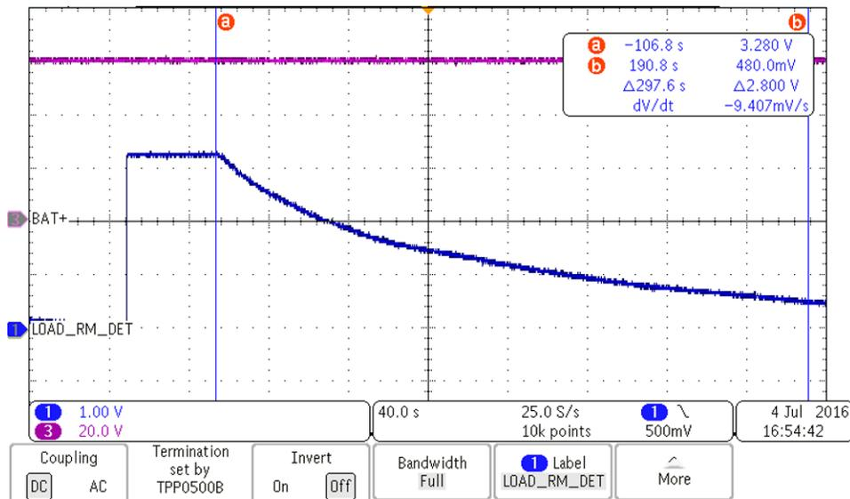
Figure 20. Load Removal Test With 60-V Battery Voltage
