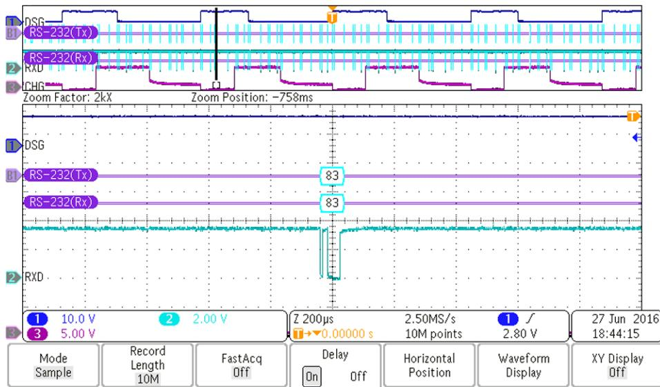
Figure 38. One Response Byte for UpperChgFetOn
