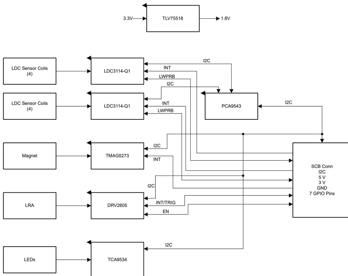
**Figure 2-1. TIDA-060039 Block Diagram**
