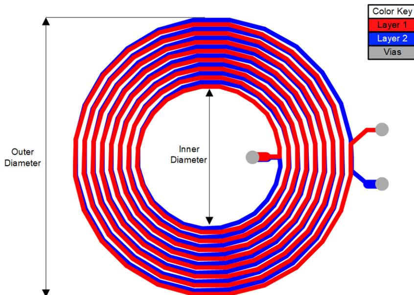
Figure 2-2. TIDA-060039 LDC Sensor Coil Layout
