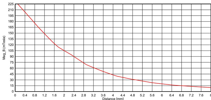
**Figure 2-5. Magnetic Field Strength Over Distance**
