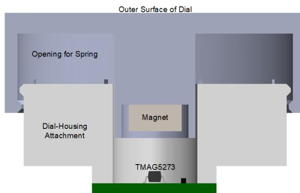
**Figure 2-6. Magnetic Dial Push Button Stackup**
