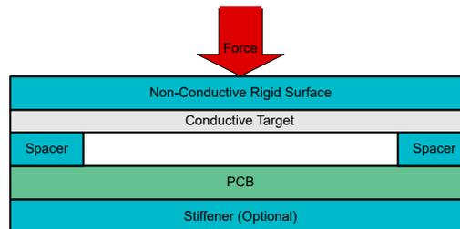
**Figure 2-4. Non-Conductive Touch Button Alternative Stackup Example**
