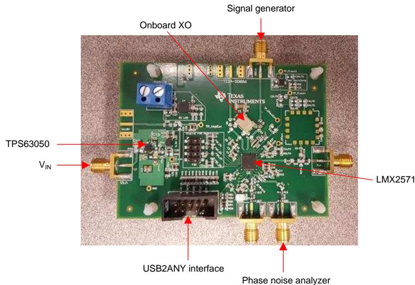
**Figure 2. TIDA-00886 Top View of PCB**
