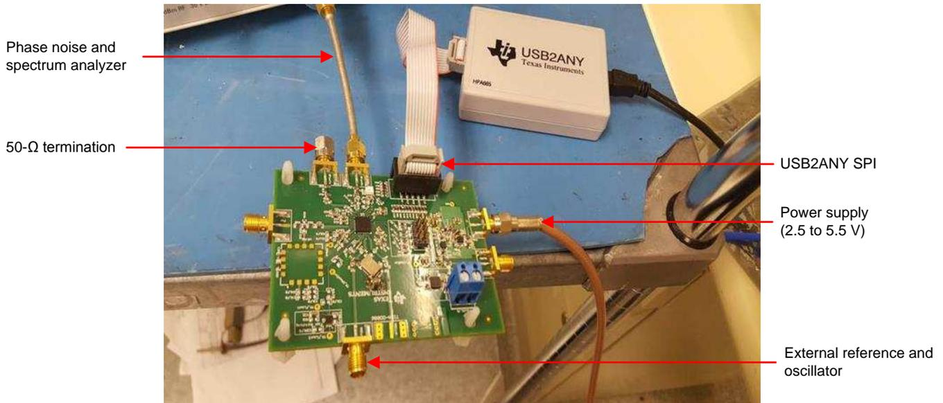
Figure 6. Test Setup Used in Lab For TIDA-00886
