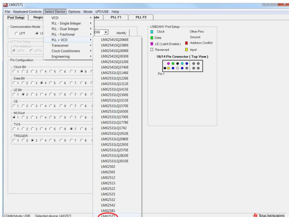
Figure 4. Selecting LMX2571 in Code Loader
