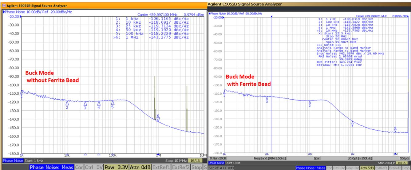
Figure 11. Spur Mitigation Using a Ferrite Bead
