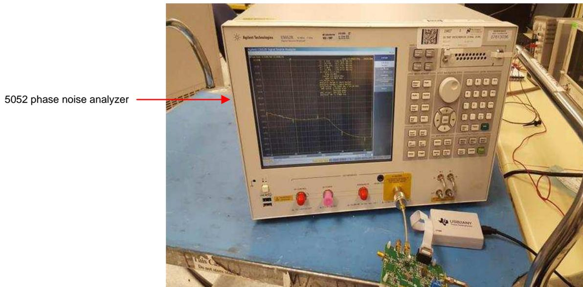
Figure 7. E5052 Phase Noise Analyzer
