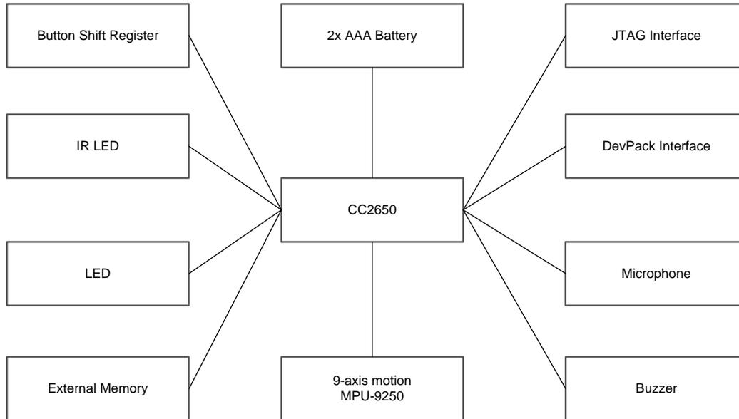
**Figure 1. CC2650 Remote Control Block Diagram**
