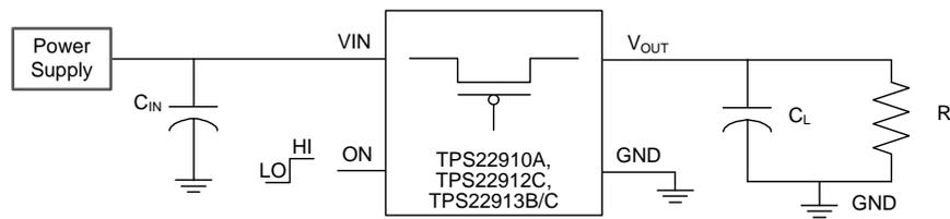
Figure 3. TPS22910A Simplified Schematic
