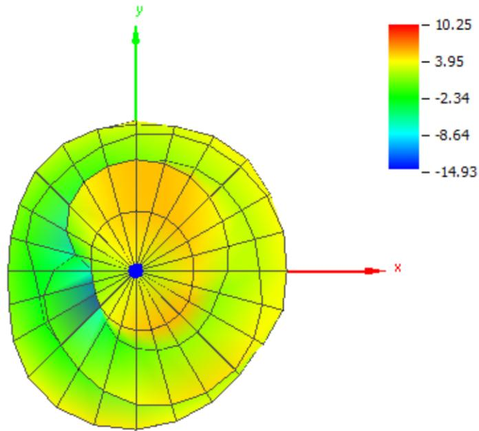
Figure 8. Radiation Pattern Plot Front
