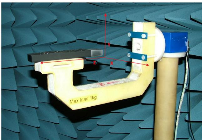
**Figure 6. DUT Mounted on Rotating Arm**
