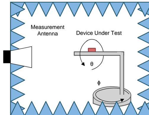
**Figure 5. Antenna Radiation Pattern**
