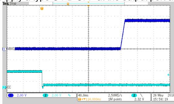
V<sub>in</sub>=6V and Attach the 5V UFP
