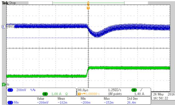
Vin=9V and Load switching from 25% to 50% Load
