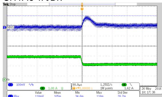
Vin=11.5V and Load switching from 75% to 50% Load
