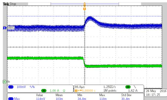
Vin=9V and Load switching from 75% to 50% Load
