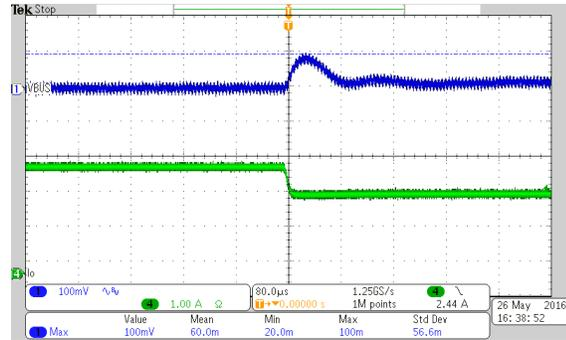
Vin=6V and Load switching from 100% to 75% Load
