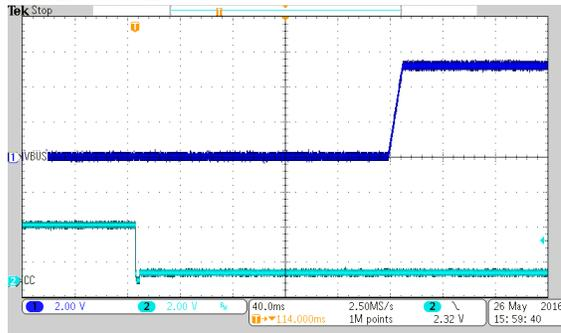
V<sub>in</sub>=9V and Attach the 5V UFP
