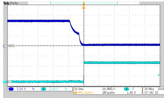
Vin=9V and Attach the 12V UFP
