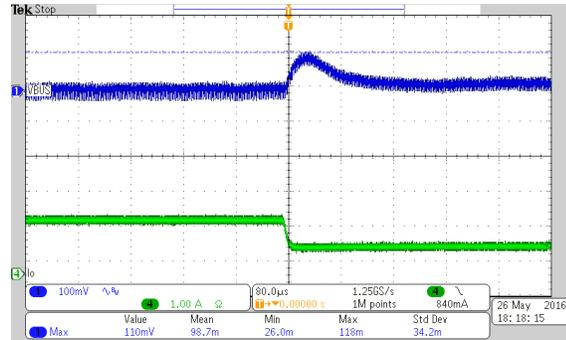
Vin=9V and Load switching from 50% to 25% Load
