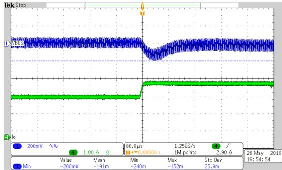
Vin=11.5V and Load switching from 75% to 100% Load
