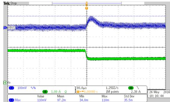
Vin=13.5V and Load switching from 100% to 75% Load
