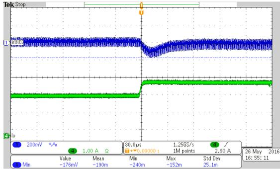
Vin=13.5V and Load switching from 75% to 100% Load
