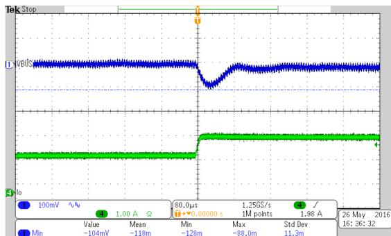
Vin=6V and Load switching from 50% to 75% Load
