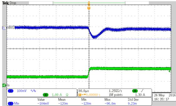
Vin=6V and Load switching from 25% to 50% Load
