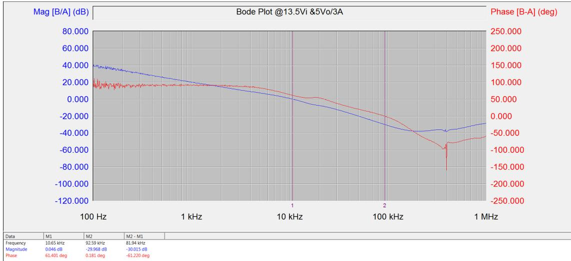
$V_{in}=13.5V$  and  $I_o=3A$
