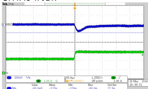
Vin=9V and Load switching from 50% to 75% Load
