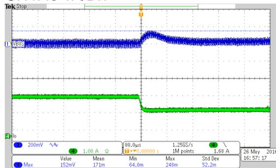
Vin=13.5V and Load switching from 75% to 50% Load
