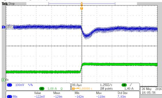
Vin=11.5V and Load switching from 25% to 50% Load
