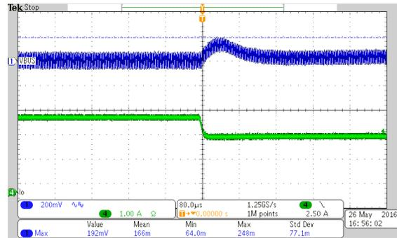
Vin=11.5V and Load switching from 100% to 75% Load
