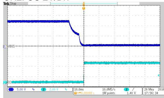
Vin=11.5V and Attach the 12V UFP
