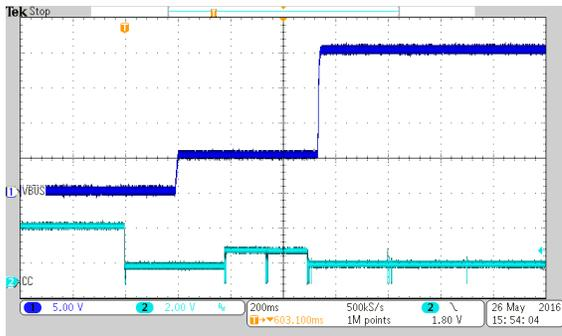
Vin=9V and Attach the 20V UFP
