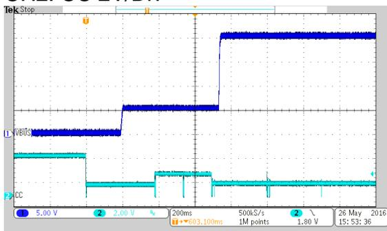
Vin=11.5V and Attach the 20V UFP
