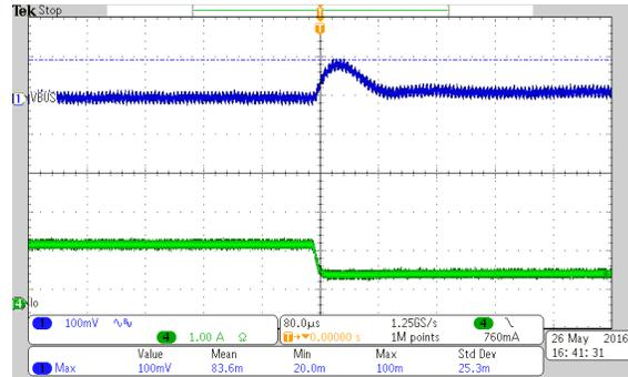
Vin=6V and Load switching from 50% to 25% Load
