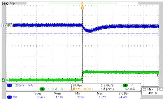
Vin=13.5V and Load switching from 0 to 25% Load
