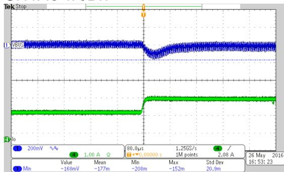
Vin=13.5V and Load switching from 50% to 75% Load
