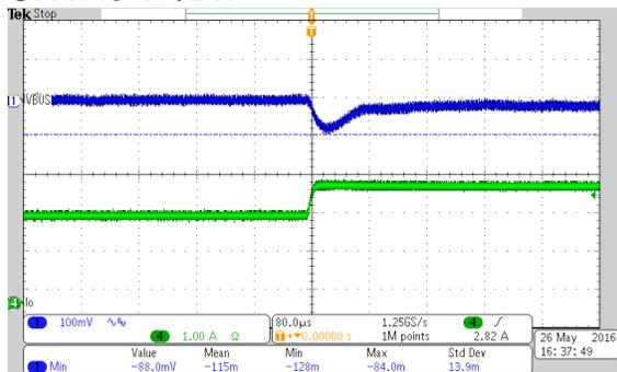
Vin=9V and Load switching from 75% to 100% Load
