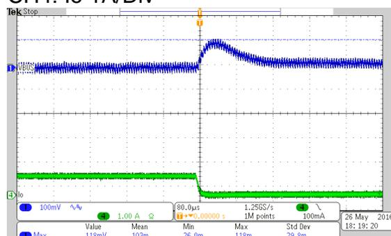
Vin=11.5V and Load switching from 25% to 0 Load
