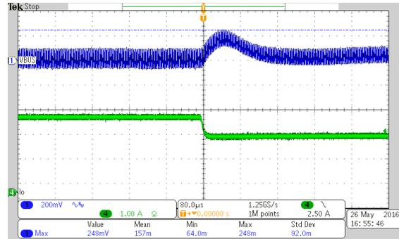
Vin=9V and Load switching from 100% to 75% Load
