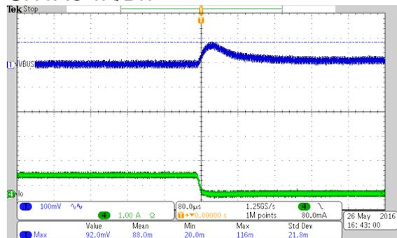
Vin=13.5V and Load switching from 25% to 0 Load
