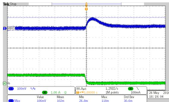
Vin=9V and Load switching from 25% to 0 Load
