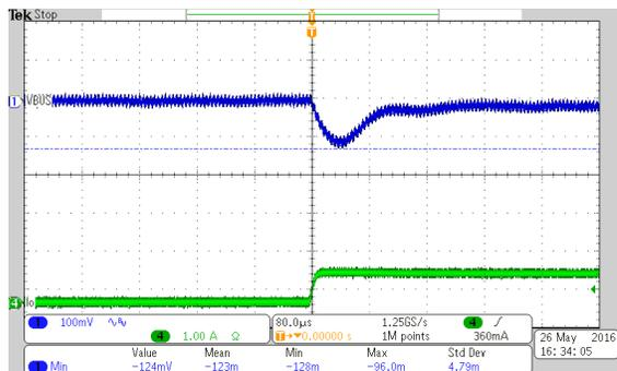
Vin=6V and Load switching from 0 to 25% Load
