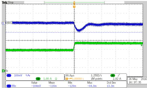
Vin=6V and Load switching from 75% to 100% Load
