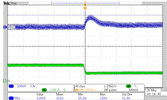
Vin=13.5V and Load switching from 50% to 25% Load
