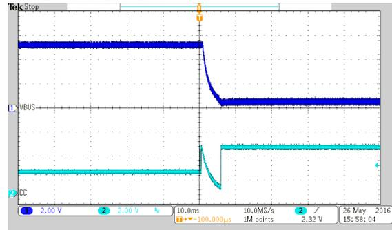
Vin=13.5V and Attach the 5V UFP
