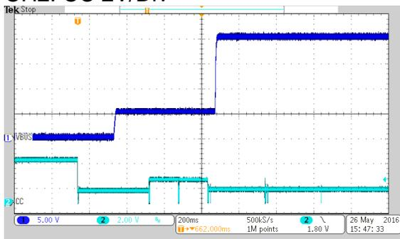
Vin=13.5V and Attach the 12V UFP
