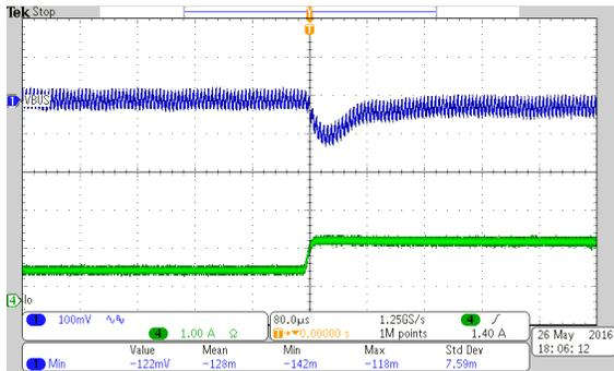
Vin=13.5V and Load switching from 25% to 50% Load
