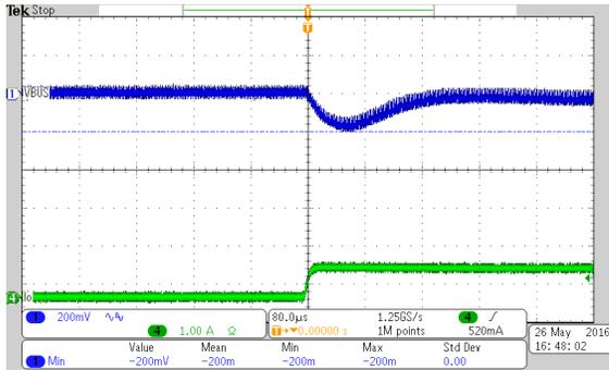
Vin=9V and Load switching from 0 to 25% Load
