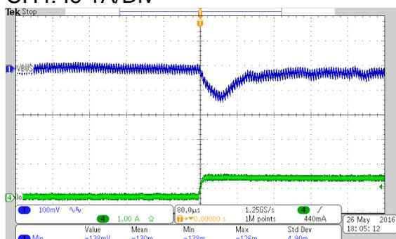
Vin=11.5V and Load switching from 0 to 25% Load
