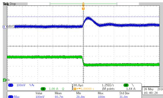
Vin=6V and Load switching from 75% to 50% Load
