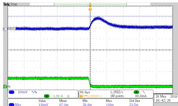
Vin=6V and Load switching from 25% to 0 Load
