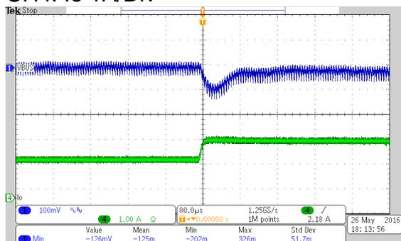
Vin=11.5V and Load switching from 50% to 75% Load
