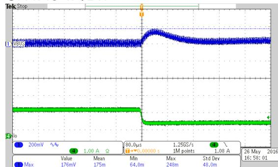
Vin=11.5V and Load switching from 50% to 25% Load
