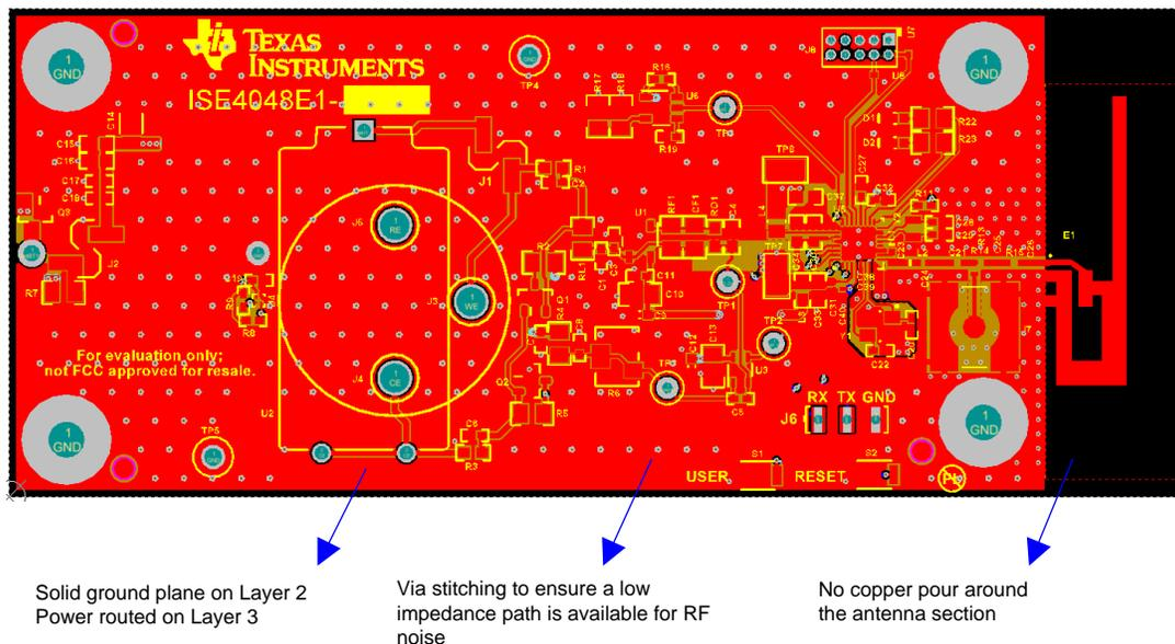
**Figure 40. Low-Power Carbon Monoxide Sensor Reference Design Layout Guidelines**
