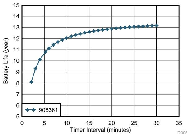
Figure 34. Battery Life versus Timer Interval
