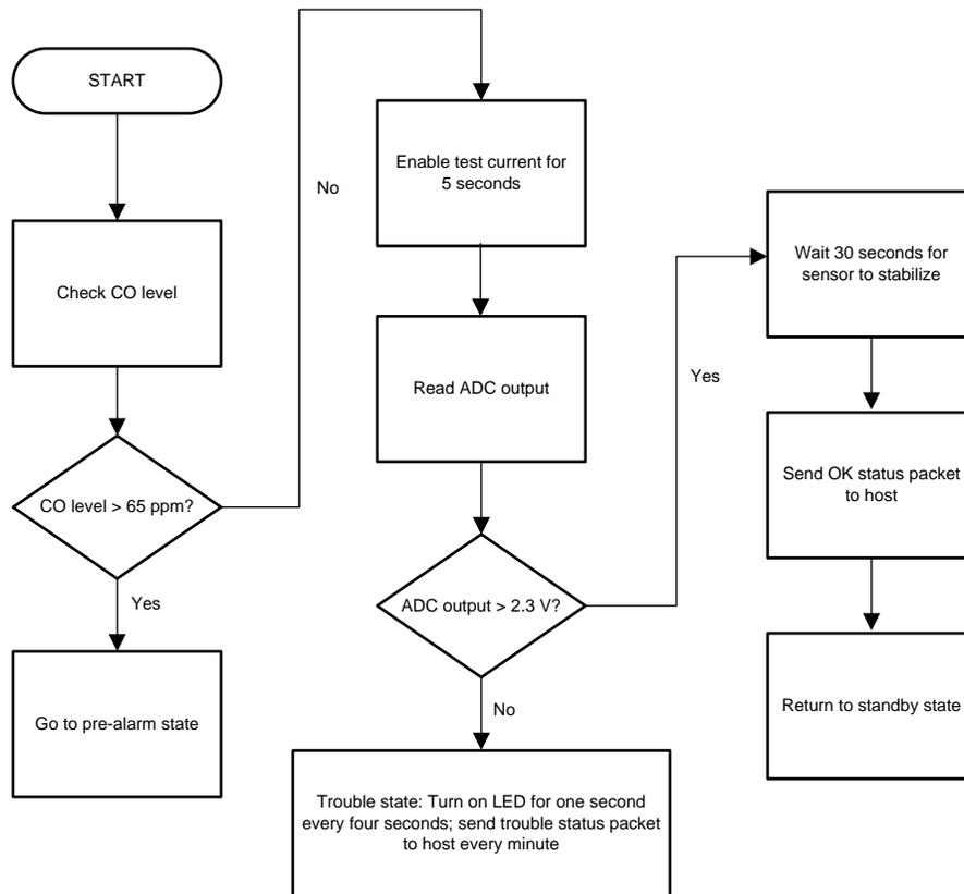
**Figure 14. Sensor Test Procedure**
