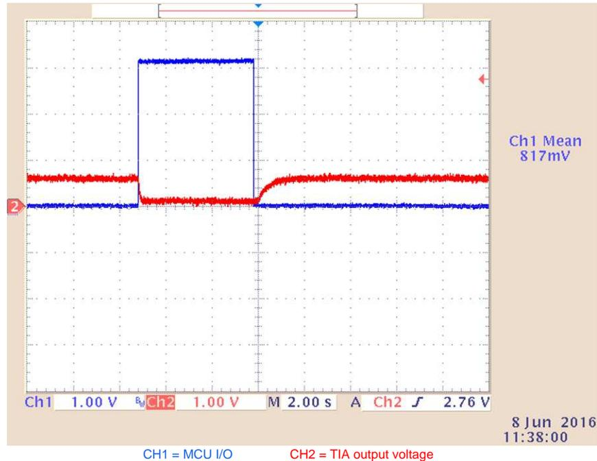
**Figure 8. Sensor in Short-Circuit**
