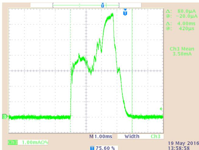
Figure 30. Transmit Current for Wireless Packet in Test State
