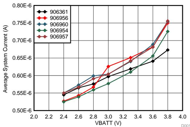
Figure 28. Standby State Current Consumption Across System Voltage
