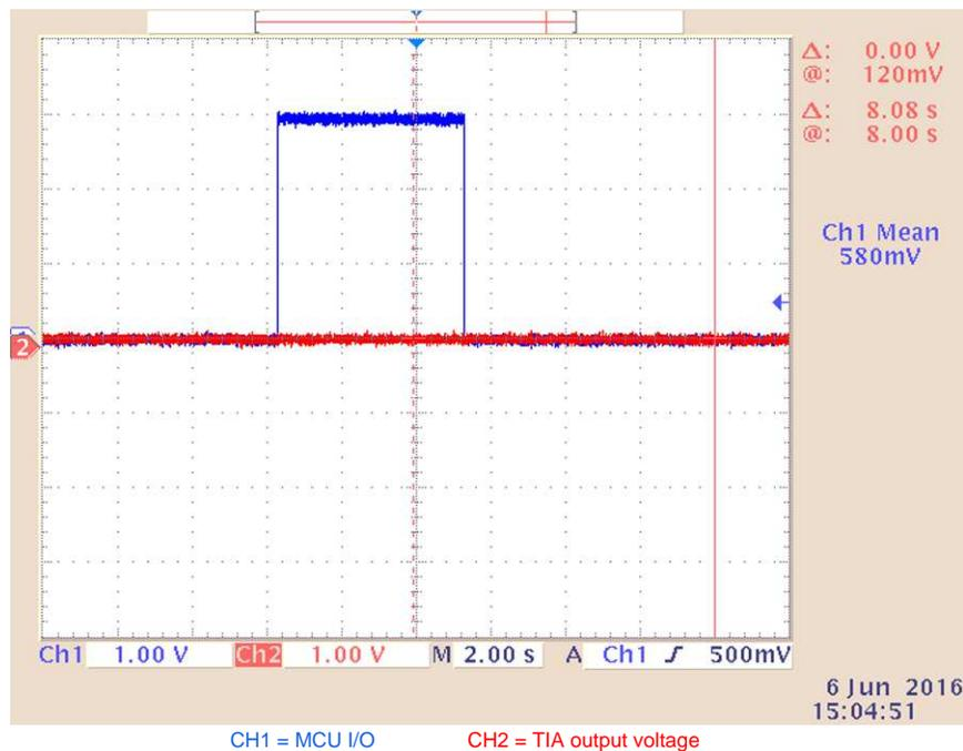
Figure 7. Sensor in Open Circuit
