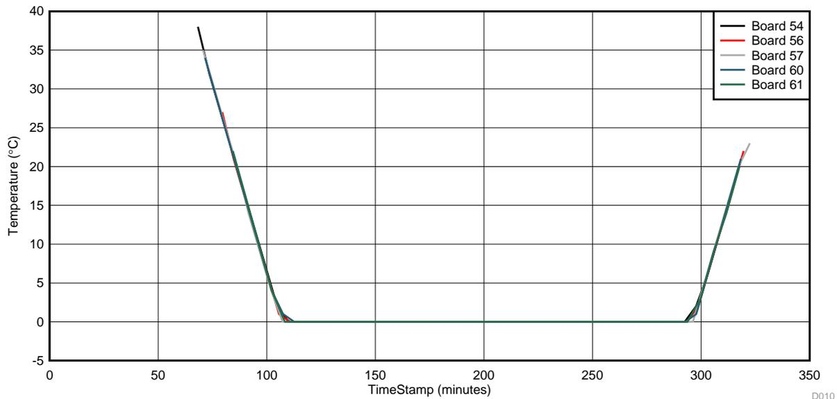
Figure 39. Sensor Temperature Readings During Low Temperature Test
