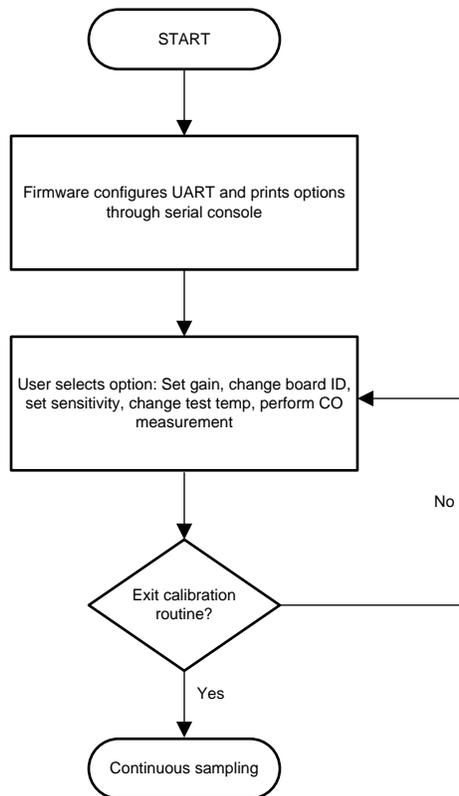
**Figure 15. Calibration Procedure**
