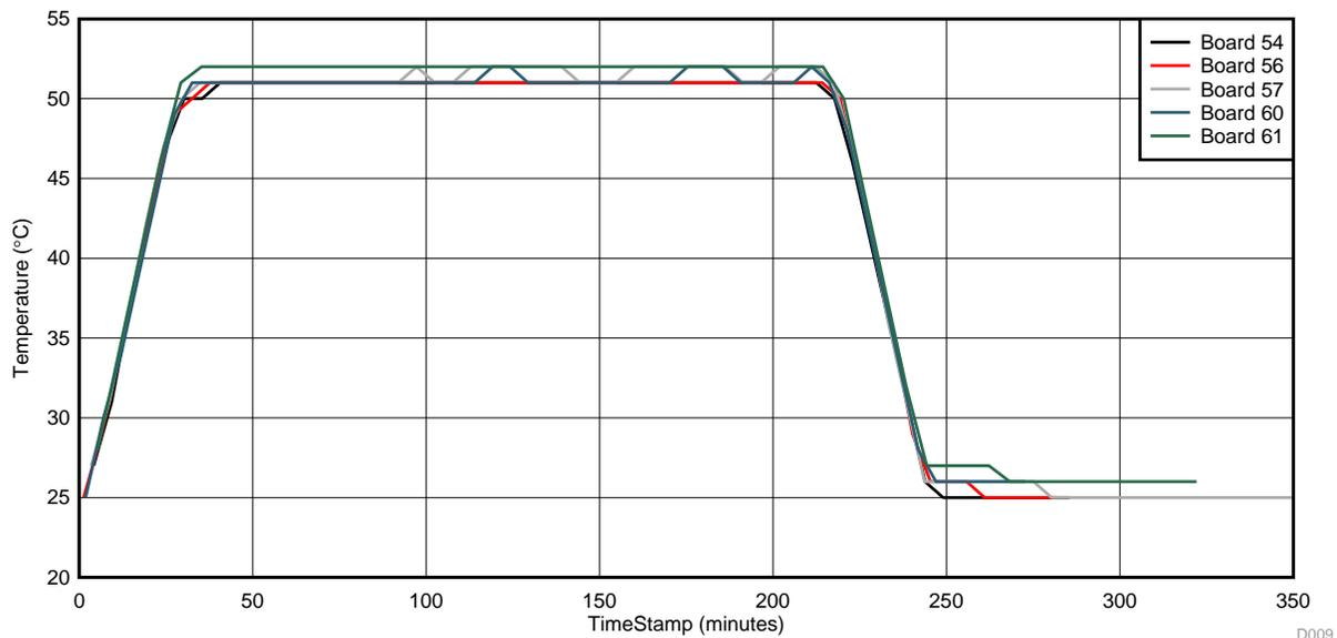
Figure 38. Sensor Temperature Readings During High Temperature Test
