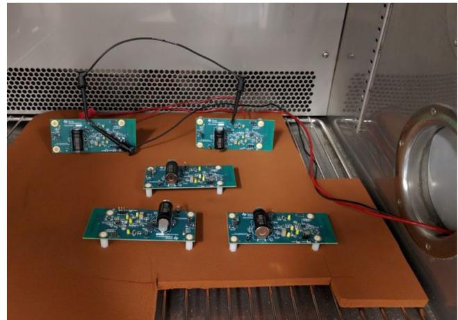
**Figure 27. Reference Design PCBs Inside Environmental Chamber**
