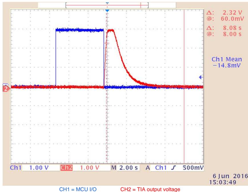
Figure 5. Normal Sensor Response to Test Current
