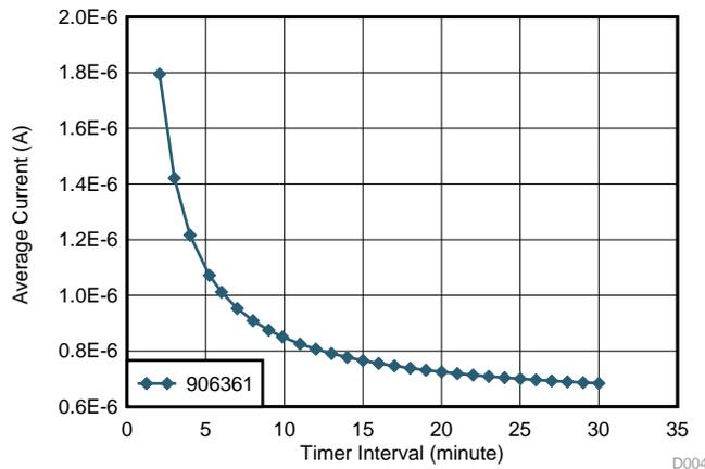
Figure 33. Combined Standby and Test State Average Current versus Timer Interval
