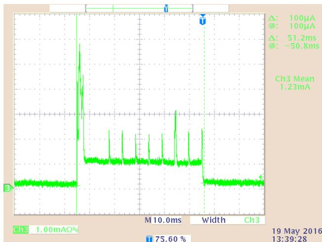
Figure 29. Startup Current at Beginning of Test State
