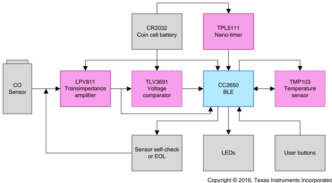
**Figure 1. Wireless CO Sensor System Block Diagram**
