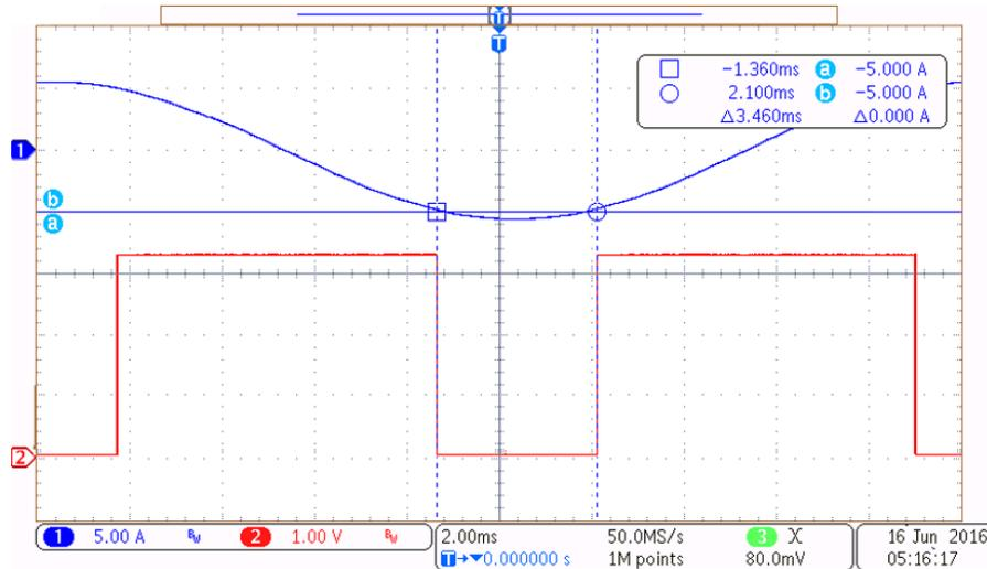
Figure 76. GND\_FAULT Detection During Negative Half Cycle
