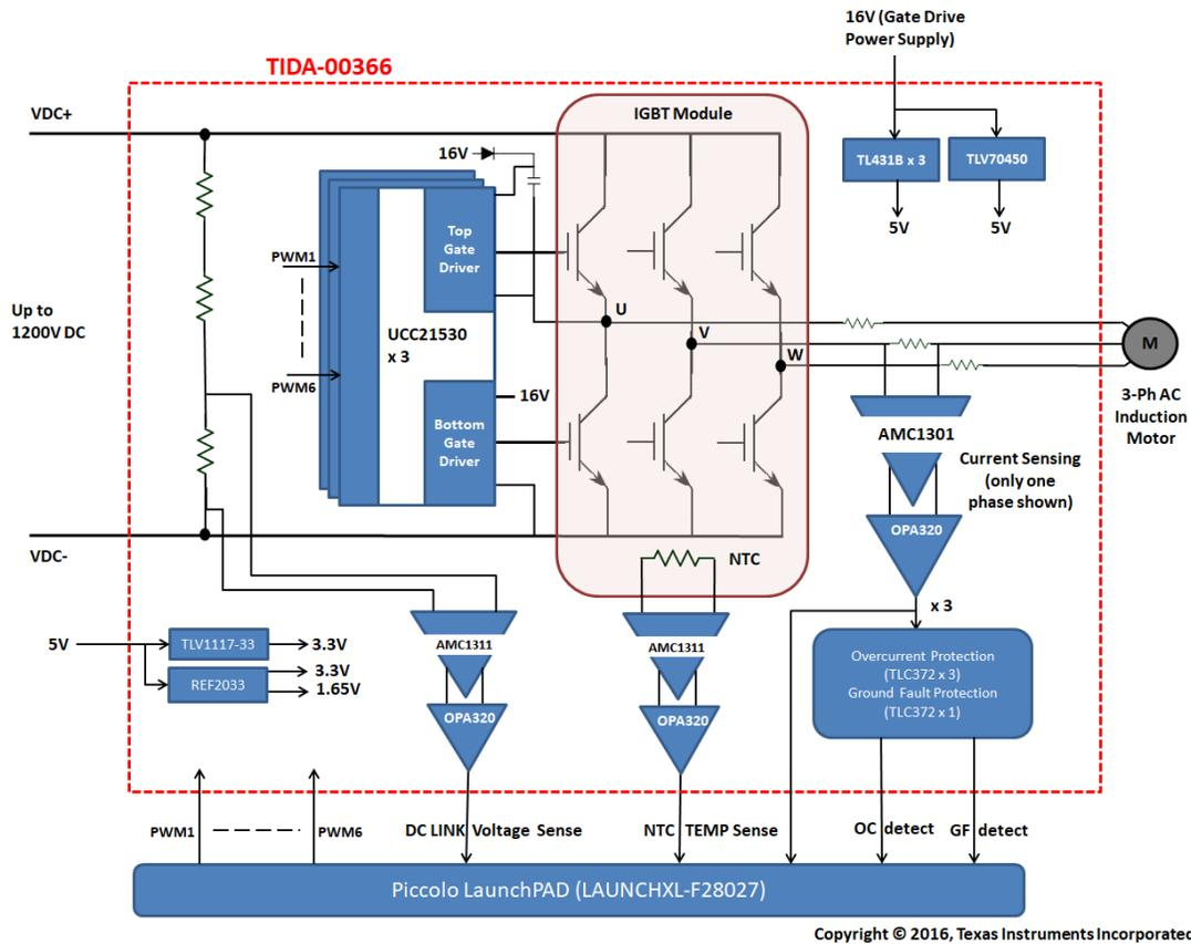
Figure 2. System Level Block Diagram for TIDA-00366
