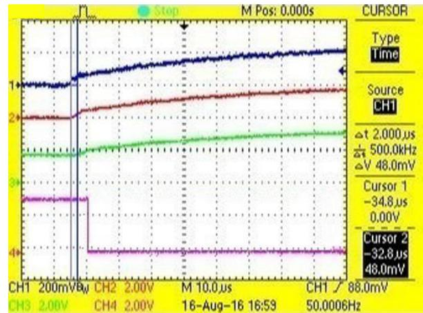
Figure 63. From AMC1301 Input to AMC1301 Output
