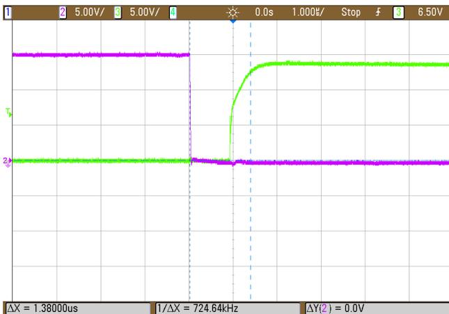
Figure 45. PWM at Gate Driver Output—Dead Time (Rising Edge)
