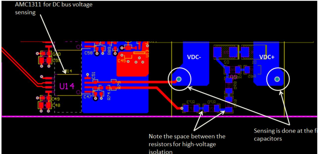
Figure 90. DC Bus Sensing Section
