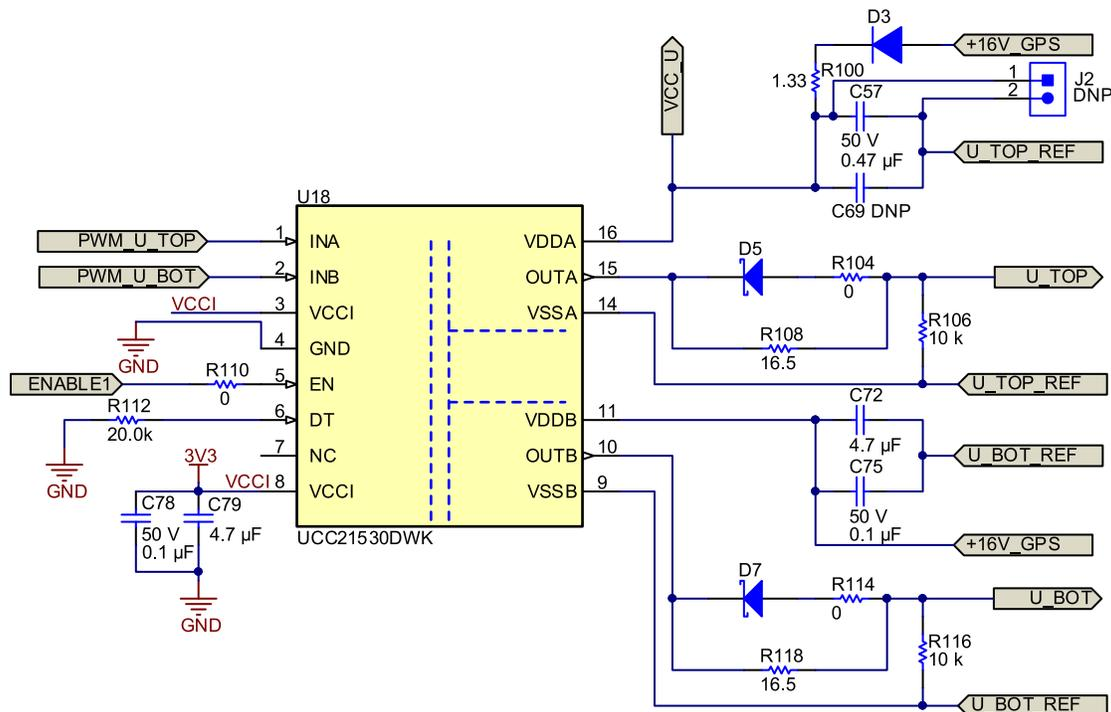
Figure 8. Gate Driver UCC21530 and Related Components and Circuits
