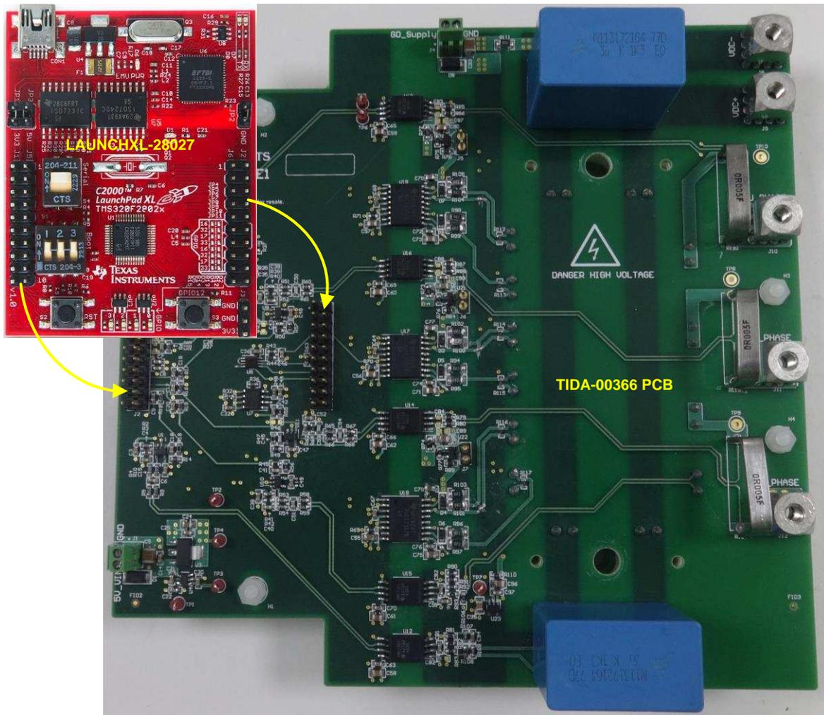
Figure 27. Connecting LAUNCHXL-F28027 Board to TIDA-00366 PCB
