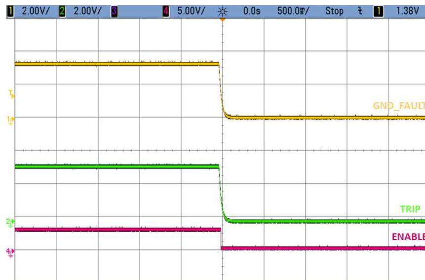
Figure 77. Latching of GND\_FAULT Detect Signal on TRIP Pin
