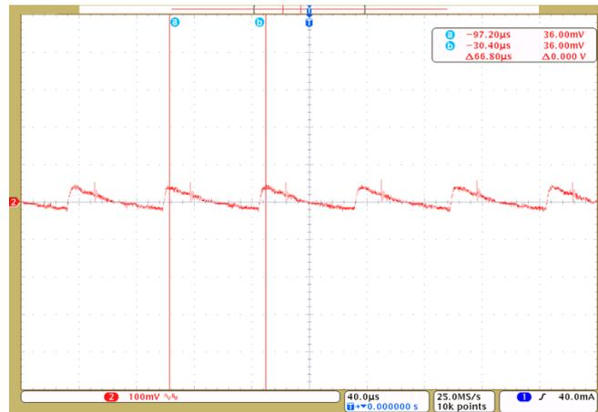
Figure 37. Ripple on 16-V Rail for Low-Side Gate Driver
