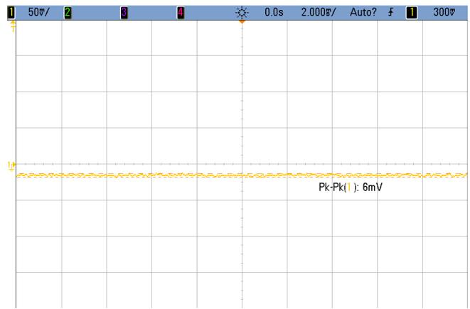
Figure 31. Ripple on 5-V Rail Generated Using TLV70450
