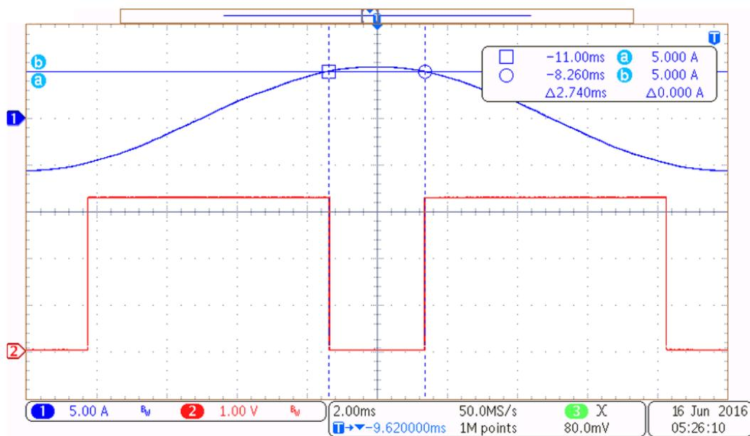
Figure 75. GND\_FAULT Detection During Positive Half Cycle
