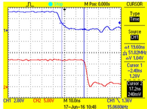
Figure 55. Propagation Delay—High-Side Gate Driver (Falling Edge)
