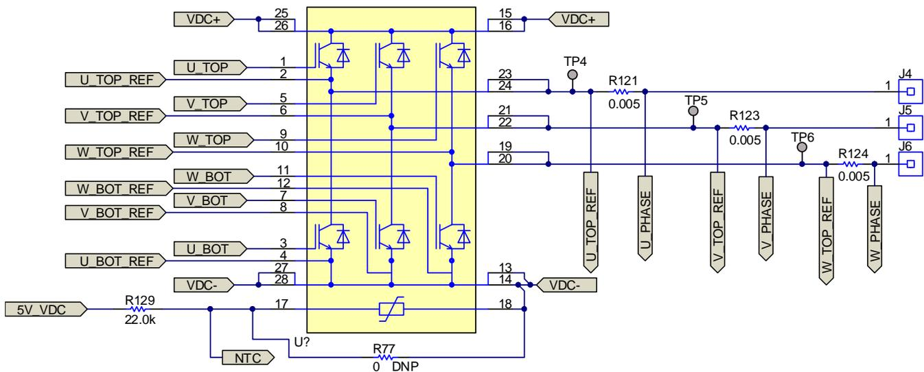
Figure 5. IGBT Module Connections
