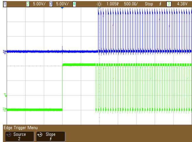
Figure 48. Startup Sequence (PWM at Gate Driver Output)
