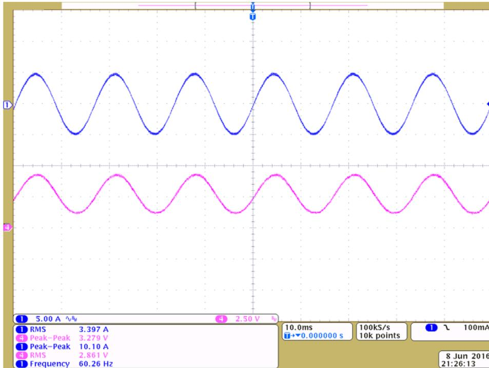
Figure 79. Motor Current Measurement
