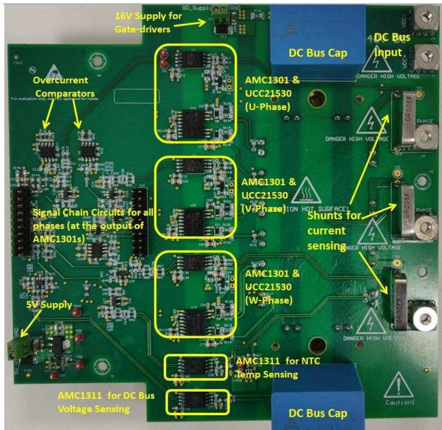
Figure 25. Top View of PCB for TIDA-00366
