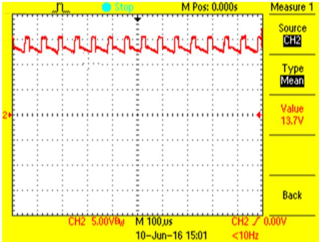
Figure 38. Bootstrap Power Supply for High-Side Gate Driver
