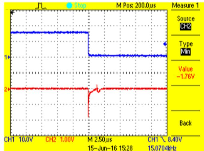
Figure 57. Sink Current to Gate Driver
