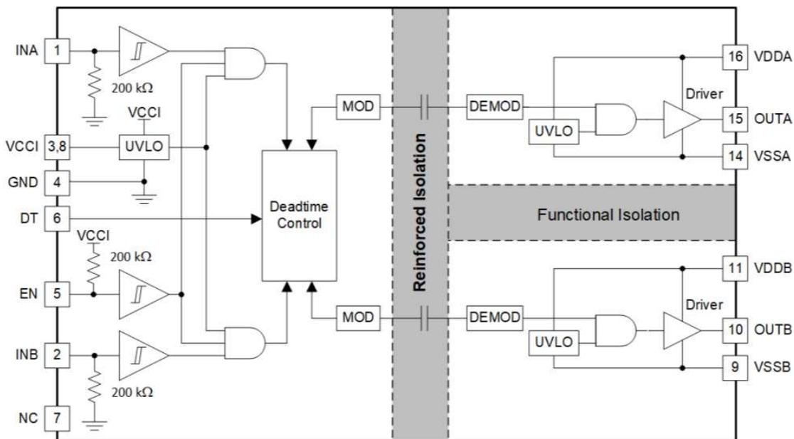
Figure 7. Functional Block Diagram of UCC21530
