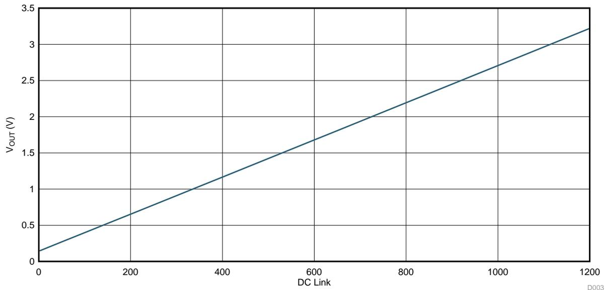
**Figure 70. Transfer Function of DC Bus Voltage Measurement**
