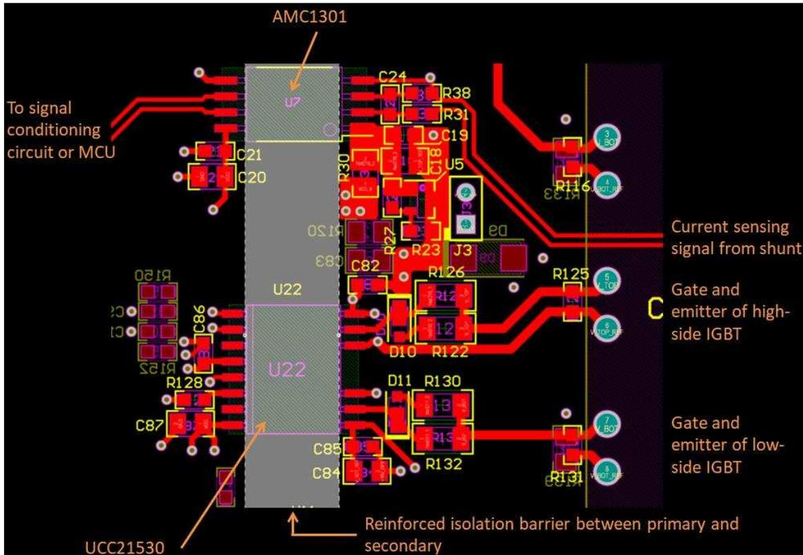
Figure 84. Gate Driver and Current Sensing Circuit
