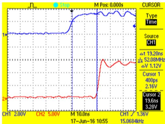
Figure 52. Propagation Delay—Low-Side Gate Driver (Rising Edge)
