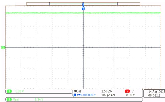
Figure 32. 3.3-V Rail Generated Using REF2033
