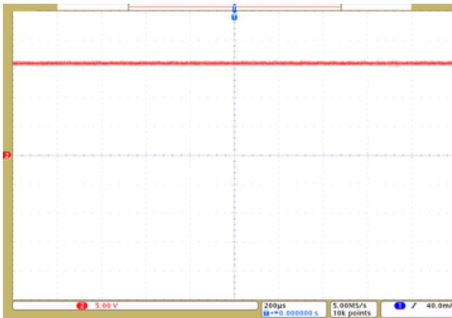
Figure 36. 16-V Rail for Low-Side Gate Driver
