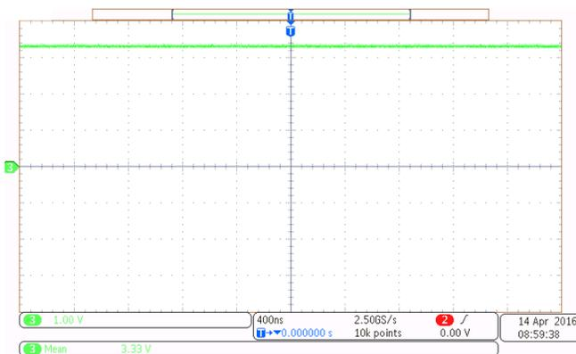
**Figure 28. 3.3-V Rail Generated Using TLV1117-33**
