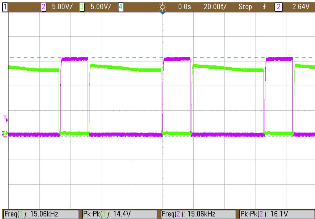
Figure 42. PWM at the Gate Driver Output
