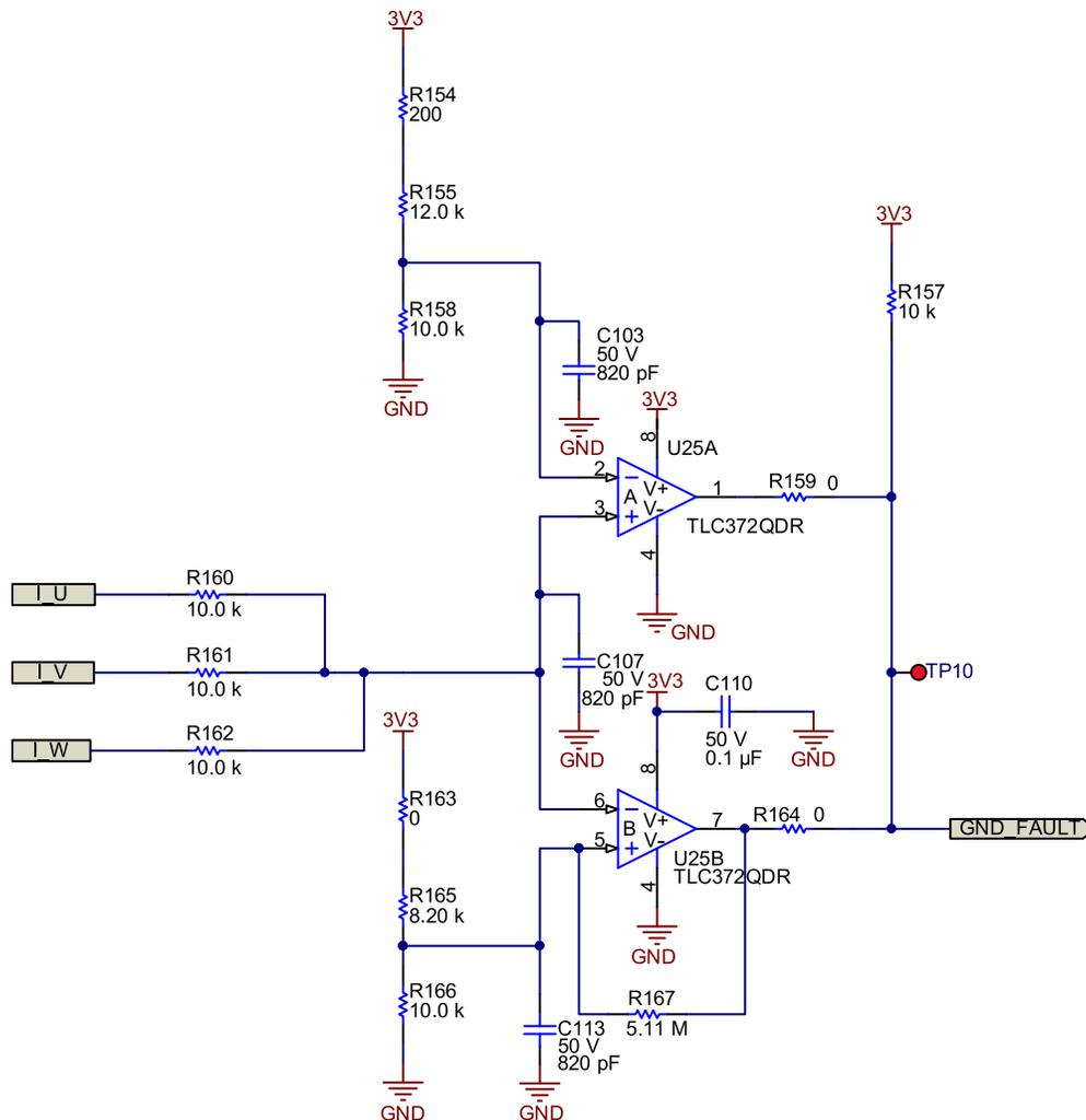
Figure 18. Ground Fault Detection Circuit
