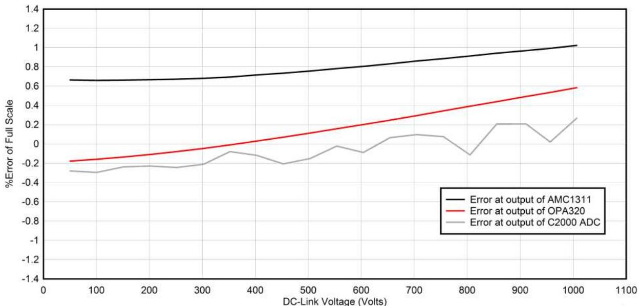
Figure 67. Uncalibrated Percentage Full-Scale Error vs DC-Link Voltage at No Load
