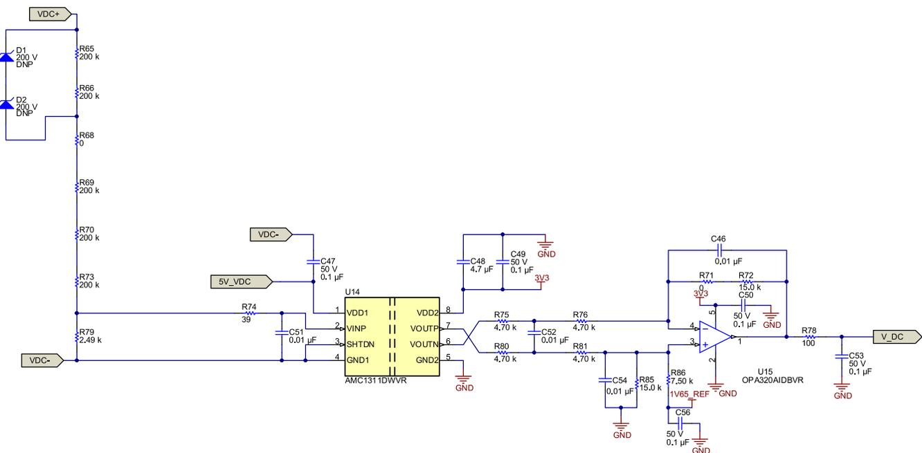
Figure 14. DC Bus Voltage Sensing Circuit
