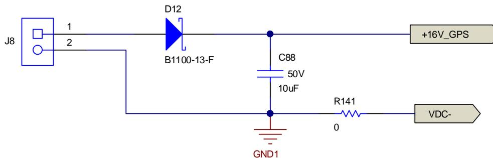
**Figure 9. Gate Driver Power Supply**
