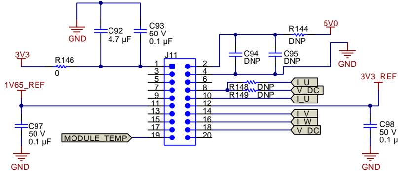
Figure 21. 20-Pin Connector to Connect With Connectors J1 and J5 on LAUNCHXL-F28027
