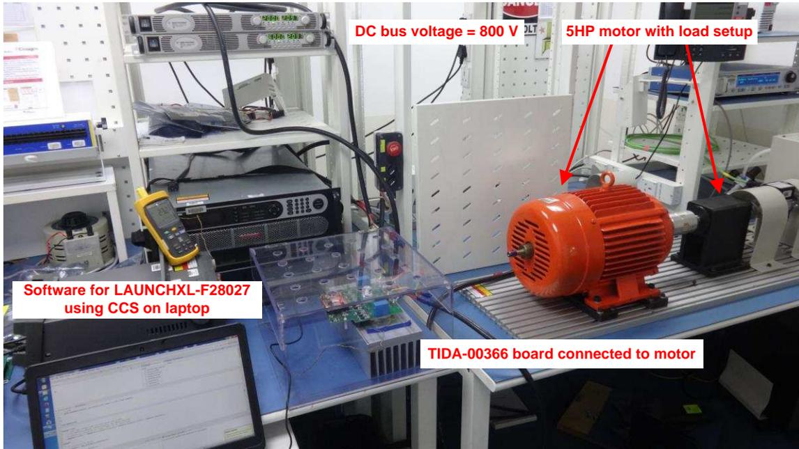
**Figure 78. TIDA-00366 Test Using ACIM and Load Setup**
