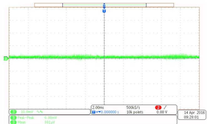
**Figure 29. Ripple on 3.3-V Rail Generated Using TLV1117-33**
