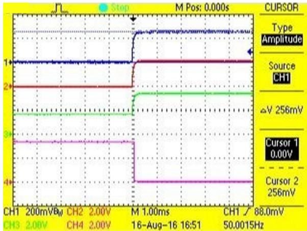
Figure 62. Step Response for Current Measurement Signal Chain
