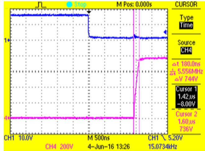
Figure 60. dv/dt During Sinking
