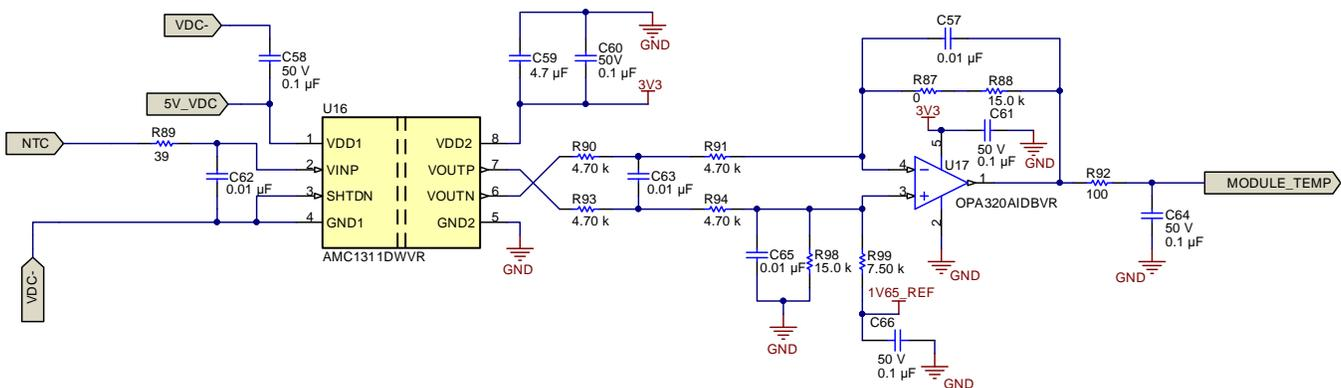
Figure 16. NTC Temperature Sensing Circuit
