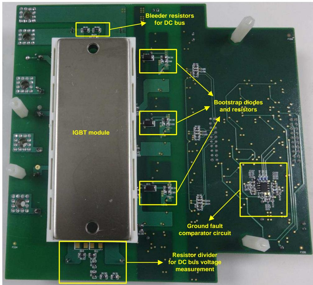
Figure 26. Bottom View of PCB for TIDA-00366
