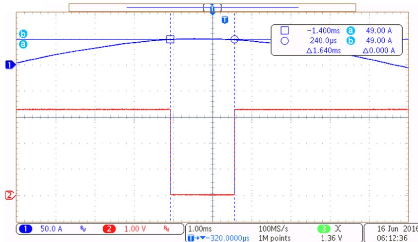
Figure 72. OVERLOAD Detection During Positive Half Cycle
