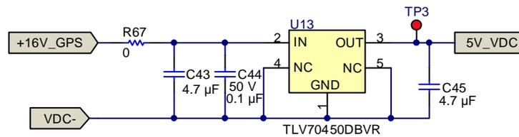
**Figure 23. 5-V Generation From 16-V Gate Drive Power Supply Input**
