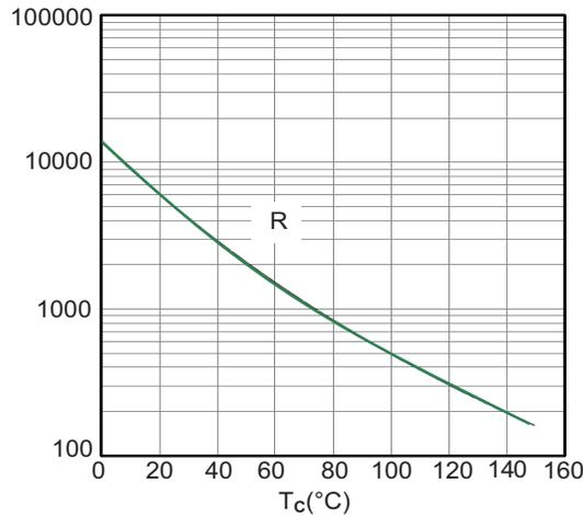
Figure 15. NTC Characteristics
