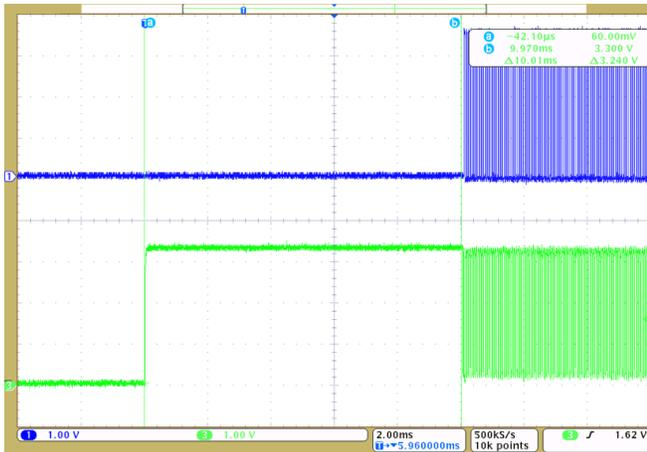
Figure 47. Startup Sequence (PWM From MCU)
