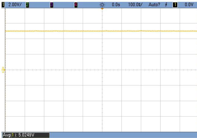
Figure 30. 5-V Rail Generated Using TLV70450
