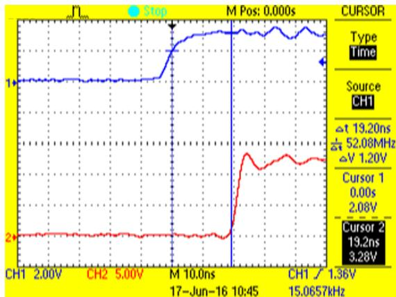
Figure 54. Propagation Delay—High-Side Gate Driver (Rising Edge)
