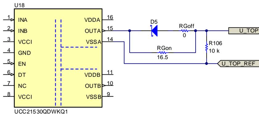
**Figure 10. Gate Resistors**
