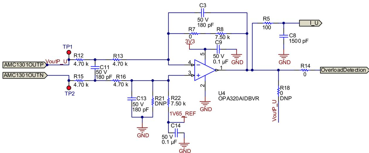
Figure 13. Differential-to-Single Ended Signal Conversion
