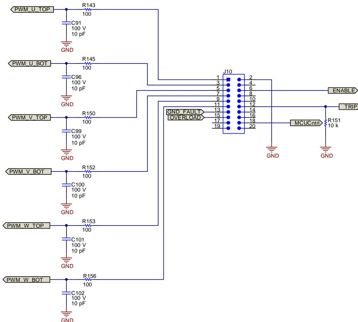
**Figure 20. 20-Pin Connector to Connect With Connectors J6 and J2 on LAUNCHXL-F28027**
