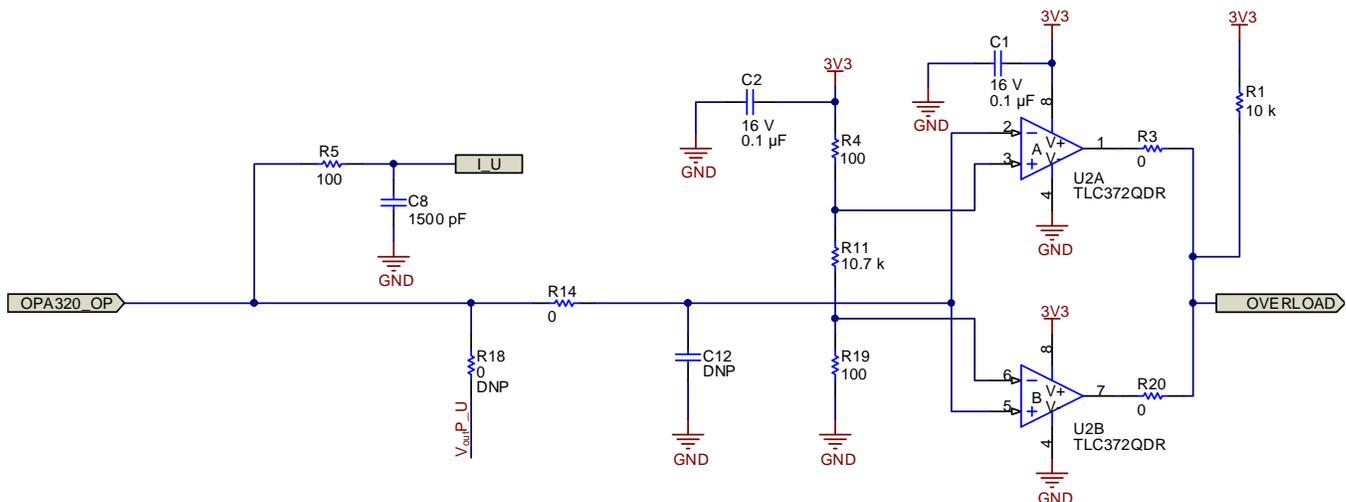
**Figure 17. Overload Protection Circuit**
