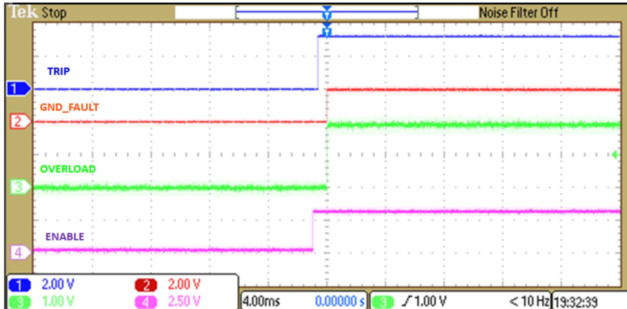
Figure 61. ENABLE Logic for Gate Drivers
