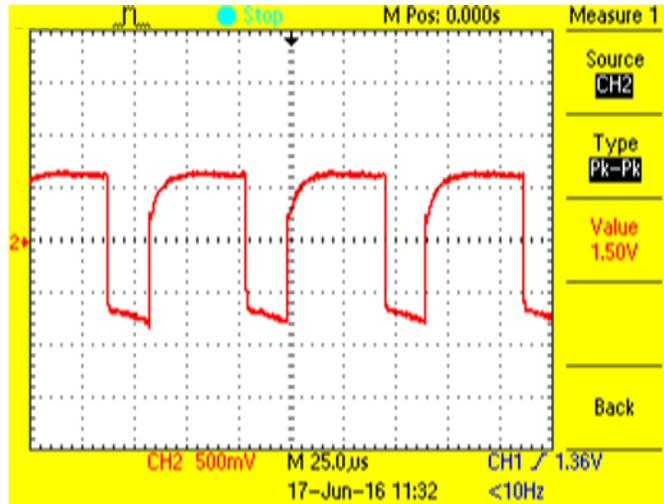
Figure 40. Bootstrap Ripple With 1- $\mu$ F Capacitor for CBST
