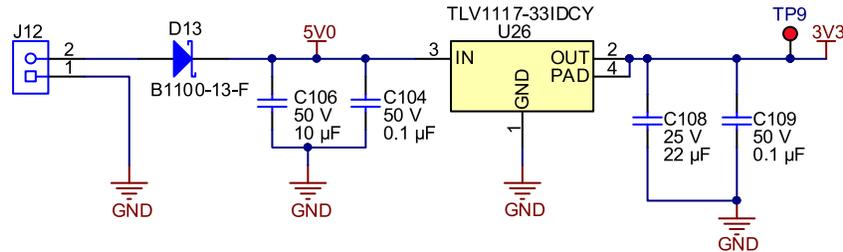
Figure 22. 3.3-V Generation From 5-V Input
