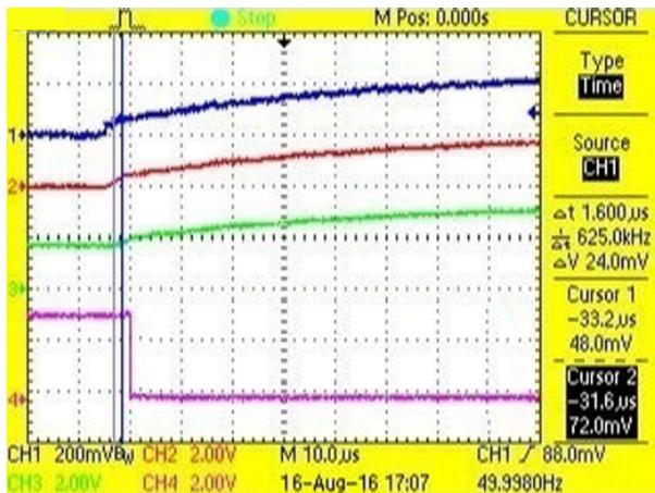
Figure 64. From AMC1301 Output to Op Amp Output
