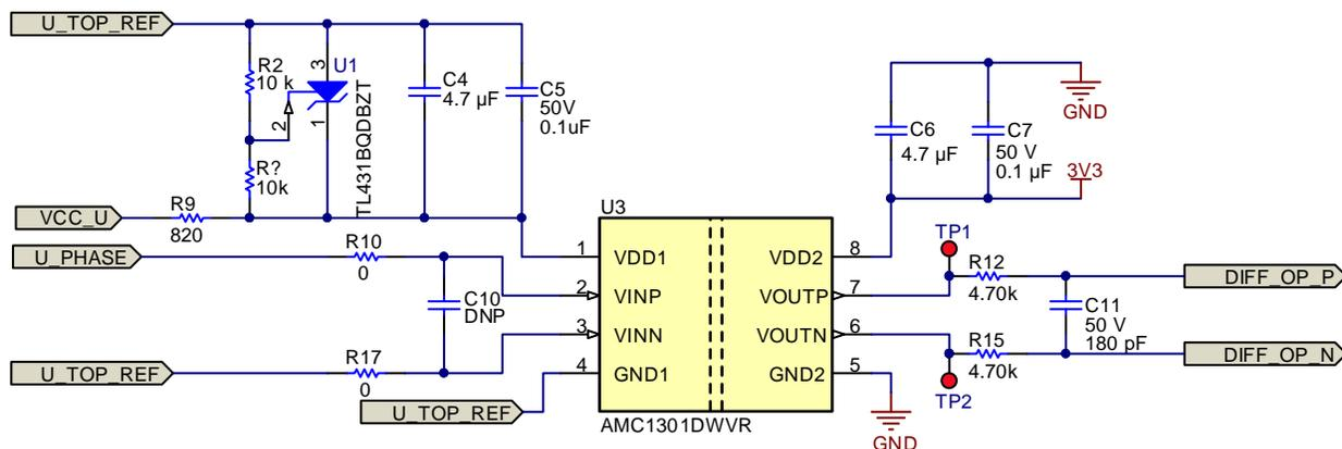
**Figure 11. Reinforced Isolated Amplifier AMC1301**
