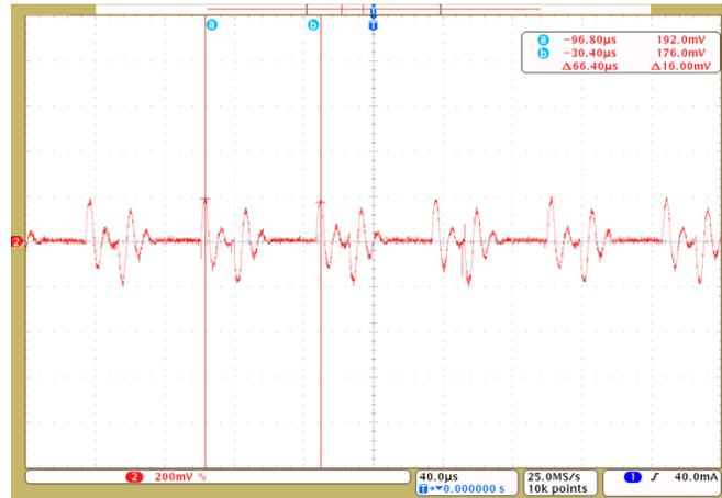
Figure 35. Ripple on 5 V to Power Hot Side of AMC1301
