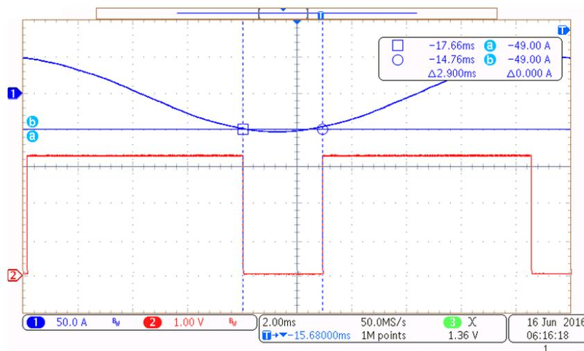
Figure 73. OVERLOAD Detection During Negative Half Cycle
