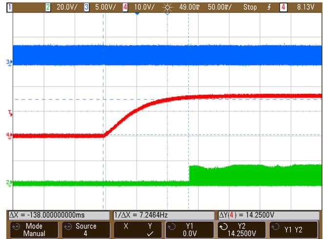
Figure 50. High-Side Gate Driver UVLO
