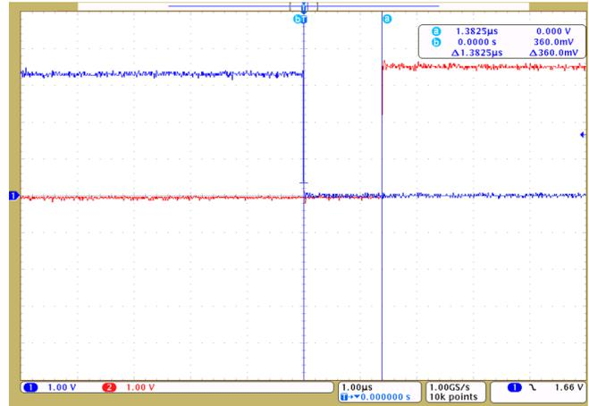
Figure 44. PWM From MCU—Dead Time (Falling Edge)
