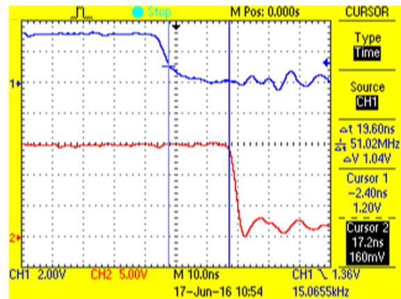
Figure 53. Propagation Delay—Low-Side Gate Driver (Falling Edge)
