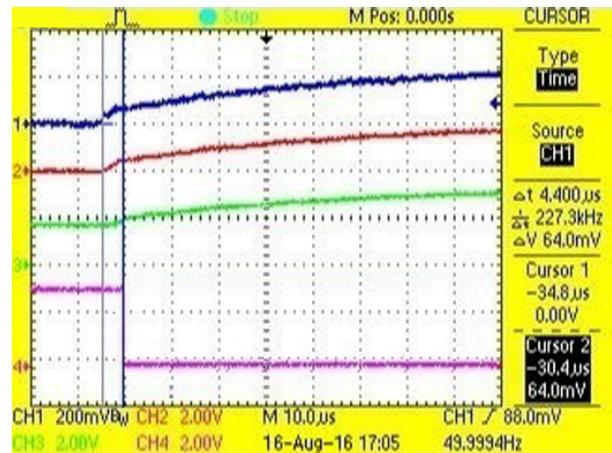
Figure 65. Propagation Delay From AMC1301 Input to Comparator Output
