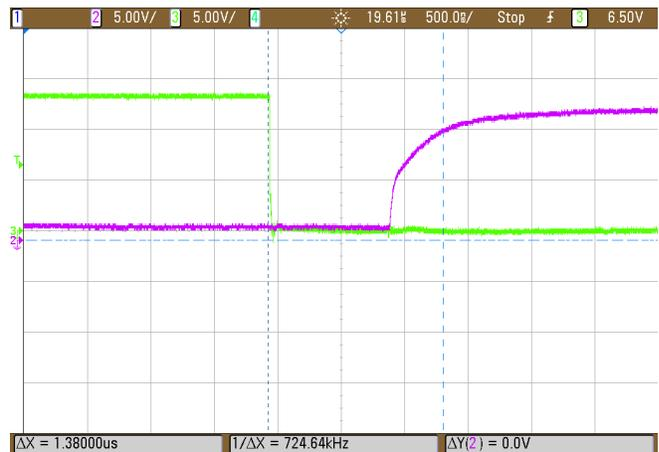
Figure 46. PWM at Gate Driver Output—Dead Time (Rising Edge)
