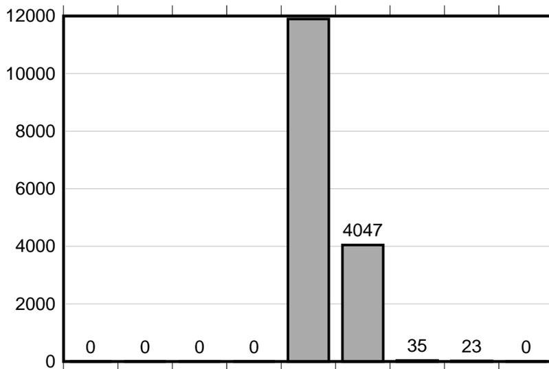
Figure 69. Histogram of DC-Link Sensing Measuring 600 V With 3 A<sub>RMS</sub> in Motor
