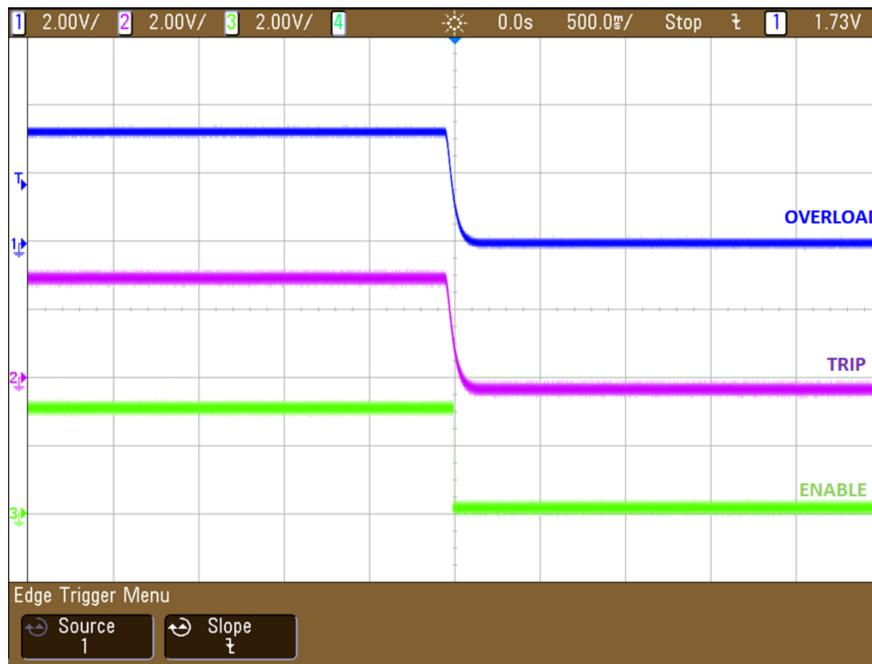
Figure 74. Latching of OVERLOAD Detect Signal on TRIP Pin
