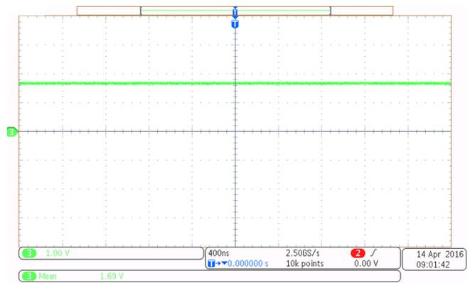
Figure 33. 1.65-V Rail Generated Using REF2033
