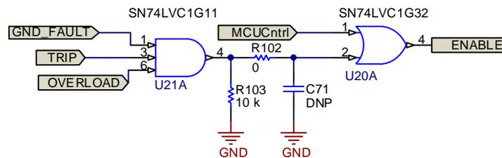
**Figure 19. ENABLE Logic Generation**
