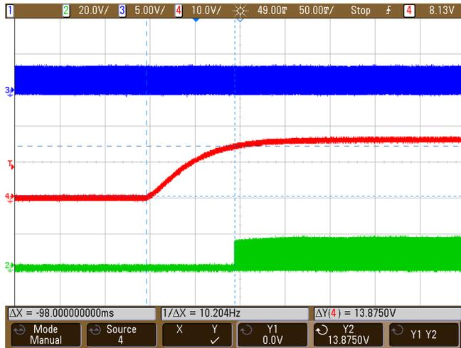
Figure 49. Low-Side Gate Driver UVLO
