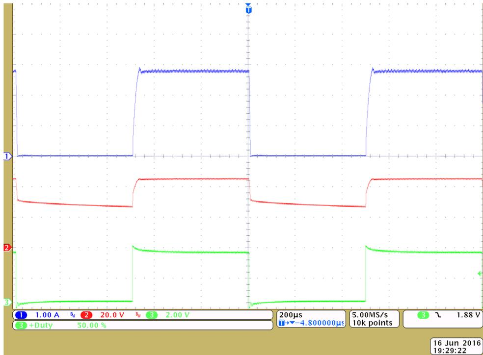
Figure 26. LED Current, LED Voltage, and UDIM Input Waveforms at 50% Duty Cycle
