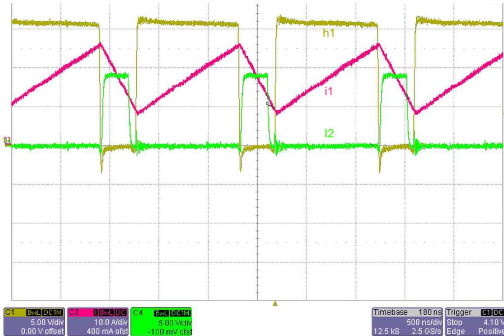
Figure 19. Switching Node Waveform Showing the Switching Node Voltage, Inductor Current, and the Low-Side MOSFET Gate Voltage
