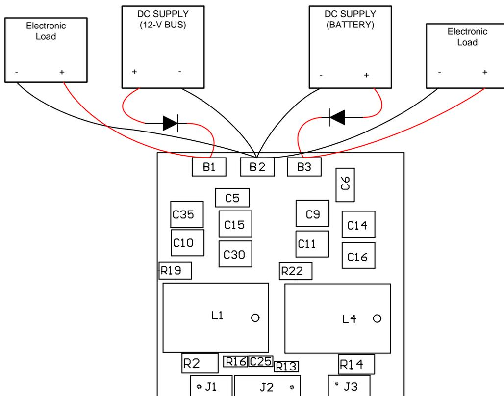
Figure 11. Recommended Test Setup for Testing TIDA-00705
