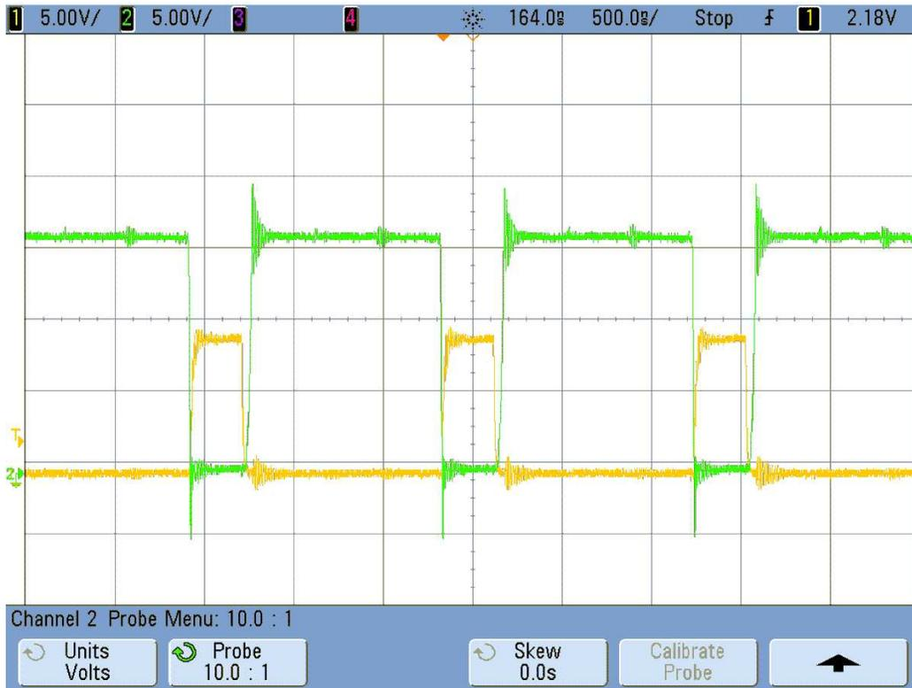
Figure 21. Switching Node Waveform Showing the Voltage Spikes at High-Side MOSFET Turn and Turn Off
