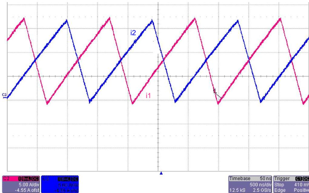
Figure 23. Two Phase Inductor Ripple Current
