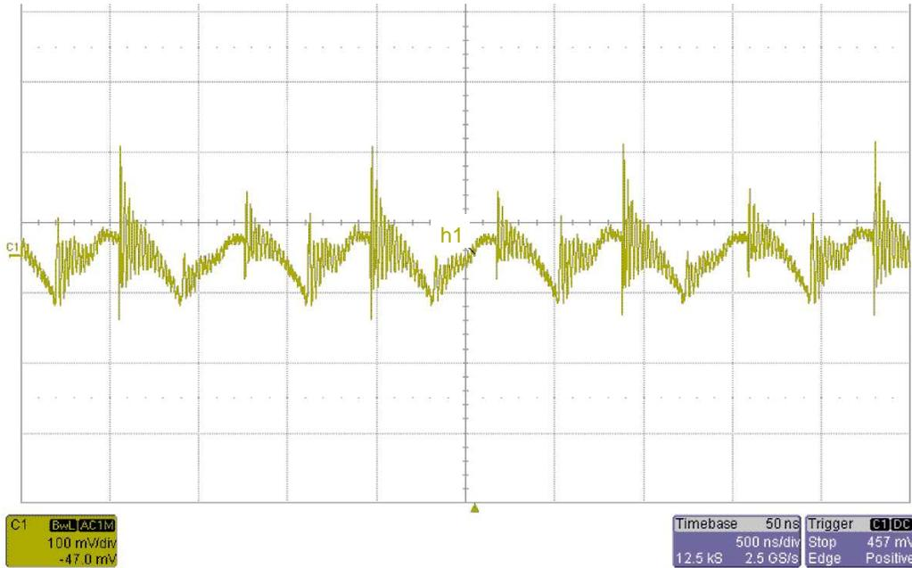
Figure 24. Input Voltage Ripple at the Battery Terminal
