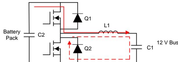
**Figure 3. Power Flow While Working as Synchronous Buck Power Stage**
