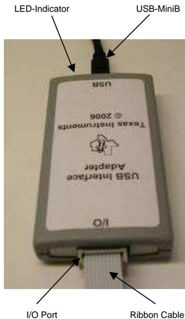
**Figure 6. USB Interface Adapter for Programming UCD3138**
