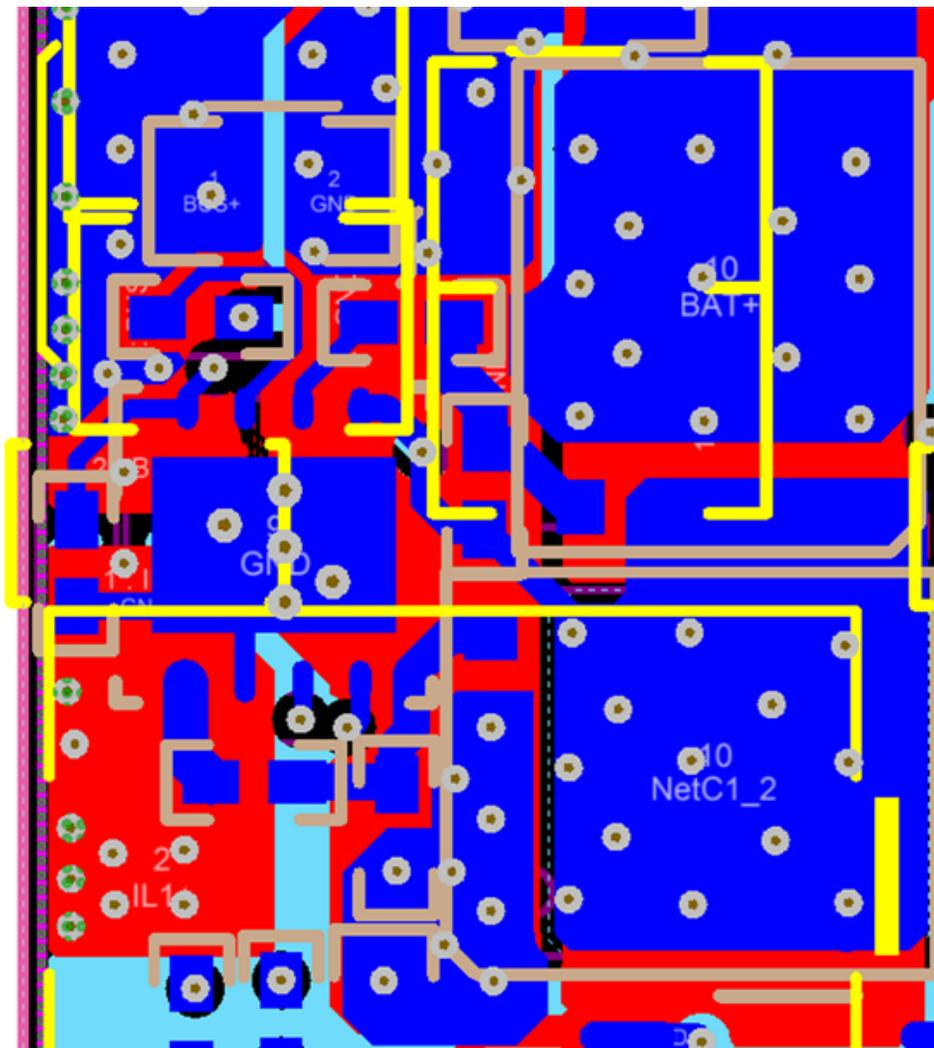
**Figure 31. Switching Node Trace Connection Between Main FET and Synchronous FET**
