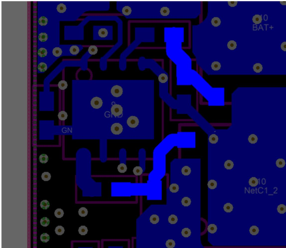
**Figure 32. Connection Between MOSFET Gate and Gate Driver Highlighted**
