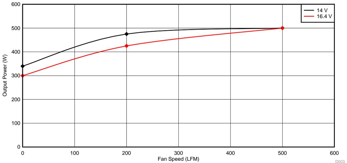
Figure 14. Short Time Output Power Capability Versus Air Flow at Various Input Voltage
