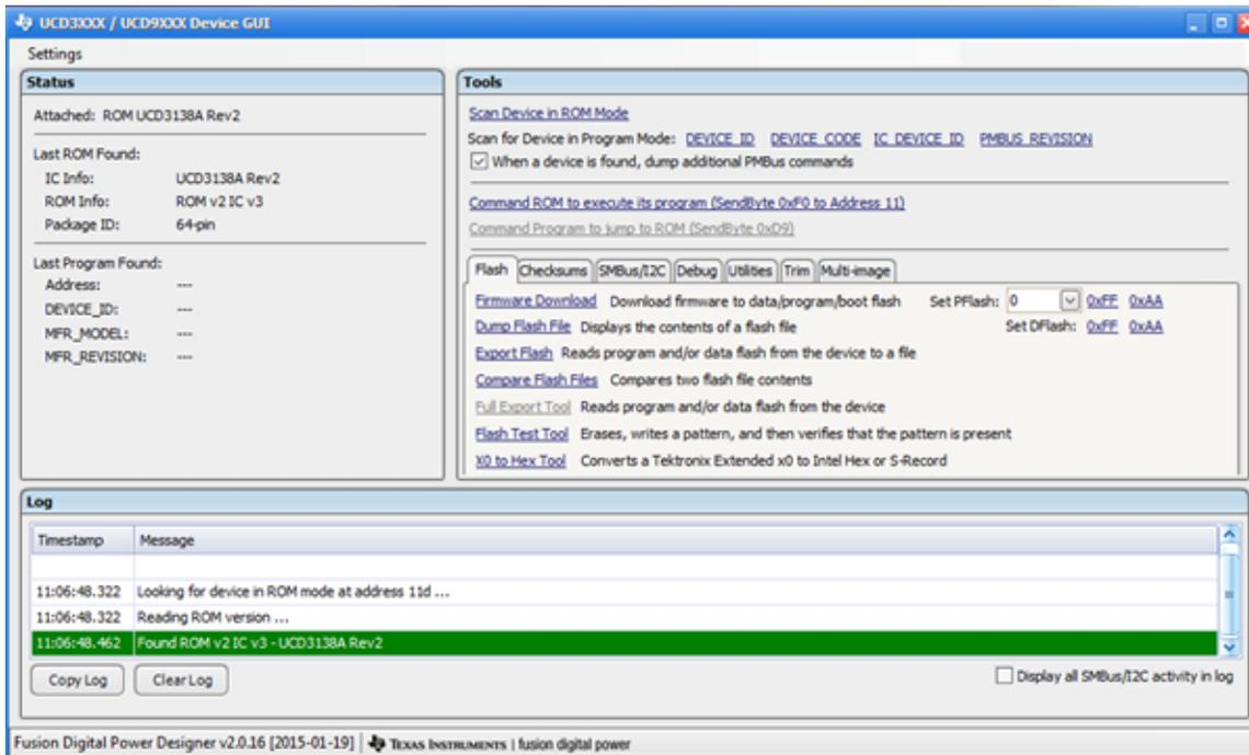
**Figure 9. GUI Screenshot Indicating UCD3138 is Detected Successfully in ROM Mode**
