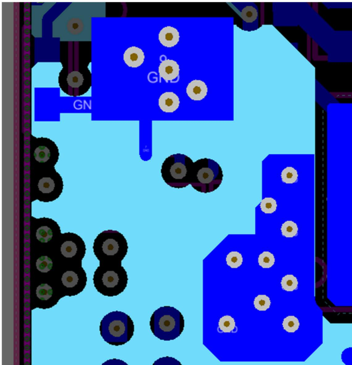
**Figure 33. Connection Between The Gate Driver Ground and Synchronous MOSFET Source**
