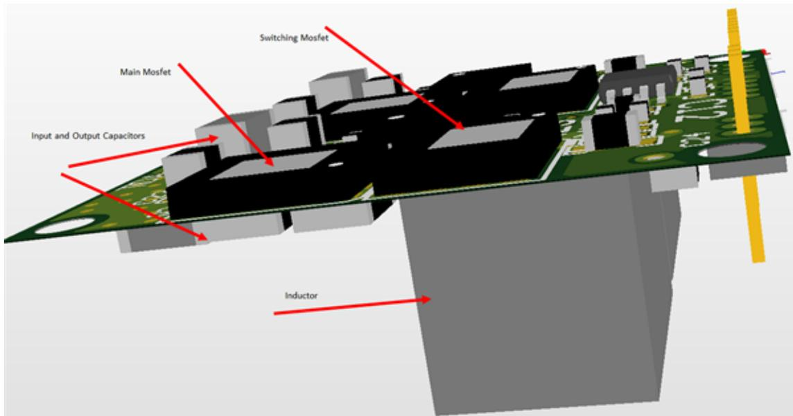
**Figure 30. 3D Image Showing Placement of Components on TIDA-00705 Power Board**
