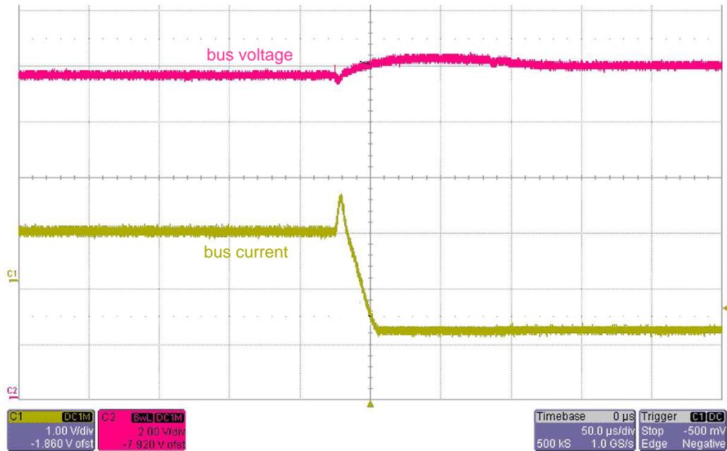
**Figure 26. Mode Change From Battery Charging to Backup Supply**
