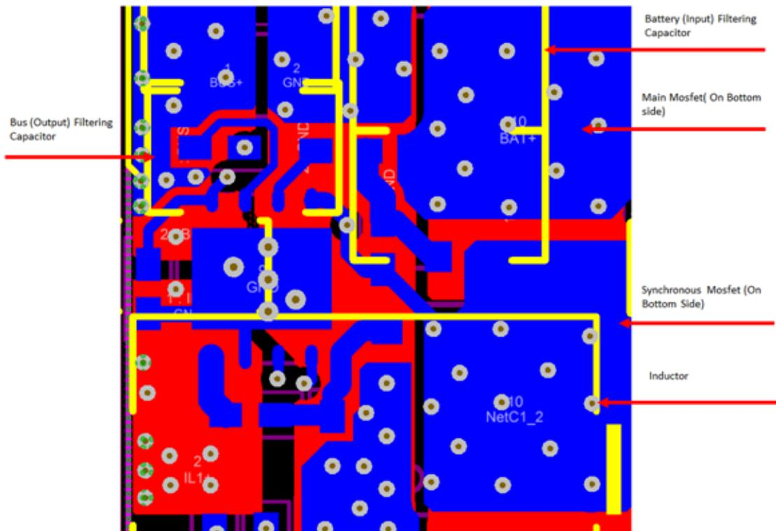
**Figure 29. Half-Bridge Switching Loop Layout Highlighting Major Components**
