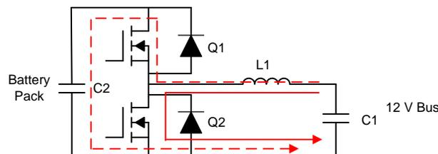
**Figure 4. Power Flow While Working as Synchronous Boost Power Stage**
