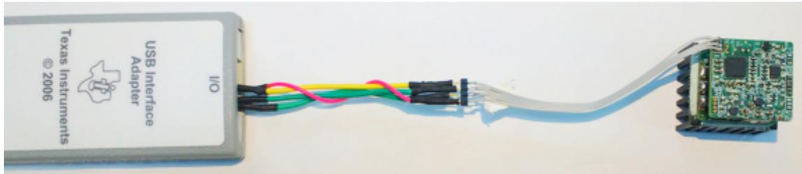
Figure 8. TIDA-00705 Setup for Programming UCD3138
