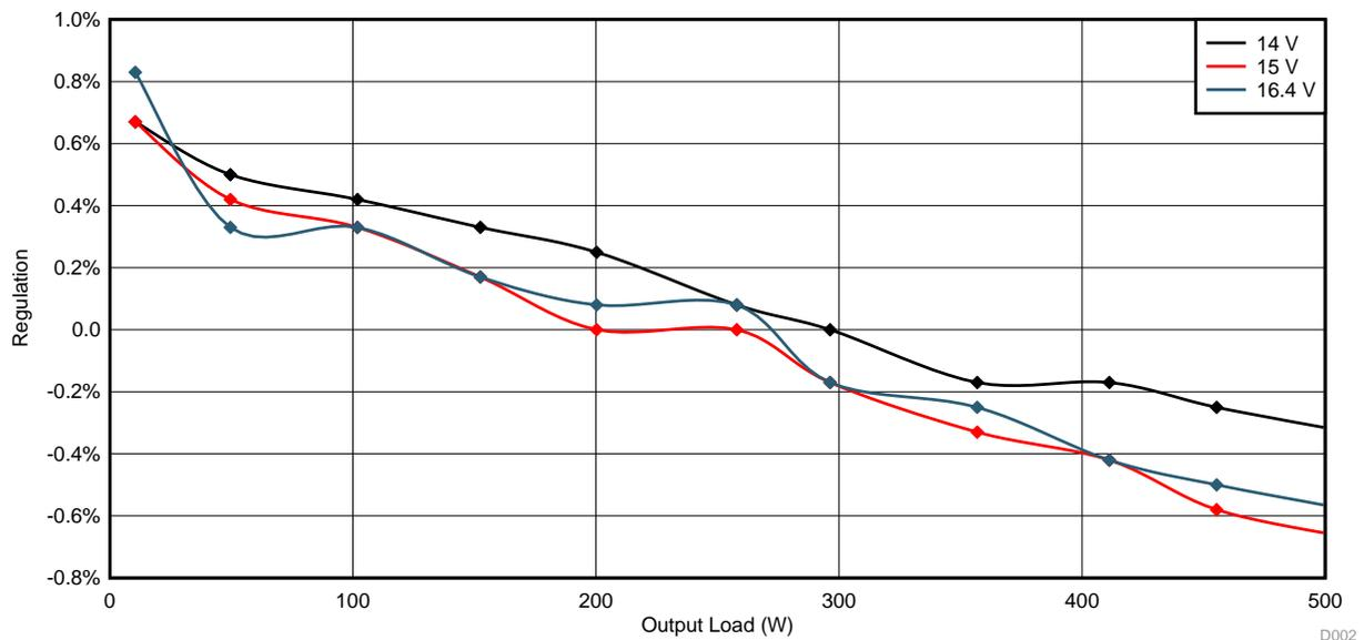
Figure 13. Output Voltage Regulation Versus Output Load Curves in Backup Supply Mode at Various Input Voltage
