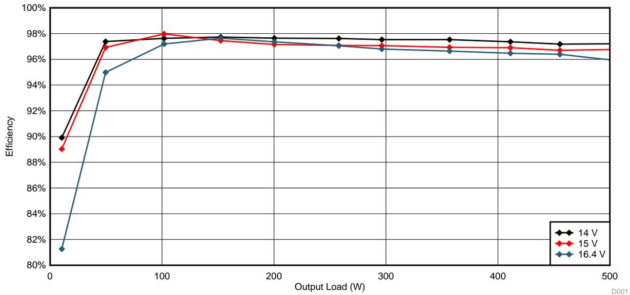
Figure 12. Efficiency Versus Output Load Curves in Backup Supply Mode at Various Input Voltage
