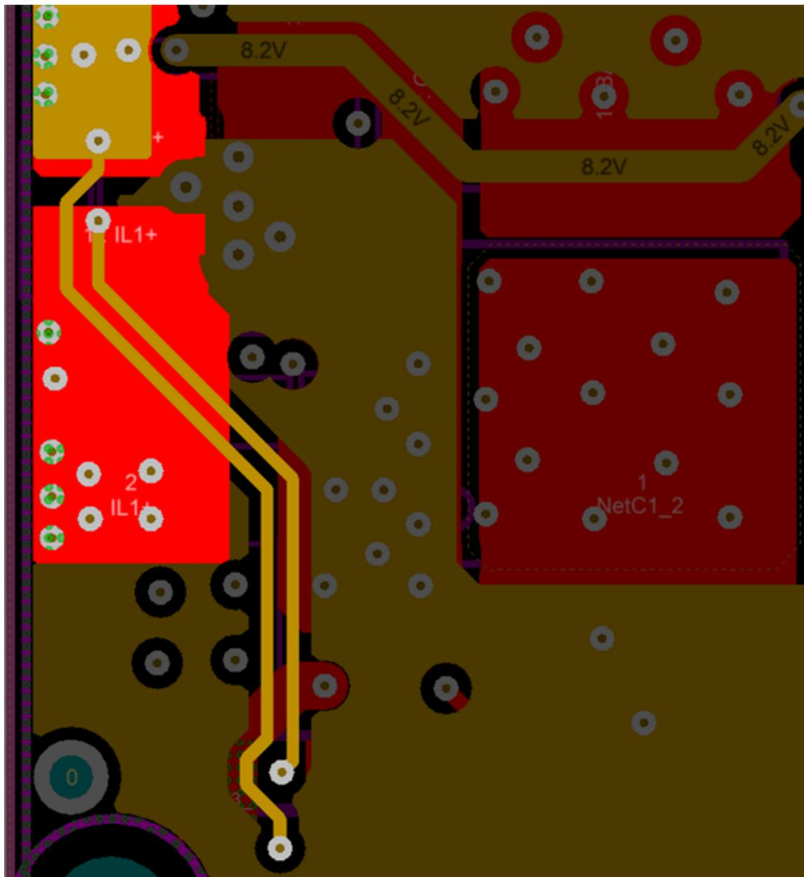
**Figure 34. Current Sense Trace From Current Sense Resistor Highlighted**
