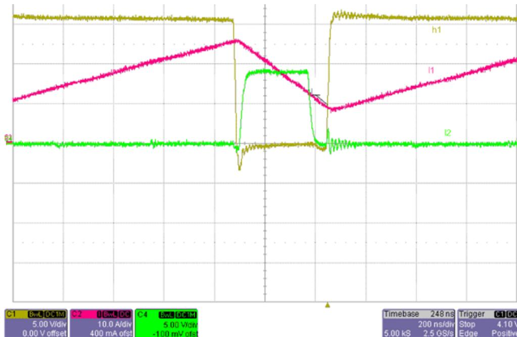
Figure 20. Switching Node Waveform Showing the Switching Node Voltage, Inductor Current, and the Low-Side MOSFET Gate Voltage (Zoomed in)
