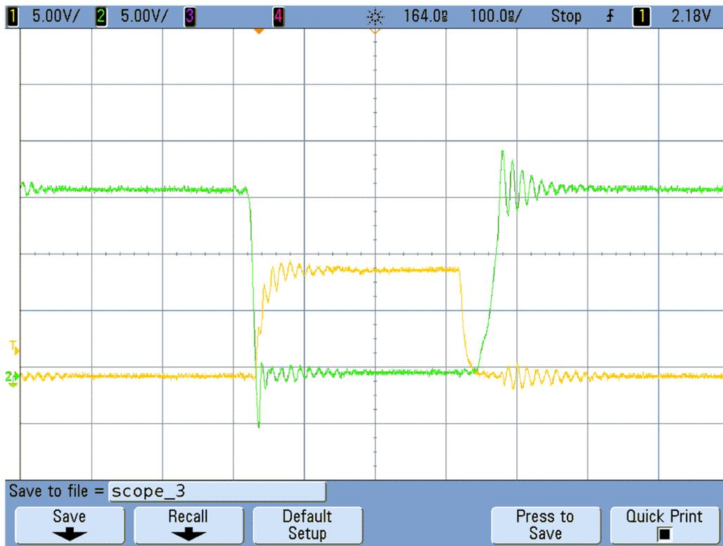
Figure 22. Switching Node Waveform Showing the Voltage Spikes at High-Side MOSFET Turn and Turn Off (Zoomed in)
