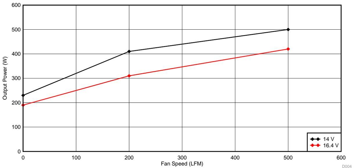
Figure 15. Continuous Output Power Capability Versus Air Flow at Various Input Voltage
