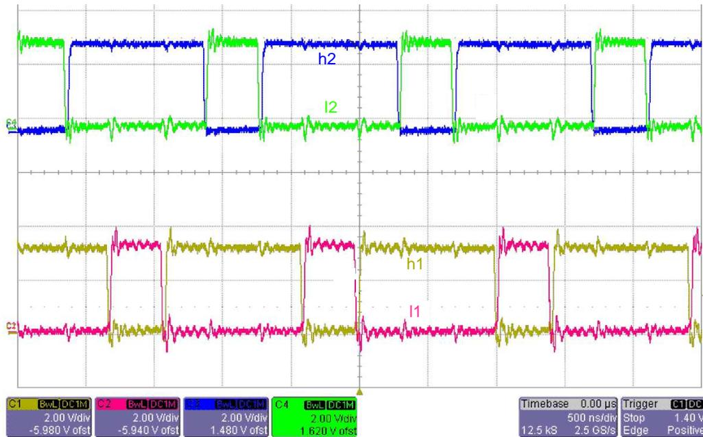
Figure 17. Complimentary PWM Outputs From UCD3138
