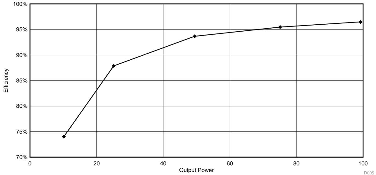
Figure 16. Efficiency Versus Output Power in Battery Charging Mode at 12-V Bus and 16.4-V Battery
