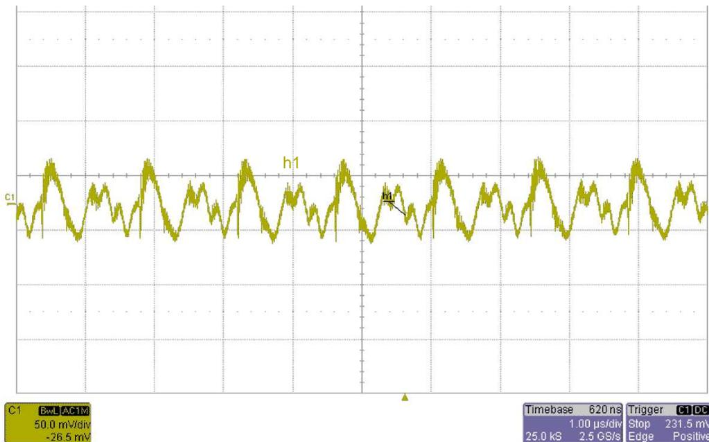
Figure 25. Output Voltage Ripple Measured at the Bus Terminal
