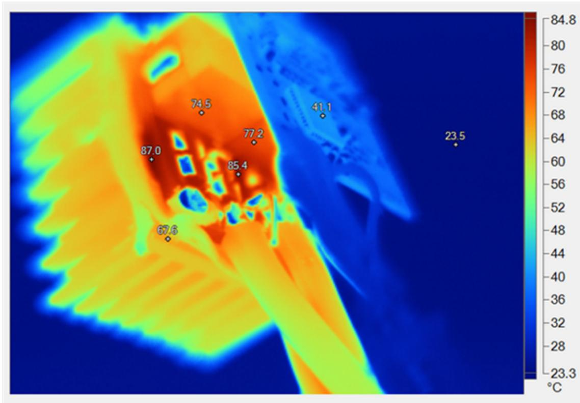
**Figure 27. Thermal Image Captured After Two Minutes When Delivering 425 W at 16.4-V Battery**
