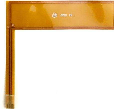
**Figure 44. NFC Flex PCB Antenna**
