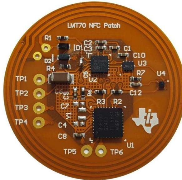
**Figure 6. NFC Temperature Patch Reference Design**
