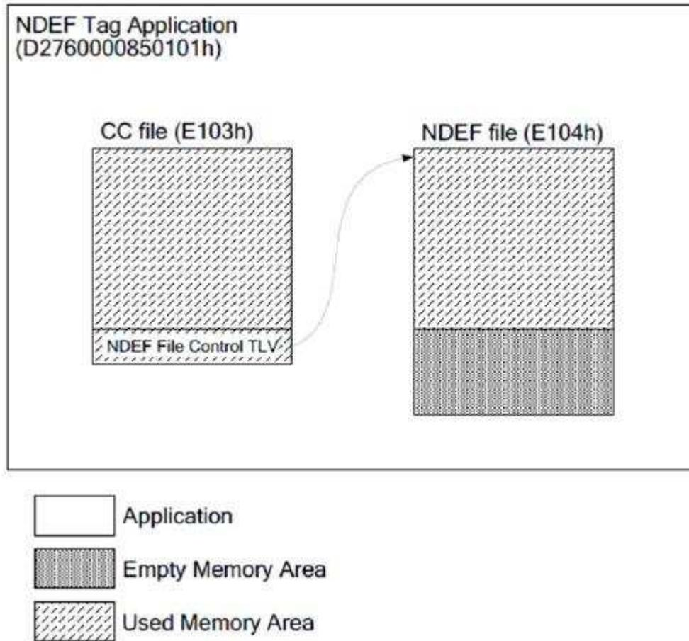
**Figure 10. NDEF Tag Application Mapping Example**
