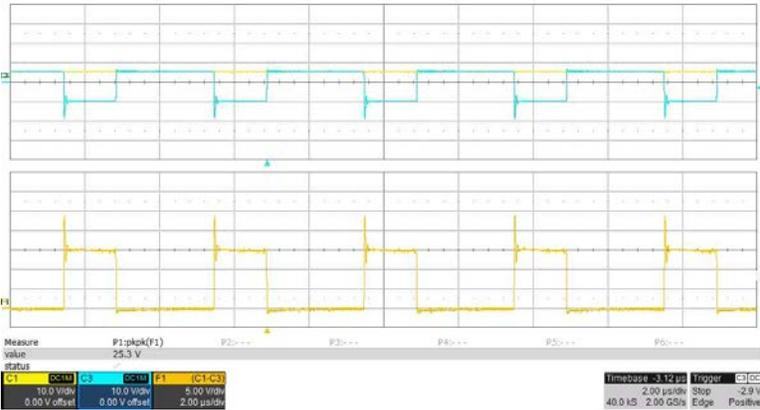
Q5 drain to source with 57V input, 1A load, and 200MHz BWL
