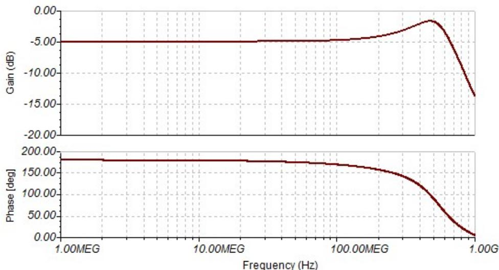
Figure 7. Transfer Function for Single-Ended to Differential Amplifier
