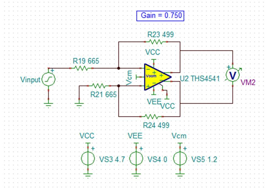
**Figure 20. Simulation Circuit for THS4541 With Updated Gain of 0.750 V/V**
