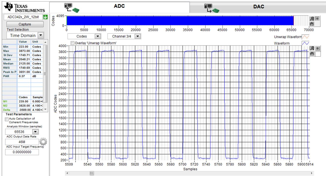
Figure 18. 1-MHz, ±1-V Square Wave Input
