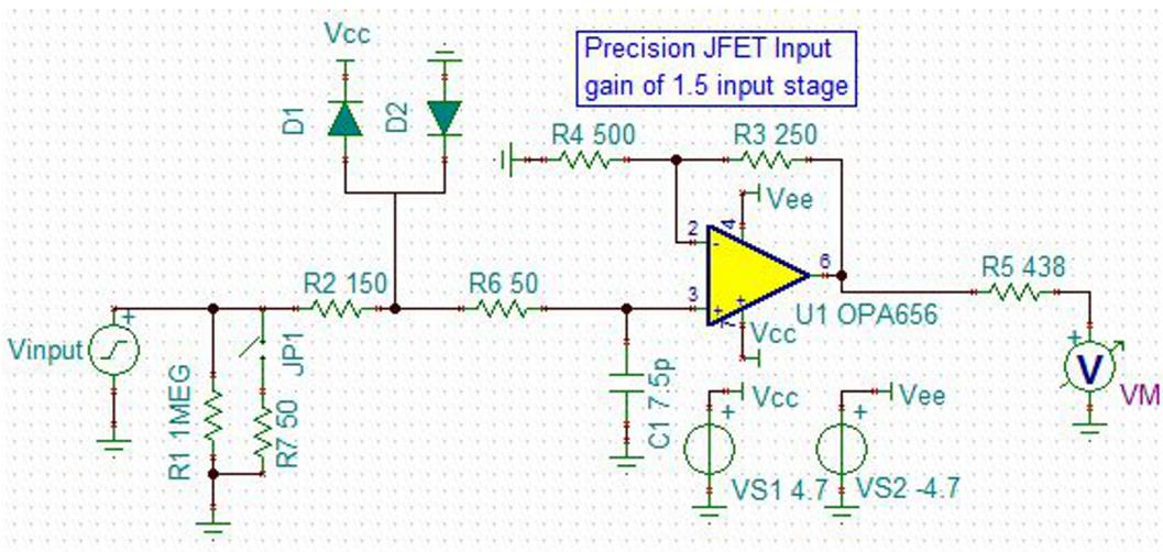
Figure 3. Simulation Circuit for OPA656
