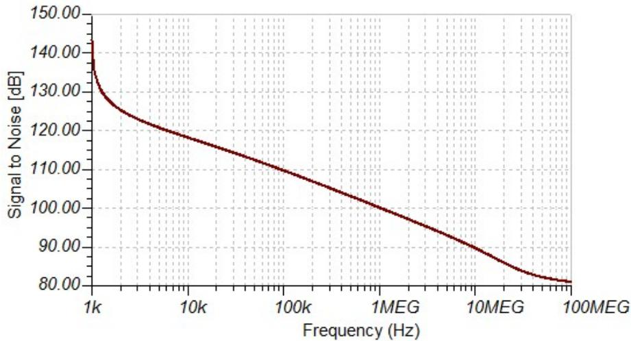
Figure 15. SNR for Complete OPA656 (JFET), Differential Amplifier (THS4541) With RLC Low-Pass Filter
