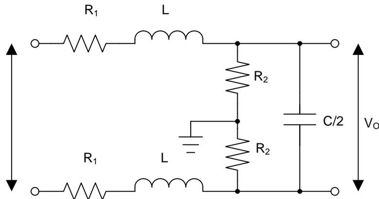
**Figure 10. Simplified Differential Low-Pass Filter**
