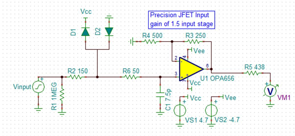
**Figure 19. Simulation Circuit for OPA656 With Updated Gain of 1.5 V/V**
