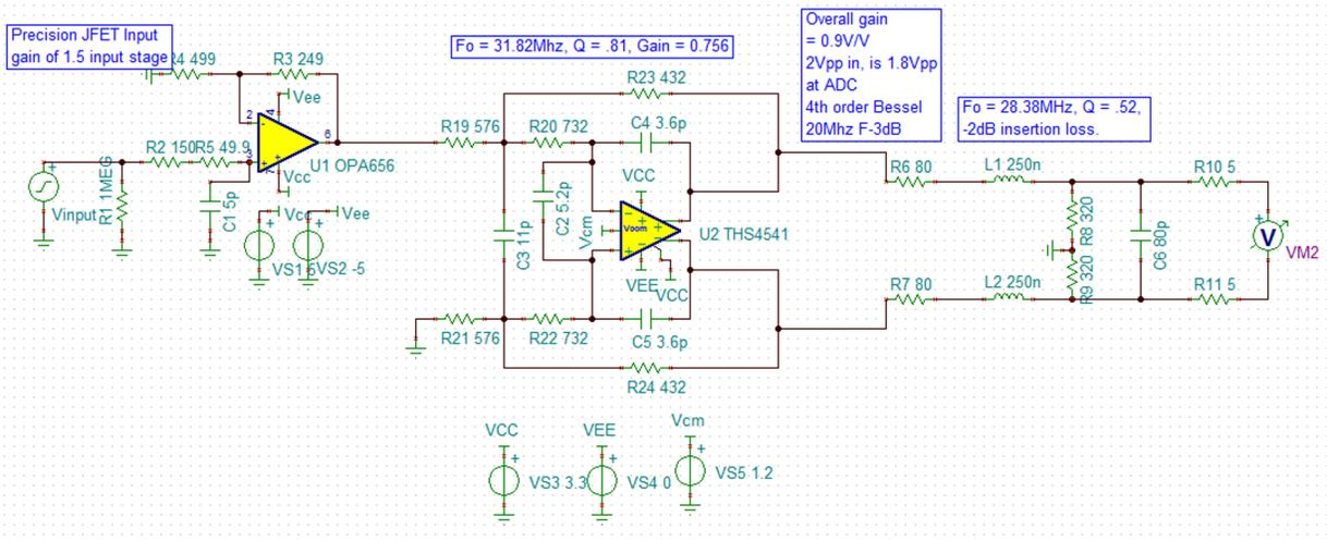
**Figure 22. Channel 3 With Active, Second-Order, MFB Low-Pass Filter Stage**
