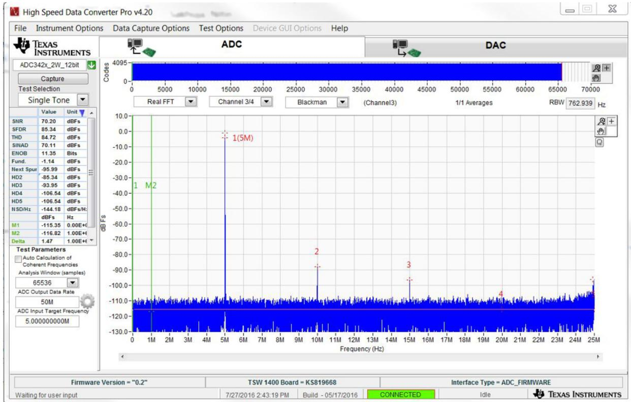
Figure 21. FFT Performance of Combined OPA656, THS4541, and RLC Low-Pass Filter With Updated Gain
