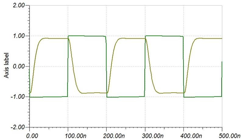
**Figure 16. Simulation With  $\pm 1$ -V, 5-MHz Input Square Wave**
