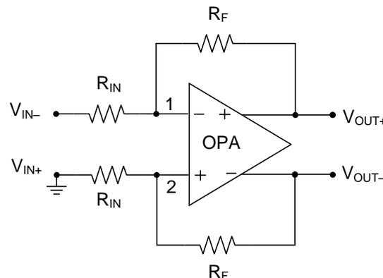
Figure 5. Single-Ended to Differential Amplifier
