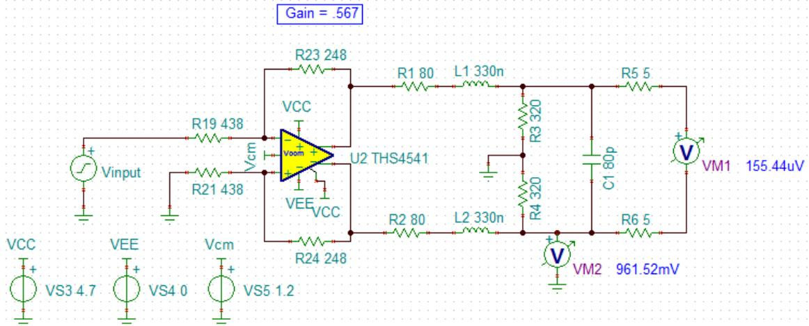
Figure 12. Simulation Circuit Differential Amplifier With RLC Low-Pass Filter
