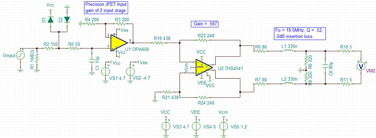
Figure 14. Simulation Circuit for Complete Channel 3
