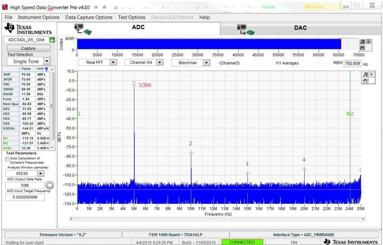
Figure 17. FFT Performance of Combined OPA656, THS4541, and RLC Low-Pass Filter
