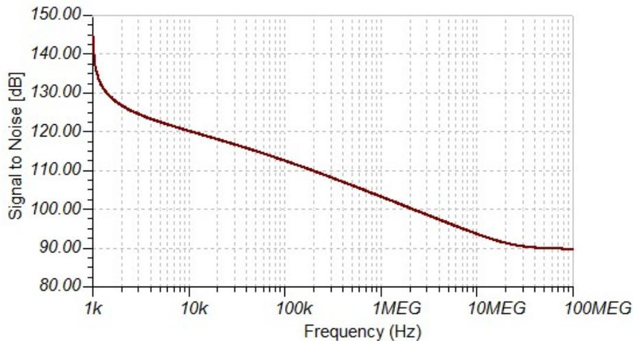
Figure 13. SNR for Differential Amplifier With RLC Low-Pass Filter
