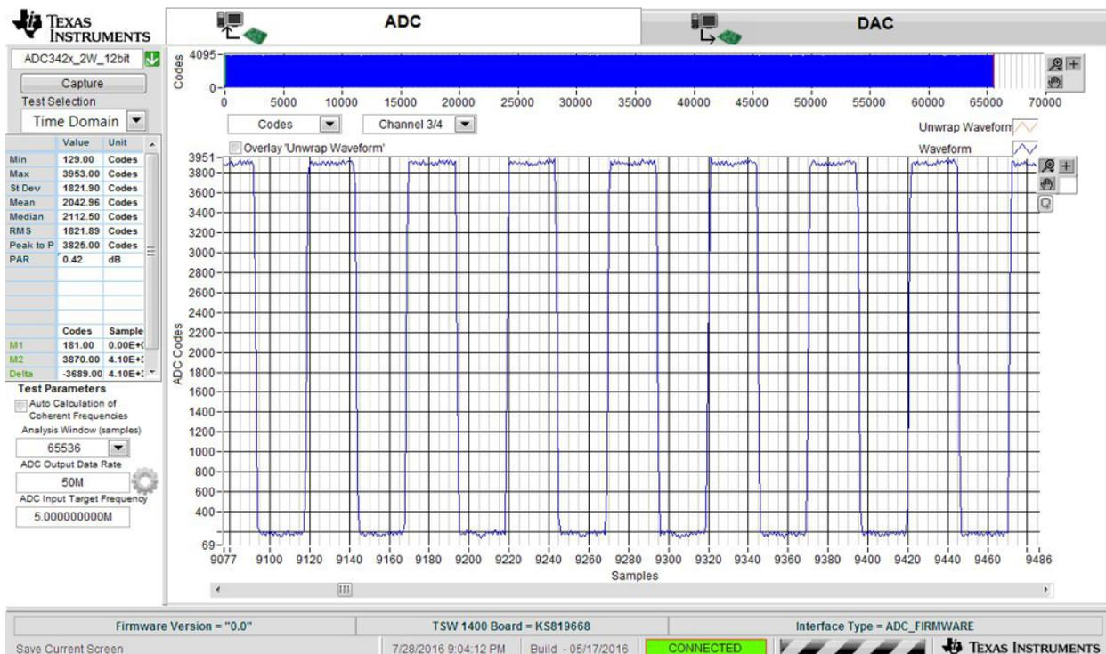
Figure 24. 1-MHz,  $\pm 1$ -V Square Wave Input
