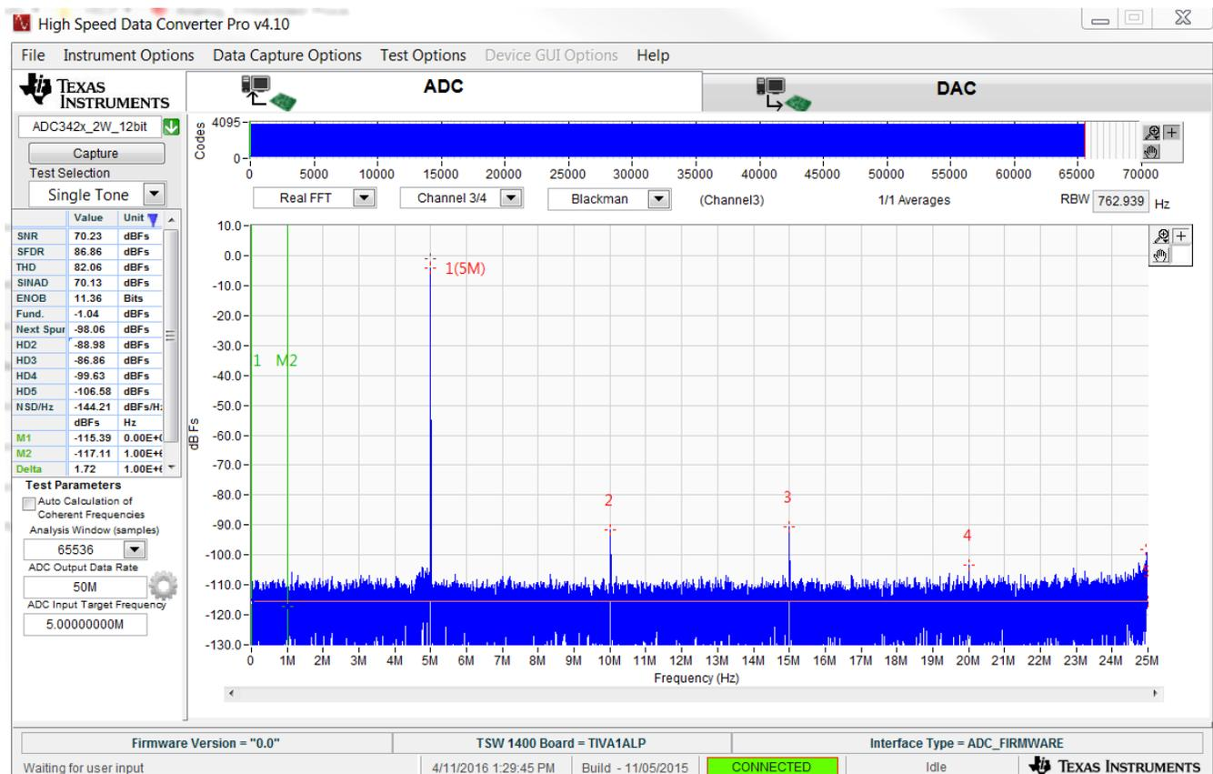
Figure 26. FFT Performance of Transformer Input
