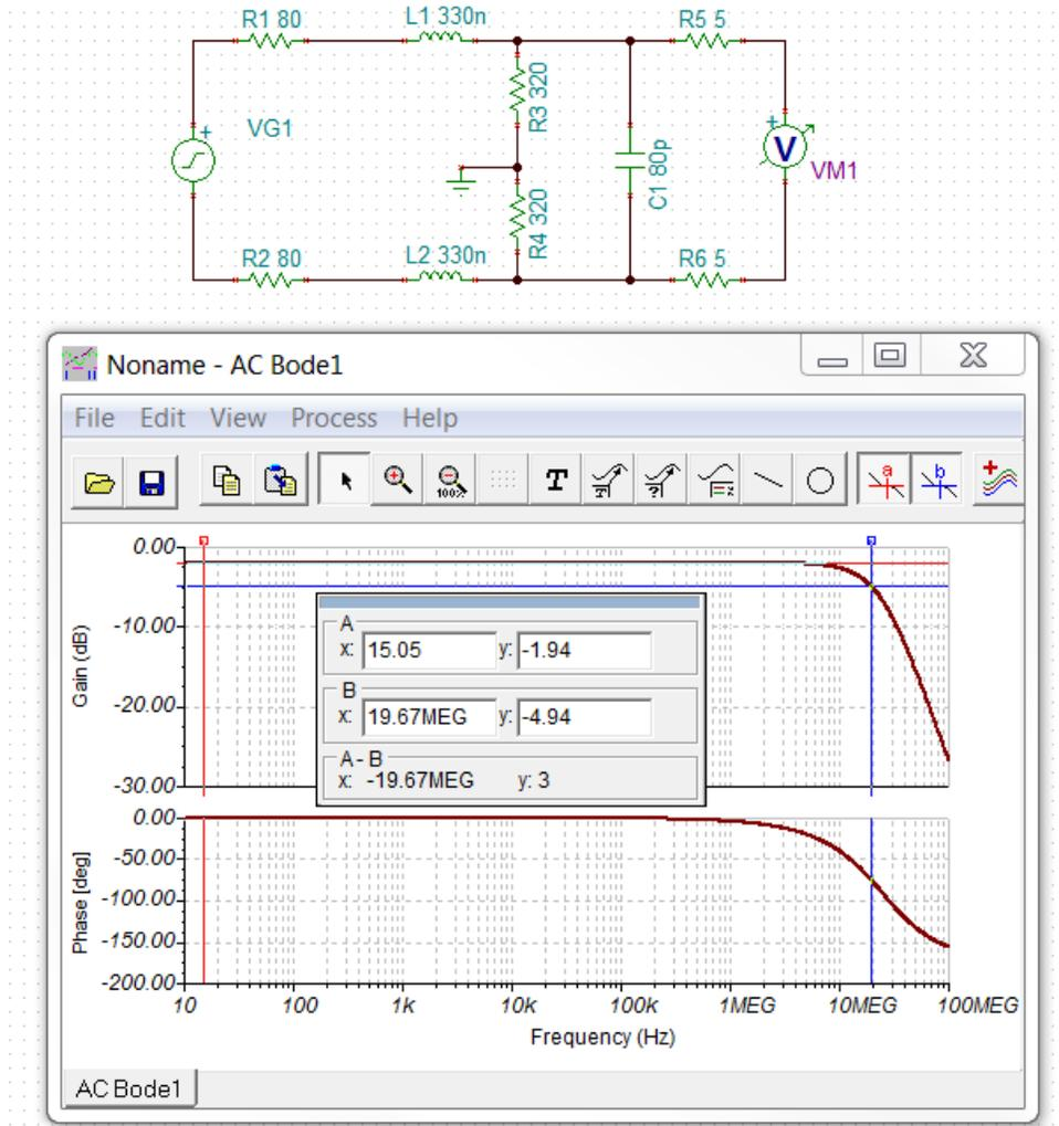
Figure 11. Simulation Circuit and Transfer Function for RLC Low-Pass Filter
