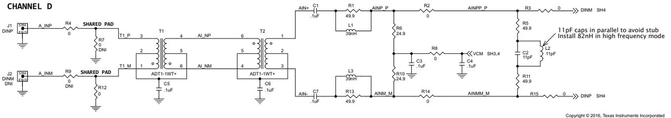
Figure 25. Transformer Coupled Input (Channel 4)
