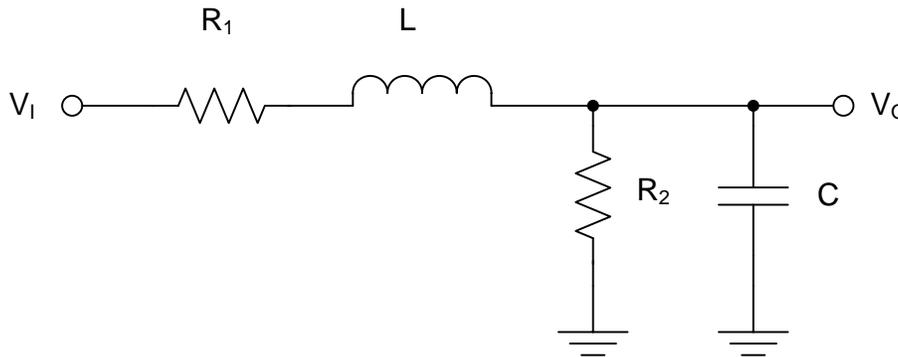
**Figure 8. Single-Ended, Low-Pass RLC Filter**
