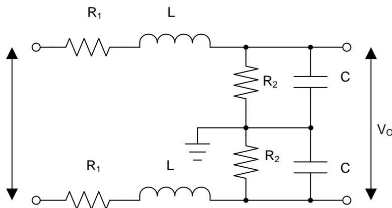
**Figure 9. Differential Low-Pass RLC Filter**
