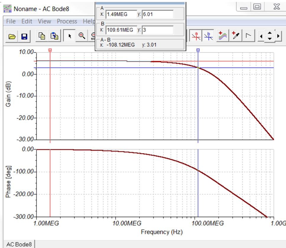
Figure 4. Transfer Function for OPA656 Stage
