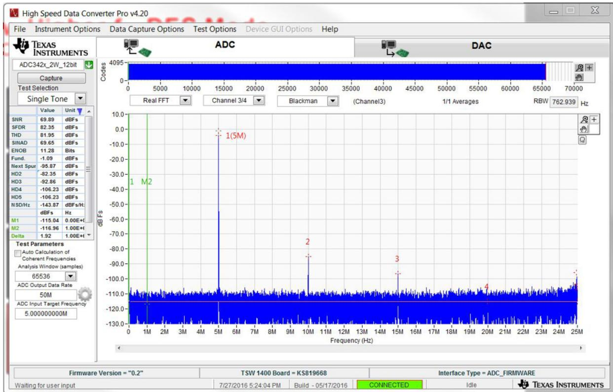
Figure 23. FFT Performance of Combined OPA656, THS4541 With Second-Order Active Filter, and RLC Low-Pass Filter
