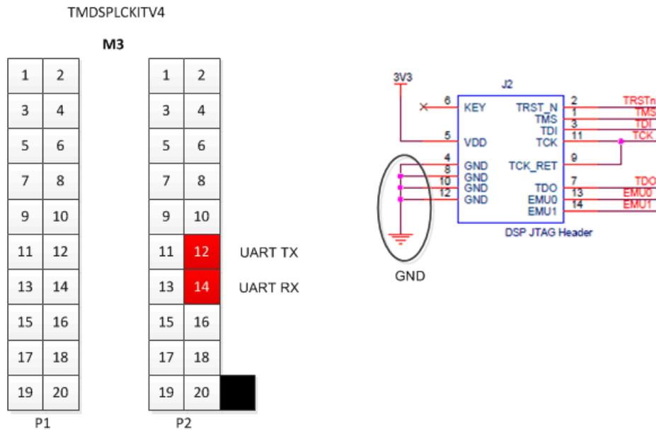
As [Figure 10](#) shows, an additional configuration change is to switch the SW2 position to OFF. Turning off the SW2 blocks UART communication with the mini-USB port in TMDSPCKITV4, which allows the M3 module to communicate with the external device through the UART without interruptions.
