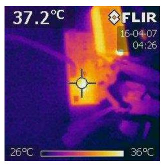
Figure 29. TIDA-00982 Temperature During 1C Discharge
