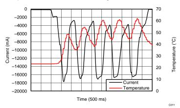
Figure 21 shows the scope shot of a 4 rotor current surge.
