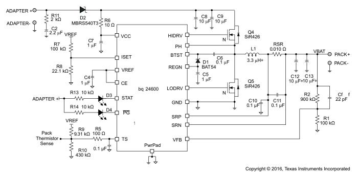
Figure 4. BQ24600 Integrated Li-Ion or Li-Polymer Switch-Mode-Battery-Change Controller.
