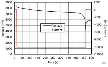
Figure 14. TIDA-00982 10 A Discharge Cycle
