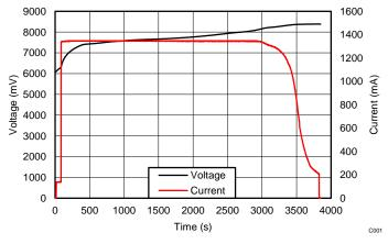
Figure 12. TIDA-00982 1.3 A Charge Cycle
