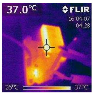
Figure 30. TIDA-00982 Maximum Temperature of Pack During 1C Discharge
