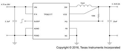
Figure 5. TPS6217x High Efficiency Synchronous Step-Down Dc/DC Converter
