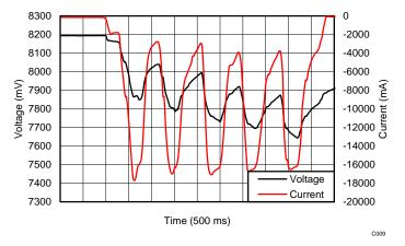
Figure 20. TIDA-00982 Drone Surge Testing for Current and Comms
