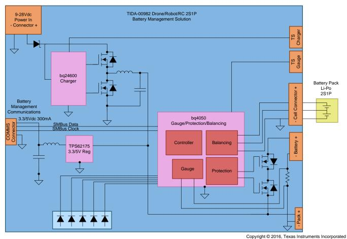
Figure 2. TIDA-00982 Block Diagram
