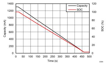
Figure 15. TIDA-00982 10 A Discharge Capacity vs SOC
