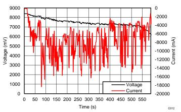
Figure 22 shows the TIDA-00982 drone surge current vs chg\_dschg mosfet temperature.
