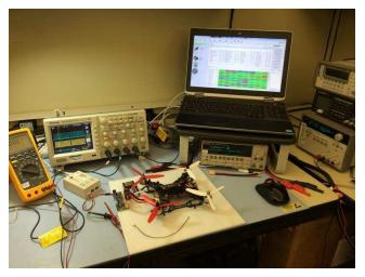
Figure 10. TIDA-00982 Test Bench
