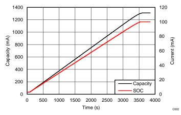
Figure 13. TIDA-00982 1.3 A Charge Capacity vs SOC
