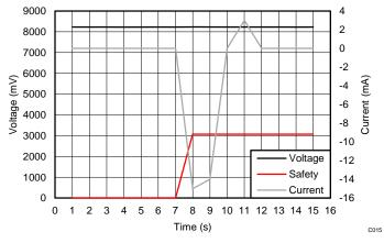
Figure 26. TIDA-00982 Safety Alert Short Circuit
