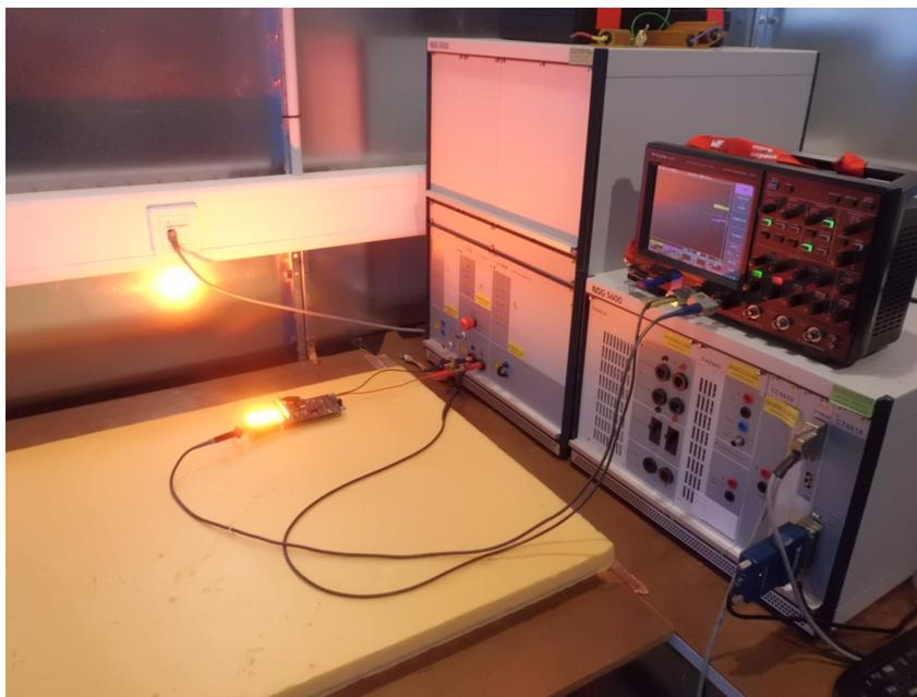
Figure 25. Setup for Transient Tests With LED Board and NSG 5500 Transient Generator
