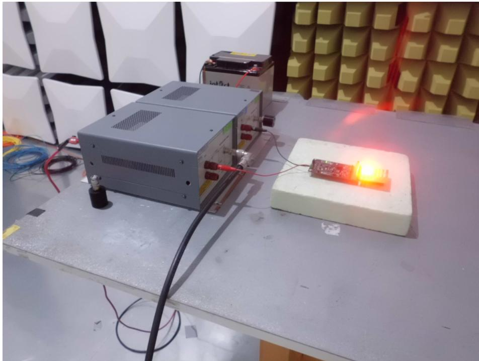
**Figure 39. Conducted-Emissions Setup**
