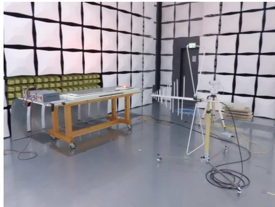
**Figure 44. Radiated Emissions Setup With a Logarithmic Antenna: 30 MHz to 2.5 GHz**
