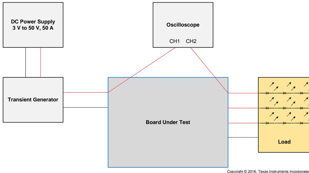
Figure 24. Test Setup for Load Dump, Cold Crank, Jump Start, and Reverse Battery
