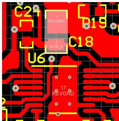
Figure 51. Input and Output Capacitor Placement
