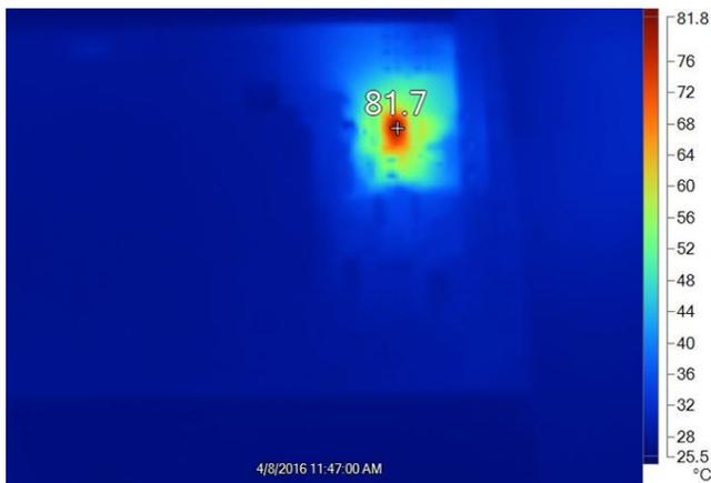
Figure 28. TPS92630-Q1 Linear LED Driver-Temperature at Three Strings of 100-mA LEDs
