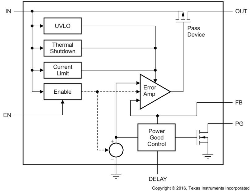
**Figure 6. TPS7A1633-Q1 LDO Voltage Regulator**
