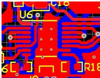
**Figure 48. TPS92630-Q1 Thermal Vias Under LED Driver**
