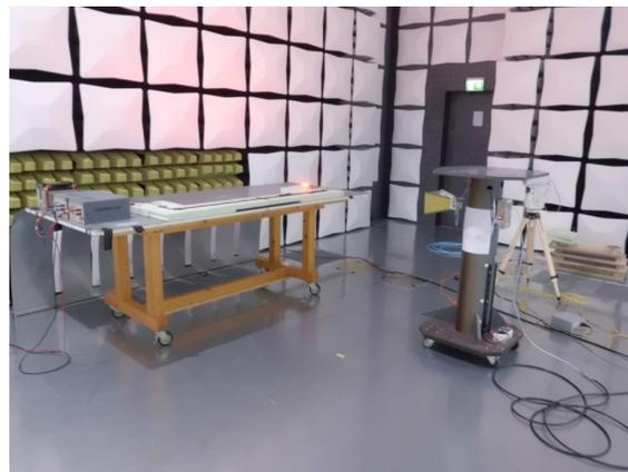
**Figure 45. Radiated Emissions Setup With a Horn Antenna: 1.447 GHz to 1 GHz**
