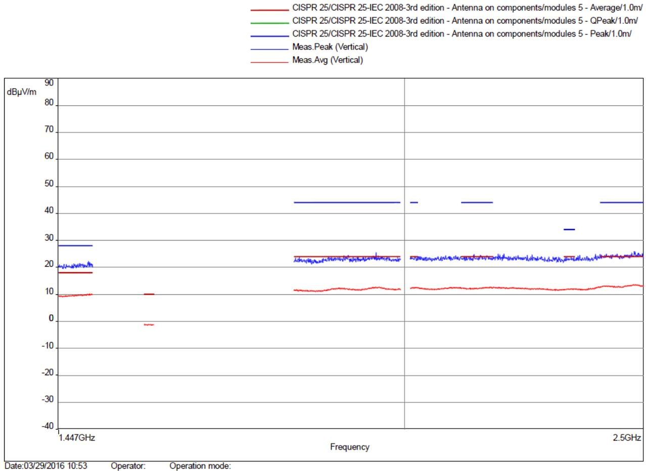
**Figure 47. Radiated Emissions: Line Side 1.44 GHz to 2.5 GHz with Horizontally-Oriented Antenna**
