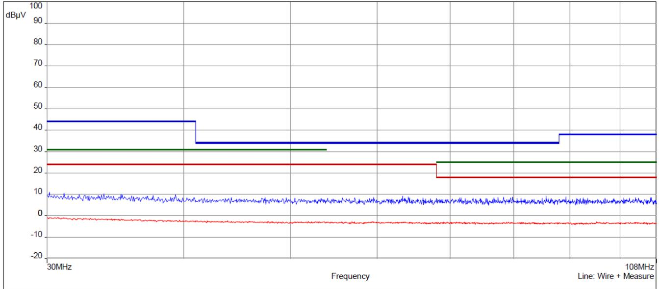
**Figure 41. Ambient-Noise Level 2: Line Side 30 MHz to 108 MHz**
