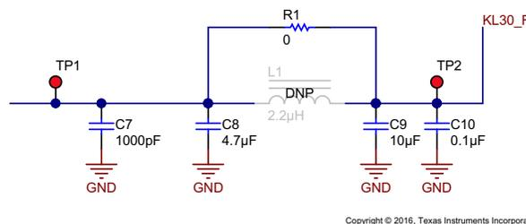
**Figure 13. Input-Voltage Noise Filter**
