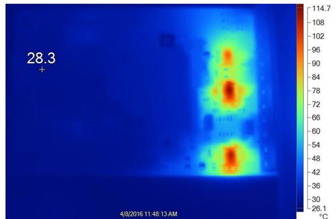
Figure 29. TPS40210 Smart-Reverse Battery Diode Temperature at 12 V Input Voltage
