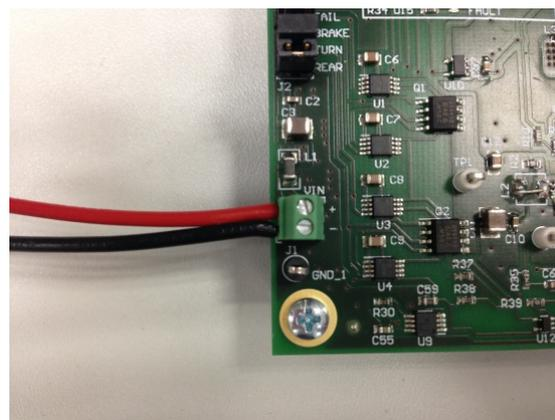
**Figure 21. Board Supply-Input Terminal**
