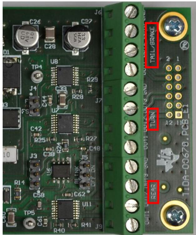
**Figure 18. Screw Terminals for LED-String Outputs (100 mA and 150 mA, Maximum of 9 Strings, Maximum Output Voltage of 16.5 V)**
