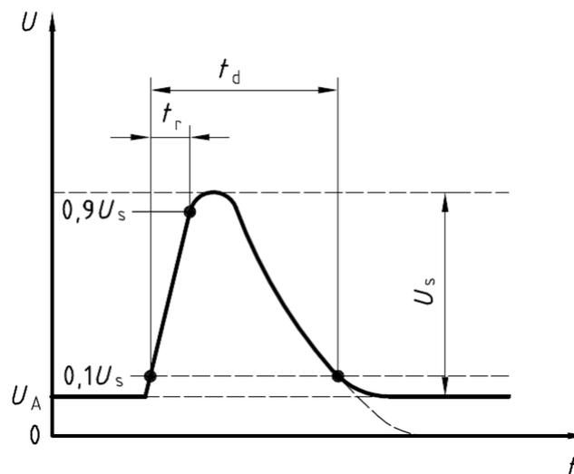
Figure 7. Load-Dump Pulse
