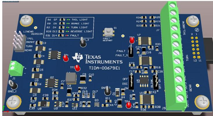
Figure 11. 3D Rendering of the TIDA-00679 Board
