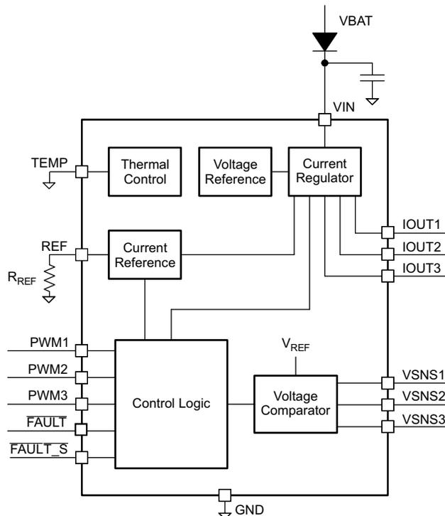
**Figure 3. TPS92630-Q1 Linear LED Block Diagram**
