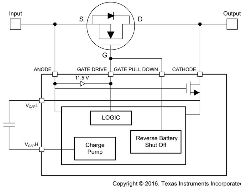
Figure 4. LM74610-Q1 Zero  $I_Q$  Reverse-Polarity Protection Smart-Diode Controller
