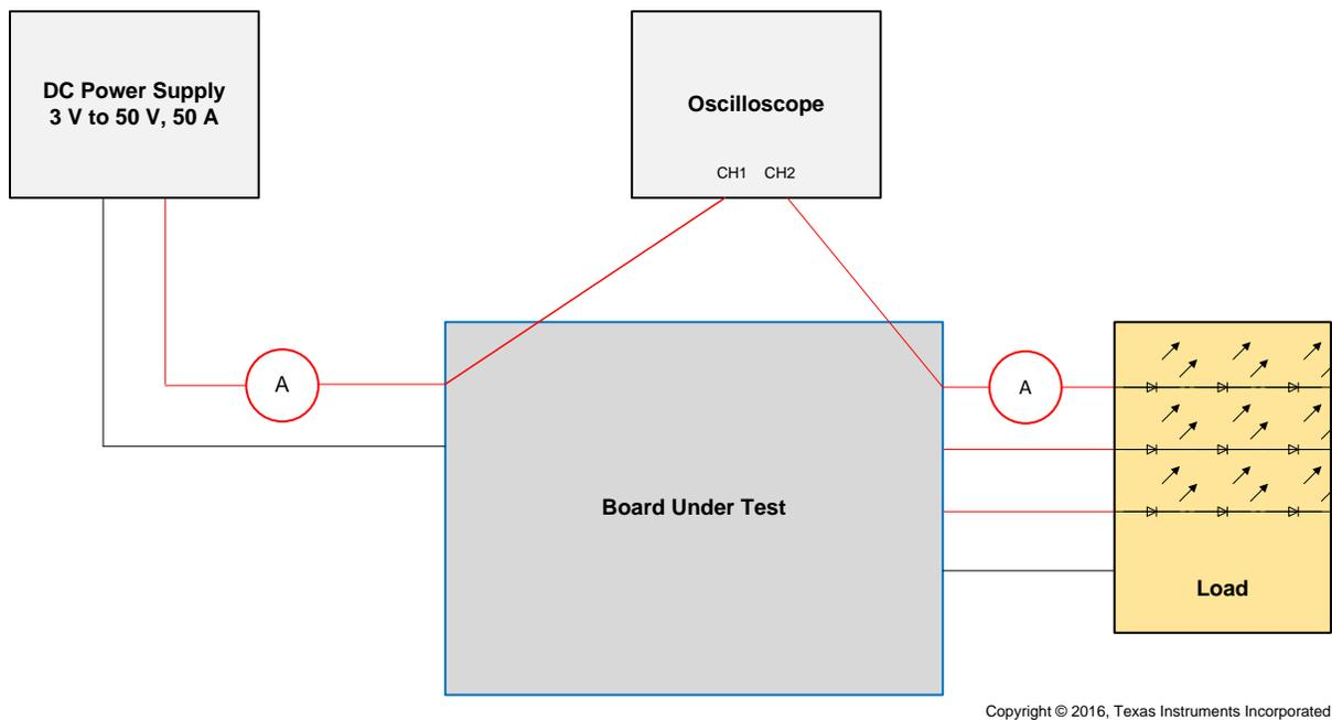
**Figure 27. Efficiency-Test Setup**
