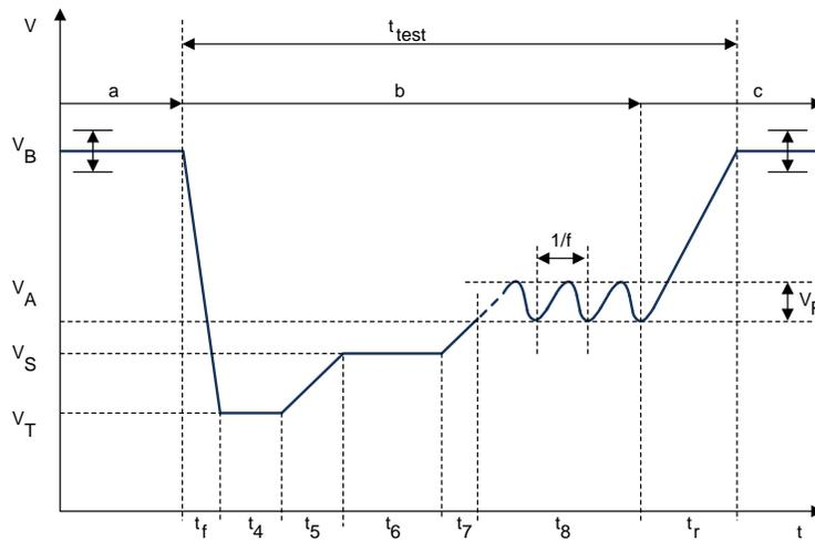
Figure 37. Cold-Crank Wave Shape
