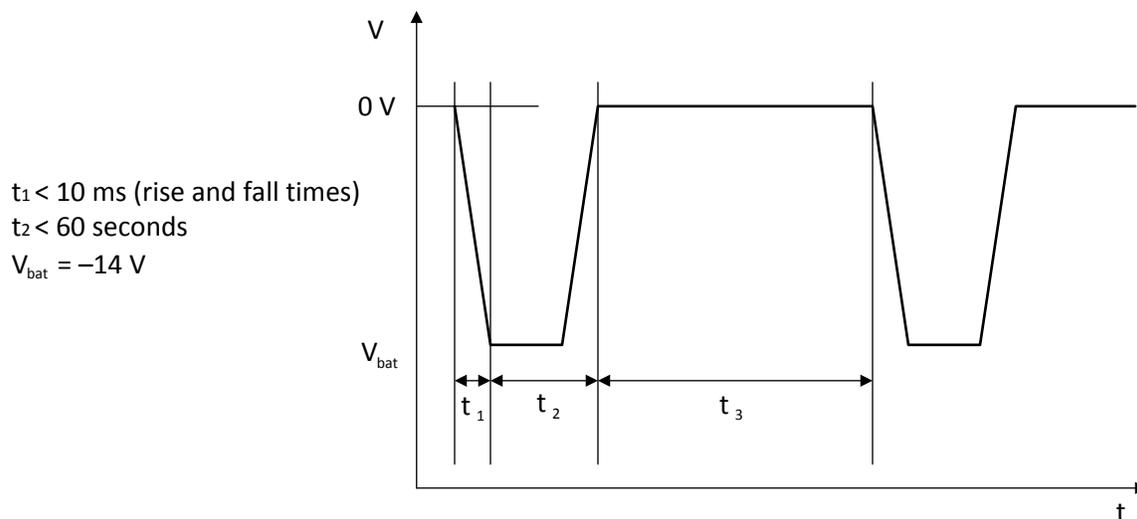
**Figure 9. Reverse-Battery Pulse**
