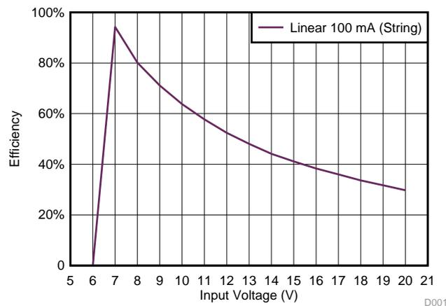
Figure 30. Efficiency Versus Input Voltage at  $I_{LED} = 100$  mA per String
