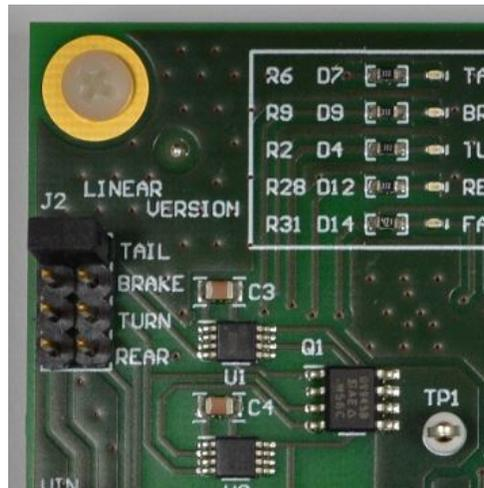
**Figure 19. Jumper J2 for Setting the Type of Light**
