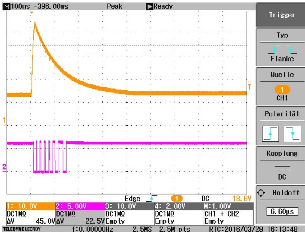
Figure 32. Load Dump and Output: Thermal Toggling and No Complete Turnoff
