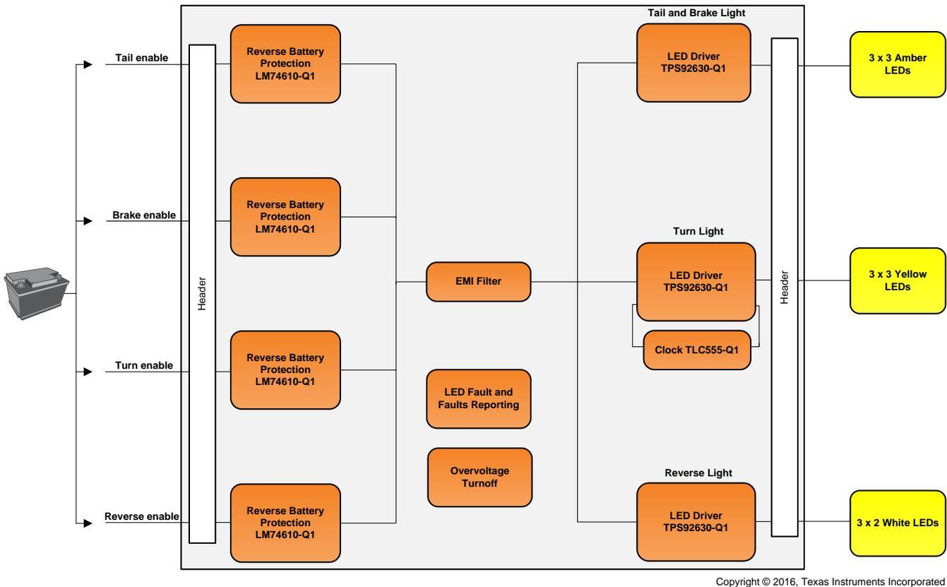
**Figure 1. Tail-Light System Driven From the Car Battery**
