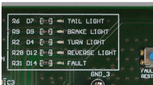
Figure 22. LEDs Indicating Failures and On Lights
