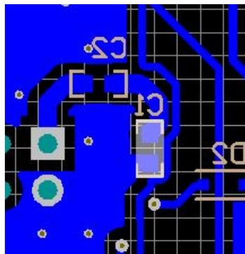
Figure 52. Arrangement of Capacitors Connected to Battery
