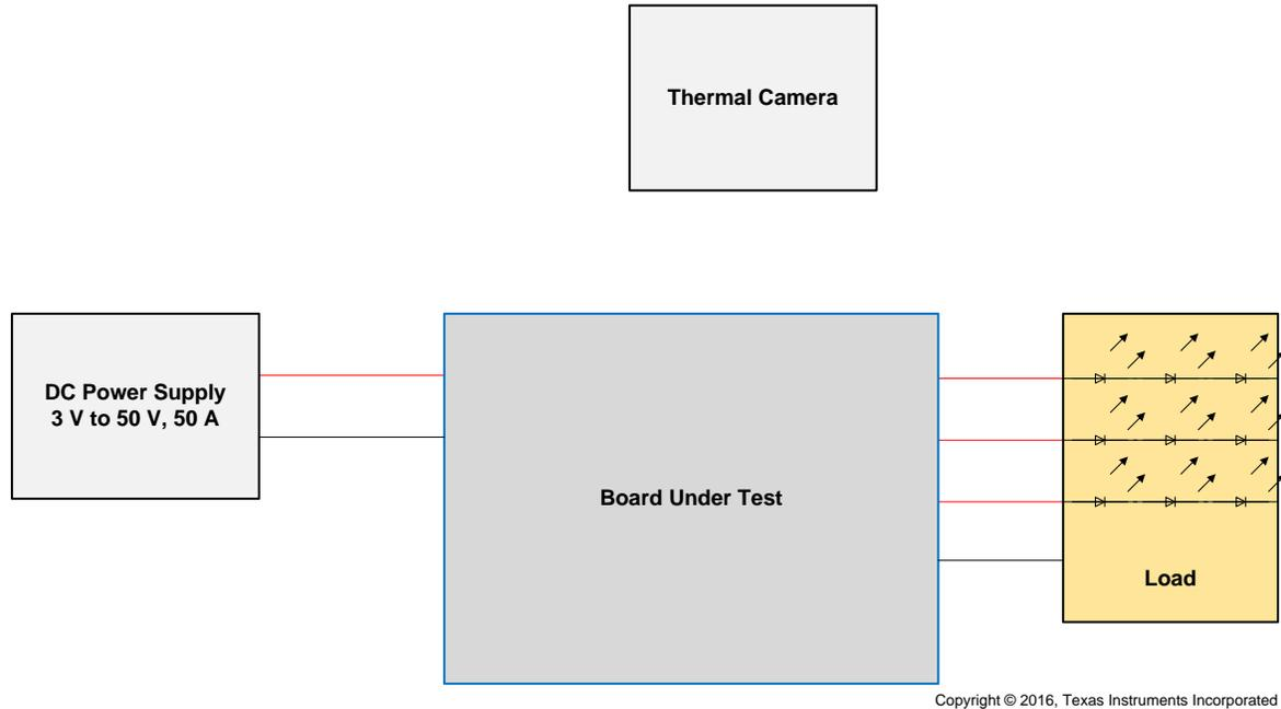
**Figure 26. Setup to Measure Thermal Behavior of the Board**
