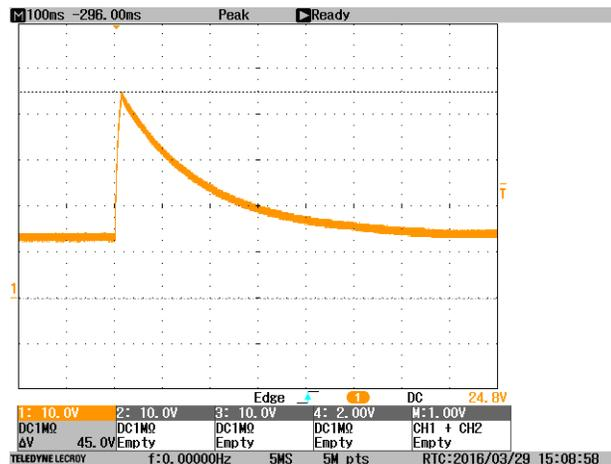
Figure 31. ISO 7637-2:2004 Pulse 4 Load Dump
