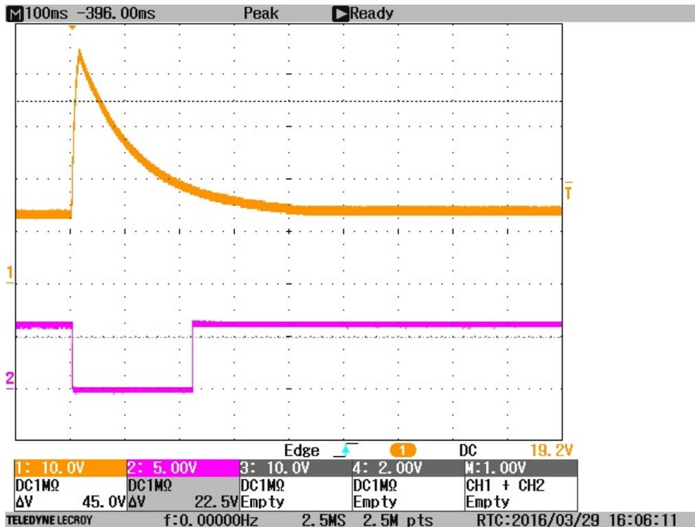
Figure 33. Load Dump and Output: Turned Off at > 17 V then Turned On
