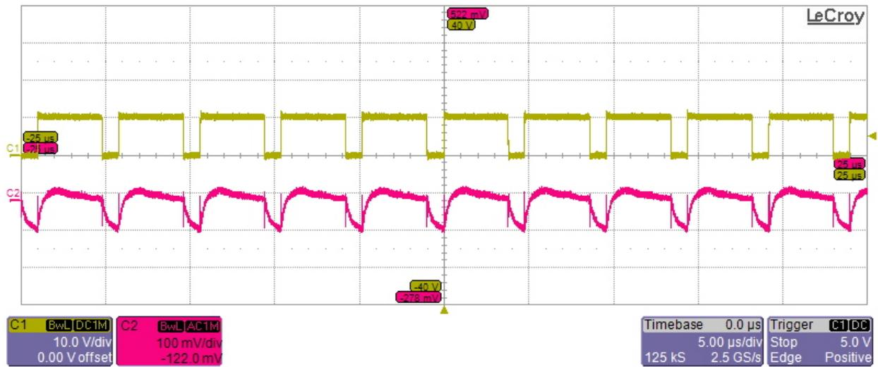
Ch2- 10V Ripple at 8Vin and 5A Load
