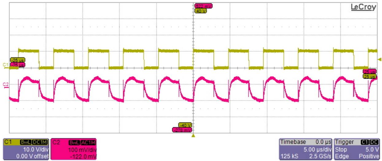
**Ch2- 10V Ripple at 6.8Vin and 5A Load**
