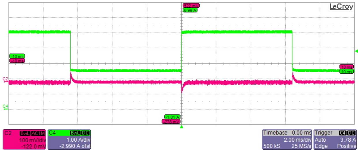
**Transient performance of 5V\_Buck at 3.5V and 2.5A to 5A Current transient (No Load on Other buck output)**
