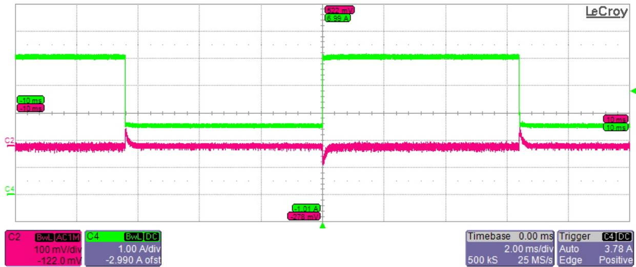
Transient performance of 5V\_Buck at 6V and 2.5A to 5A Current transient (No Load on Other buck output)
