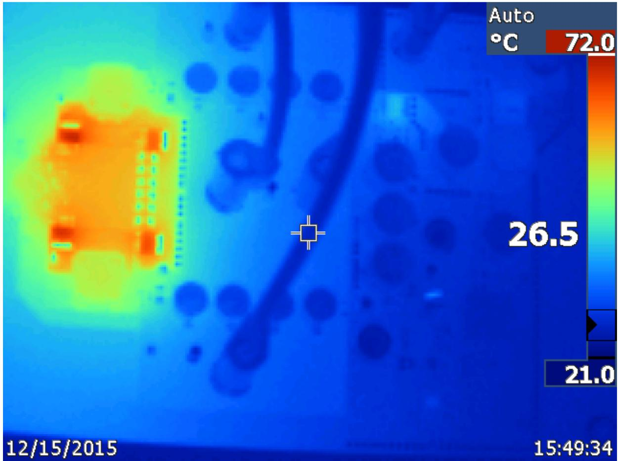
IR thermal image taken at steady state with 6 Vin and 5V@5A and 3.3V @ 5A (Boost is operational)
