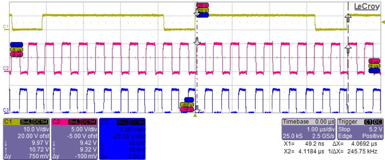
**C2 – 5V Switch node at 8Vin and 5A Load**
