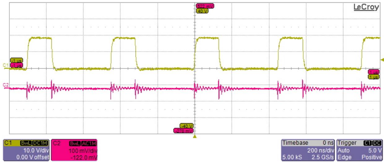
**Ch2- 5V Ripple at 18 Vin and 5A Load**
