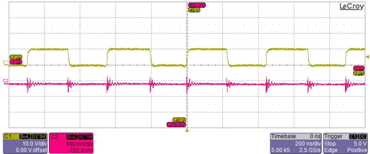
Ch2- 5V Ripple at 3.5 Vin and 5A Load
