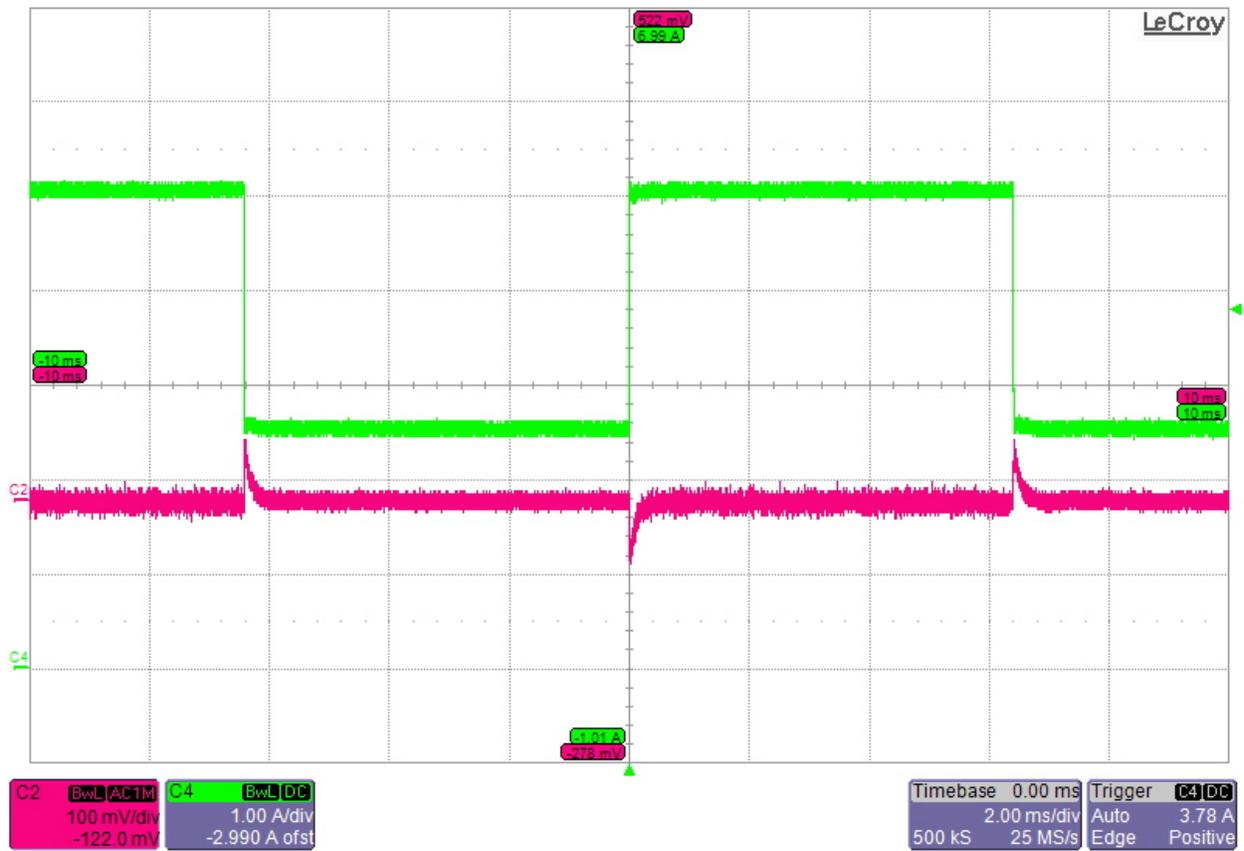
**Transient performance of 5V\_Buck at 12V and 2.5A to 5A Current transient (No Load on Other buck output)**
