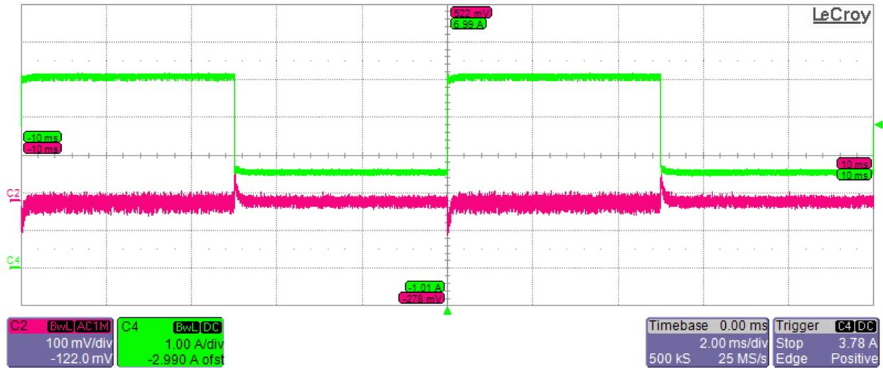
Transient performance of 3.3V\_Buck at Low Vin (5V) and 2.5A to 5A Current transient (No Load on Other buck output)
