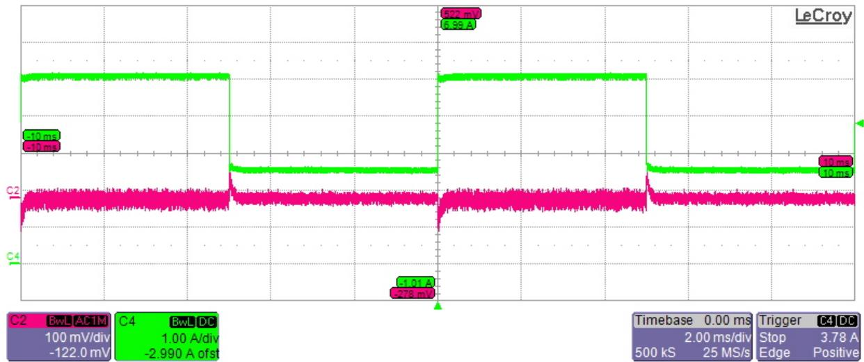
Transient performance of 3.3V\_Buck at 6V and 2.5A to 5A Current transient (No Load on Other buck output)
