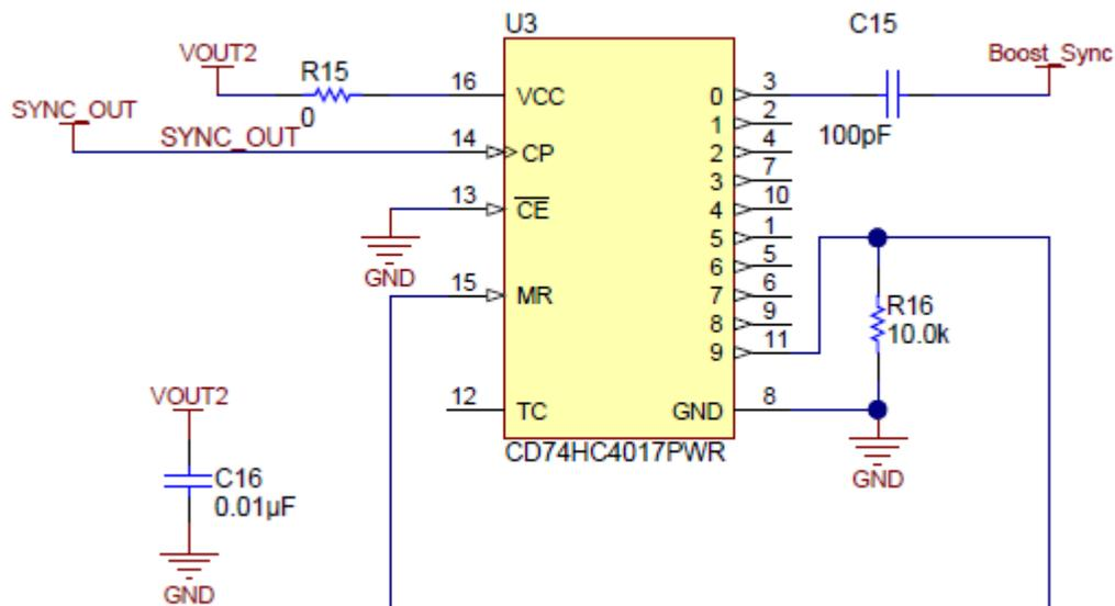
Buck SYNC\_OUT used to synchronize Boost controller at Freq/9 (divide/9through counter)
