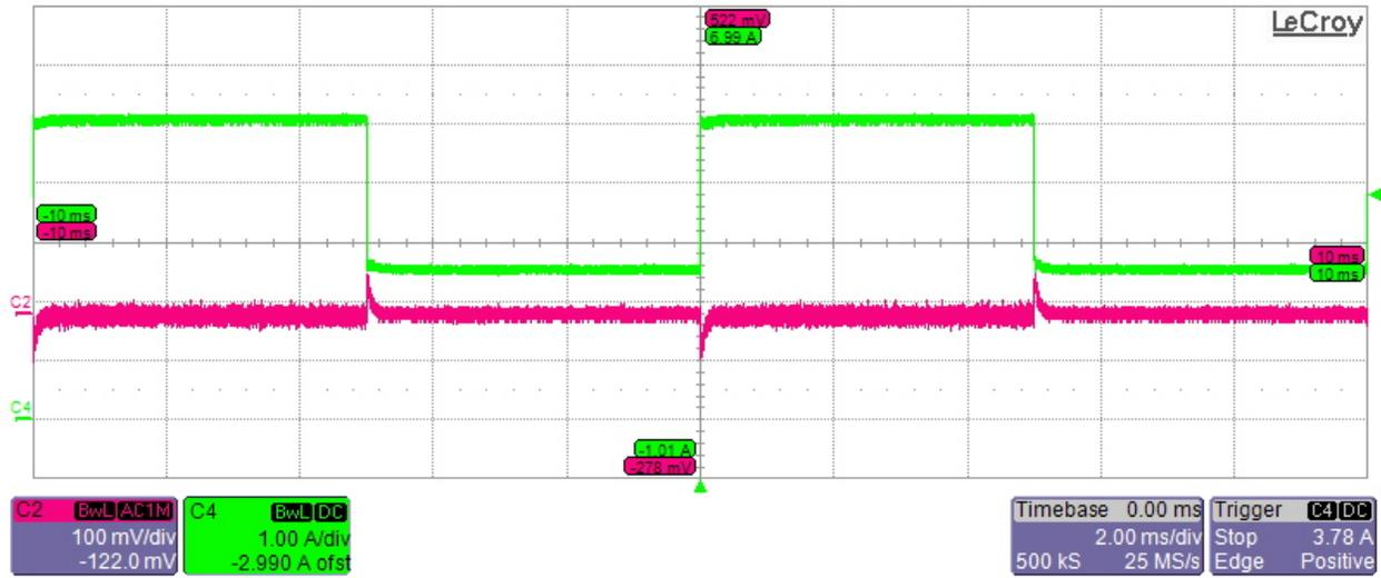
Transient performance of 3.3V\_Buck at 8V and 2.5A to 5A Current transient (No Load on Other buck output)
