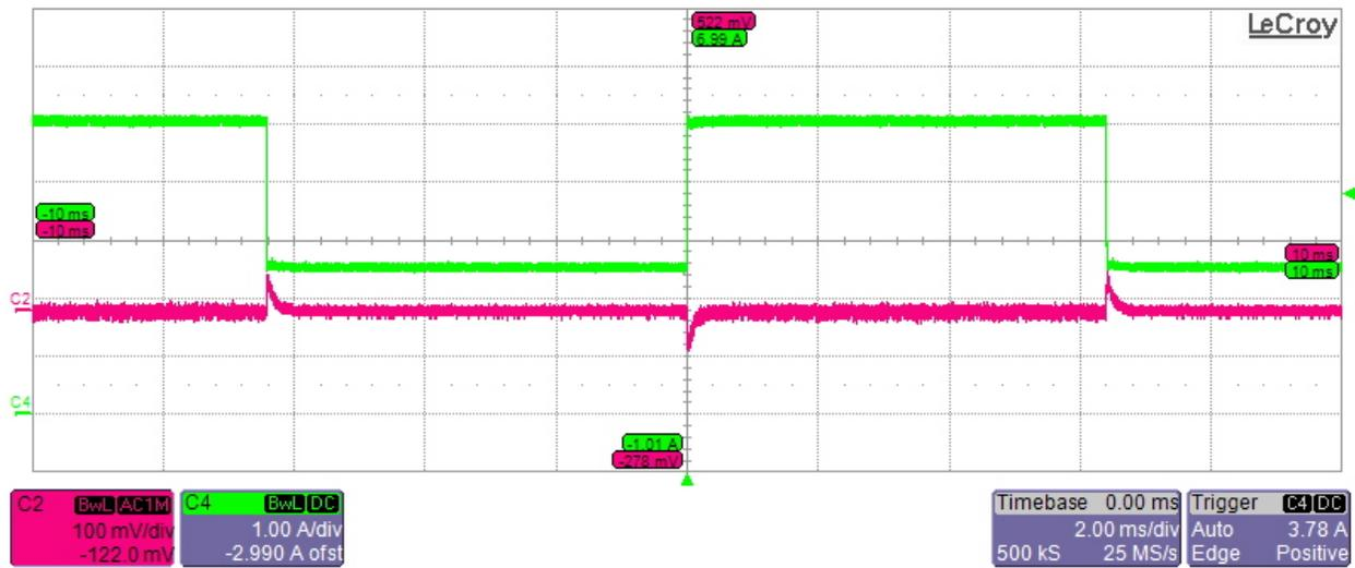
Transient performance of 5V\_Buck at 4.5V and 2.5A to 5A Current transient (No Load on Other buck output)
