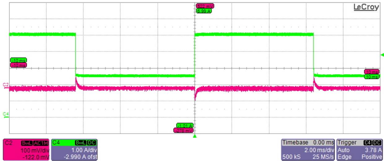
**Transient performance of 5V\_Buck at 8V and 2.5A to 5A Current transient (No Load on Other buck output)**
