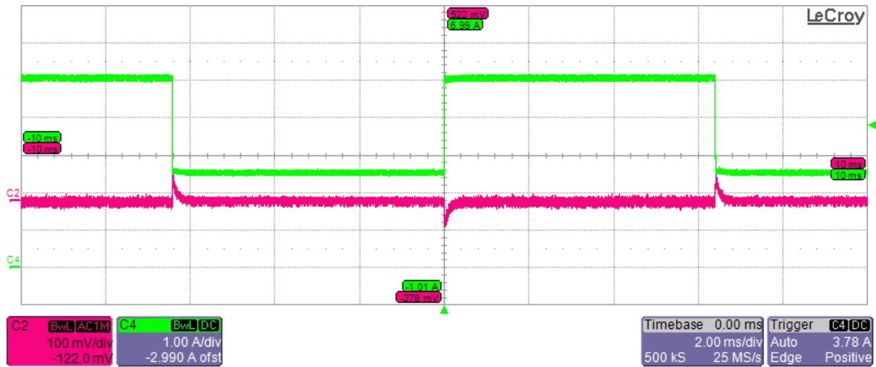
**Transient performance of 5V\_Buck at 18V and 2.5A to 5A Current transient (No Load on Other buck output)**
