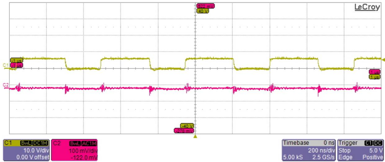
**Ch2- 3.3V Ripple at 6Vin and 5A Load**
