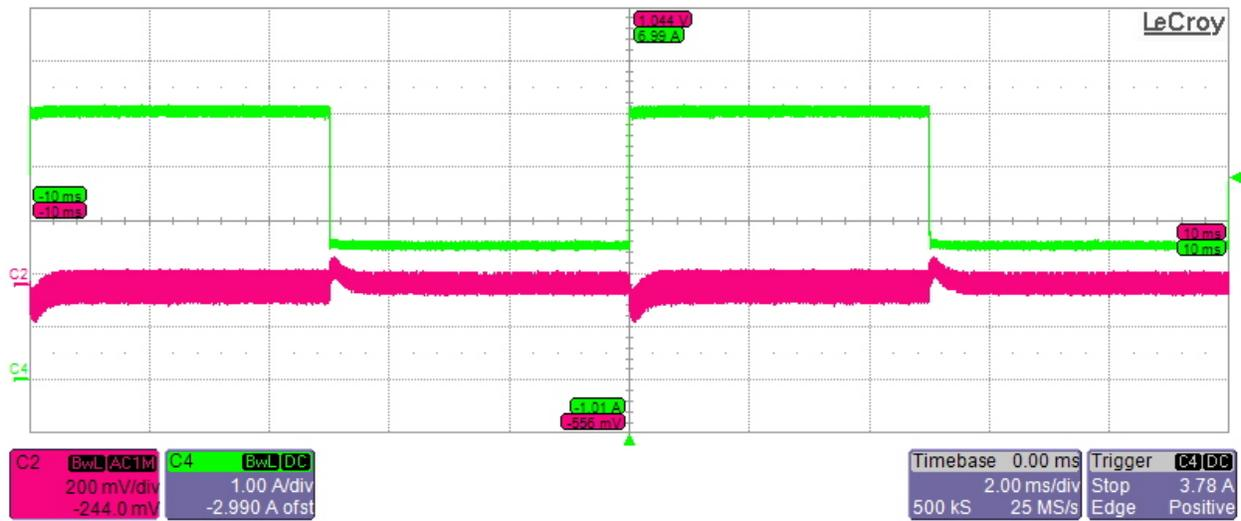
Transient performance of 10V\_Boost at 8V and 2.5A to 5A Current transient (Load on Boost output only)
