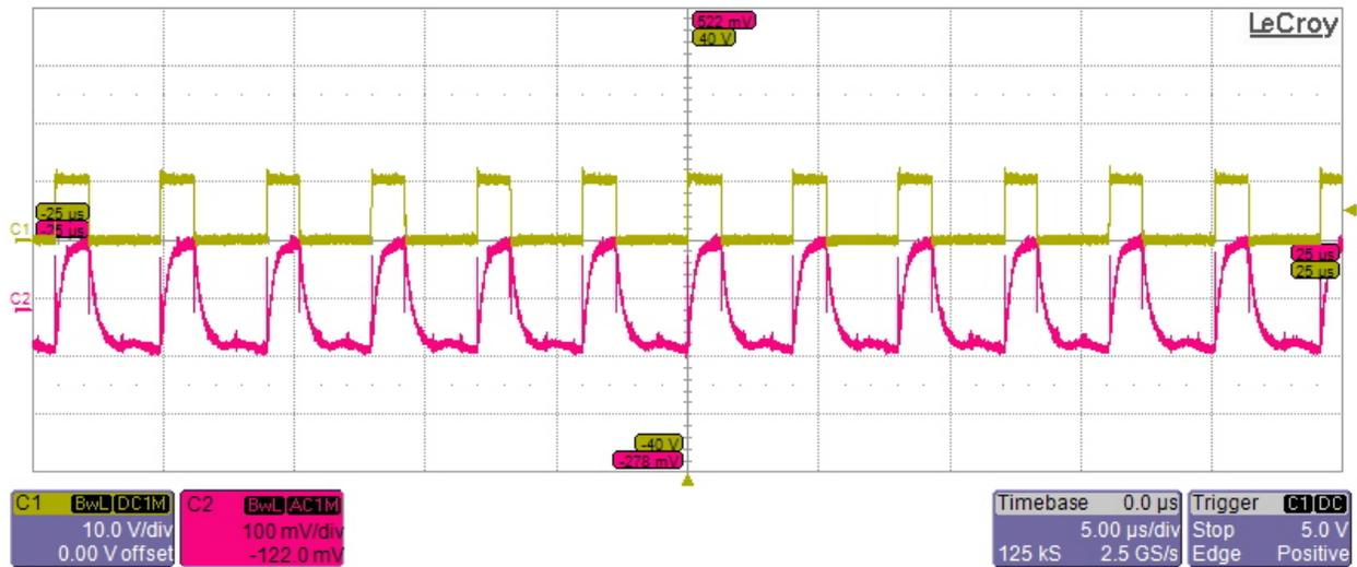
Ch2- 10V Ripple at 3.5Vin and 5A Load
