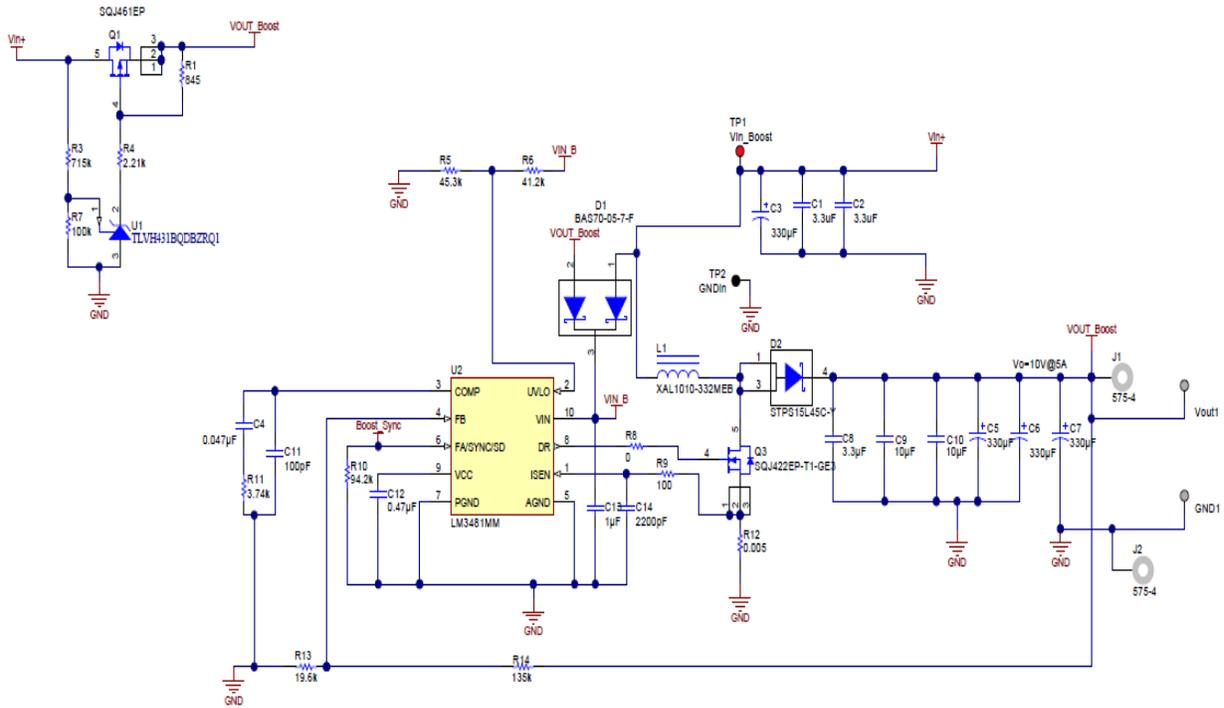
So When  $V_{in} > 10.5\text{ V}$  , Boost is bypassed through PFET .
