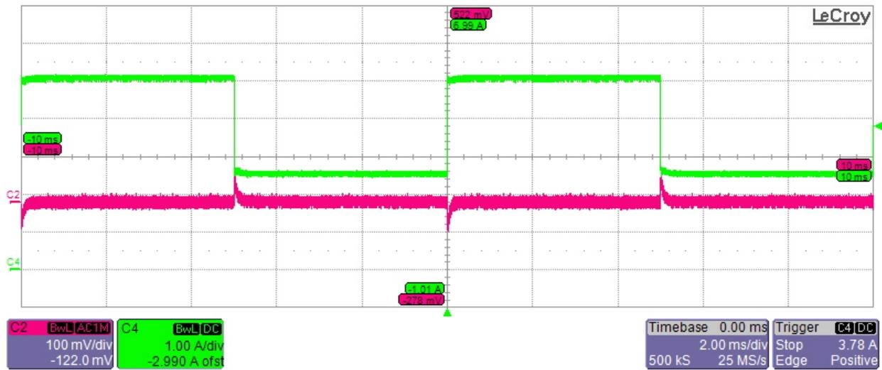
Transient performance of 3.3V\_Buck at 18V and 2.5A to 5A Current transient (No Load on Other buck output)
