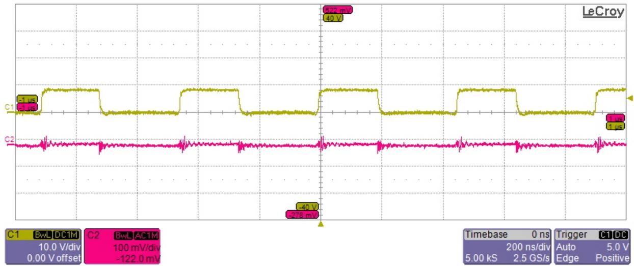
**Ch2- 3.3V Ripple at 8 Vin and 5A Load**
