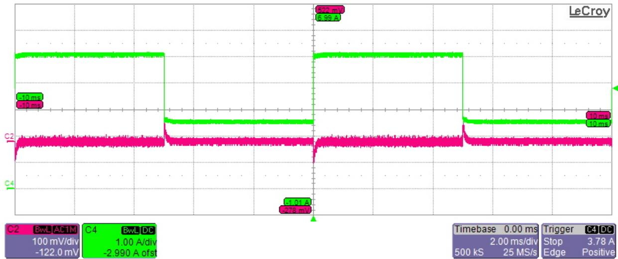
Transient performance of 3.3V\_Buck at 12V and 2.5A to 5A Current transient (No Load on Other buck output)
