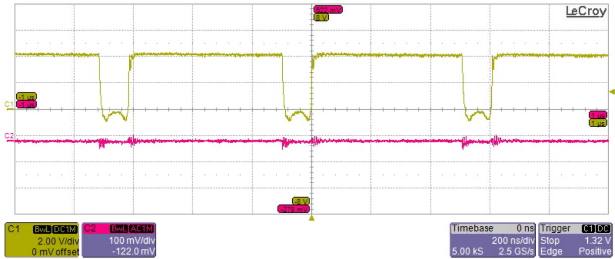
**Ch2- 3.3V Ripple at 4.5 Vin and 5A Load**
