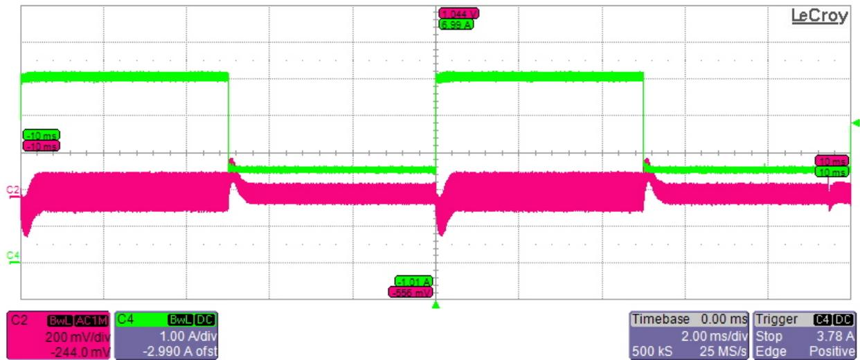
Transient performance of 10V\_Boost at Low Vin (4V) and 2.5A to 5A Current transient (Load on Boost output only)
