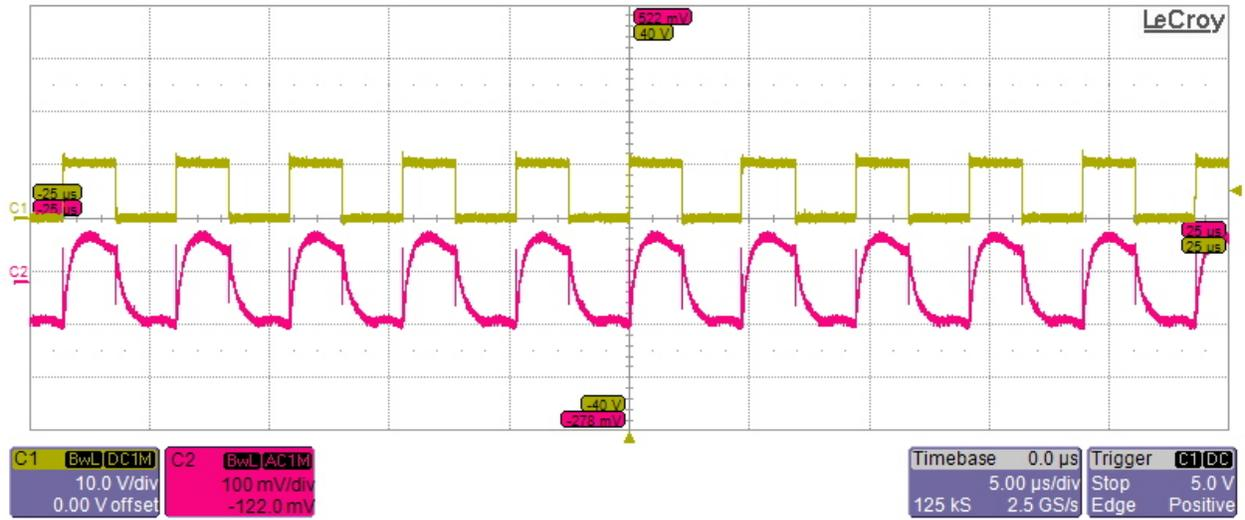
Ch2- 10V Ripple at 5Vin and 5A Load
