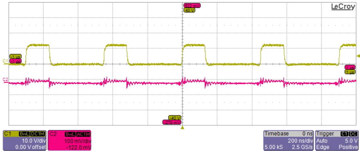
**Ch2- 3.3V Ripple at 12 Vin and 5A Load**
