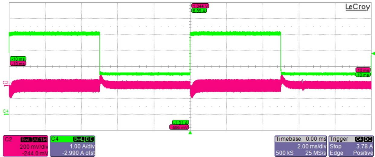
Transient performance of 10V\_Boost at 6V and 2.5A to 5A Current transient (Load on Boost output only)
