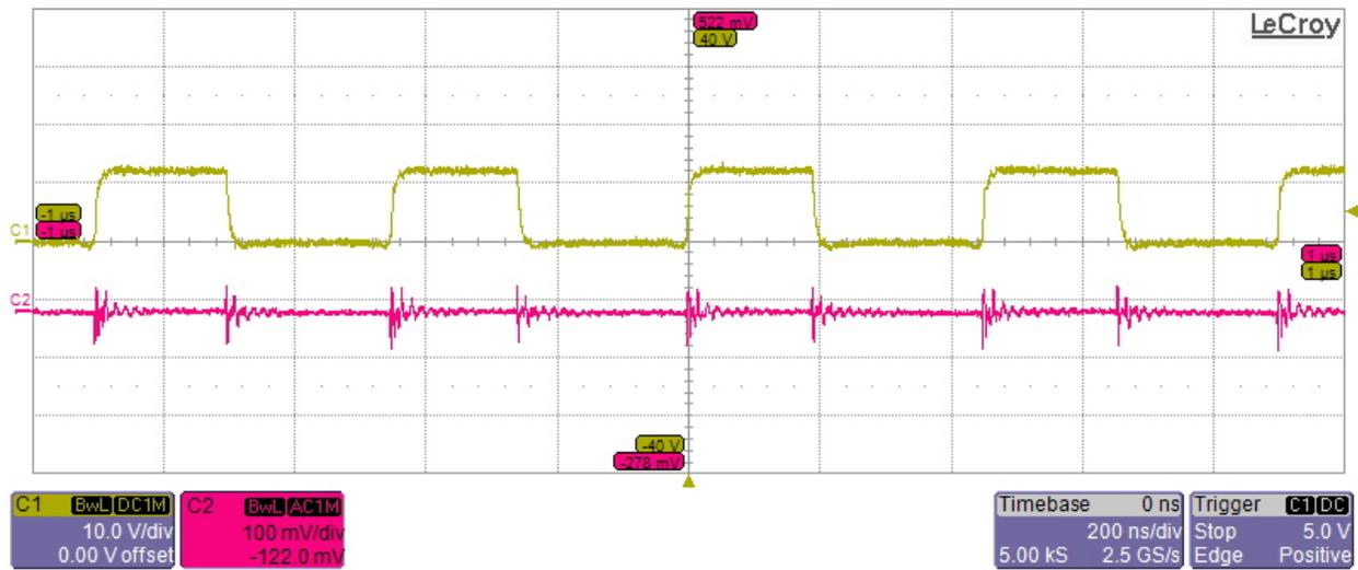
**Ch2- 5V Ripple at 12 Vin and 5A Load**
