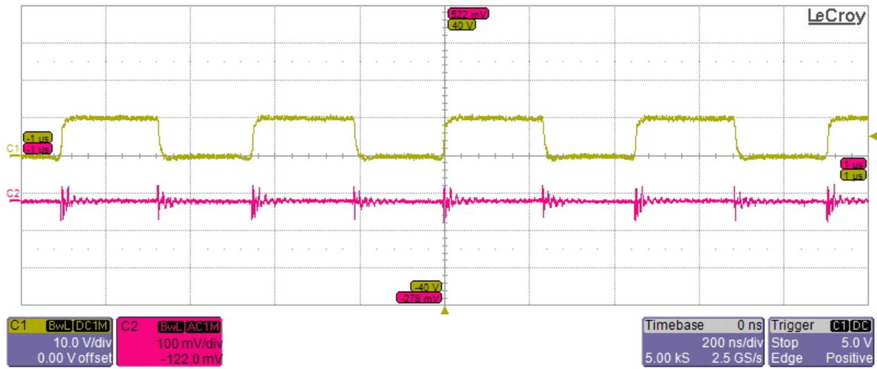
**Ch2- 5V Ripple at 8 Vin and 5A Load**
