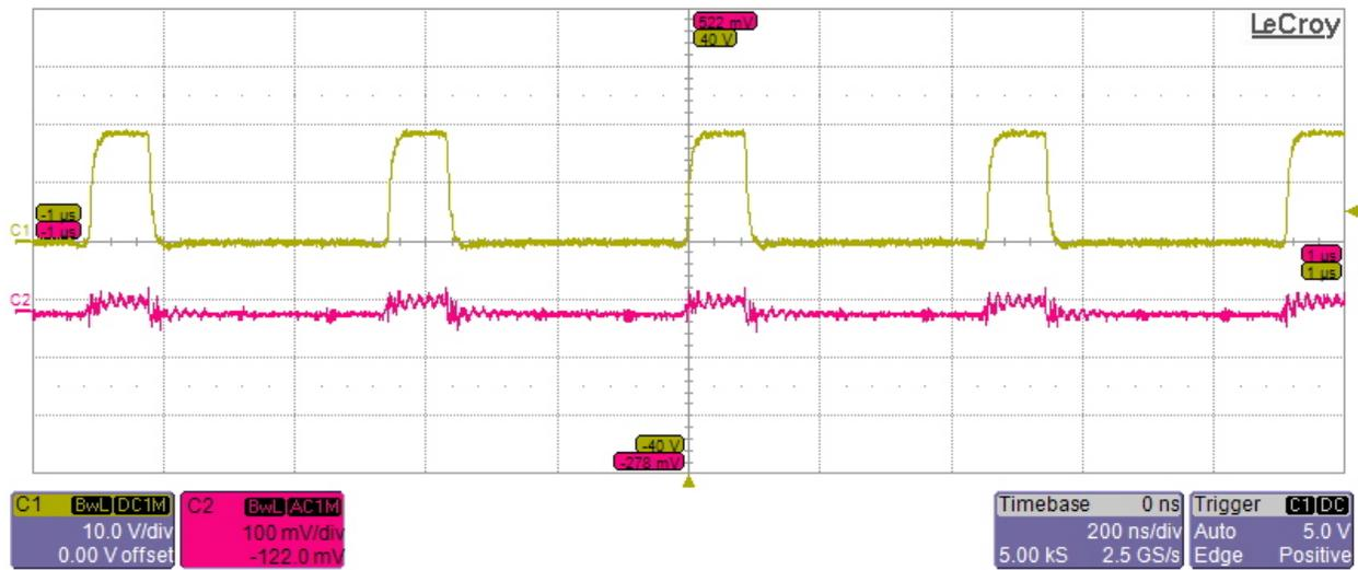
**Ch2- 3.3V Ripple at 18 Vin and 5A Load**
