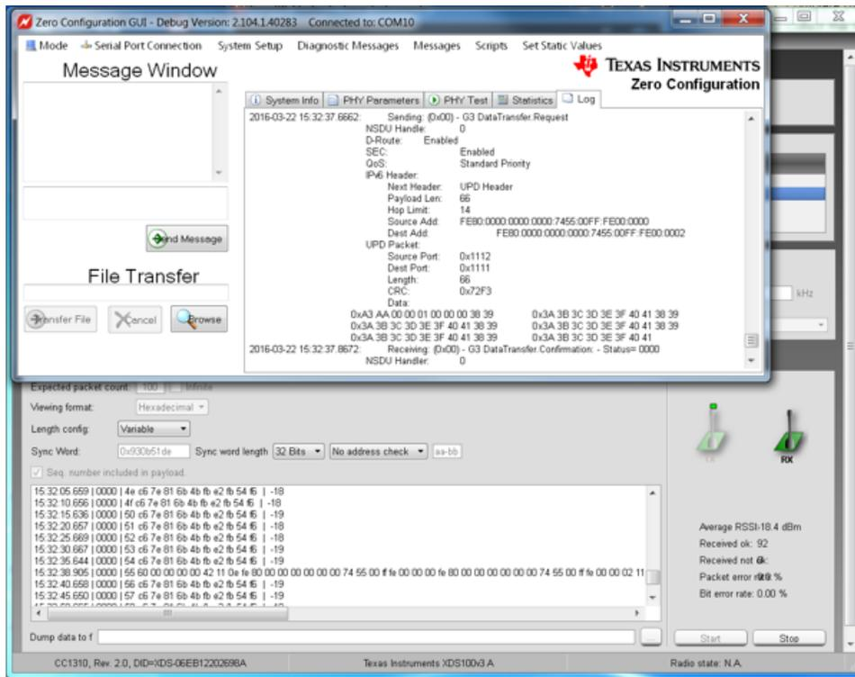
Figure 29 shows test results of the RF-to-PLC repeater. For the test, the RF node sent a 5B text message. Once the 5B packet is received at the Hybrid RF/PLC node, the node passes the received data to the PLC link. The zero-configuration GUI shows the packet reception (in forms of G3 Data Transfer Indication) in the zero-configuration GUI (top in Figure 29). The received packet at PLC includes 6B of information (5B message + 1B sub-header inserted by the RF transmitter).
