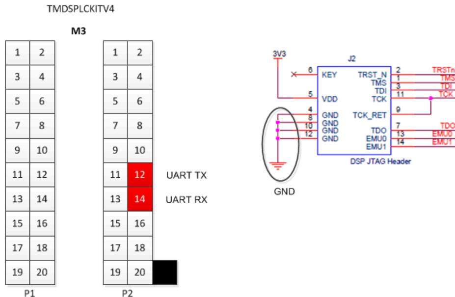
As shown in Figure 10, additional configuration change is SW2 position to OFF. Turning off the SW2 blocks UART communication with the mini-USB port in TMDSPCKITV4. Thus, it allows the M3 module to communicate with external device through UART without any interrupts.
