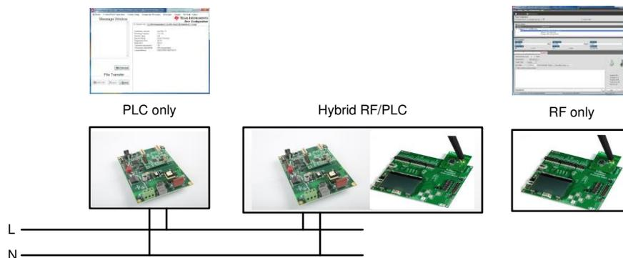
For the Hybrid RF/PLC test, the PLC only node is configured as the G3-PLC mini-DC node. The RF only node can run as the PACKET\_RX mode to capture RF packets or the PACKET\_TX mode to transmit RF packets. The PACKET\_RX mode shows simultaneous transmissions from the Hybrid RF/PLC node, and the PACKET\_TX mode shows RF-to-PLC repeater functionality on the Hybrid RF/PLC node.
