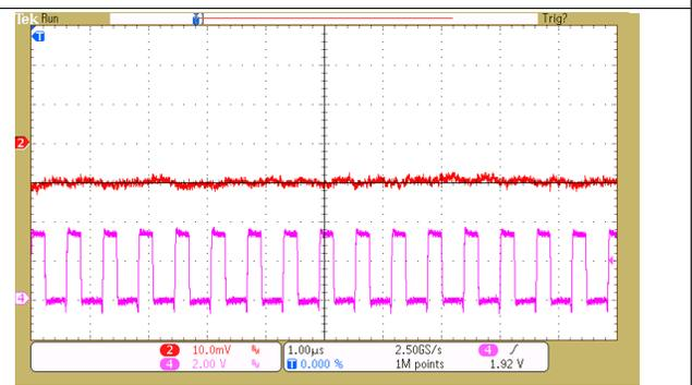
Figure 20. TPS6508640 BUCK4 – VMGTAVCC Output Ripple
