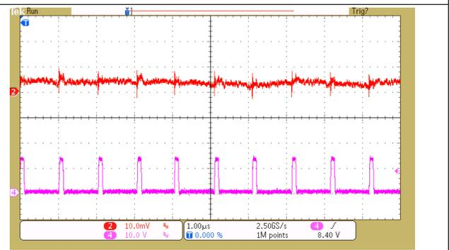
Figure 22. TPS6508640 BUCK6 – VCCODDR Output Ripple
