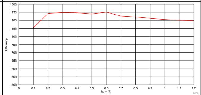
Figure 8. TPS6508640 BUCK5 – 1.8-V AUX Efficiency
