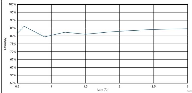
Figure 5. TPS6508640 BUCK2 – VCCPINT Efficiency
