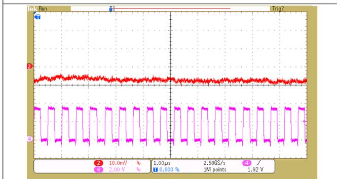
Figure 19. TPS6508640 BUCK3 – VGM TAVTT Output Ripple
