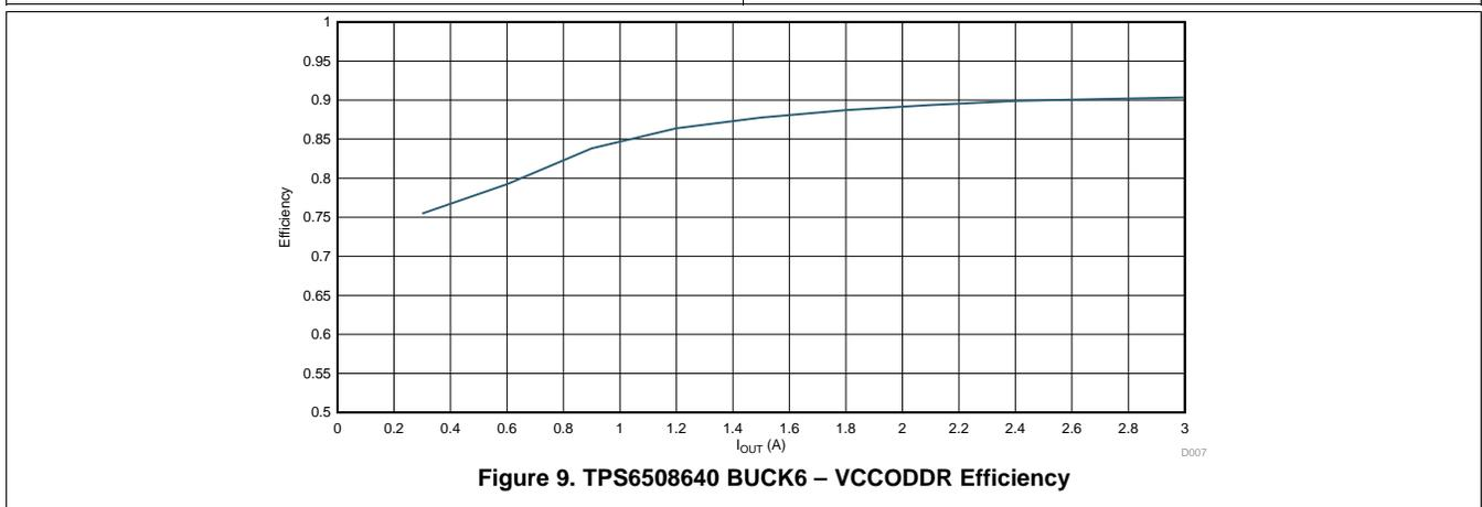
Figure 9. TPS6508640 BUCK6 – VCCODDR Efficiency
