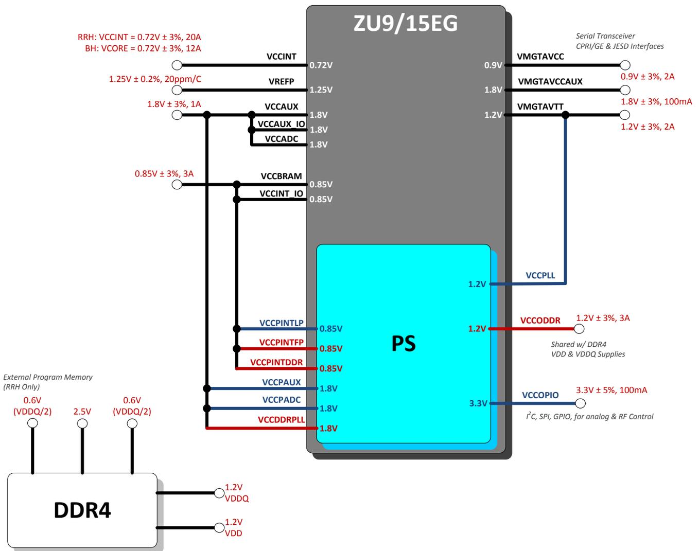
Figure 1. ZU9EG or ZU15EG RHH and Wireless BH DFE Power Supplies
