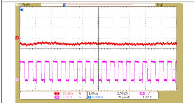
Figure 21. TPS6508640 BUCK5 – 1.8-V AUX Output Ripple
