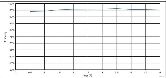
Figure 4. TPS6508640 BUCK1 – 3.3-V Efficiency
