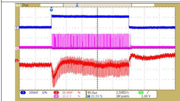
Figure 12. TPS6508640 BUCK2 – VCCPINT Load Transient
