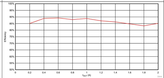
Figure 6. TPS6508640 BUCK3 – VMGTAVTT Efficiency
