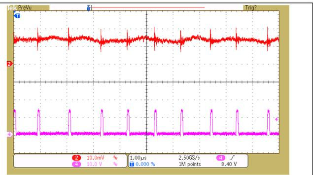
Figure 18. TPS6508640 BUCK2 – VCCPINT Output Ripple
