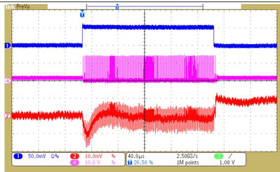
Figure 16. TPS6508640 BUCK6 – VCCODDR Load Transient
