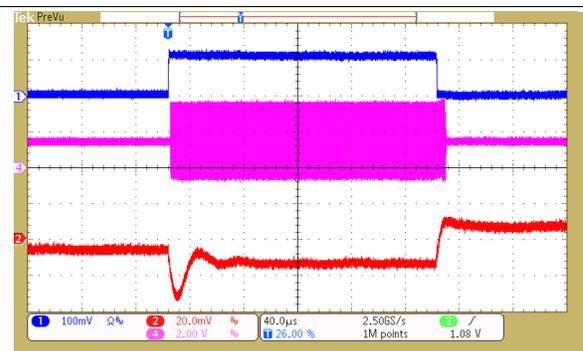
Figure 13. TPS6508640 BUCK3 – VMGTAVTT Load Transient
