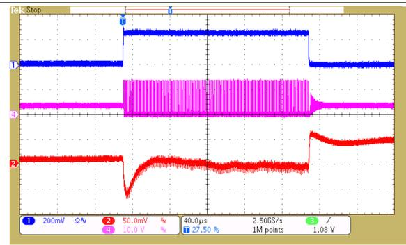
Figure 11. TPS6508640 BUCK1 – 3.3-V Load Transient
