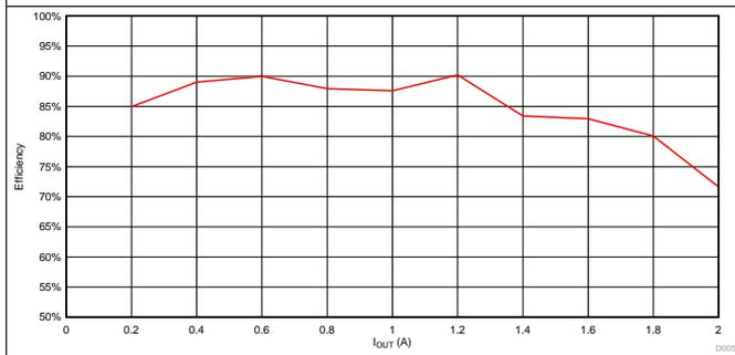
Figure 7. TPS6508640 BUCK4 – VMGTAVCC Efficiency
