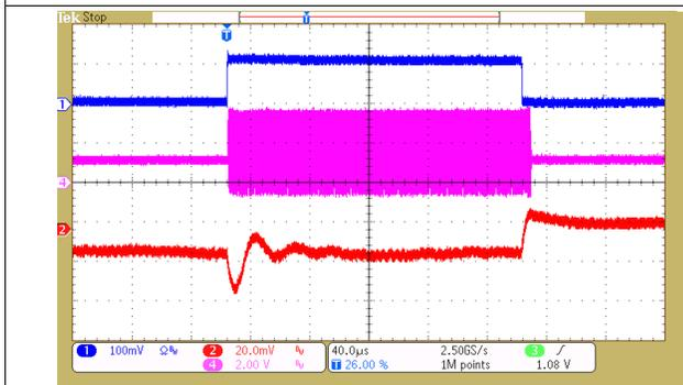
Figure 14. TPS6508640 BUCK4 – VMGTAVCC Load Transient
