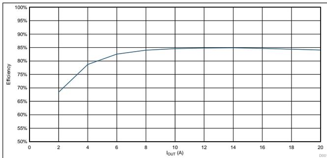
Figure 3. TPS544C25 – VCCINT Efficiency
