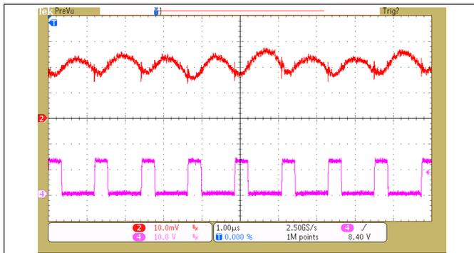
Figure 17. TPS6508640 BUCK1 – 3.3-V Output Ripple
