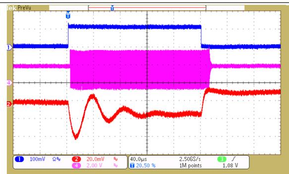
Figure 15. TPS6508640 BUCK5 – 1.8-V AUX Load Transient
