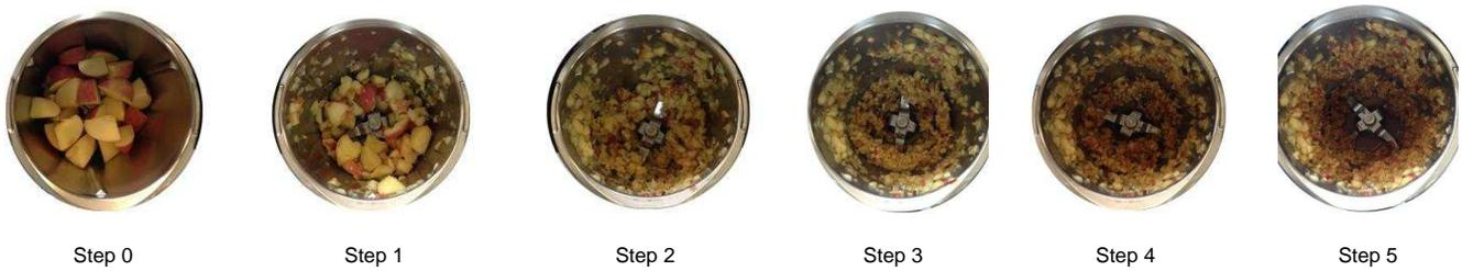
**Figure 39. Visual Feedback of Vibration Level versus Progress of Food Processing**
