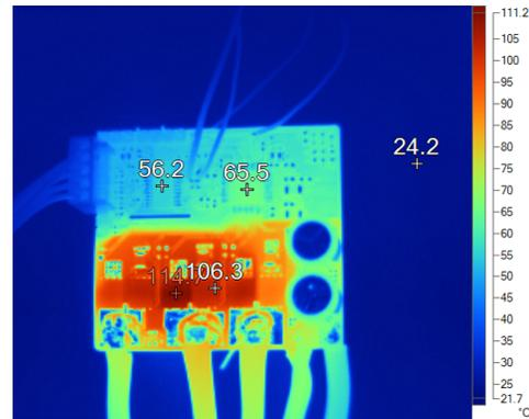
Figure 40. Thermal Image at 6-V DC Input, 25-A<sub>RMS</sub> Winding Current, 100% Duty Cycle
