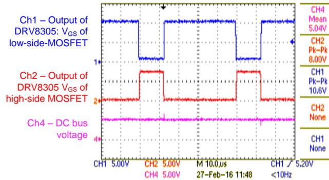
Figure 23. High-Side and Low-Side Gate Drive Output From DRV8305 at DC Input Voltage of 5 V
