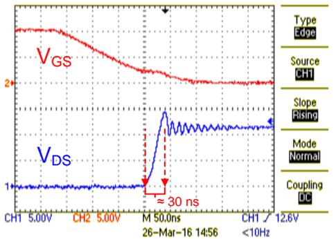
Figure 29. Low-Side FET Turn OFF Waveform (250-mA Sink Current)
