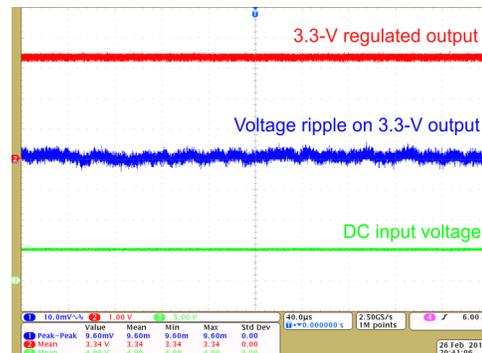
Figure 19. 3.3-V Regulator Output at 5-V DC Input
