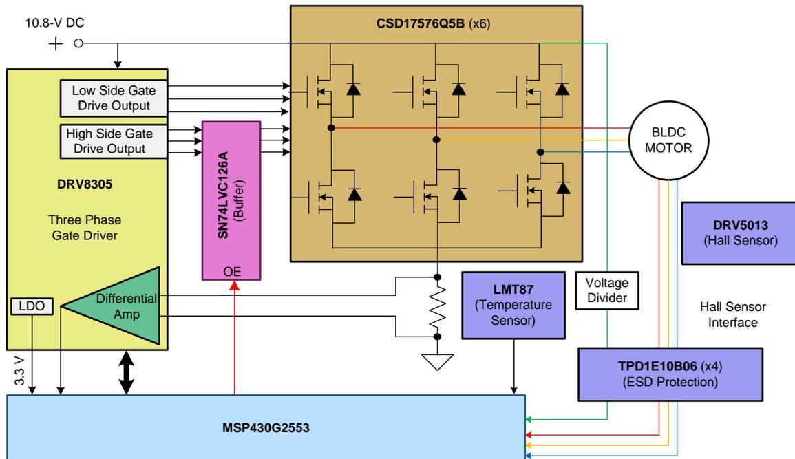
Figure 14. Block Diagram of TIDA-00771
