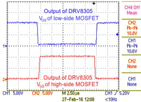
Figure 21. High-Side and Low-Side Gate Source Voltage From DRV8305
