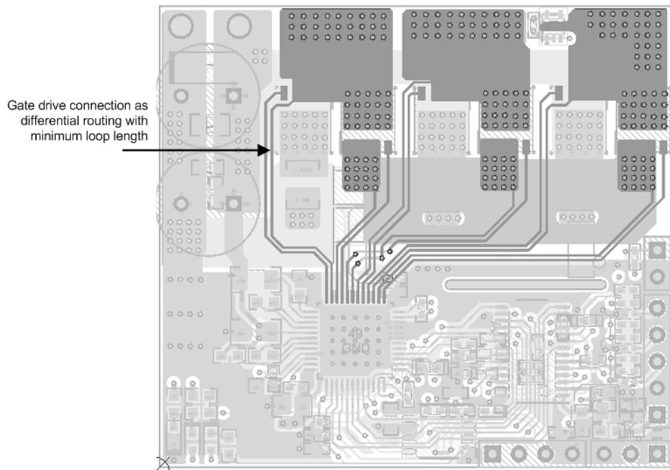
**Figure 67. Gate Drive Connection From DRV8305 as Differential Routing With Minimum Loop Length**
