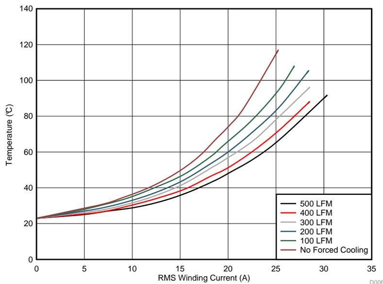
Figure 63. Maximum Steady State Temperature on MOSFETs With Different Airflow
