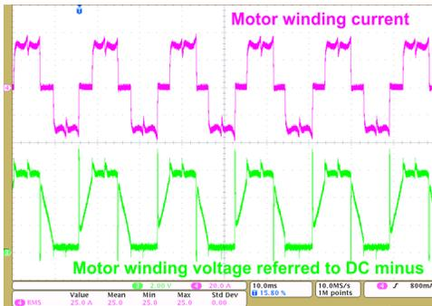
Figure 39. Load Test Results at 6-V DC Input, 25-A<sub>RMS</sub> Winding Current, 100% Duty Cycle
