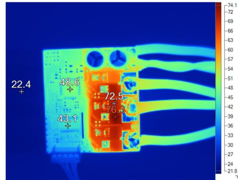
Figure 32. Thermal Image at 5-V DC Input, 20-A<sub>RMS</sub> Winding Current, 100% Duty Cycle
