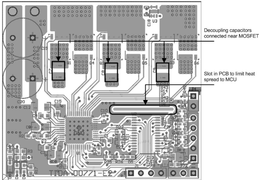
**Figure 69. Placement of Decoupling Capacitors for Inverter Legs**
