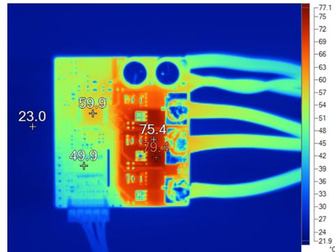
**Figure 36. Thermal Image at 12.6-V DC Input, 20-A<sub>RMS</sub> Winding Current, 100% Duty Cycle**
