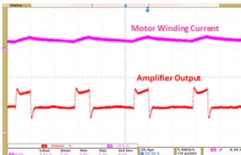
Figure 49. Amplifier Output Without Blanking
