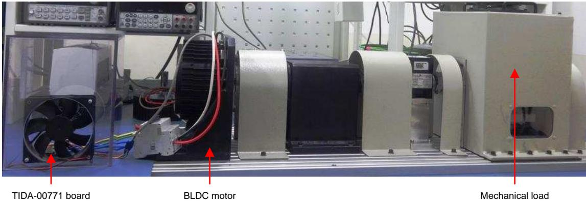
**Figure 17. Board and Motor Test Setup**
