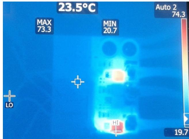
Figure 65. Thermal Image of Board After 1.4 Seconds With 73.6-A Peak Current in Motor Winding
