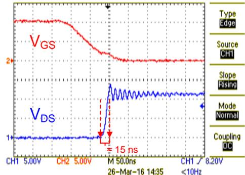
Figure 30. Low-Side FET Turn OFF Waveform (500-mA Sink Current)
