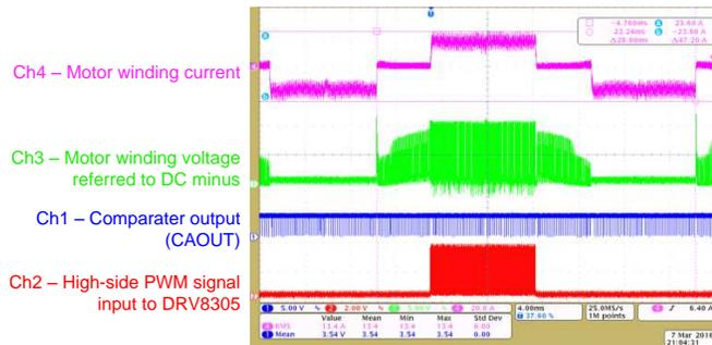
Figure 51. Cycle-by-Cycle Overcurrent Protection by Loading
