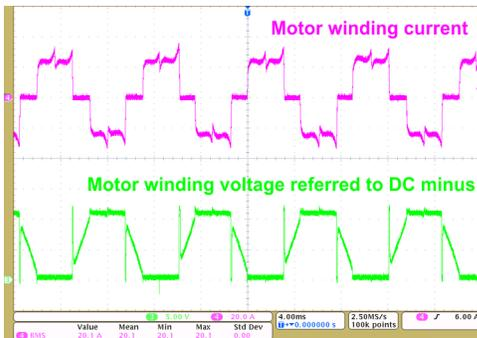
Figure 33. Load Test Results at 10.8-V DC Input, 20-A<sub>RMS</sub> Winding Current, 100% Duty Cycle
