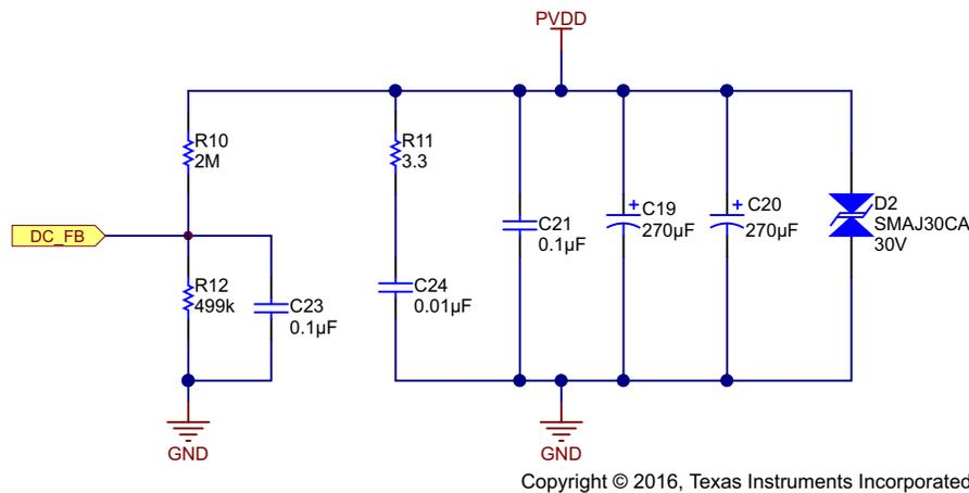
**Figure 2. Schematic of Battery Power Input Section**
