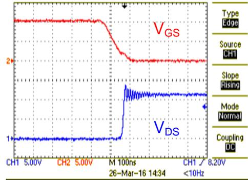
Figure 26. Low-Side FET Turn OFF Waveforms
