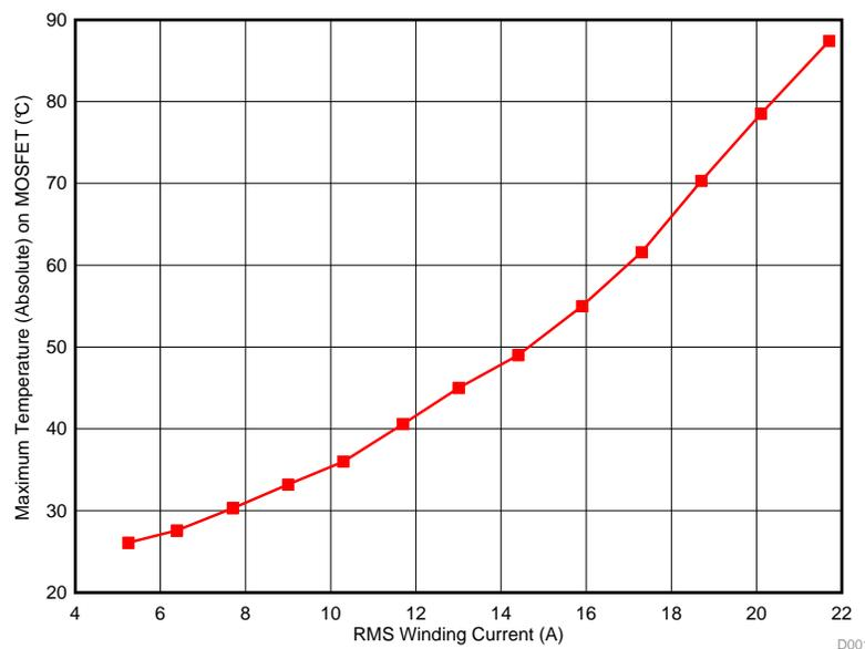
Figure 42. Maximum Steady State Temperature on FET With Different Winding Current
