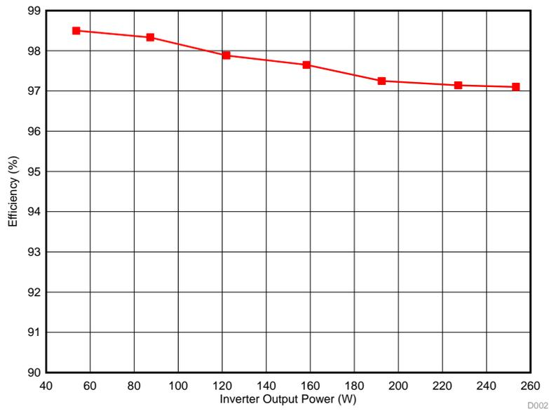
**Figure 43. Inverter Efficiency vs Output Power**
