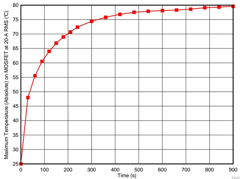
Figure 46. MOSFET Temperature Rise at 10.8-V DC Input, 20-A<sub>RMS</sub> Winding Current, 100% Duty Cycle
