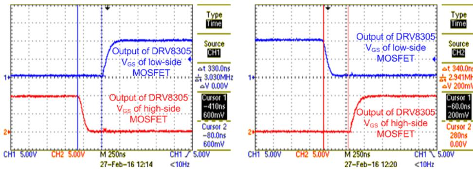
Figure 22. Dead Time Provided by DRV8305 at Both Edges of PWM
