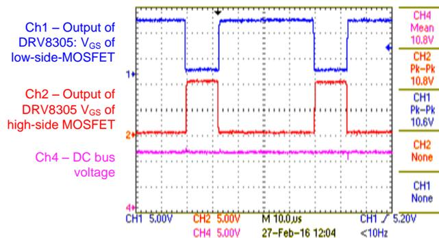
Figure 24. High-Side and Low-Side Gate Drive Output From DRV8305 at DC Input Voltage of 10.8 V
