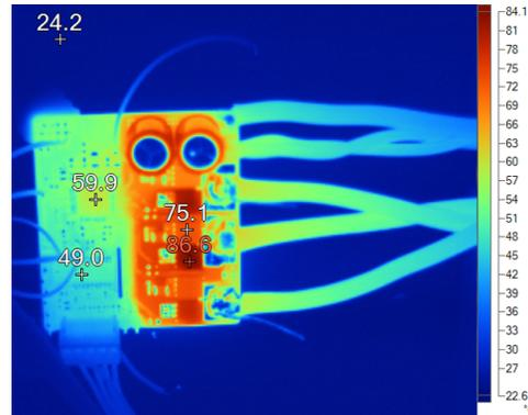
**Figure 38. Thermal Image at 10.8-V DC Input, 20-A<sub>RMS</sub> Winding Current, 50% Duty Cycle**
