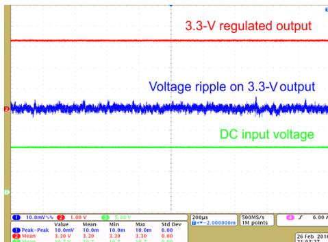
Figure 18. 3.3-V Regulator Output at 10.8-V DC Input
