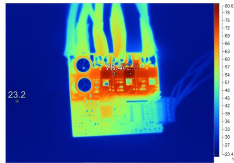
Figure 45. Steady State Thermal Image of Board When Gate Drive Source Current is Set at 125 mA and Sink Current is Set at 80 mA
