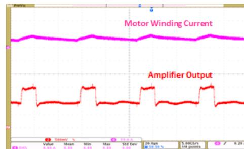
Figure 50. Amplifier Output With 500-ns Blanking
