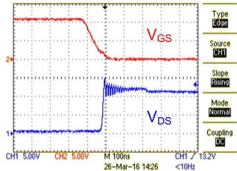
Figure 28. High-Side FET Turn OFF Waveforms
