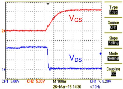
Figure 27. High-Side FET Turn ON Waveforms
