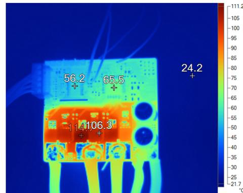
Figure 34. Thermal Image at 10.8-V DC Input, 20-A<sub>RMS</sub> Winding Current, 100% Duty Cycle
