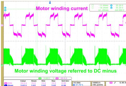
**Figure 37. Load Test Results at 10.8-V DC Input, 20-A<sub>RMS</sub> Winding Current, 50% Duty Cycle**
