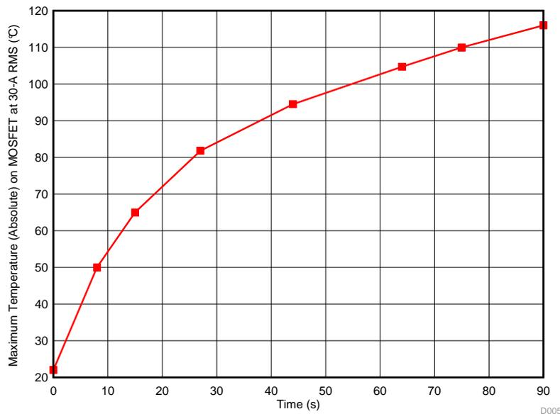
**Figure 48. MOSFET Temperature Rise at 10.8-V DC Input, 30- $A_{RMS}$  Winding Current, 100% Duty Cycle**
