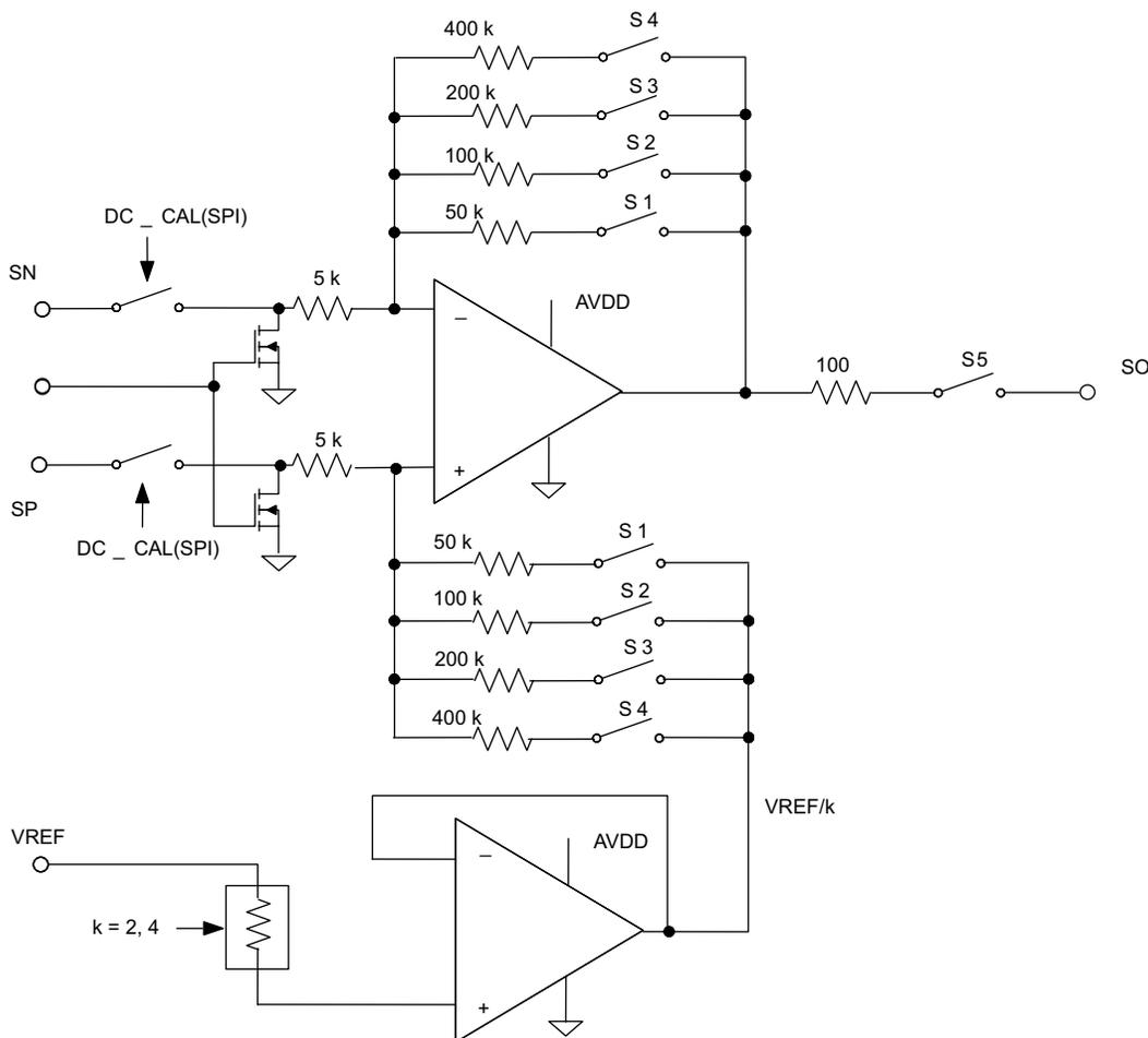
Figure 5. DRV8305 Current Shunt Amplifier Simplified Block Diagram
