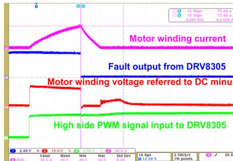
Figure 61. Overcurrent Latch Protection With Inverter Output Shorted
