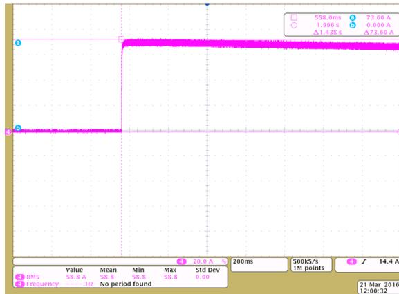
Figure 64. 73.6-A Peak Current in Motor Winding During Motor Stall
