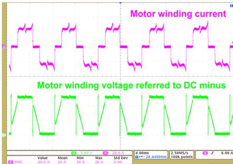
**Figure 35. Load Test Results at 12.6-V DC Input, 20-A<sub>RMS</sub> Winding Current, 100% Duty Cycle**
