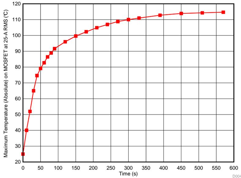
**Figure 47. MOSFET Temperature Rise at 10.8-V DC Input, 25- $A_{RMS}$  Winding Current, 100% Duty Cycle**
