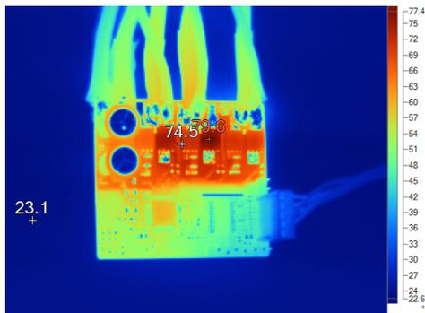
Figure 44. Steady State Thermal Image of Board When Gate Drive Source and Sink Current are Set to 1 A
