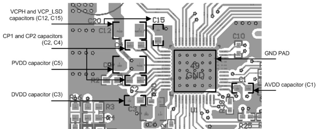
**Figure 66. Layout Recommendations for Decoupling Capacitors of DRV8305**
