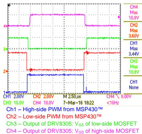
Figure 20. PWM Signals From MSP430G2553 and Corresponding Gate Drive Output From DRV8305
