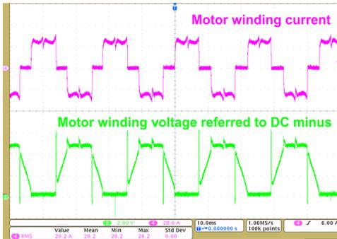
Figure 31. Load Test Results at 5-V DC Input, 20-A<sub>RMS</sub> Winding Current, 100% Duty Cycle
