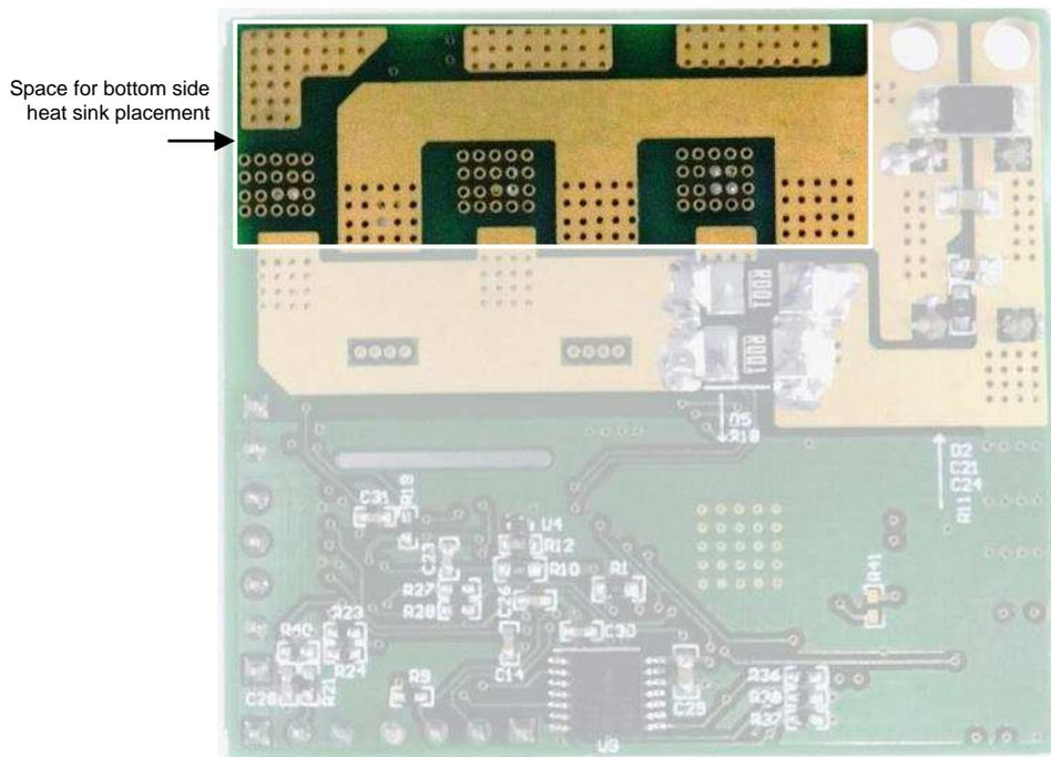
**Figure 70. Space for Bottom-Side Heat Sink**
