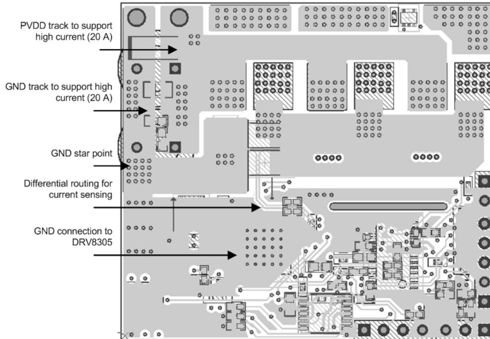
**Figure 68. Bottom Layer of PCB Showing Power Tracks and GND Star Connection**
