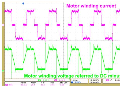
Figure 41. Load Test Results at 6-V DC Input, 30-A<sub>RMS</sub> Winding Current, 100% Duty Cycle
