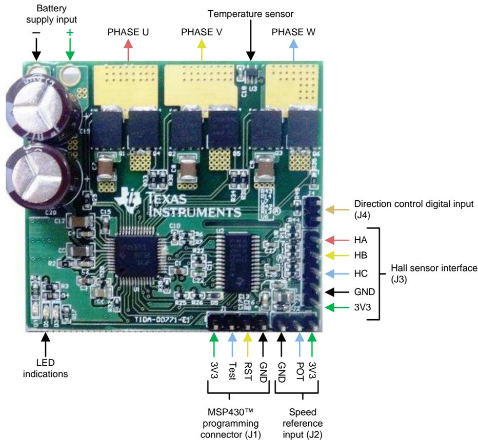
Figure 15. TIDA-00771 PCB Connectors
