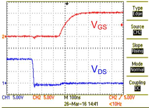
Figure 25. Low-Side FET Turn ON Waveforms
